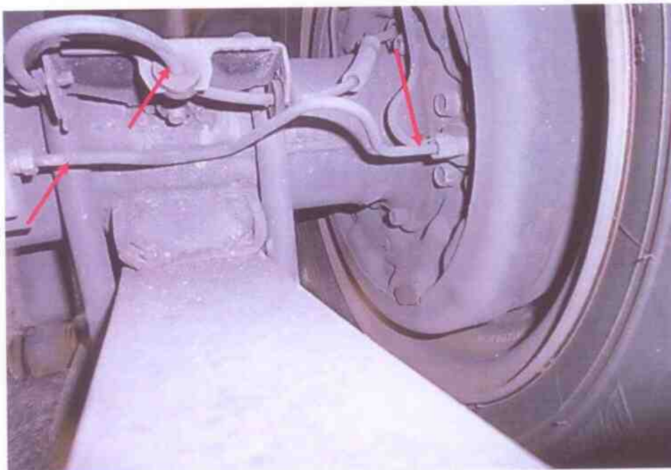
Photo 17 shows the brake pipe (arrowed) at the left rear wheel of the Motor Lorry. We did not observe any leakage of brake fluid at the time of our inspection of the Motor Lorry. Our static tests had indicated that there was no internal leakage of pressure/vacuum. Hence the braking system of the Motor Lorry was likely to be in serviceable condition at the material time of accident.
