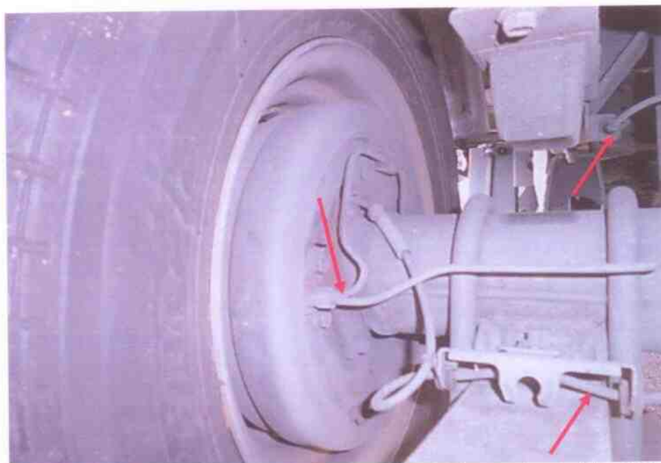
Photo 18 shows the brake pipe (arrowed) at the right rear wheel of the Motor Lorry. We did not observe any leakage of brake fluid at the time of our inspection of the Motor Lorry. Our static tests had indicated that there was no internal leakage of pressure/vacuum. Hence the braking system of the Motor Lorry was likely to be in serviceable condition at the material time of accident.
