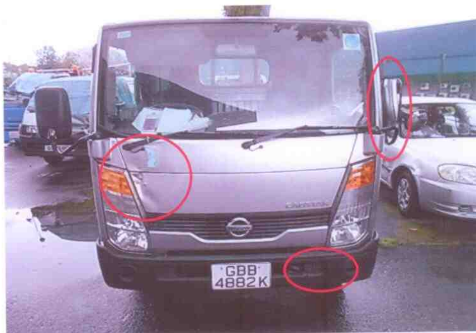
Photo 2 shows The Motor Lorry was observed to have sustained relatively minor damages at its front right panel, front right wiper panel, front left lower bumper, front left side mirror (tilt inwards) and front right fender were amongst the body parts that were damaged as a result of the accident (circled).
