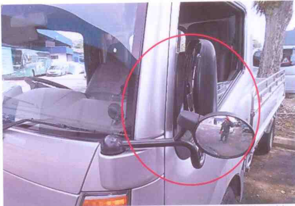
Photo 5 shows the damage sustained on the front left wing mirror (tilt inwards) as a result of the accident.
