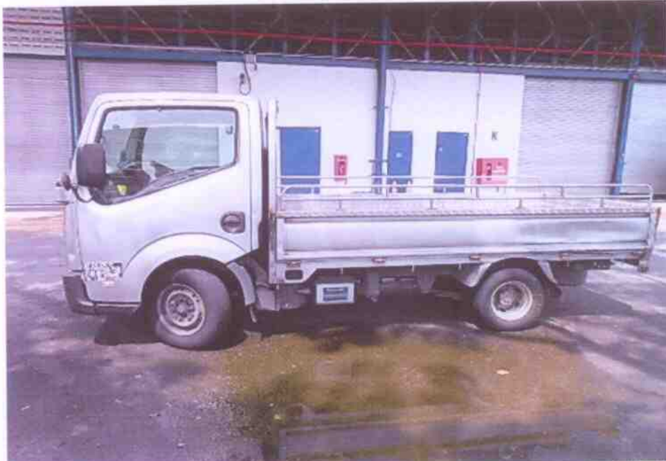
Photo 19 shows the front left wheel of the Motor Lorry turned to its full left. During our steering system test, we did not experience any abnormal free play and/or resistance when we had turned the steering wheel towards full left and full right.
