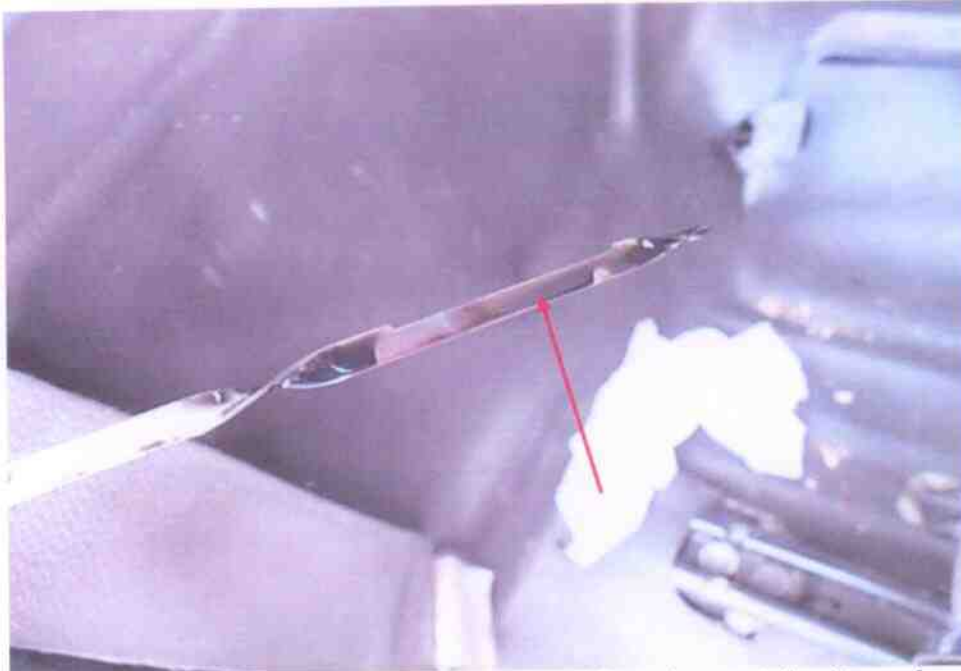
Photo 16 shows the engine dip stick of the Motor Lorry at the time of our inspection. The engine oil was observed to be of sufficient level and without any visible contamination (arrowed).
