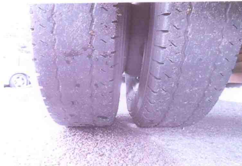
Photo 12 shows the condition of the rear right tyres of the Motor Lorry, which were observed to be in serviceable condition with remaining tread depth of approximately 1.6mm. There was also no tear, cut or burst mark(s) on the outer and the inner sidewalls.
