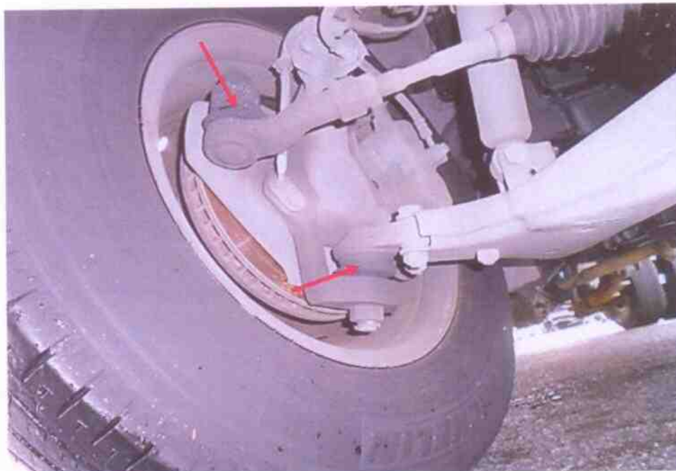
Photo 20 shows the various undercarriage components at the front right wheel of the Motor Lorry, in particular the steering tie rod end (arrowed). The various steering components were all found to be intact. There was also no sign of fluid stain(s) observed on the various undercarriage components.
