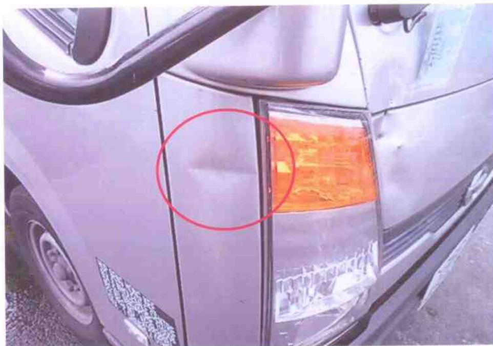
Photo 7 shows the damage sustained on the front right fender as a result of the accident.
