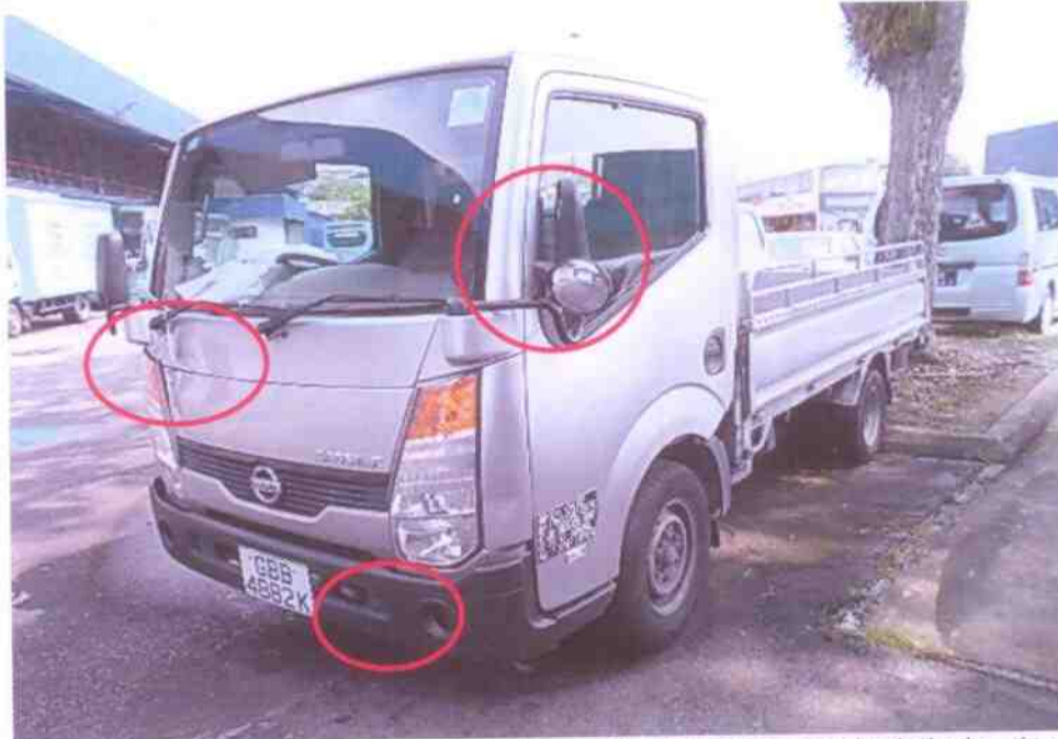
Photo 3 shows The Motor Lorry was observed to have sustained relatively minor damages at its front right panel, front right wiper panel, front left lower bumper, front left side mirror (tilt inwards) and front right fender were amongst the body parts that were damaged as a result of the accident (circled).
