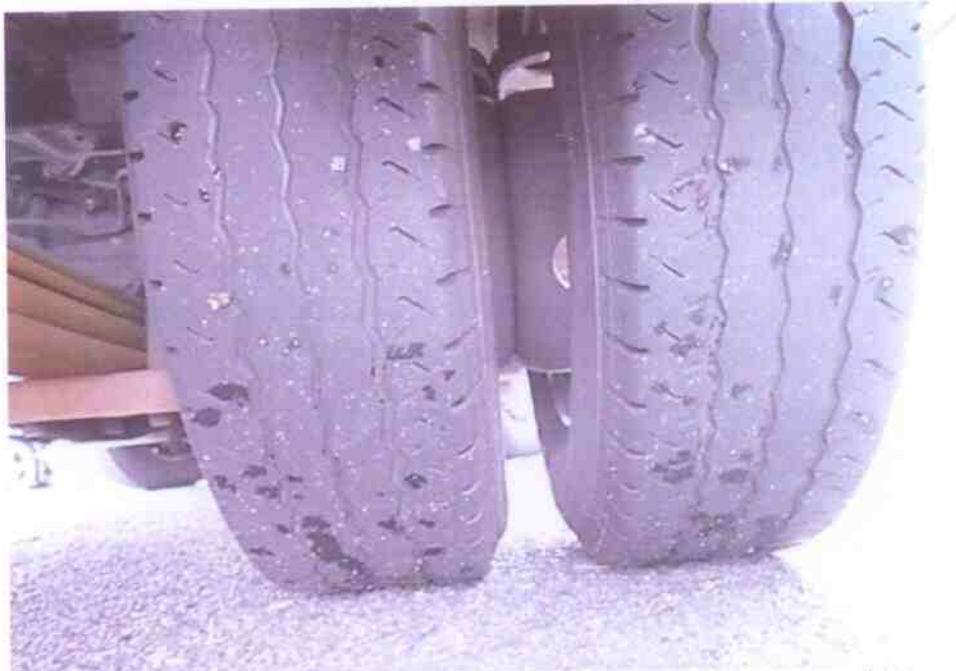
Photo 11 shows the condition of the rear left tyres of the Motor Lorry, which was observed to be in serviceable condition with remaining tread depth of approximately 1mm. The tyres, which were wrapped around standard alloy wheel rim, were also observed to be sufficiently inflated for vehicular operation.
