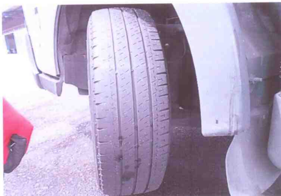
Photo 10 shows the condition of the front right tyre of the Motor Lorry, which was observed to be in serviceable condition with remaining tread depth of approximately 5mm. The tyre, which was wrapped around standard alloy wheel rim, was also observed to be sufficiently inflated for vehicular operation.
