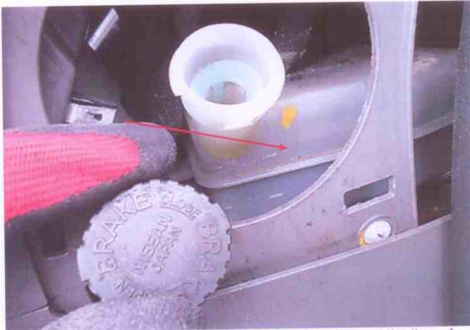
Photo 14 shows the brake fluid reservoir of the Motor Lorry at the time of our inspection. The brake fluid was observed to be of sufficient level and without any visible contamination.
