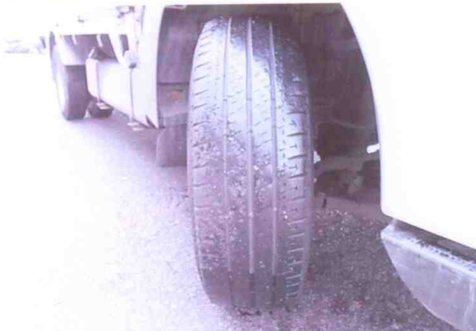
Photo 9 shows the condition of the front left tyre of the Motor Lorry, which was observed to be in serviceable condition with remaining tread depth of approximately 4mm. The tyre, which was wrapped around standard alloy wheel rim, was also observed to be sufficiently inflated for vehicular operation. There was no tear, cut or burst mark(s) on the outer and the inner sidewalls.
