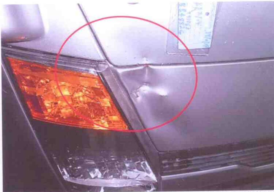
Photo 6 shows the damage sustained on the front right panel & wiper panel as a result of the accident.
