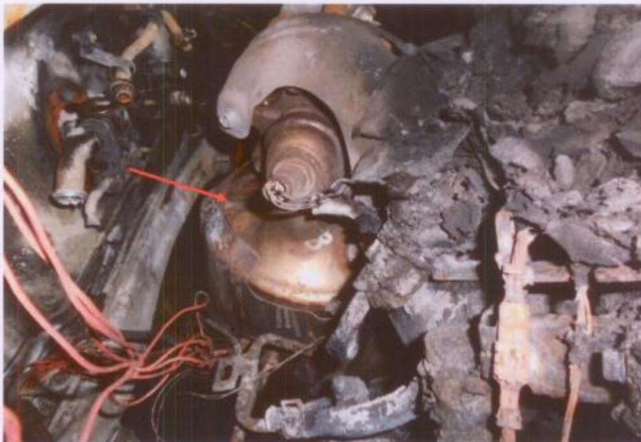
Photo 11 shows the DPF (Diesel Particulate Filter) of the Motor Taxi (arrowed). Although the DPF was located in the immediate vicinity of where the fire to the Motor Taxi had originated. The exterior surfaces of the exhaust manifold and the DPF both did not contain any sign(s) of being directly exposed to high heat intensity (whitish burn marks) that could have suggested that fluid had leaked onto the hot surfaces of the exhaust pipes to cause the fluid to self-ignite.
