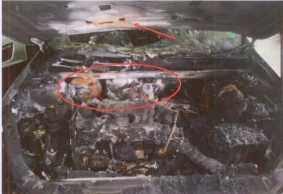
Photo 6 shows the approximate location of where the fire had originated. This was around the rear right area of the engine compartment (circled), as determined from the rust that had developed on the underside of the Motor Taxi's front bonnet (arrowed). The development of rust is a consequence of that area being exposed to prolong high heat intensity, where such exposure usually causes the steel/metal material body parts to be exposed to natural environmental condition.
