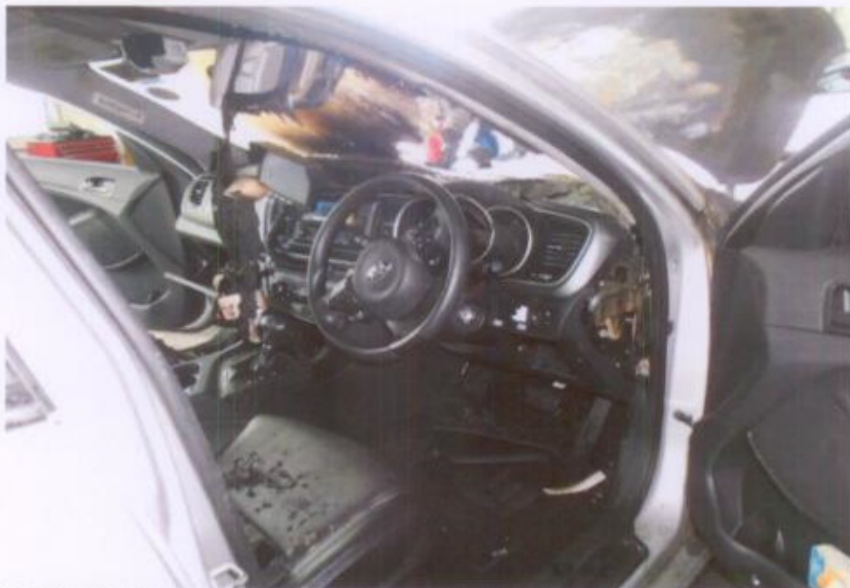
Photo 4 shows the interior compartment of the Motor Taxi at the time of inspection. Parts towards the front area of the interior compartment were found to be burnt and/or partially melted as a result of the fire. This had included the dashboard, upholstery and carpet amongst others.
