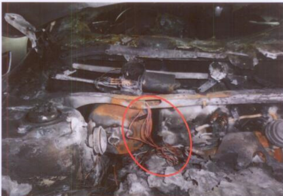
Photo 7 shows the wirings around the rear right of the engine compartment, which was where the fire to the Motor Taxi had likely started. The wirings (circled) were found to have been burnt internally to its bare copper state, suggesting occurrence of an electrical short circuit.
