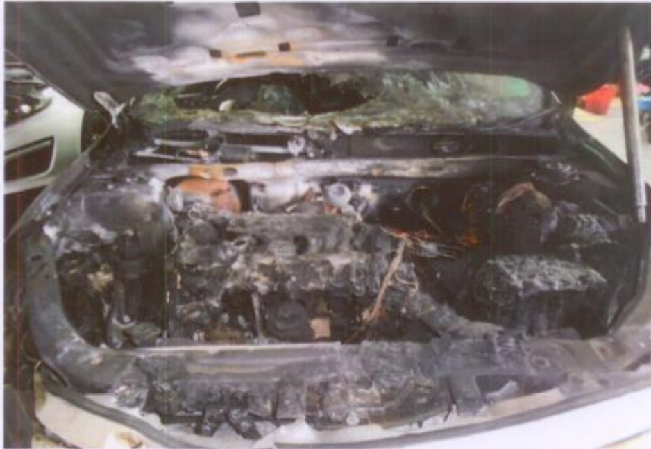
Photo 3 shows the engine area of the Motor Taxi at the time of inspection. Almost all the parts inside the engine compartment were observed to be completely burnt and/or melted as a result of the fire. This had included its radiator, cooling fan, engine housing, fuel rail, brake booster and fuse box amongst others.
