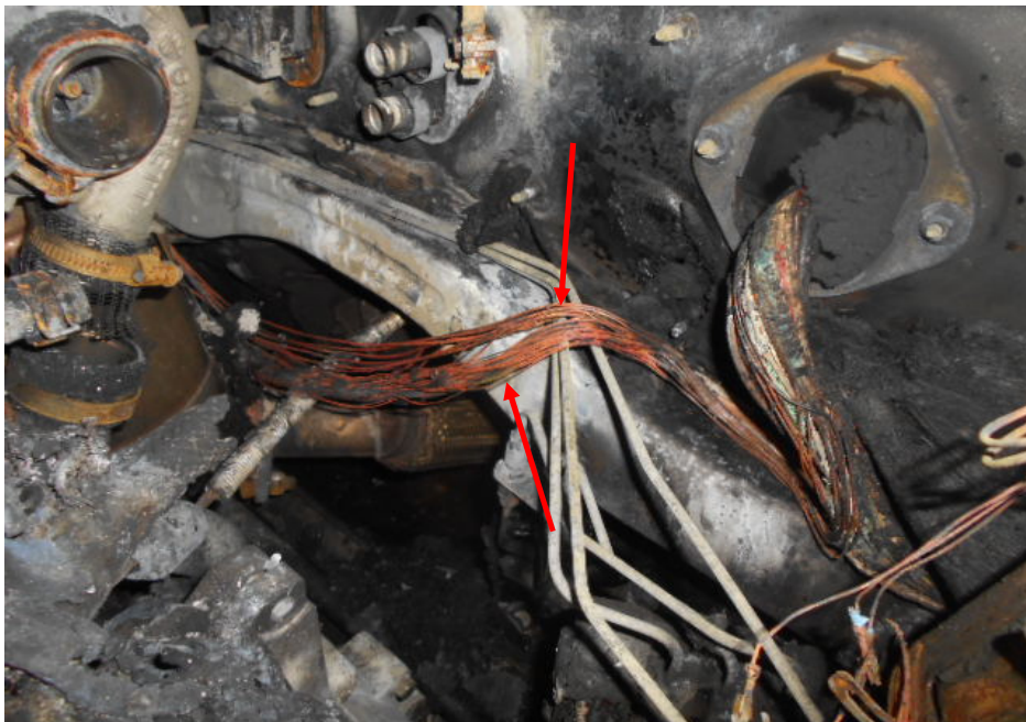
Photo 8 shows another stretch of wirings around the rear of the engine compartment, which was in the immediate vicinity where the fire to the Motor Taxi had likely started. The wirings were found to have been burnt internally to its bare copper state, suggesting occurrence of an electrical short circuit.
