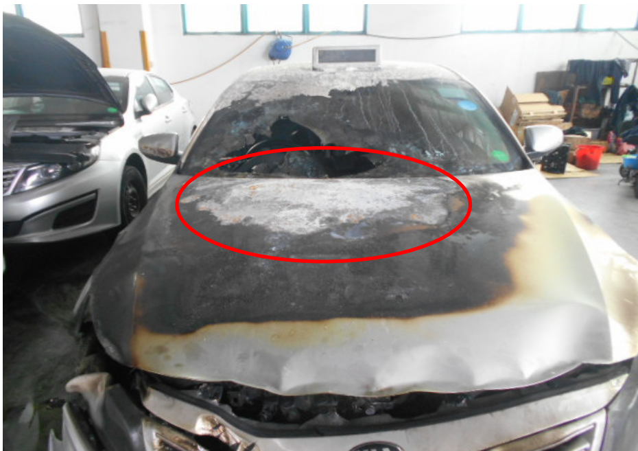
Photo 5 shows the whitish burn marks (circled) that were found on the top side of the Motor Taxi's front bonnet. Such whitish burn marks are a result of exposure to prolonged heat intensity, which may indicate where the fire had started. Rust would also begin to develop on these areas soon after the fire.
