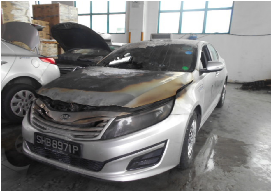
Photo 1 shows a general view of the front left body of the Motor Taxi at the time of inspection. The Motor Taxi was observed to have been severely burnt at its frontal portion. Its front bumper, front bonnet, front grille, front left headlamp, front left fender, roof panel and front windscreen were amongst the body parts that were found to have been affected as a result of the fire.
