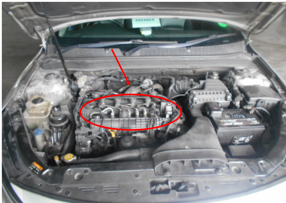
Photo 9 shows the engine layout of a similar make and model motor taxi as the Motor Taxi. The fuel rail and fuel injectors were located towards the front area of the engine compartment (circled), away from the hot surfaces of the exhaust manifold and the DPF, which are both located towards the rear of the engine compartment (arrowed).
