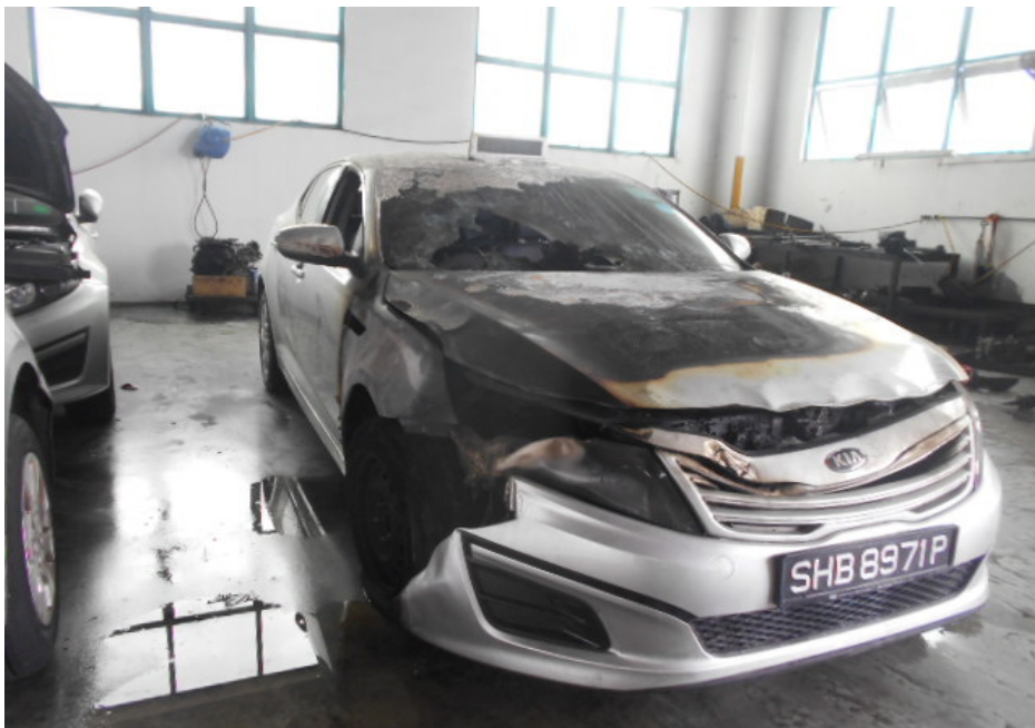
Photo 2 shows a general view of the front right body of the Motor Taxi at the time of inspection. The Motor Taxi was observed to be severely burnt at its frontal portion. Its front bumper, front bonnet, front right headlamp, front right fender, roof panel and right side wing mirror were amongst the body parts that were found to have been affected as a result of the fire.
