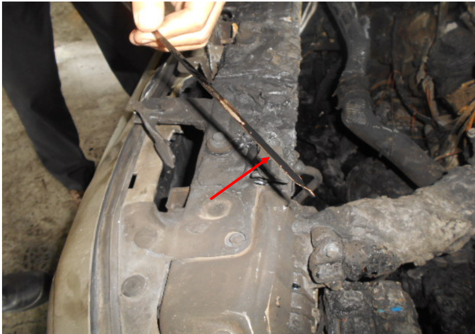
Photo 10 shows the engine oil dip stick of the Motor Taxi. The engine oil of the Motor Taxi was found to be of sufficient level (arrowed) for operating purposes, indicating no leakage of engine oil. In general, there appears to be no sign(s) or indication(s) to suggest that the Motor Taxi had experienced fluid leakage prior to the fire incident. Cause of fire being due to fluid leakage would then be unlikely.
