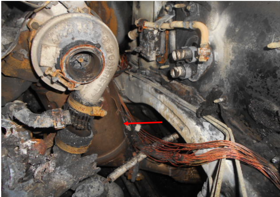
Photo 12 shows the DPF (Diesel Particulate Filter) of the Motor Taxi (arrowed). Although the DPF was located in the immediate vicinity of where the fire to the Motor Taxi had originated. The exterior surfaces of the exhaust manifold and the DPF both did not contain any sign(s) of being exposed to high heat intensity (whitish burn marks) that could have suggested that fluid had leaked onto the hot surfaces of the exhaust pipes to cause the fluid to self-ignite.
