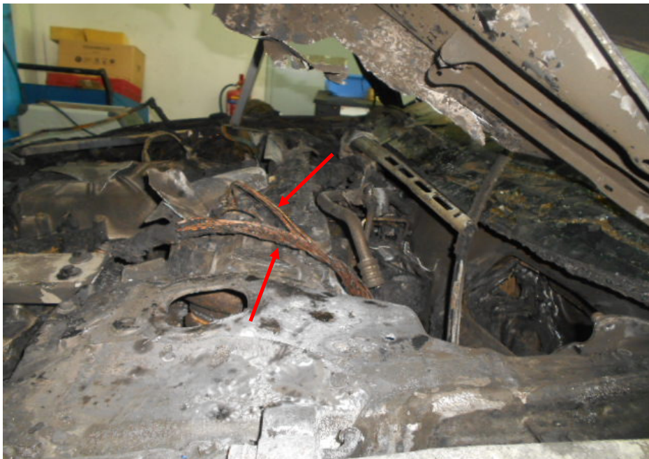
Photo 7 shows the wirings at the left rear area of the Insured Vehicle's engine compartment. The wirings (arrowed) were found to be completely burned to its bare copper state. The bright reddish colour of the copper wires suggest that the wirings were exposed to high heat. Such condition normally indicate internal heating of copper wires which is a sign of an electrical short circuit occurring. The wires were likely to be original wire harnesses of the Insured Vehicle.
