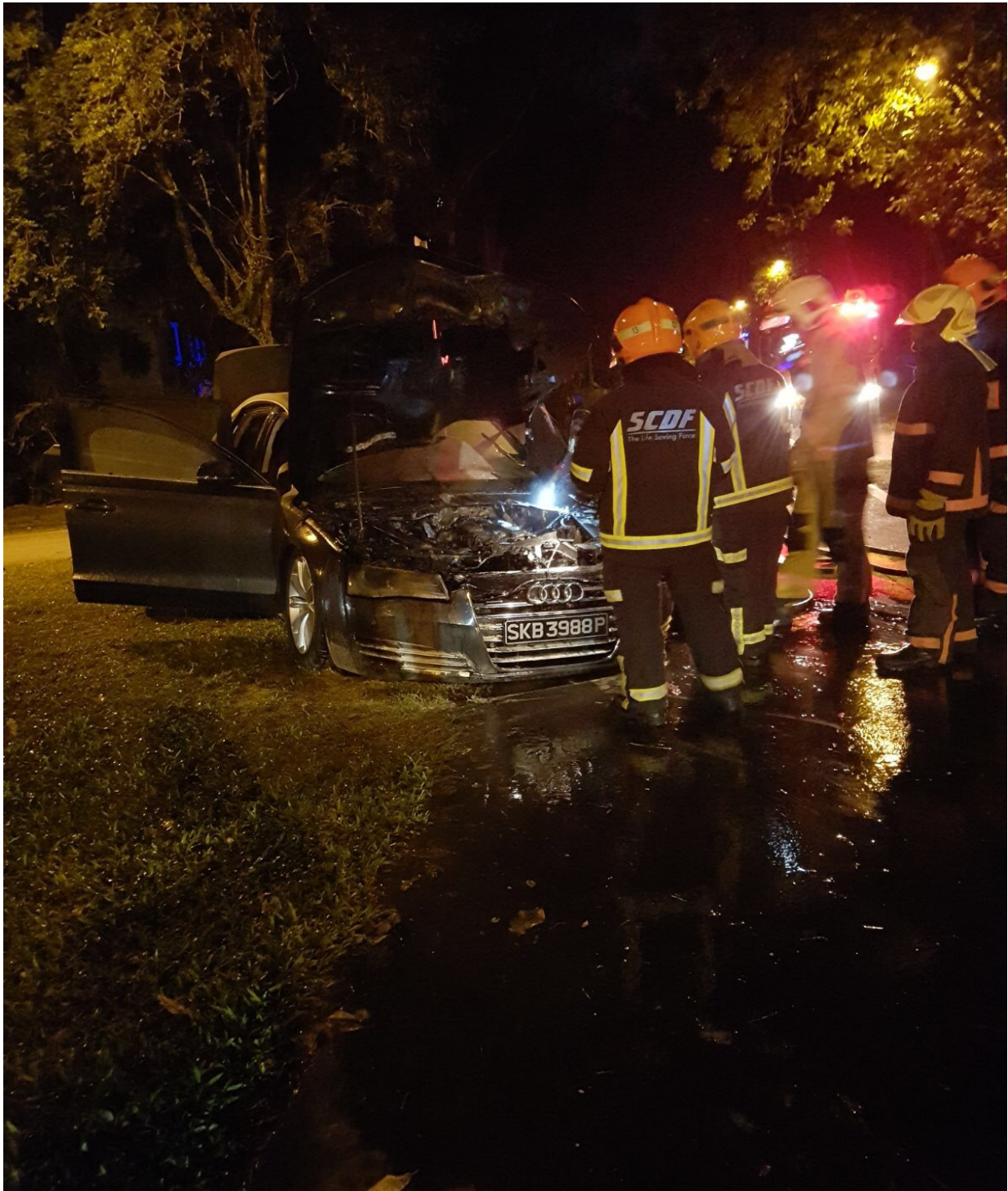
Photo 6 shows the Insured Vehicle at the incident scene after the fire was extinguished. SCDF officers could be seen examining the left side of the engine compartment. The left front side of the Insured Vehicle was where smoke was first detected by the driver of the Insured Vehicle and also where flames were first seen by another driver.
