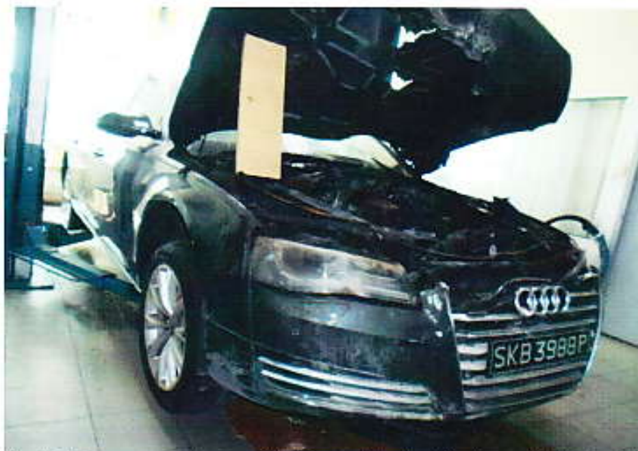
Photo 1 shows a general view of the front right body of the Insured Vehicle at the time of inspection. The Insured Vehicle was observed to be severely burnt at its front body. Its front bumper, front bonnet, front grille, front right headlamp and front right fender were amongst the body parts that were found to have been affected as a result of the fire.
