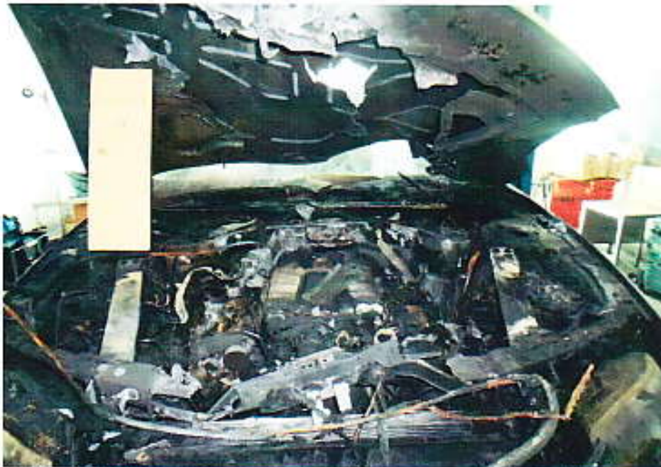
Photo 3 shows the engine compartment of the Insured Vehicle at the time of inspection. Almost all the parts inside the engine area were observed to be burnt and/or melted as a result of the fire. These parts had included its radiator, air condenser, cooling fan, intake manifold, front bonnet absorbers, air duct, hoses and pipes amongst others.
