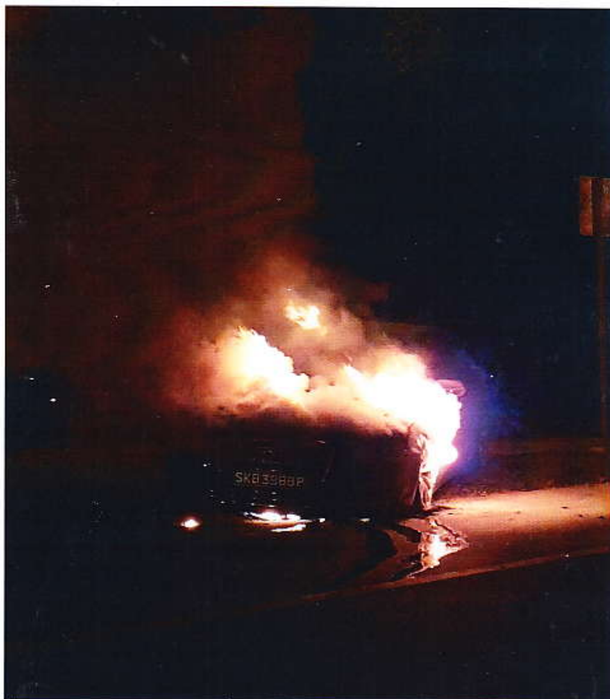
Photo 5 shows the Insured Vehicle at the incident scene with flames engulfing its left front body. Trails of fluid could be seen on the ground beneath the front left side, and in front of the Insured Vehicle. These leaked fluid were unlikely the source of fire as the fluid were not combusted. There was also no unusual foreign material(s) and/or object(s) on the ground in the immediate area of where the Insured Vehicle was parked.
