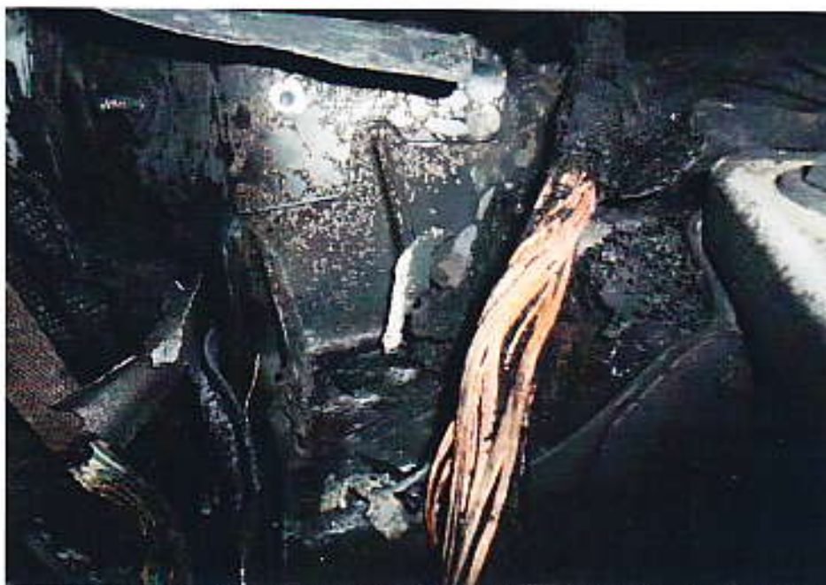
Photo 9 shows a closer view of another stretch of wirings at the left rear area of the Insured Vehicle's engine compartment. The bright reddish colour of the copper wires suggest that the wirings were exposed to high heat. Such condition normally indicate internal heating of copper wires which is a sign of an electrical short circuit occurring. This would then appear to suggest that the cause of fire to the Insured Vehicle could have possibly been due to electrical in nature.
