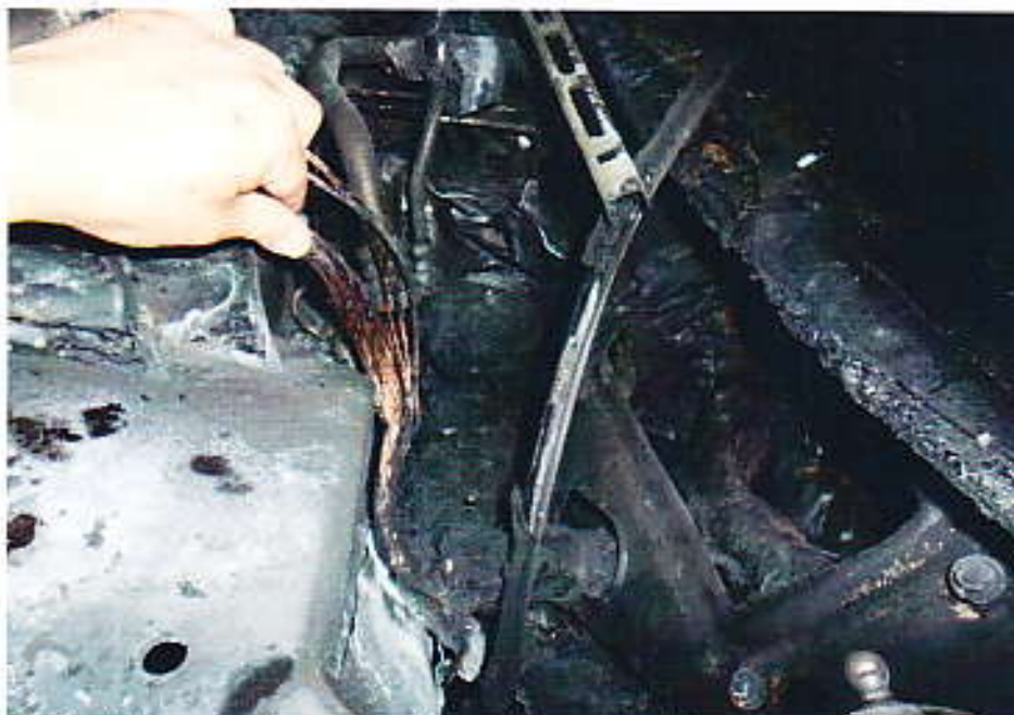
Photo 8 shows a closer view of the wirings at the left rear area of the Insured Vehicle's engine compartment. The wirings were found to be completely burned to its bare copper state. Such condition normally indicate internal heating of copper wires which is a sign of an electrical short circuit occurring.
