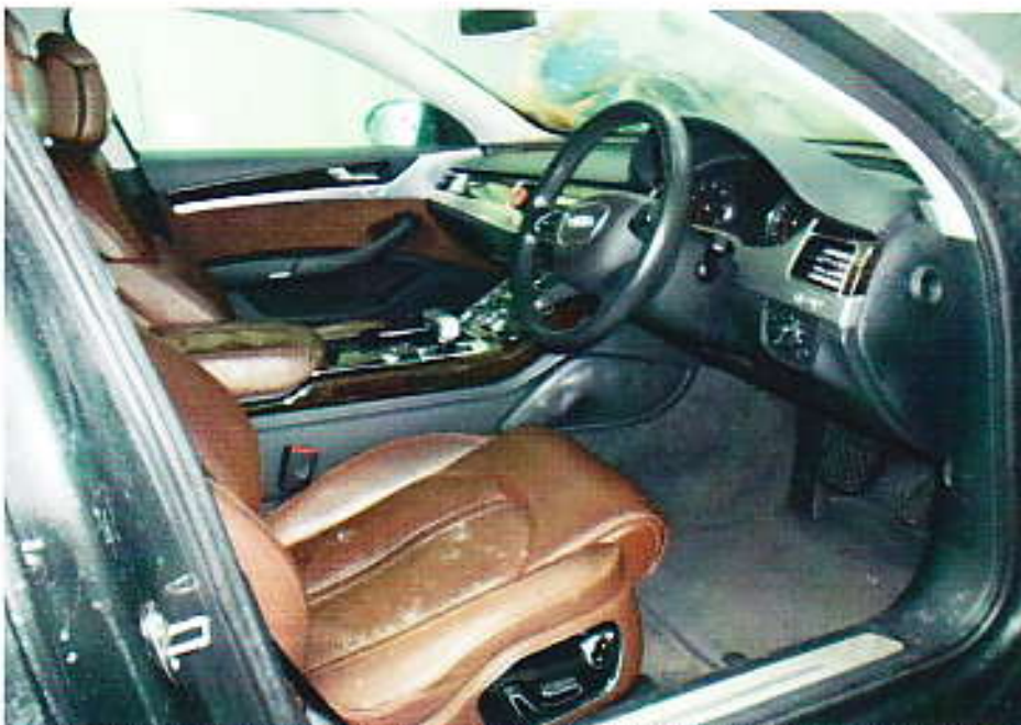
Photo 4 shows the interior compartment of the Insured Vehicle at the time of inspection. The interior compartment and rear body of the Insured Vehicle was unaffected by the fire.
