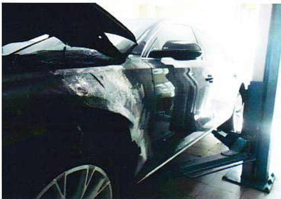
Photo 2 shows a general view of the front left body of the Insured Vehicle at the time of inspection. The Insured Vehicle was observed to be severely burnt at its front body. Its front left fender, front left wheel rim, front left tyre, front bonnet and front windscreen were amongst the body parts that were found to have been burnt and/or melted as a result of the fire.
