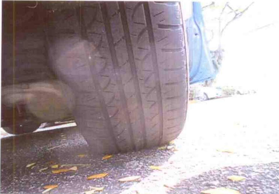
Photo 10 shows the condition of the rear right tyre of the Motor Taxi, which was observed to be in serviceable condition with remaining tread depth of approximately 4mm.
