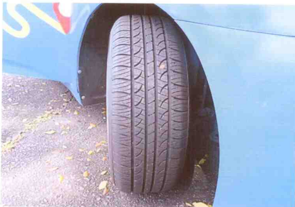
Photo 7 shows the condition of the front right tyre of the Motor Taxi, which was observed to be in serviceable condition with remaining tread depth of approximately 7mm. There was no tear, cut or burst mark(s) on the outer and the inner sidewalls.
