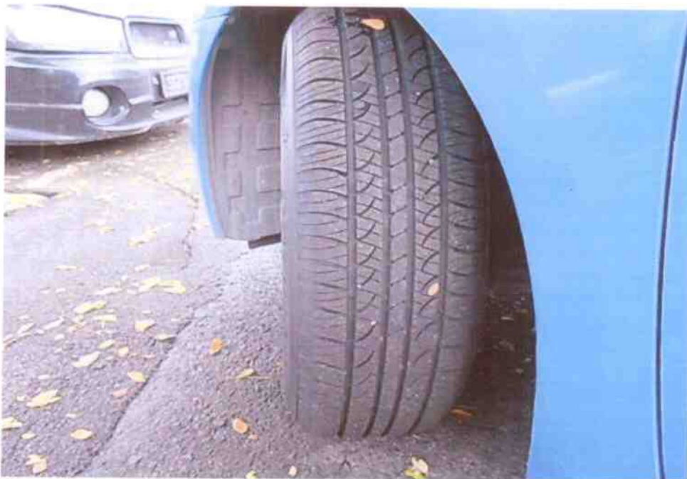
Photo 8 shows the condition of the front left tyre of the Motor Taxi, which was observed to be in serviceable condition with remaining tread depth of approximately 7mm. The tyre, which was wrapped around alloy wheel rim, was also observed to be sufficiently inflated for vehicular operation.
