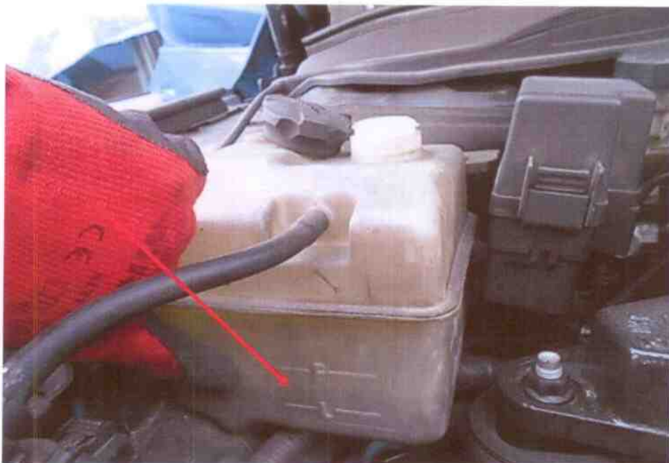
Photo 13 shows the engine coolant fluid reservoir of the Motor Taxi at the time of our inspection. The engine coolant fluid was observed to be of sufficient level and without any visible contamination.
