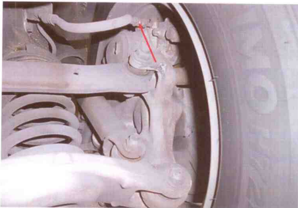
Photo 16 shows the brake hose (arrowed) at the rear right wheel of the Motor Taxi. We did not observe any leakage of brake fluid at the time of our inspection of the Motor Taxi. Our visual inspection of the various mechanical components of the Motor Taxi's braking system revealed all to be intact without visible damage.
