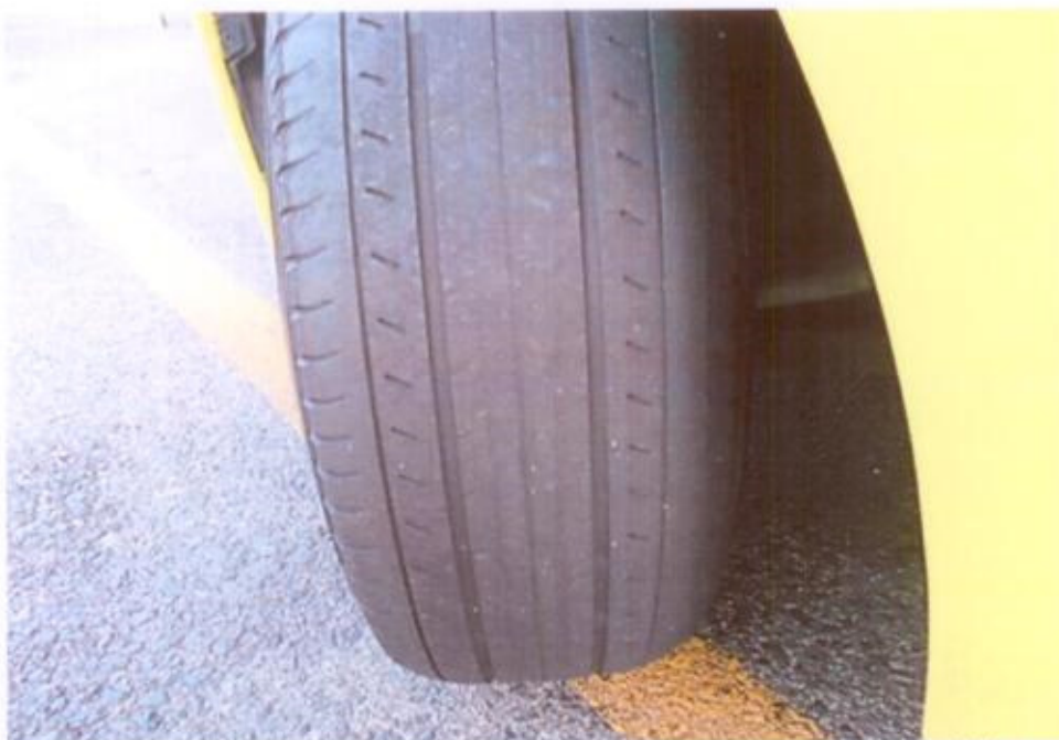
Photo 11 shows the condition of the front left tyre of the Motor Taxi, which was observed to be in serviceable condition with remaining tread depth of approximately 4mm. The tyre, which was wrapped around alloy wheel rim, was also observed to be sufficiently inflated for vehicular operation.
