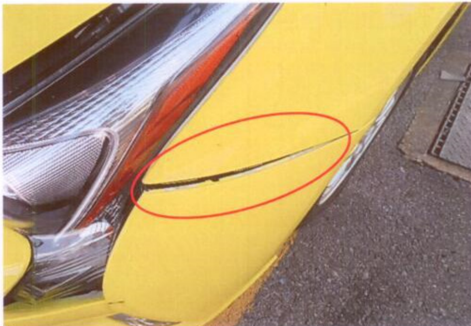
Photo 6 shows a close up view of the front bumper of the Motor Taxi at the time of our inspection. The Motor Taxi had sustained relatively minor impact at the front bumper of the Motor Taxi.
