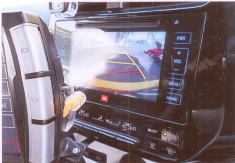
Photo 24 shows reverse sensor camera on the LCD panel of the Motor Taxi while performing operational test. This would suggest that it was able to move forward and backward normally.
