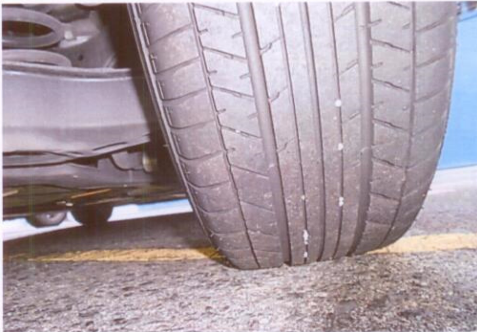
Photo 13 shows the condition of the rear right tyre of the Motor Taxi, which was observed to be in serviceable condition with remaining tread depth of approximately 5mm. There was also no tear, cut or burst mark(s) on the outer and the inner sidewalls as well as across the tread of the 4 tyres.
