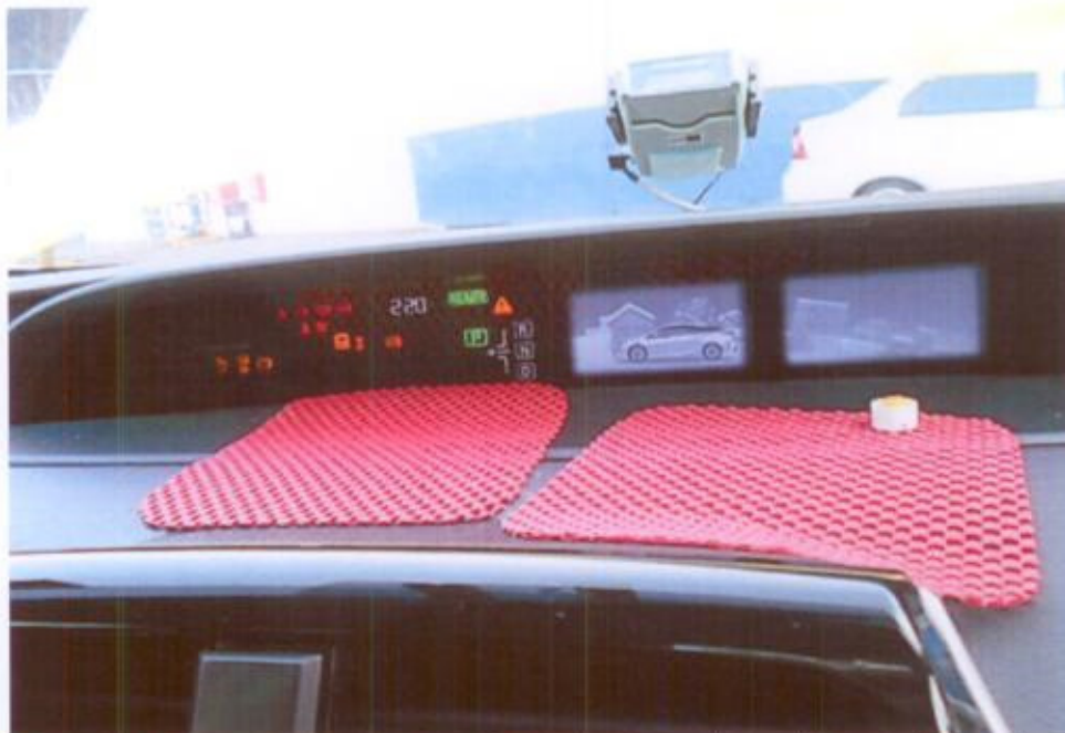
Photo 22 shows the warning lights for the various electronic operating systems of the Motor Taxi appearing on its instrument panel during the self-test when the engine is cranked, in particular the ABS light and SRS light.
