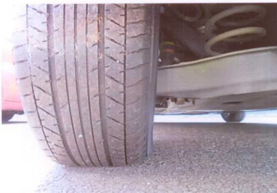
Photo 12 shows the condition of the rear left tyre of the Motor Taxi, which was observed to be in serviceable condition with remaining tread depth of approximately 5mm. The tyre, which was wrapped around alloy wheel rim, was also observed to be sufficiently inflated for vehicular operation.
