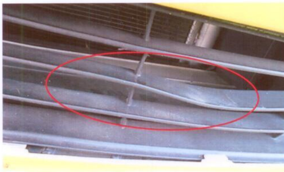
Photo 7 shows a close up view of the lower bumper of the Motor Taxi at the time of our inspection. The Motor Taxi had sustained relatively minor impact at the lower bumper of the Motor Taxi.
