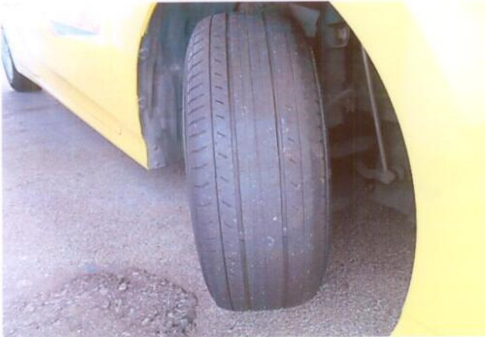
Photo 10 shows the condition of the front right tyre of the Motor Taxi, which was observed to be in serviceable condition with remaining tread depth of approximately 3mm. There was no tear, cut or burst mark(s) on the outer and the inner sidewalls.
