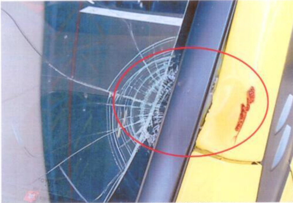
Photo 5 shows a close up view of the windshield & left hand door outer pillar of the Motor Taxi at the time of our inspection. It was observed to have sustained relatively minor impact at the highlighted area of the Motor Taxi.
