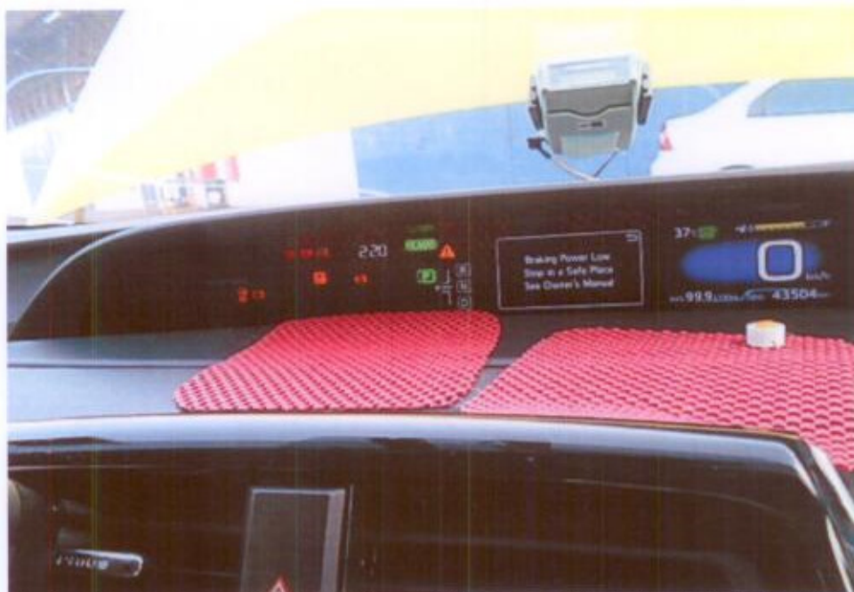
Photo 23 shows no warning lights illuminated on the instrument panel of the Motor Taxi after the engine was cranked. This would suggest that there was no abnormality to the various electronic operating systems of the Motor Taxi, like the ABS and SRS.
