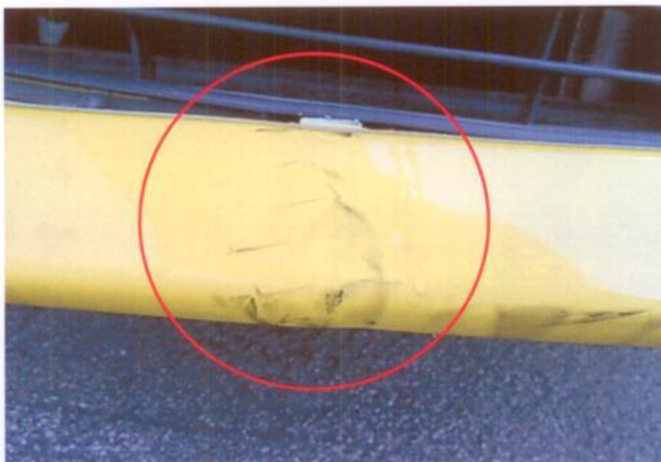
Photo 7 shows a close up view of the lower bumper of the Motor Taxi at the time of our inspection. The Motor Taxi had sustained relatively minor impact at the lower bumper of the Motor Taxi.
