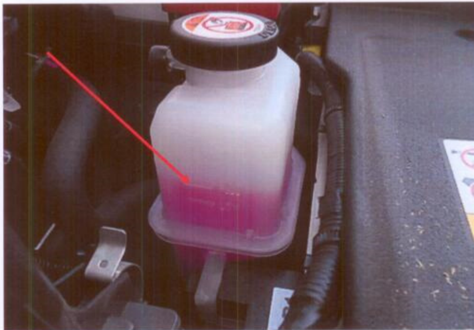
Photo 16 shows the engine coolant fluid reservoir of the Motor Taxi at the time of our inspection. The engine coolant fluid was observed to be of sufficient level and without any visible contamination.
