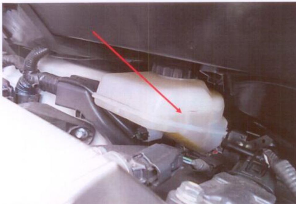
Photo 15 shows the brake fluid reservoir of the Motor Taxi at the time of our inspection. The brake fluid was observed to be of sufficient level (arrowed) and without any visible contamination.
