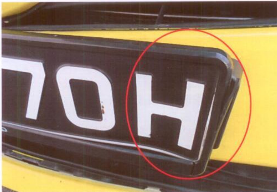
Photo 4 shows a close up view of the front number plate/base of the Motor Taxi at the time of our inspection. The Motor Taxi had sustained relatively minor impact at the front number plate/base of the Motor Car.
