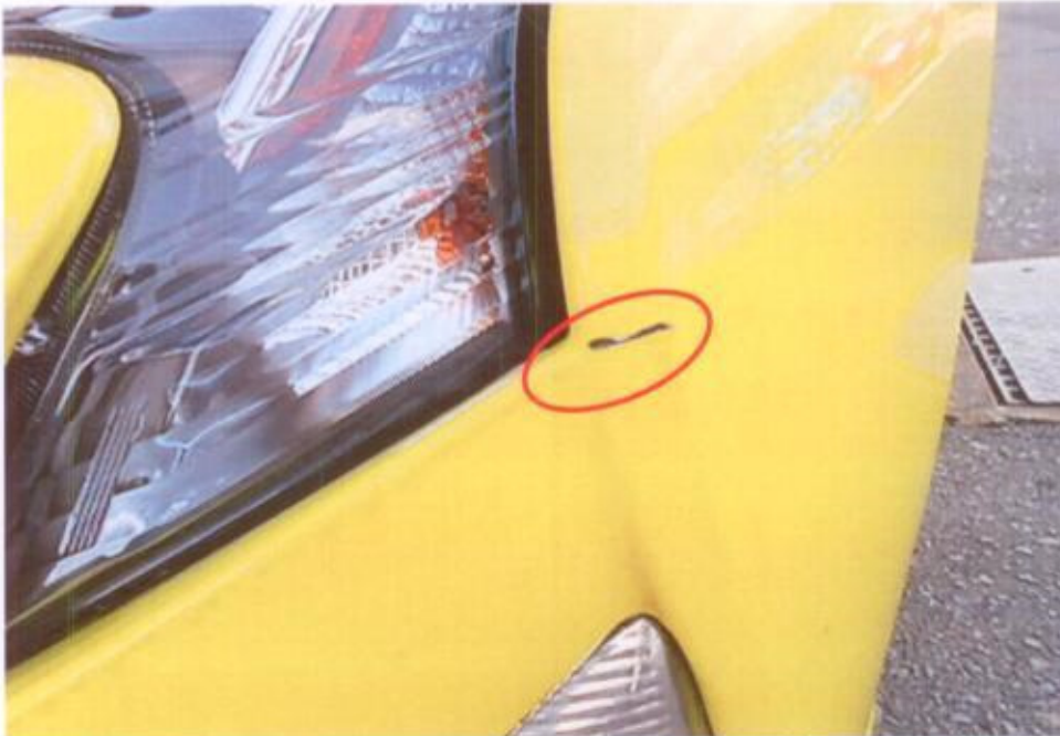
Photo 9 shows a close up view of the front bumper of the Motor Taxi at the time of our inspection. The Motor Taxi had sustained relatively minor scratch at the front bumper of the Motor Taxi.
