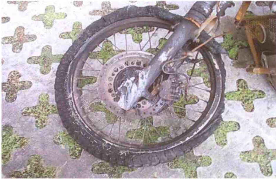
Photo 3 shows a closer view of the partially burnt front wheel rim and melted front tyre.
