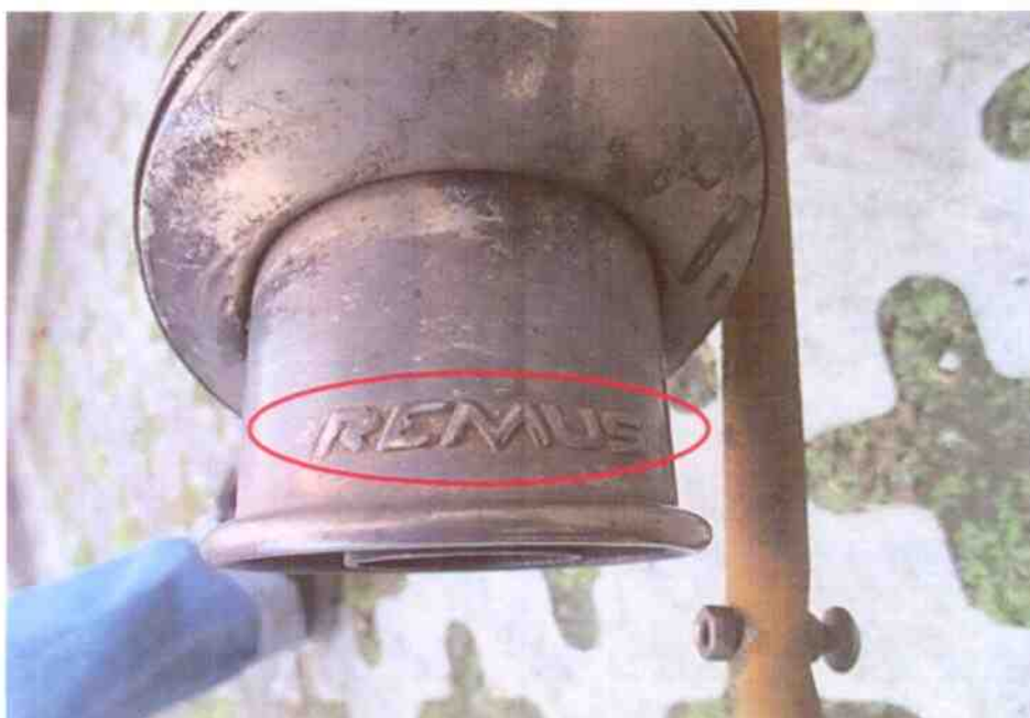
Photo 9 shows a close up top view of the non-standard rear exhaust muffler that was found to be fitted on the Insured Motorcycle at the time of our inspection. The brand of the rear exhaust muffler was 'REMUS' (circled).
