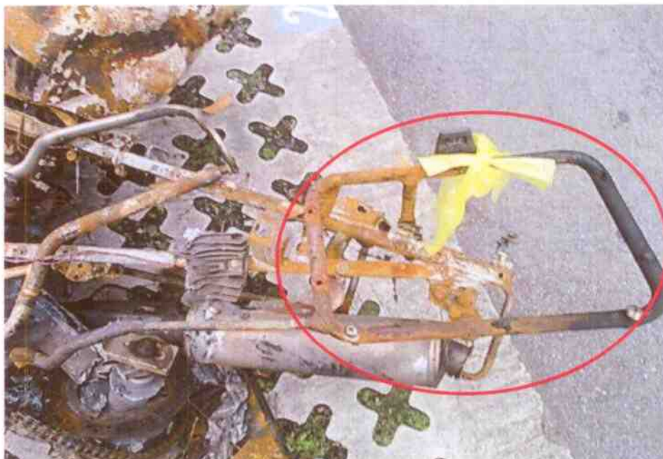
Photo 7 shows the side pannier rack (circled) fitted on the Insured Motorcycle which had accumulated rust as a result of exposure to environmental condition for a period of time.
