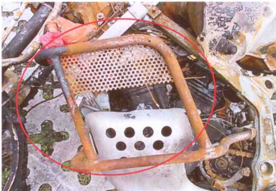
Photo 6 shows the engine crash bar (circled) fitted on the Insured Motorcycle which had accumulated rust as a result of exposure to environmental condition for a period of time.
