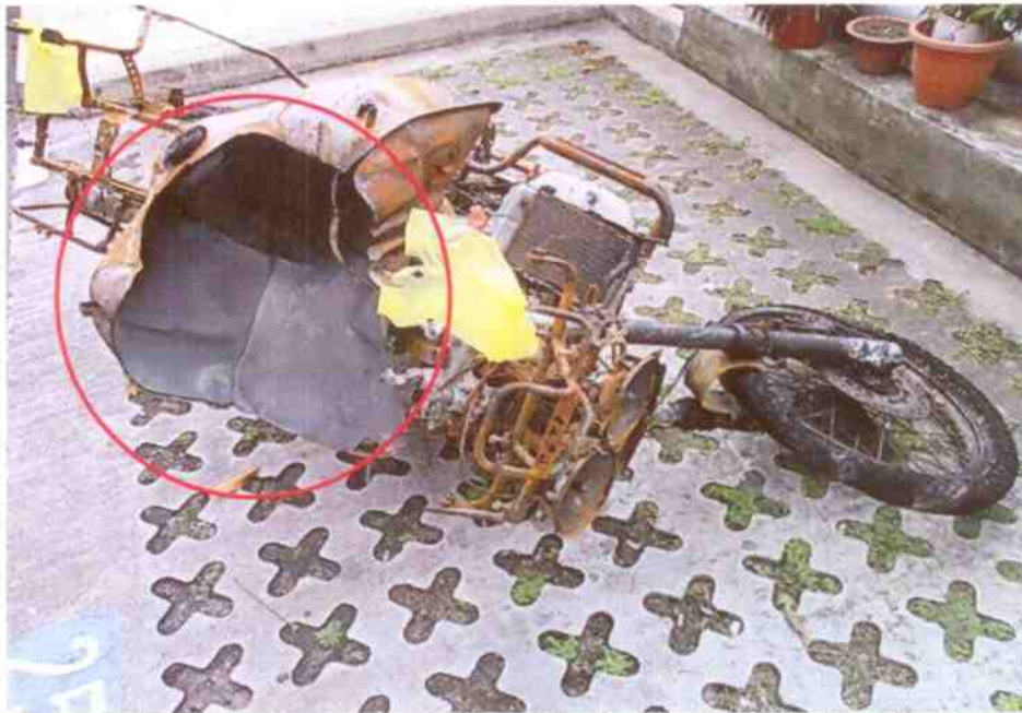
Photo 1 shows the general front view of the Insured Motorcycle at the time of inspection. The Insured Motorcycle was observed to have sustained severe fire damage all around. The fire caused the fuel tank to explode, exposing the internal part of the fuel tank (circled). Parts that were made of plastic and rubber type of material at its exterior body as well as some of its engine components were found to be severely burnt and/or melted. The drive train had sustained extensive fire damage, rendering the Insured Motorcycle immobile. Rust had accumulated all over the Insured Motorcycle as a result of exposure to environmental condition for a period of time.
