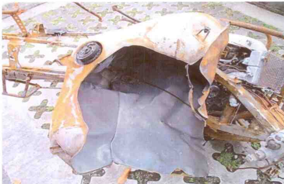
Photo 2 shows a closer view of the exposed internal part of the fuel tank as a result of the explosion caused by the fire.
