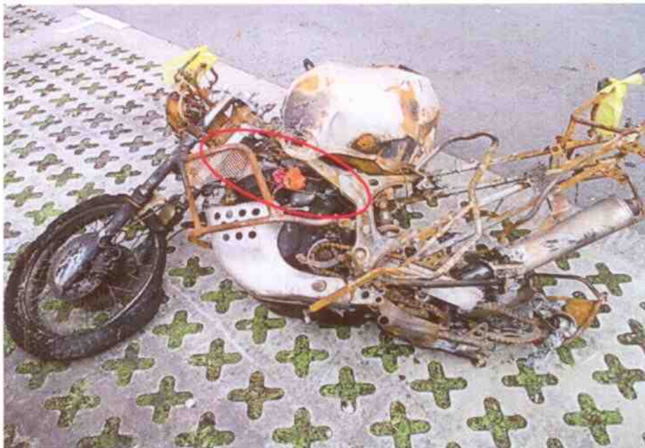
Photo 10 shows a view of the left side of the Insured Motorcycle. Upon closer examination of the left side of the Insured Motorcycle below the fuel tank which was where the fire had likely started, we had found several stretches of wirings with greenish residue (circled). These wirings were original factory fitted wirings. The presence of such greenish residue suggests occurrence of an electrical short circuit.
