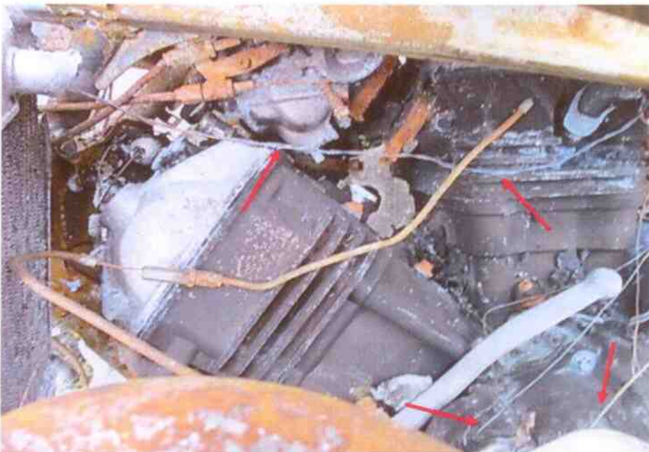
Photo 12 shows a closer view of the wirings with greenish residue (red arrows). The presence of greenish residue indicates internal heating of copper wires, a sign of an electrical short circuit occurring.
