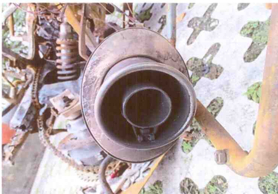
Photo 8 shows the front view of the non-standard rear exhaust muffler that was found to be fitted on the Insured Motorcycle at the time of our inspection.
