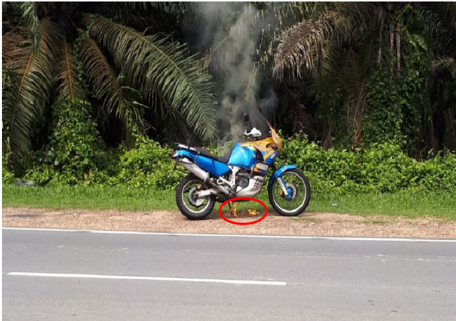
Photo 17 shows the Insured Motorcycle after the fire had started (circled). In general, the information that could be gathered from this photograph had corresponded to the events that were related to us by Mr Simon, which is the fire started from the left side.
