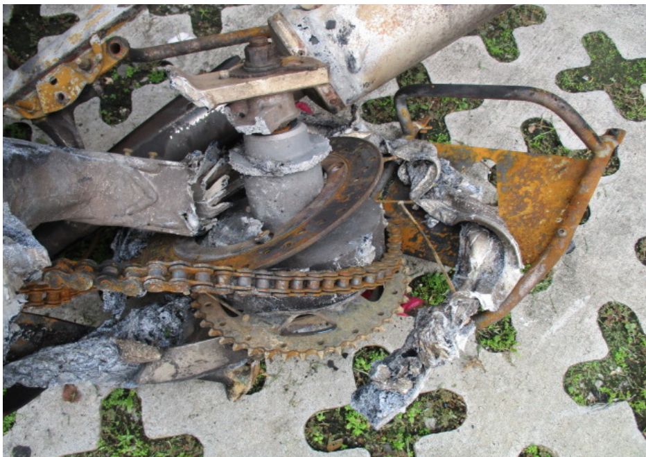
Photo 4 shows a closer view of the drive train which had sustained extensive fire damage, rendering the Insured Motorcycle immobile.
