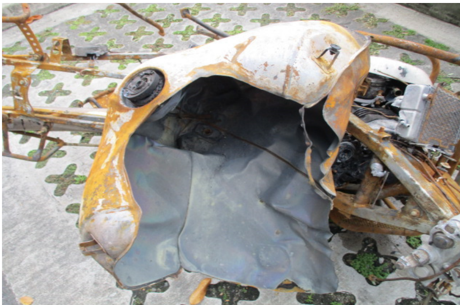
Photo 2 shows a closer view of the exposed internal part of the fuel tank as a result of the explosion caused by the fire.
