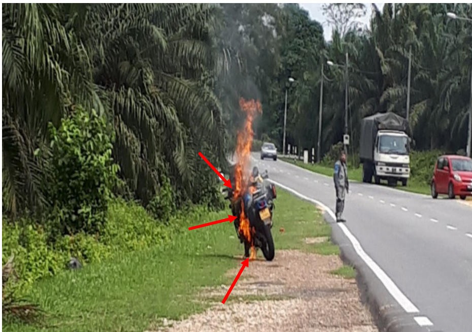
Photo 18 shows the rear view of the Insured Motorcycle as the fire began to spread. In general, the information that could be gathered from this photograph had corresponded to the events that were related to us by Mr Simon, which is the fire started from the left side (red arrows).
