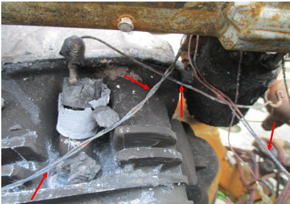
Photo 14 shows a close up view of the wirings with greenish residue (red arrows). The presence of greenish residue indicates internal heating of copper wires, a sign of an electrical short circuit occurring.
