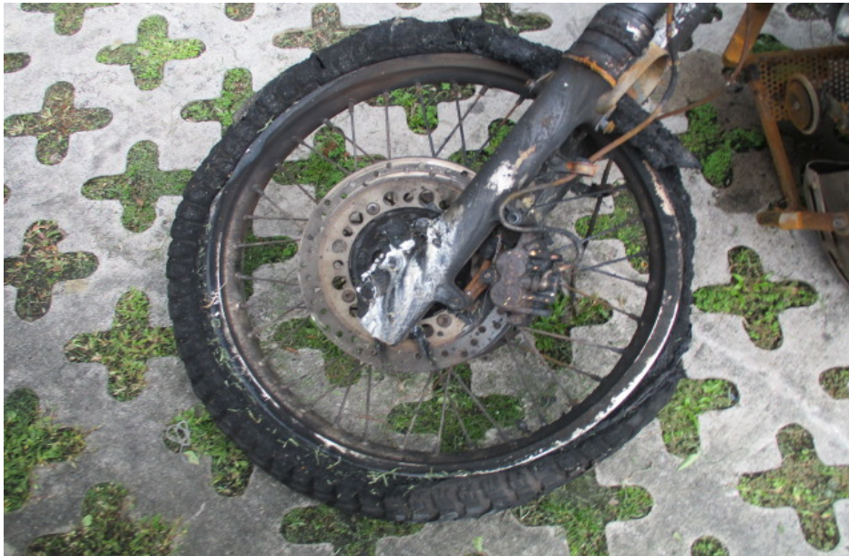
Photo 3 shows a closer view of the partially burnt front wheel rim and melted front tyre.
