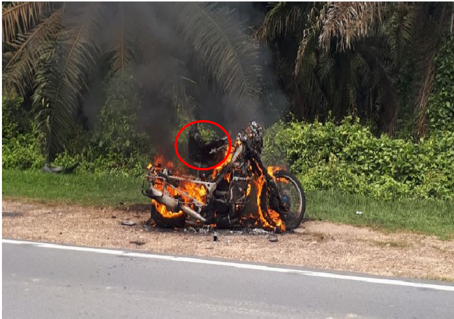
Photo 19 shows flames engulfing the Insured Motorcycle. In general, the information that could be gathered from this photograph had corresponded to the events that were related to us by Mr Simon, which is the fuel tank exploded shortly after the fire broke out (circled).
