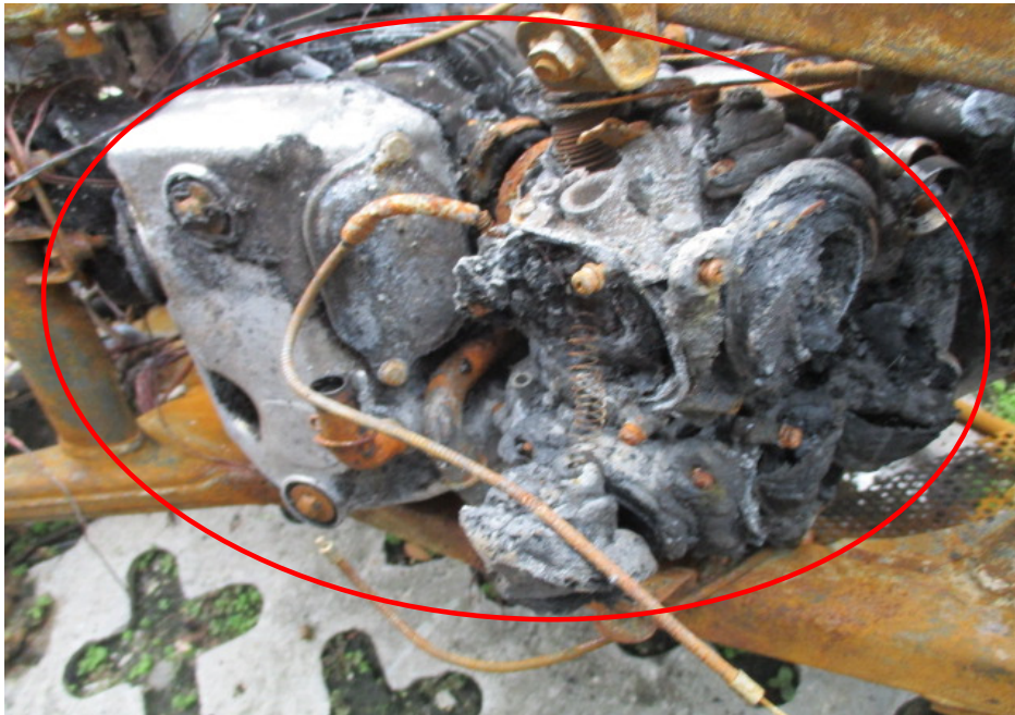
Photo 5 shows a close up view of the severely burnt and/or melted engine components of the Insured Motorcycle as a result of the fire (circled).
