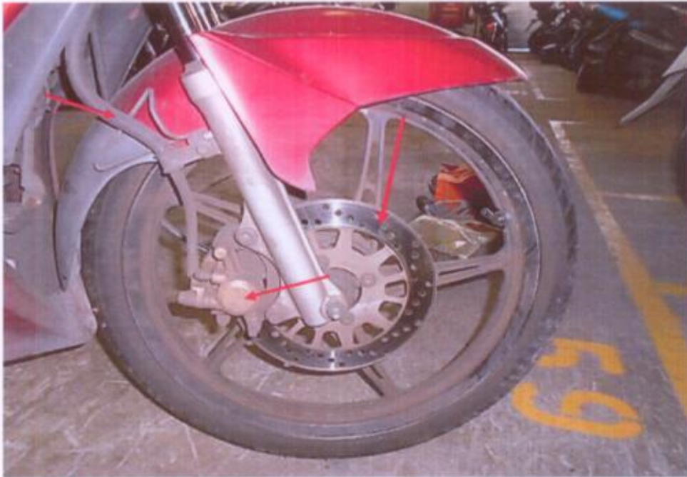
Photo 13 shows the front brake calliper, front brake disc and front brake hose of the Motorcycle (arrowed), which are all part of the components in the front brake system of the Motorcycle. Our visual checks of these various components had revealed all to be intact with no visible damage. No leakage of brake fluid was also observed.
