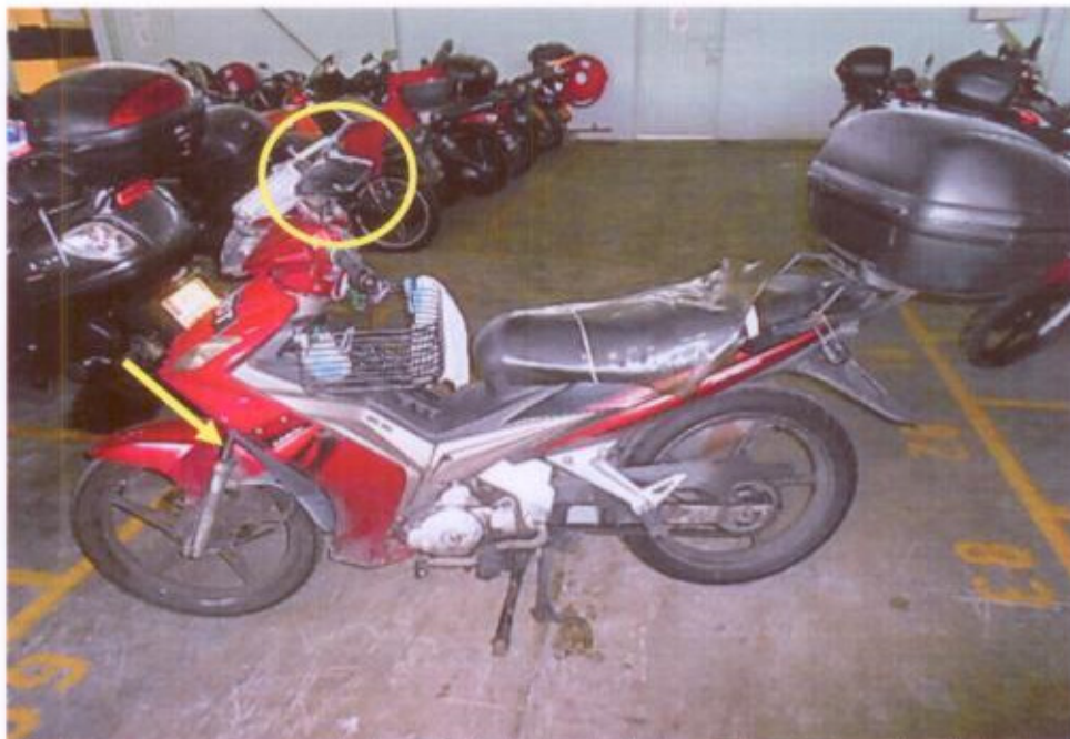
Photo 2 shows a general view of the left side body of the Motorcycle at the time of our inspection. The Motorcycle was observed to be sustained with relatively minor impact due to the accident collision. The body parts that were found to have been damaged include its front left wing mirror & its front fork assembly as a result of the accident.
