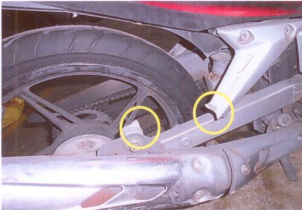
Photo 5 shows a close-up view of the broken passenger foot rest of the Motorcycle due to the accident collision.
