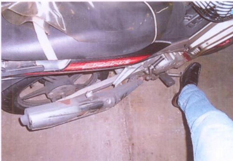
Photo 16 shows the rear brake static test of the Motorcycle. The type of brake system for the rear wheel was of mechanical type, controlled by the brake foot pedal of the Motorcycle. Our static brake test revealed that the rear brake system of the Motorcycle was in serviceable condition without damage.
