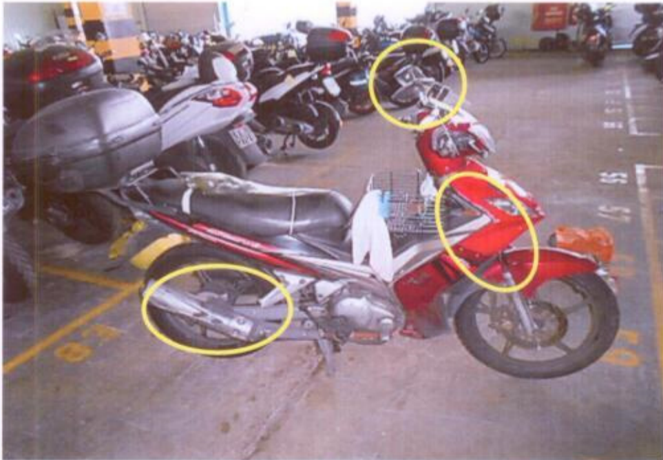
Photo 3 shows a general view of the right side body of the Motorcycle at the time of our inspection. The body parts that were found to have been damaged include its front left wing mirror, broken pillion's right foot rest, minor scratches at right hand side fairing and exhaust pipe amongst others. Its front fork assembly was also observed to be bent slightly to the right as a result of the accident.
