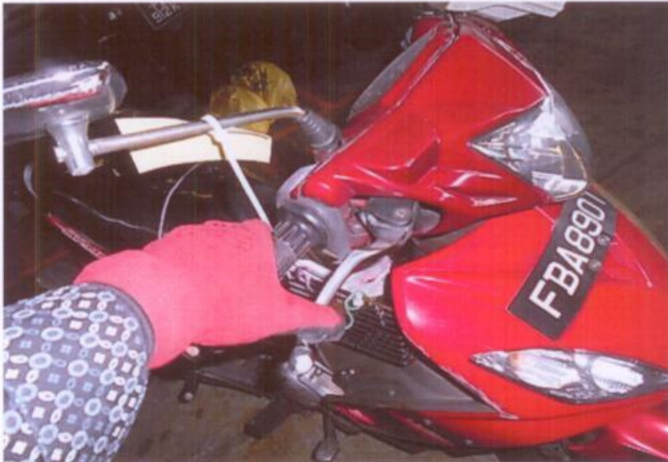
Photo 15 shows the front brake static test. It was observed to be in serviceable condition at time of our inspection.
