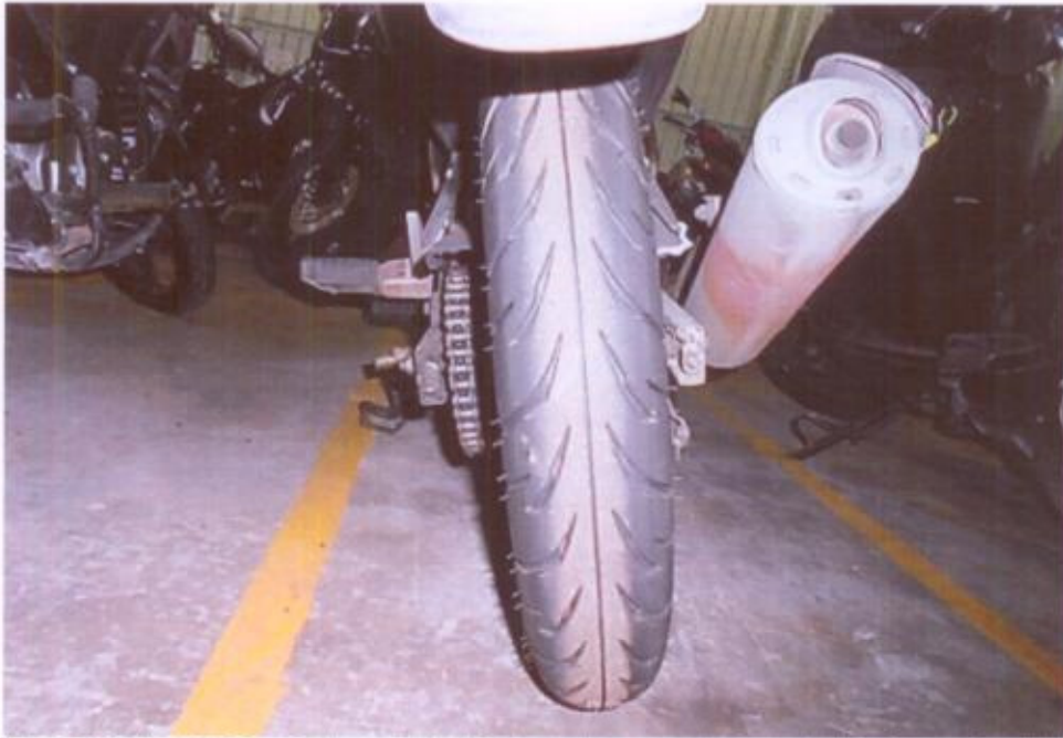
Photo 6 shows the rear tyre of the Motorcycle was observed to be in serviceable condition with remaining tread depth of approximately 3mm. The tyre was also observed to be sufficiently inflated for vehicular operation. There was no significant damage observed on the rear wheel rim & tyre.
