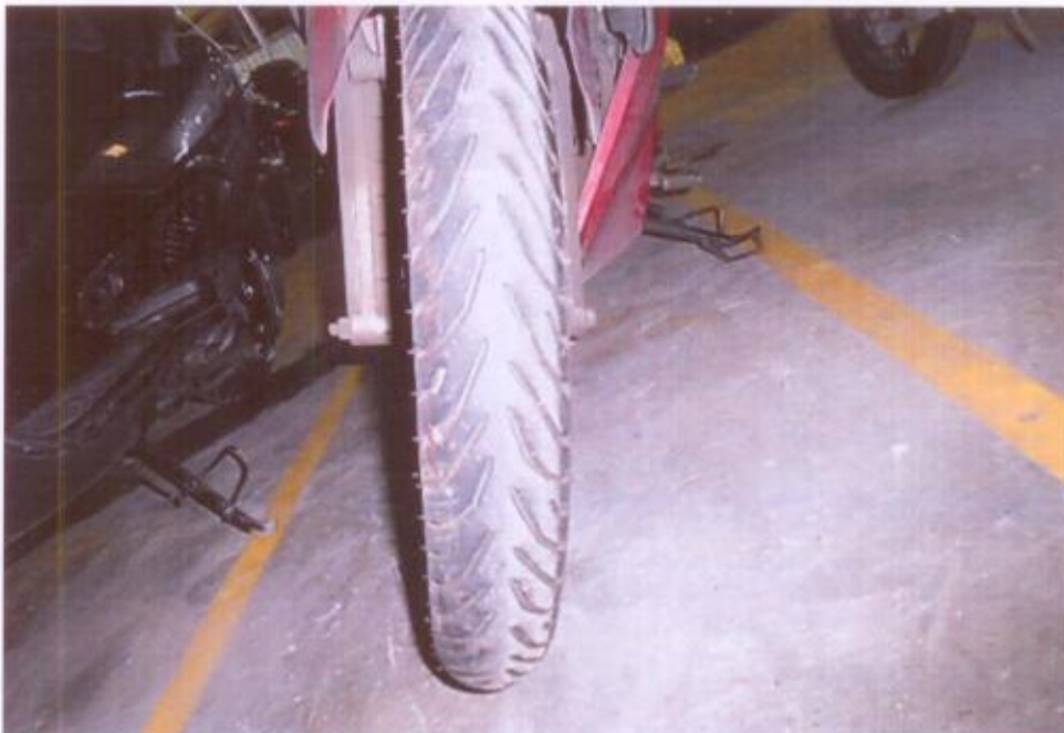
Photo 7 shows the front tyre of the Motorcycle. There was no tear, burst mark(s) and/or punctured hole(s) on the sidewalls as well as across the tread of the front tyre.
