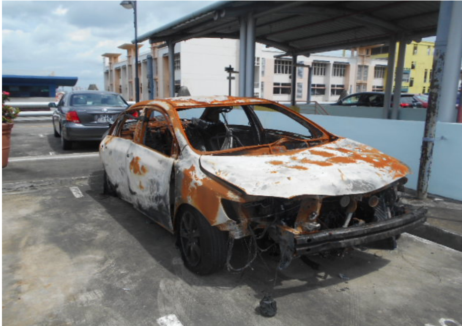
Photo 1 shows a general view of the front right body of the Insured Vehicle at the time of my inspection. The Insured Vehicle was observed to have sustained extensive fire damage all around. Almost all the body panels were found to have been burnt to char. Its front bonnet, front fenders, front doors, rear door and roof panel were all extensively burnt.
