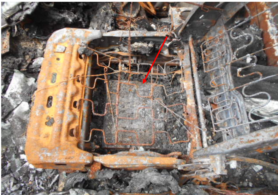
Photo 6 shows the audio amplifier (arrowed) that was found fitted under the front left passenger seat of the Insured Vehicle at the time of my inspection.
