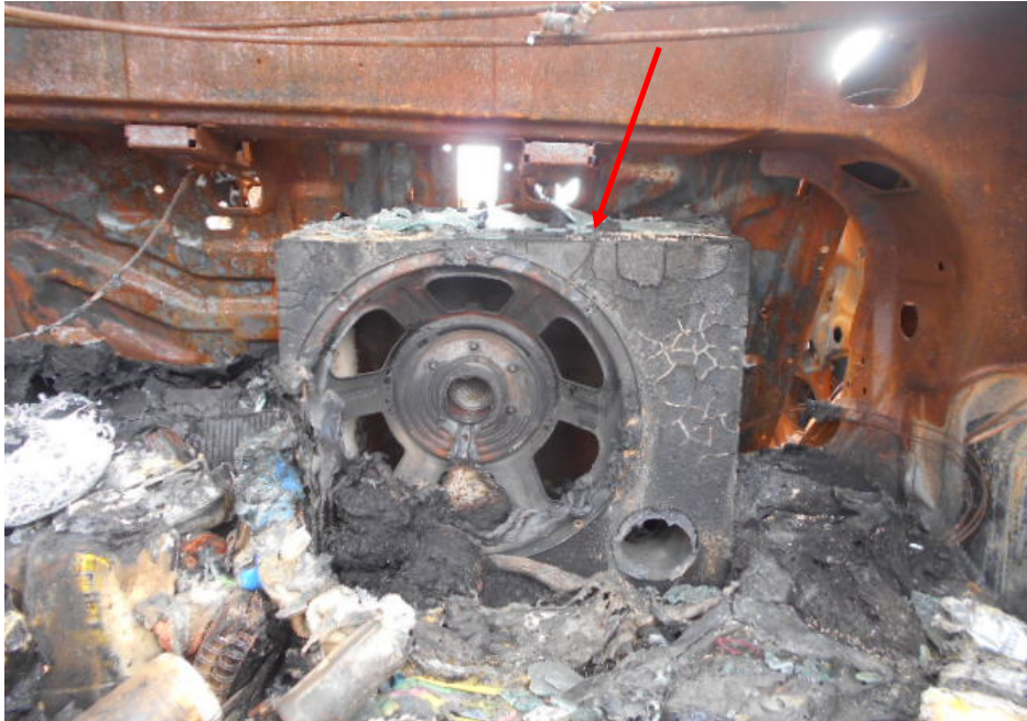
Photo 5 shows the woofer speaker (arrowed) that was found fitted inside the rear boot compartment of the Insured Vehicle at the time of my inspection.
