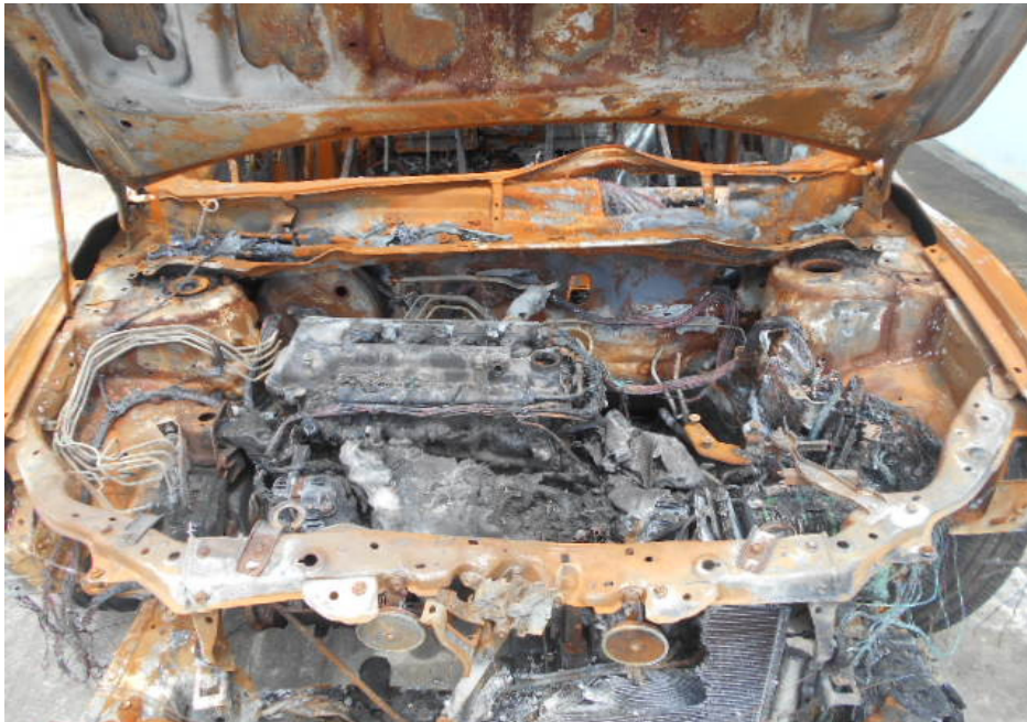
Photo 4 shows the engine compartment of the Insured Vehicle at the time of my inspection. The various parts and components inside the engine compartment were observed to have been completely burnt.
