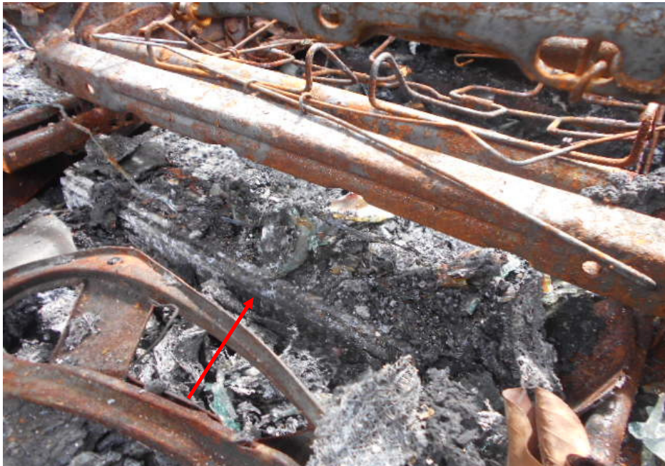
Photo 8 shows a closer view of the audio amplifier (arrowed) that was found fitted under the driver's seat of the Insured Vehicle at the time of my inspection.
