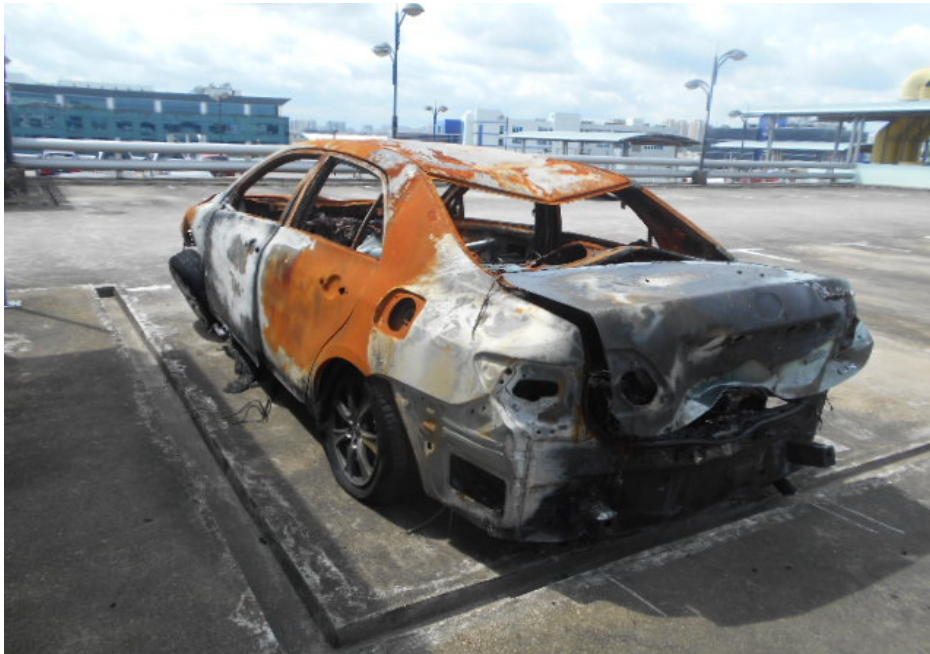
Photo 2 shows a general view of the rear left body of the Insured Vehicle at the time of my inspection. The Insured Vehicle was observed to have sustained extensive fire damage all around. Almost all the body panels were found to have been burnt to char.
