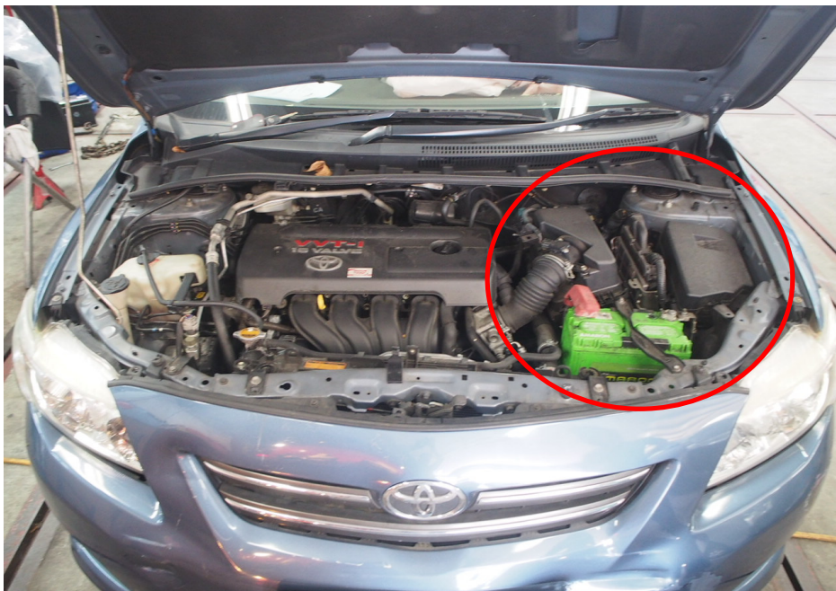
Photo 9 shows the engine layout of a similar make and model vehicle as the Insured Vehicle. There was no fluid carrying hoses or pipes around the left side of the engine compartment (circled), which could have leaked onto the hot surfaces of the exhaust pipes. Fire as a result of fluid leakage would then seem unlikely for this case. This follows the description of Mr Ang that flames were seen coming out from the left side of the front bonnet.
