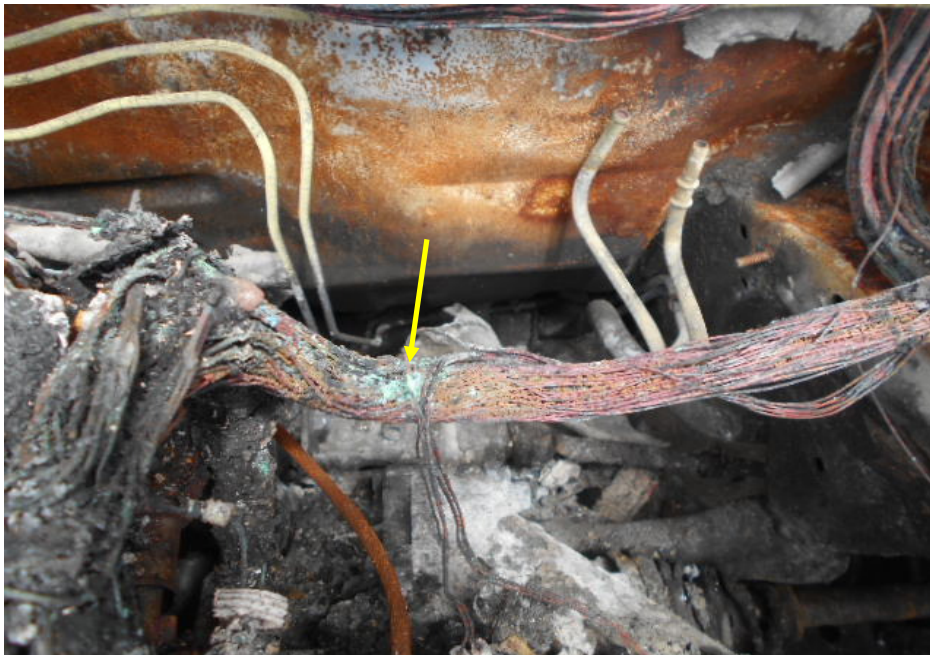
Photo 12 shows another stretch of wirings, at the left side of the engine compartment, where greenish residue were found. The wirings were original wires connecting to the engine control module of the Insured Vehicle.
