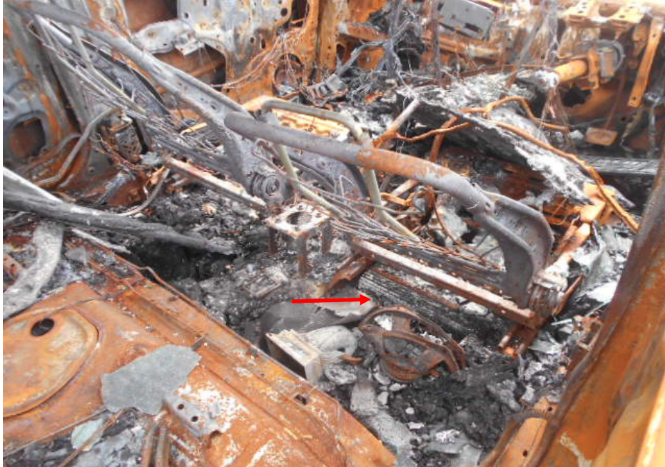
Photo 7 shows the audio amplifier (arrowed) that was found fitted under the driver's seat of the Insured Vehicle at the time of my inspection.
