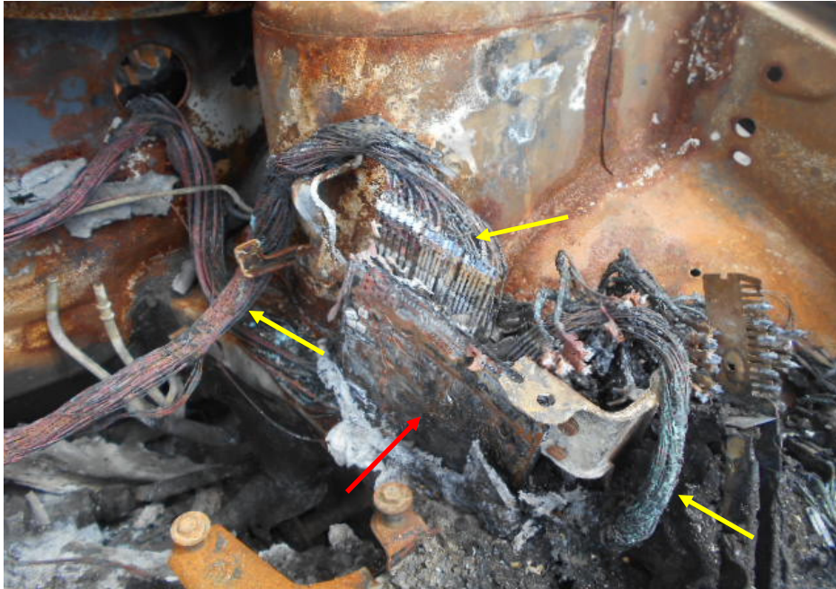
Photo 11 shows the engine compartment of the Insured Vehicle, at the left side area. Upon further examination, I had found greenish residue on several stretches of wirings (yellow arrow) around this area. The wirings were original wires connecting to the engine control module (red arrow) of the Insured Vehicle. The presence of greenish residue indicates internal heating of copper wires, a sign of an electrical short circuit occurring.
