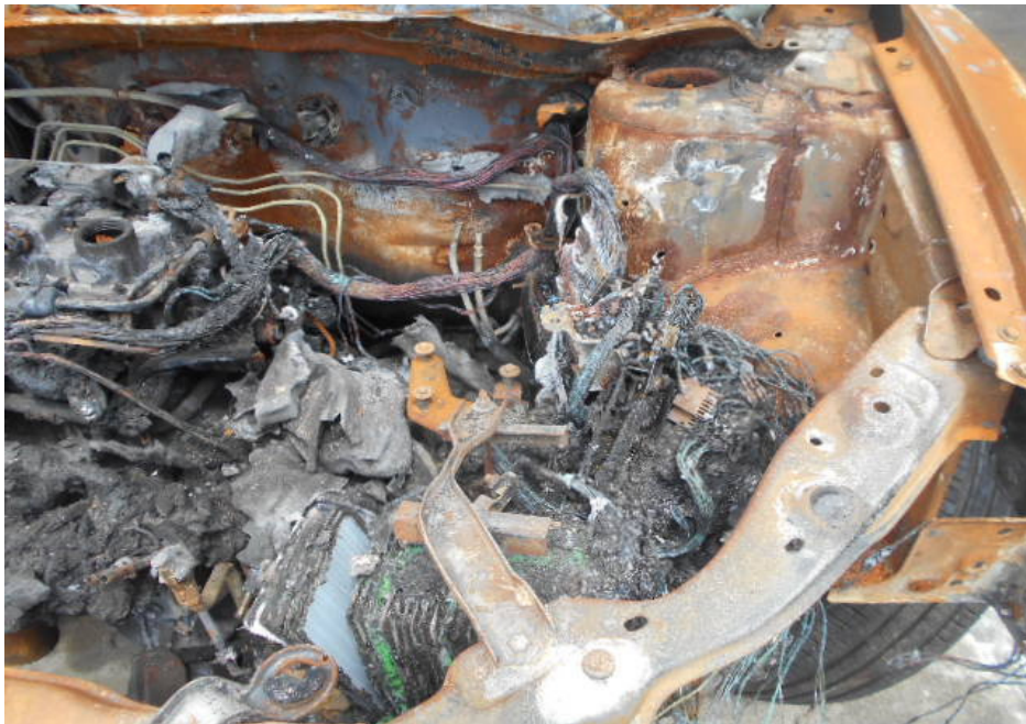
Photo 10 shows the engine compartment of the Insured Vehicle, at the left side area. The driver of the Insured Vehicle had seen flames coming from the left side of the front bonnet. From my observations, the battery, engine control unit and fuse box were amongst the parts that were around the left side of the engine compartment.
