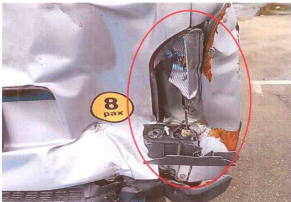
Photo 4 shows the damage sustained on the rear right tail lamp as a result of the accident.
