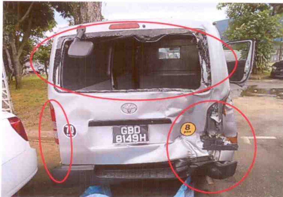
Photo 1 shows a general view of the rear body of the Motor van at the time of our inspection. The Motor Van was observed to have sustained damages at its rear right portion, rear window glass, rear tail lamp, rear exhaust pipe, rear door, rear lower bumper & left rear lower side panel, was amongst the body parts that were damaged as a result of the accident. (circled).
