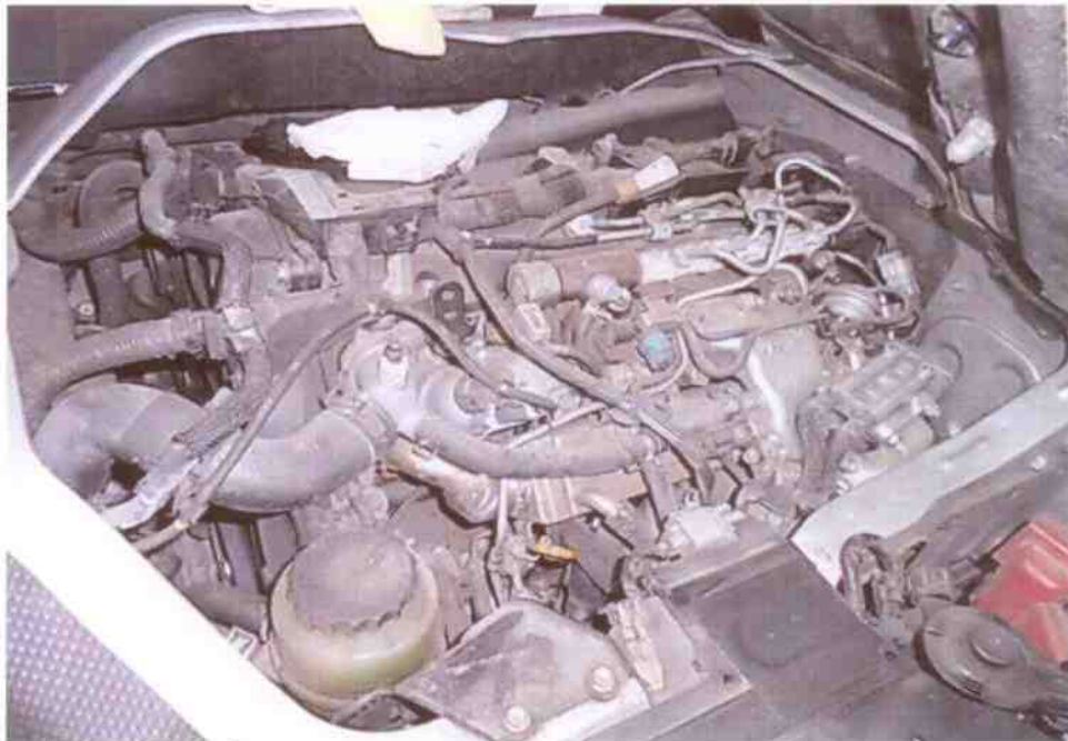
Photo 12 shows a general view of the Motor Van's engine compartment, which was accessed by lifting the passenger's seat of the Motor Van. The various parts and components inside the engine compartment were unaffected by the accident. There was also no sign(s) or indication(s) of fresh fluid leakage and/or fluid stain within the engine compartment.
