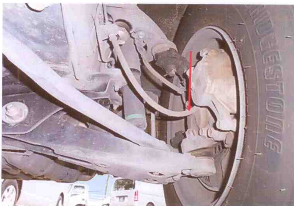
Photo 20 shows the various undercarriage components at the front right wheel of the Motor van, in particular the steering tie rod end. The various steering components were all found to be intact, suggesting that it's in serviceable condition at the material time of accident. There was also no sign of fluid stain(s) observed on the various undercarriage components. (arrowed)
