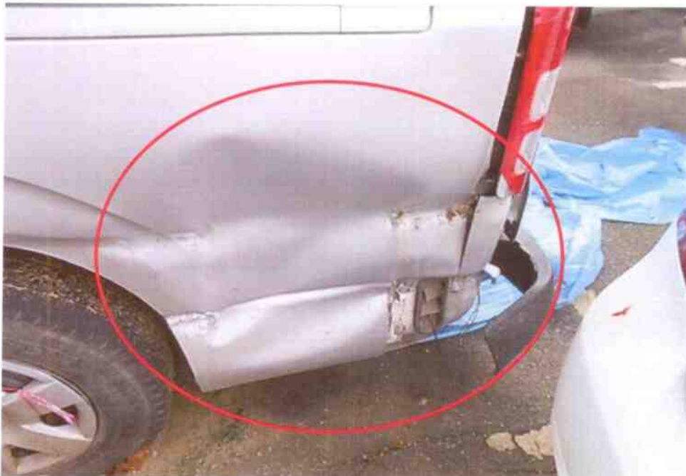
Photo 2 shows a general view of the rear left body of the Motor Van at the time of my inspection. The Motor Van was observed to have sustained damages at its rear left panel.
