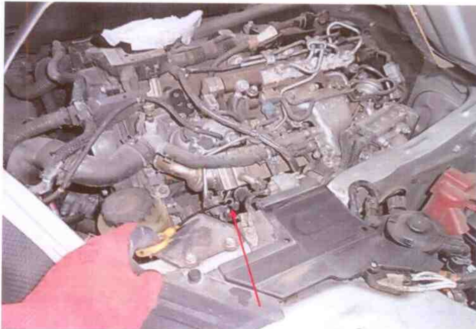
Photo 16 shows the engine dip stick (general view) of the Motor Van at the time of our inspection. The engine oil was observed to be of sufficient level and without any visible contamination (arrowed).
