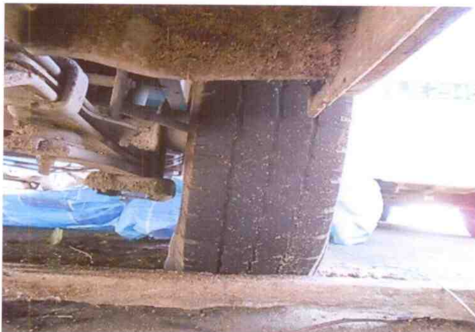
Photo 10 shows the condition of the rear left tyres of the Motor Van, which was observed to be in serviceable condition with remaining tread depth of approximately 2mm. The tyres, which were wrapped around standard wheel rim, were also observed to be sufficiently inflated for vehicular operation.
