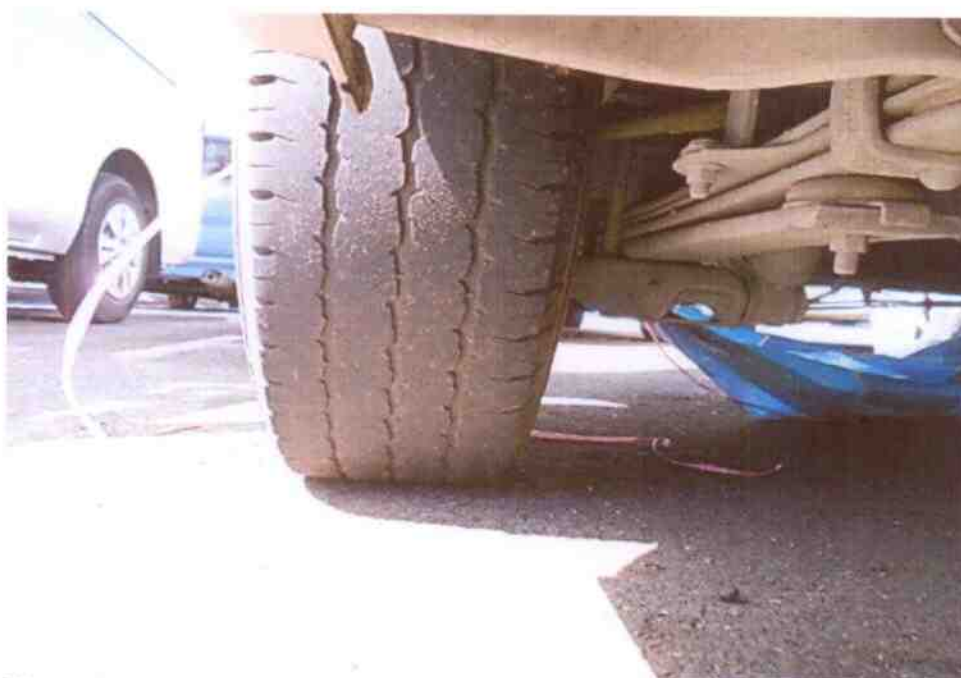
Photo 11 shows the condition of the rear right tyres of the Motor Van, which were observed to be in serviceable condition with remaining tread depth of approximately 2mm. There was also no tear, cut or burst mark(s) on the outer and the inner sidewalls as well as across the tread of the 4 tyres that were fitted on the Motor Van.
