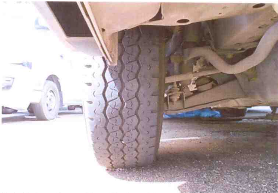
Photo 9 shows the condition of the front right tyre of the Motor Van, which was observed to be in serviceable condition with remaining tread depth of approximately 6mm.
