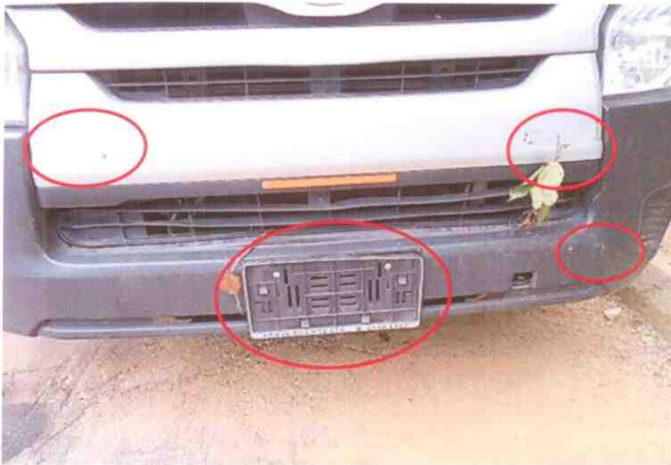
Photo 6 shows the damage sustained on the frontal portion dents & scratches inclusive number plate base.
