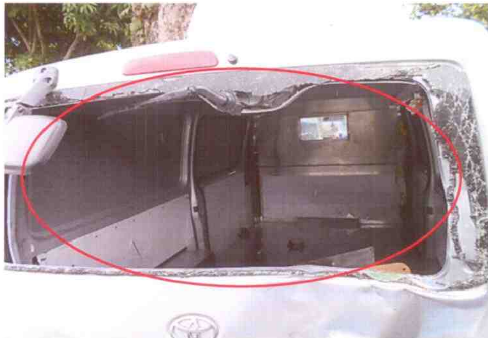
Photo 3 shows the damage sustained on the rear window glass as a result of the accident.
