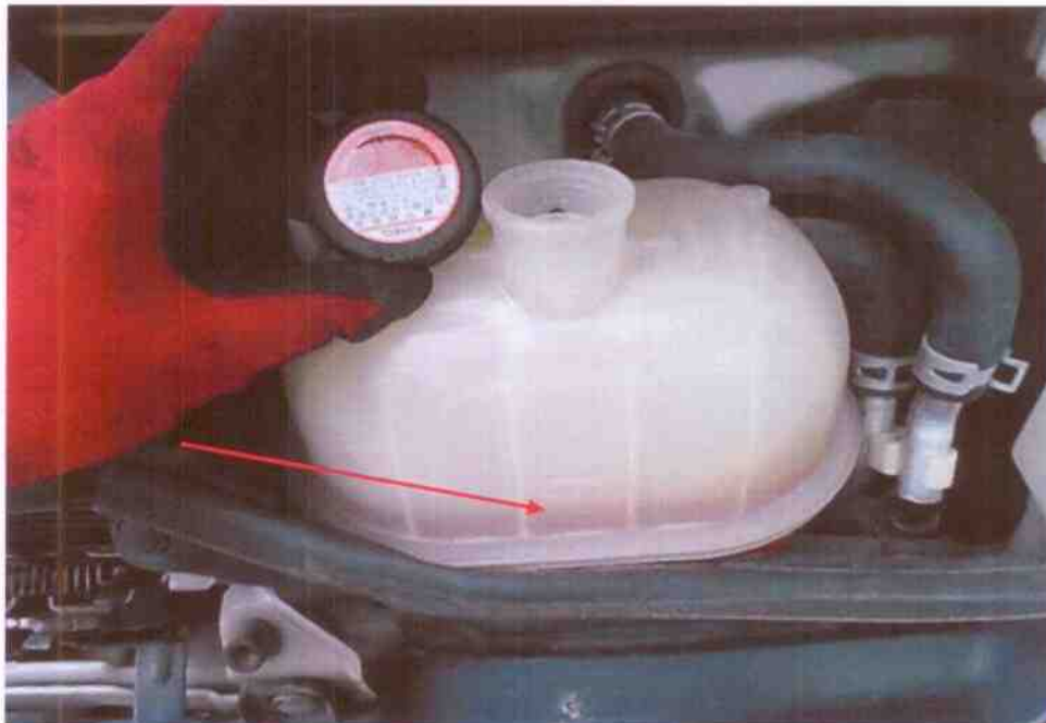
Photo 14 shows the engine coolant reservoir of the Motor van at the time of our inspection. The coolant was observed to be of sufficient level and without any visible contamination.
