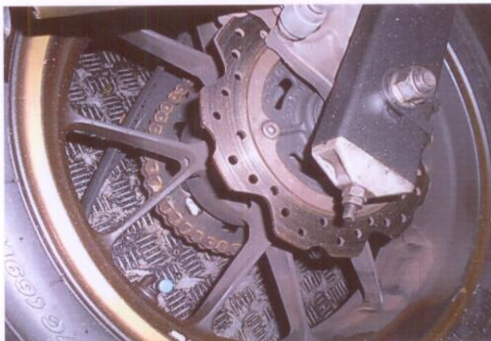
Photo 7 shows the rear tyre of the Motorcycle at the time of our inspection. The rear tyre was observed to be in serviceable condition with remaining tread depth of approximately 5mm. The tyre was also observed to be sufficiently inflated for vehicular operation. There was no significant damage observed on the rear wheel rim & tyre.
