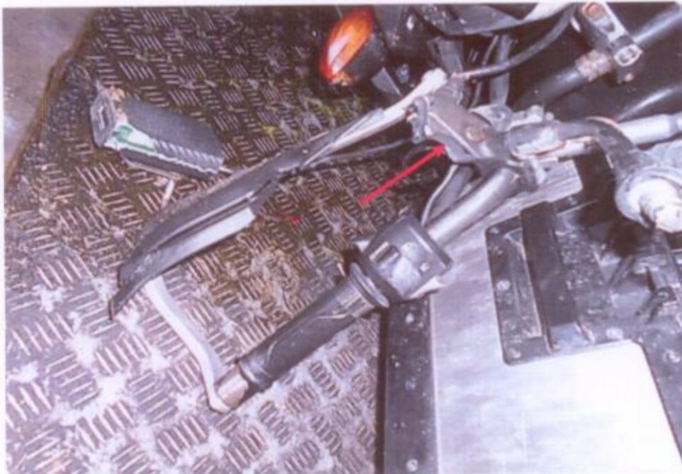
Photo 14 shows the hand brake lever (arrowed) was observed to be broken likely due to the result of the accident. Hence, we are unable to conduct any tests on the braking system of the Motorcycle.
