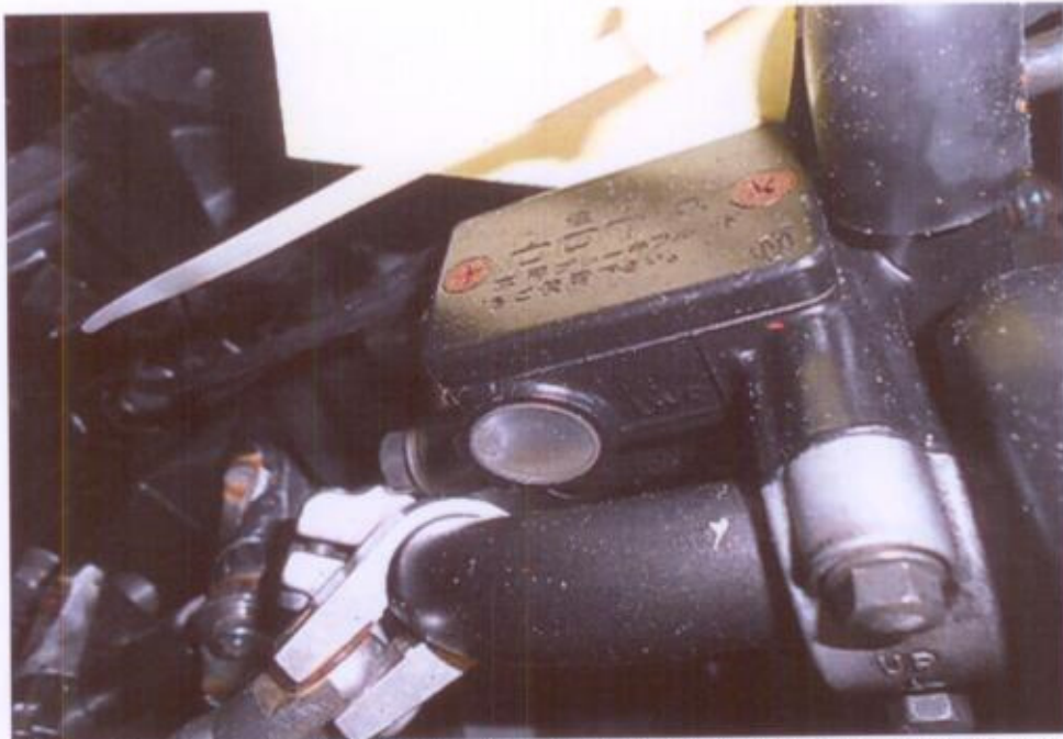
Photo 18 shows the front brake fluid reservoir of the Motorcycle which was observed to be insufficient due to the leakage likely caused by the accident's collision.
