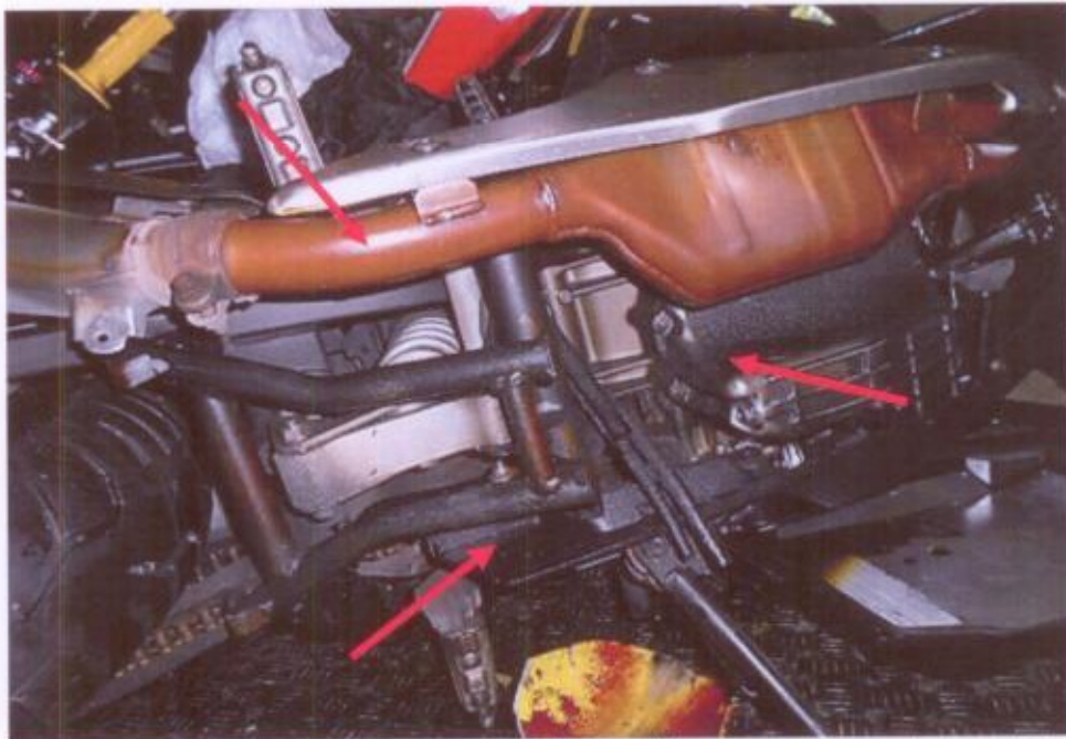
Photo 11 shows sign(s) or indication(s) of fluid leakage observed around the engine's underside area of the Motorcycle.
