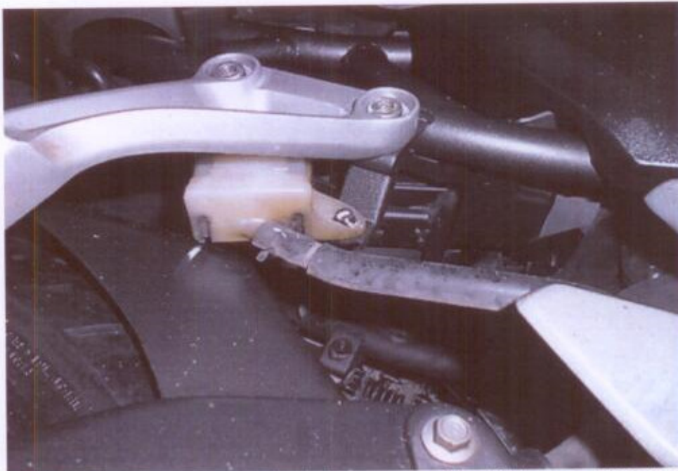
Photo 19 shows the rear brake fluid reservoir of the Motorcycle which was observed to be sufficient at time of our inspection.
