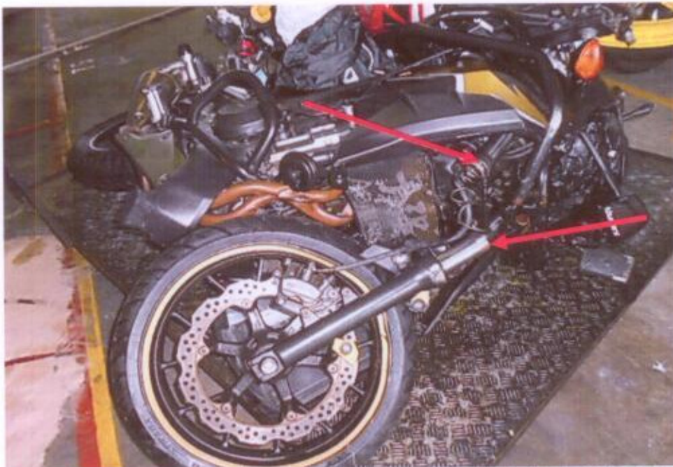
Photo 2 shows a general view of the front right body of the Motorcycle at the time of our inspection. The Motorcycle was observed to have sustained with relatively extensive impact due to the accident collision. Amongst the body parts damaged was its front fork (arrowed), which was observed to be broken into 2 pieces.
