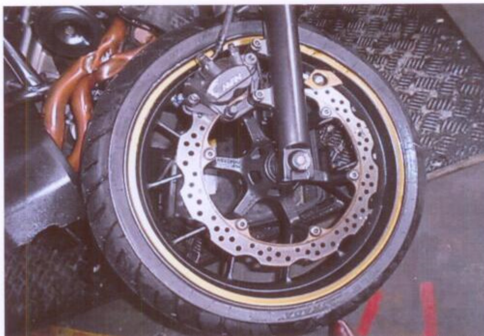
Photo 8 shows the front tyre of the Motorcycle at the time of our inspection. The pattern of the tread was clearly visible. There was no tear, burst mark(s) and/or punctured hole(s) on the sidewalls as well as across the tread of the front tyre.
