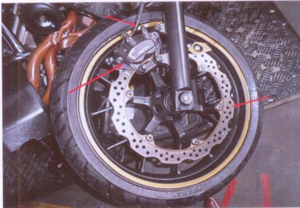
Photo 16 shows the front brake calliper, front brake disc and front brake hose of the Motorcycle (arrowed in red), which are all part of the components in the front brake system of the Motorcycle. Our visual checks of these various components had revealed all to be intact with no visible damage.
