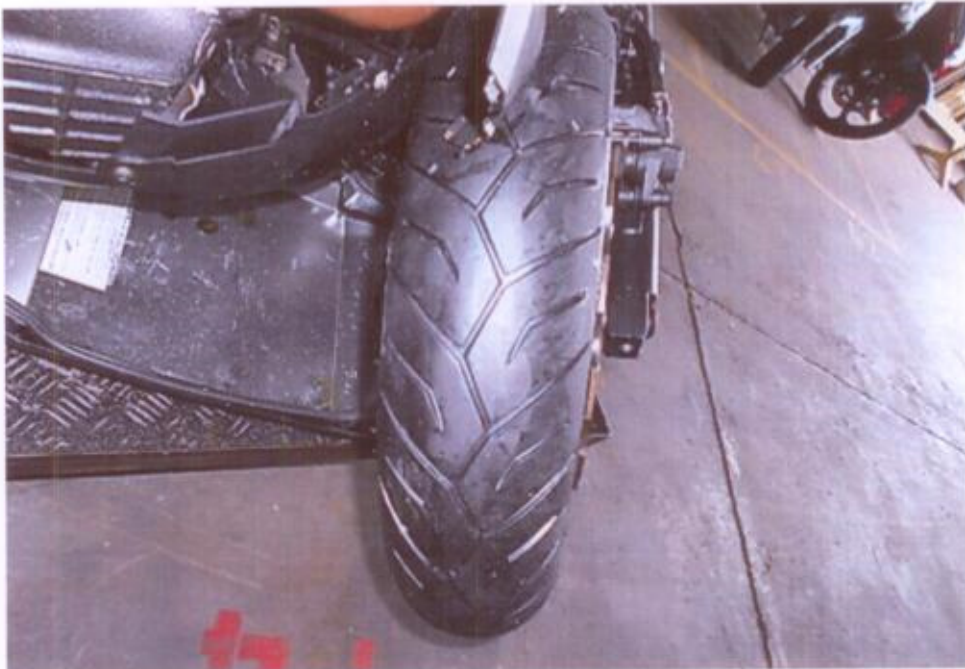
Photo 9 shows the front tyre of the Motorcycle at the time of our inspection. The pattern of the tread was clearly visible. There was no tear, burst mark(s) and/or punctured hole(s) on the sidewalls as well as across the tread of the front tyre.
