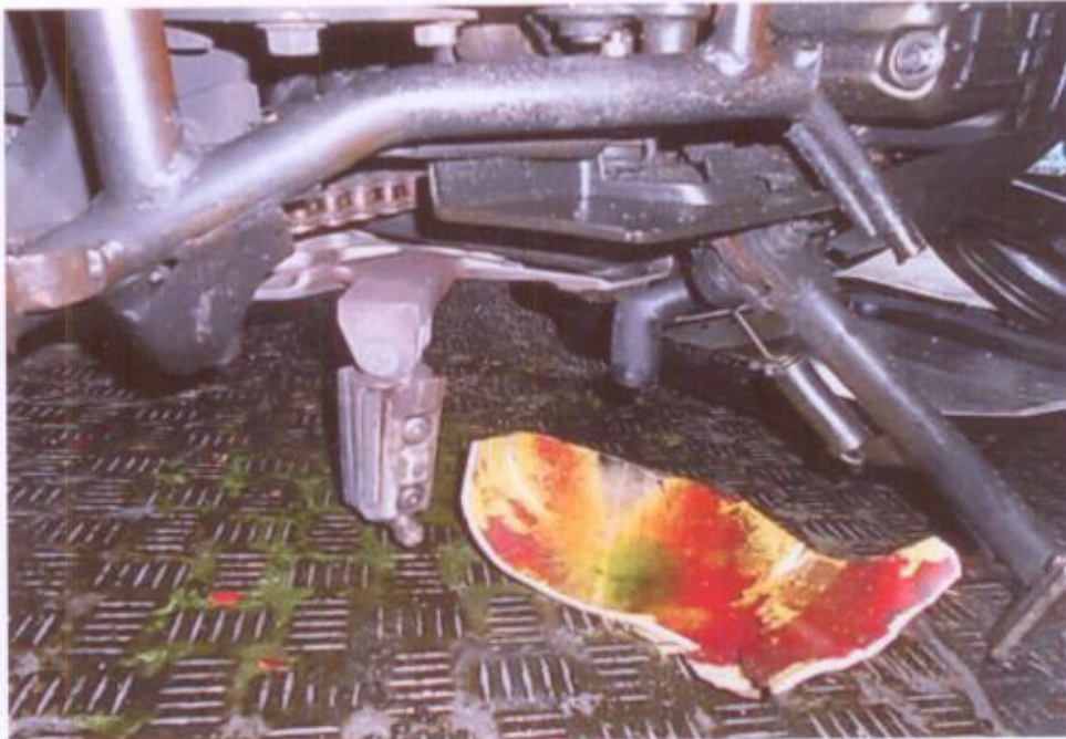
Photo 12 shows sign(s) or indication(s) of fluid leakage observed around the engine's area of the Motorcycle.
