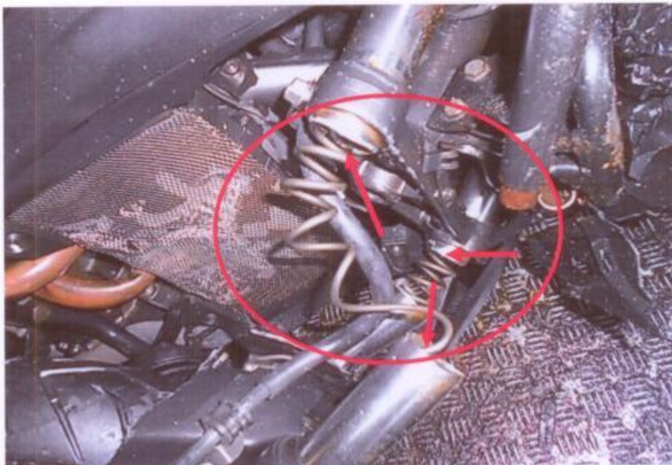
Photo 6 shows a close-up view of the frontal portion of the Motorcycle at the time of our inspection. The Motorcycle was observed to have sustained relatively extensive impact including damages to the broken front fork (circled) likely due to the accident collision.
