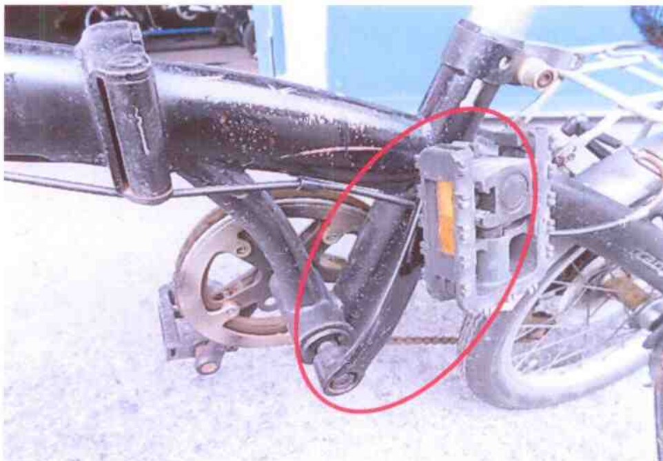
Photo 4 shows a close-up view of the left pedal of the Bicycle at the time of our inspection. It was observed to have sustained damages at the left pedal of the Bicycle.
