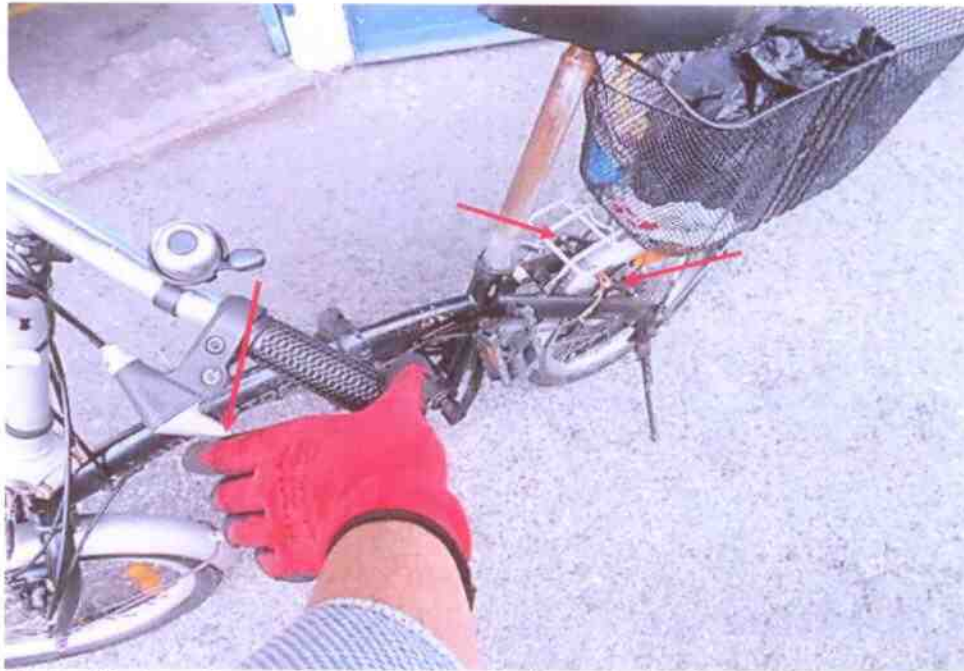
Photo 12 shows the rear brake static test before gripping the brake lever.
