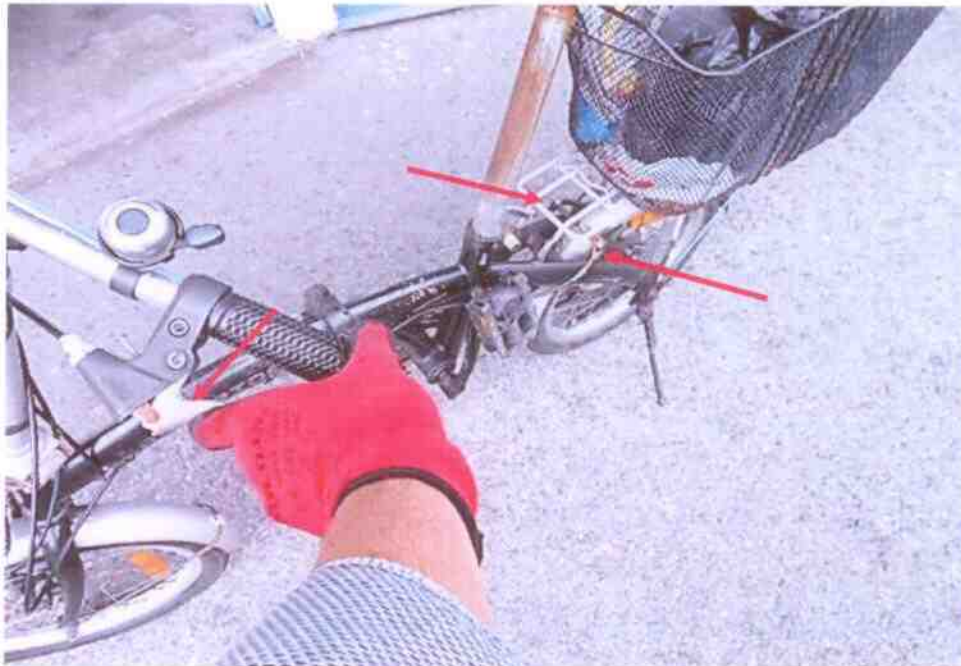
Photo 13 shows the rear brake static test upon gripping the brake lever. It responded to the braking action indicates that it was in serviceable condition.
