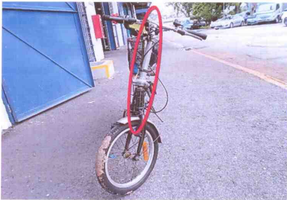
Photo 2 shows the frontal portion of the Bicycle at time of inspection. Misalignment of the handle bar & front tyre was observed.
