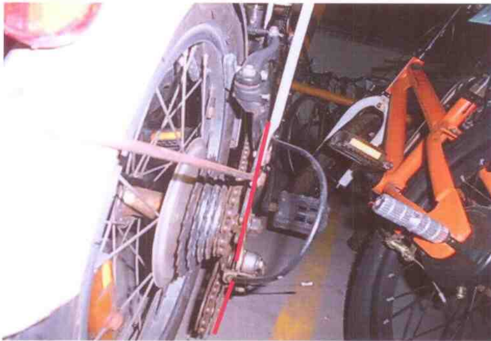
Photo 8 shows the general view of the gear train of the Motorcycle, which was observed to be misaligned due to the accident. It was not adequately lubricated at time of inspection.
