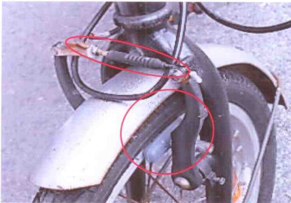
Photo 9 shows the front brake (circled) was observed to be intact without any damages. Static brake test was conducted on both front & rear brake & found to be in serviceable condition.
