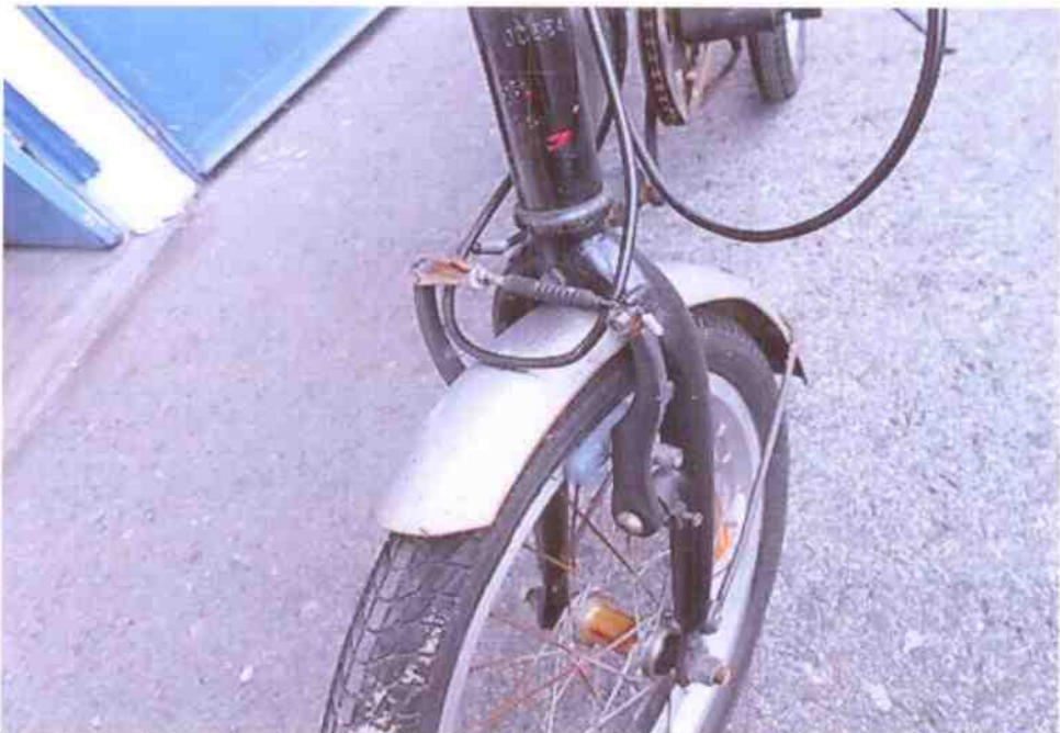
Photo 7 shows the front tyre of the Motorcycle. The pattern of the tread was clearly visible. There was no tear, burst mark(s) and/or punctured hole(s) on the sidewalls as well as across the tread of the front tyre.
