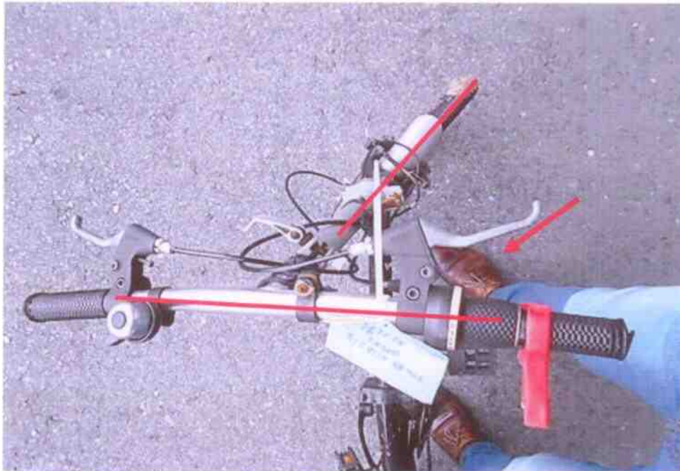
Photo 3 shows the frontal portion of the Bicycle (top view) at time of inspection. Misalignment of the handle bar & front tyre was observed.
