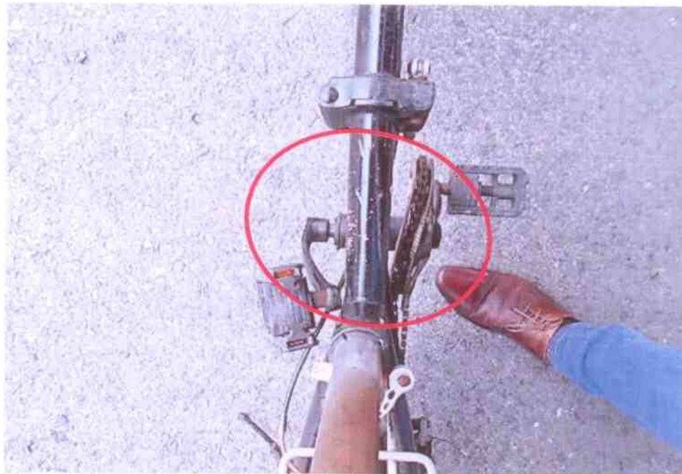
Photo 5 shows a close-up view (top view) of the left pedal & the drive train of the Bicycle at the time of our inspection. It was observed to have sustained damages at the circled area of the Bicycle due to the accident.
