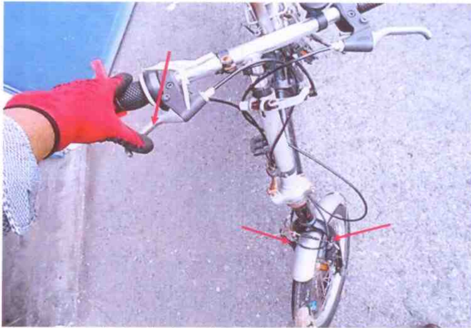
Photo 10 shows the front brake static test before gripping the brake lever.
