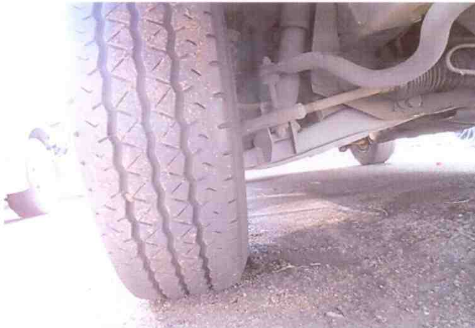
Photo 9 shows the condition of the front right tyre of the Motor Van, which was observed to be in serviceable condition with remaining tread depth of approximately 5mm.
