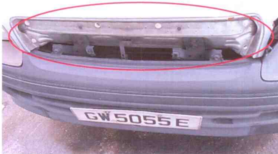
Photo 5 shows the damage sustained on the front grille (missing) as a result of the accident.
