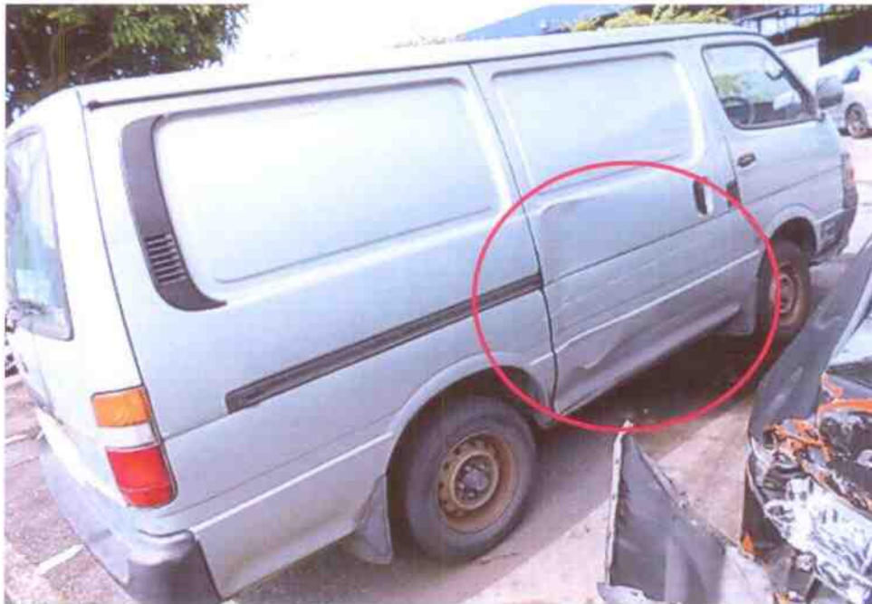
Photo 6 shows the damage sustained on the right hand side dents & scratches.
