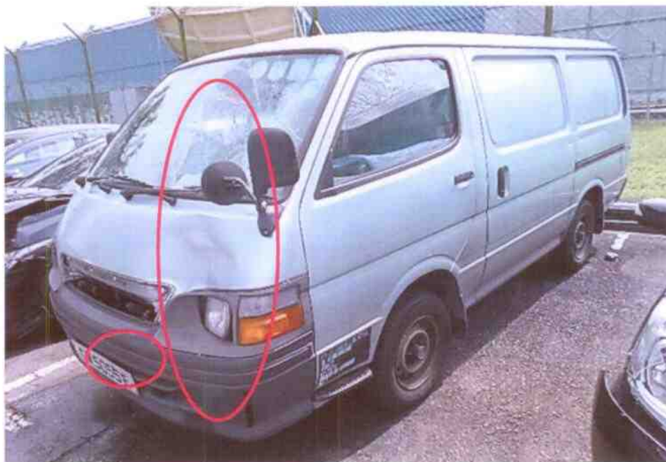
Photo 2 shows a general view of the front left body of the Motor Van at the time of my inspection. The Motor Van was observed to have sustained damages at its left panel, front left wiper panel, front grille, were amongst the body parts that were damaged as a result of the accident. Its front windscreen was also broken at the left bottom area. Its left panel was observed to sustained scratches.
