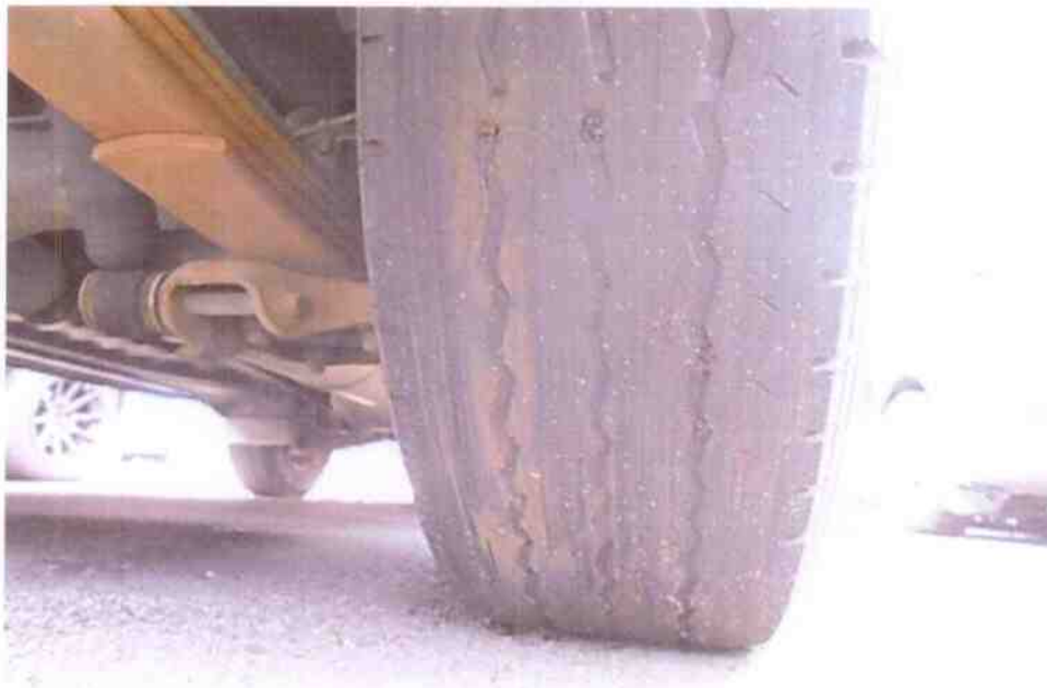
Photo 11 shows the condition of the rear right tyres of the Motor Van, which were observed to be in serviceable condition with remaining, tread depth of approximately 1.6mm. There was also no tear, cut or burst mark(s) on the outer and the inner sidewalls as well as across the tread of the 4 tyres that were fitted on the Motor Van.
