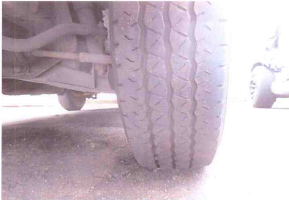
Photo 8 shows the condition of the front left tyre of the Motor Van, which was observed to be in serviceable condition with remaining tread depth of approximately 6mm.
