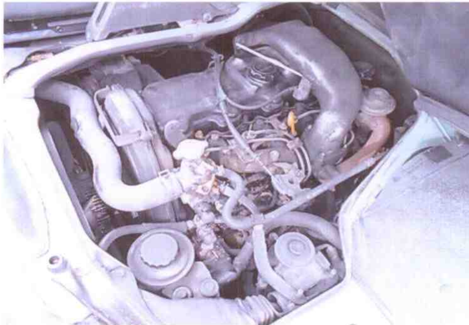
Photo 12 shows a general view of the Motor Van's engine compartment, which was accessed by lifting the passenger's seat of the Motor Van. The various parts and components inside the engine compartment were unaffected by the accident. There was also no sign(s) or indication(s) of fresh fluid leakage and/or fluid stain within the engine compartment except oil stain was observed to be pre-existed prior the accident looking at the dust accumulated with it.
