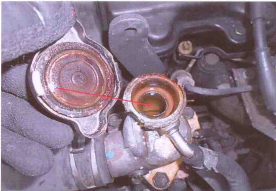
Photo 14 shows the radiator coolant reservoir of the Motor van at the time of our inspection. The radiator coolant was observed to be of sufficient level and without any visible contamination.
