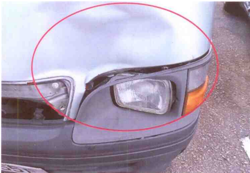
Photo 4 shows the damage sustained on the front left panels & headlamp as a result of the accident.
