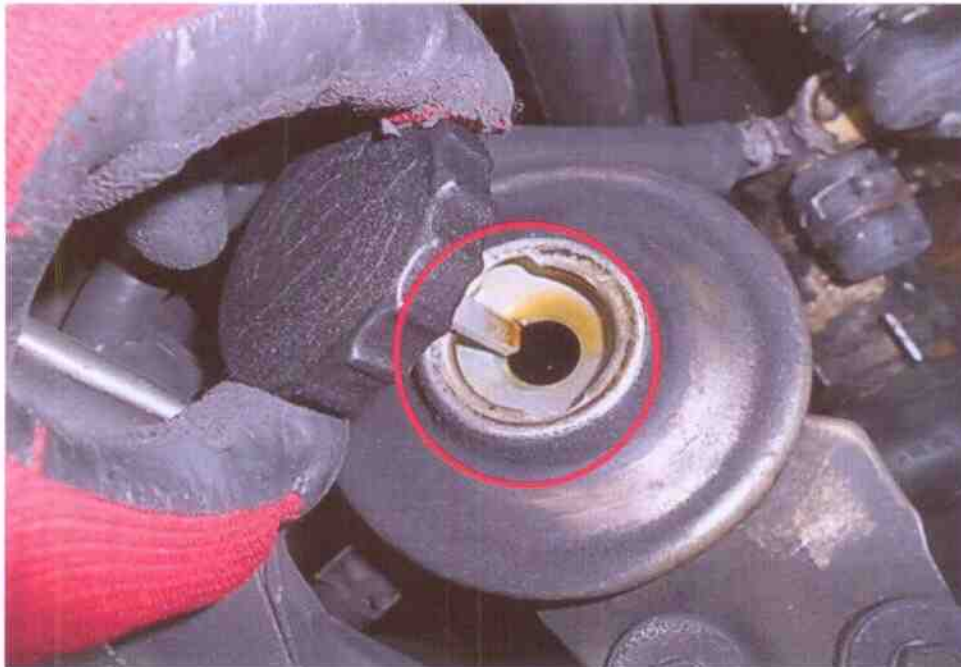
Photo 15 shows the power steering fluid reservoir of the Motor Van at the time of our inspection. The power steering fluid (circled) was observed to be of sufficient level and without any visible contamination.
