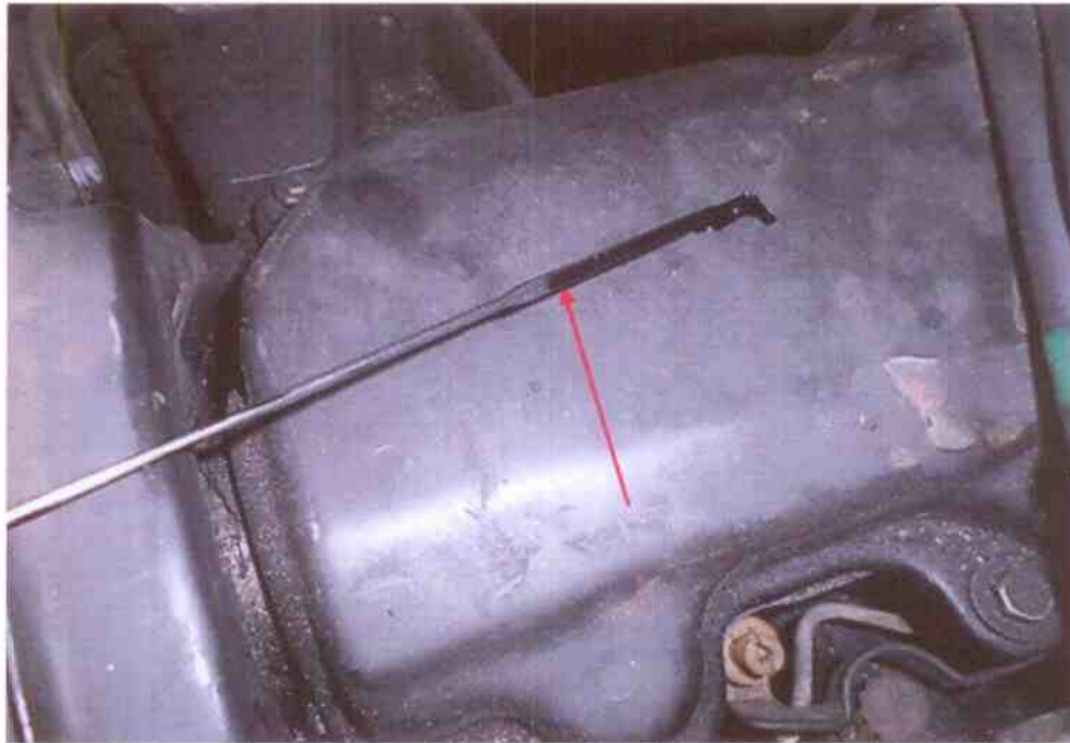
Photo 17 shows the close-up view engine dip stick of the Motor Van at the time of our inspection. The engine oil was observed to be of sufficient level and without any visible contamination (arrowed).
