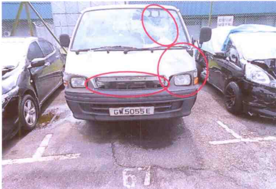
Photo 1 shows a general view of the front left body of the Motor van at the time of our inspection. The Motor Van was observed to have sustained damages at its front left panel and front grille was amongst the body parts that were damaged as a result of the accident. Its front windscreen was also broken at the left area (circled).
