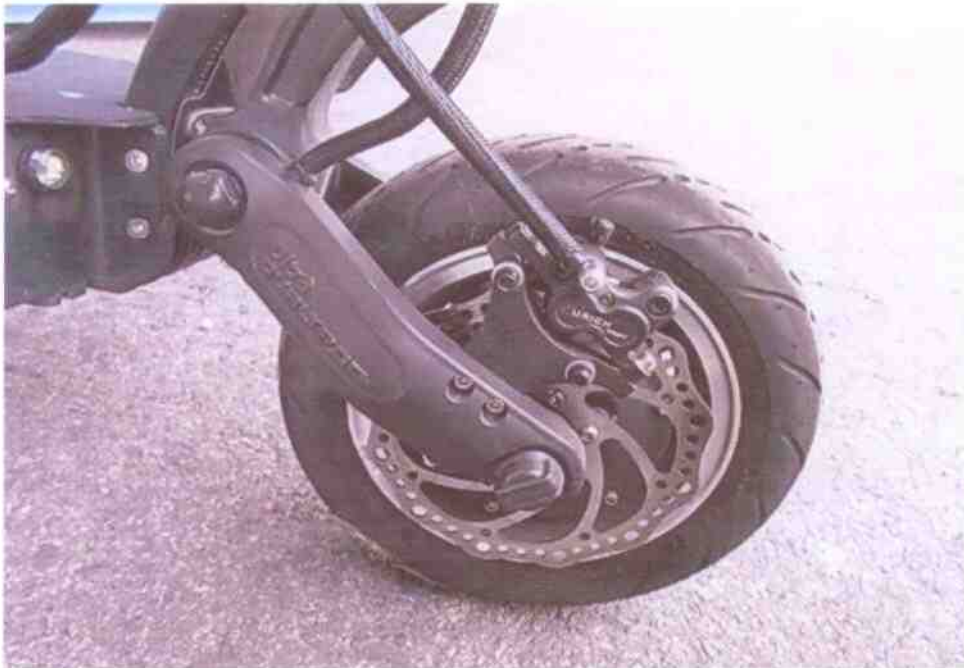
Photo 6 shows the front tyre of the Electric Scooter at the time of our inspection. The tread pattern of the 2 tyres was clearly visible. We did not observe any tear, burst mark(s) and/or punctured hole(s) on the sidewalls.
