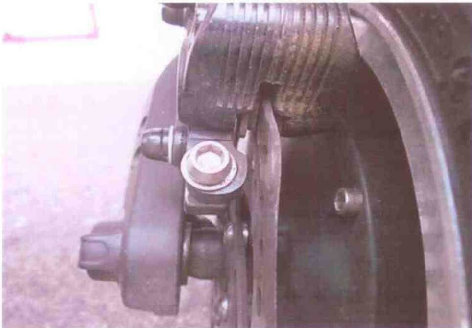
Photo 9 shows the front brake callipers (brake pad), revealed that it was in a serviceable condition.
