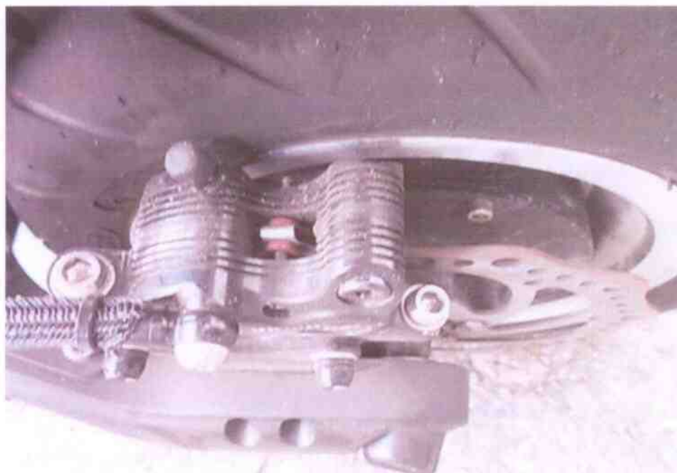
Photo 10 shows the rear brake callipers (brake pad), revealed that it was in a serviceable condition.
