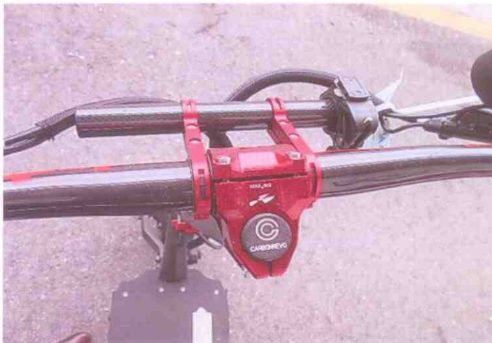
Photo 7 shows steering components of the Electric Scooter had revealed that its steering system was in serviceable condition & its front fork was found to be intact and undamaged. It was observed to be able to turn to full left & full right.
