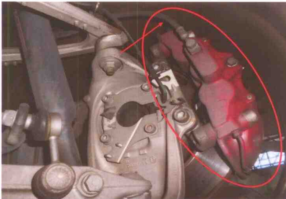
Photo 14 shows the brake hose/pipe (arrowed) at the front right wheel of the Motor Car. No leakage of brake fluid was observed. Visual examination of the various components of the braking system like the brake caliper (circled), brake booster, brake pedal etc had revealed all to be intact and without visible damage.
