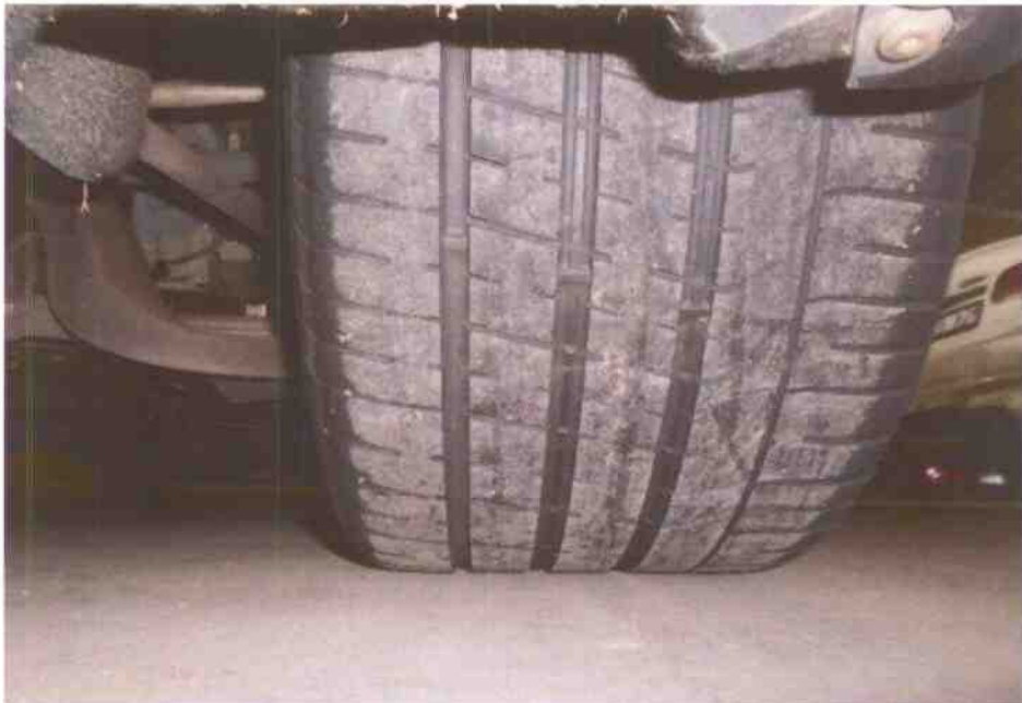
Photo 7 shows the condition of the rear right tyre of the Motor Car, which was observed to be in serviceable condition with remaining tread depth of approximately 4mm. There was also no tear, cut or burst mark(s) on the outer and the inner sidewalls as well as across the tread of the Motor Car's 4 tyres.
