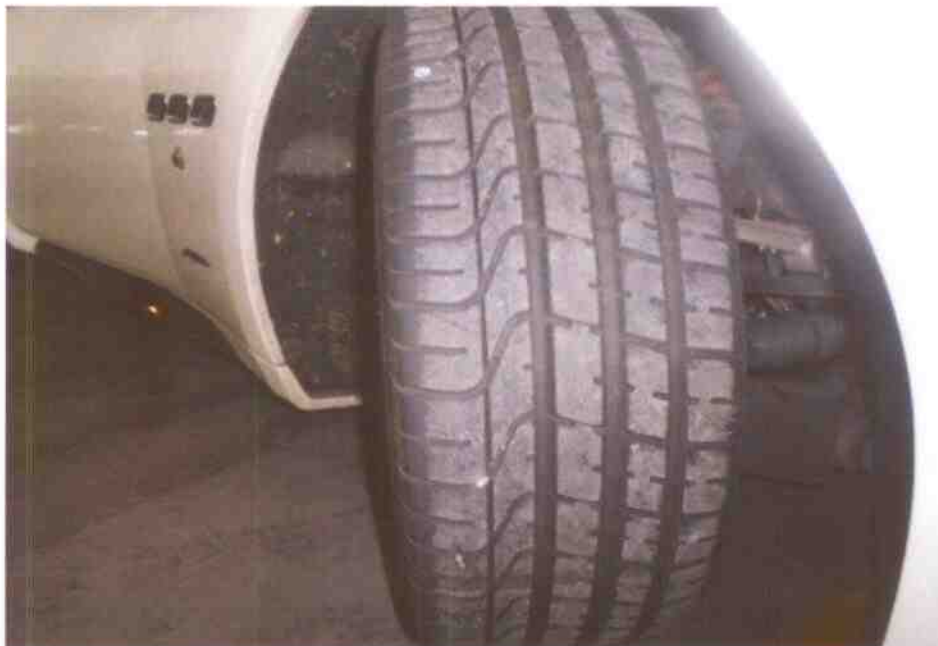
Photo 5 shows the condition of the front right tyre of the Motor Car, which was observed to be in serviceable condition with remaining tread depth of approximately 5mm. The tyre, which was wrapped around alloy wheel rim, was also observed to be sufficiently inflated for vehicular operation.
