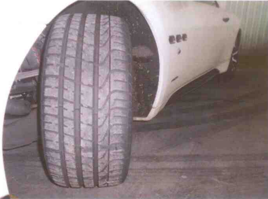
Photo 4 shows the condition of the front left tyre of the Motor Car, which was observed to be in serviceable condition with remaining tread depth of approximately 5mm. The tyre was wrapped around alloy wheel rim that was found to be without any visible damage. The tyre was also observed to be sufficiently inflated for vehicular operation with no tear, cut or burst mark(s) on the outer and the inner sidewalls as well as across the tread.
