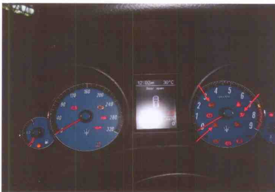
Photo 18 shows the warning lights for the various electronic operating systems of the Motor Car appearing on its instrument panel during the self-test when the engine is cranked, in particular the ABS light, DSC light and SRS light (arrowed).
