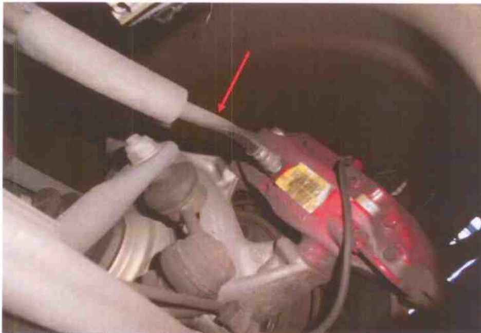
Photo 13 shows the brake hose/pipe (arrowed) at the rear left wheel of the Motor Car. I did not observe any leakage of brake fluid at the time of my inspection of the Motor Car. Static tests of the Motor Car's braking system had indicated that there was no internal leakage of pressure/vacuum. The undercarriage components of the Motor Car were also all found to be intact and without any visible damage.
