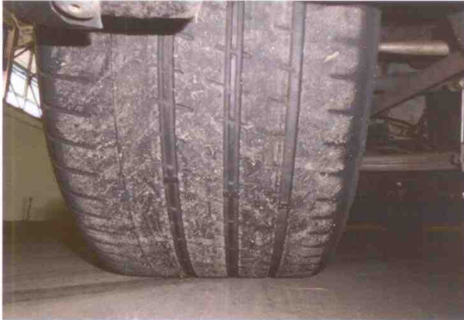
Photo 6 shows the condition of the rear left tyre of the Motor Car, which was observed to be in serviceable condition with remaining tread depth of approximately 4mm. The tyre, which was wrapped around alloy wheel rim, was also observed to be sufficiently inflated for vehicular operation. There was also no visible damage found on the 4 wheel rims of the Motor Car.
