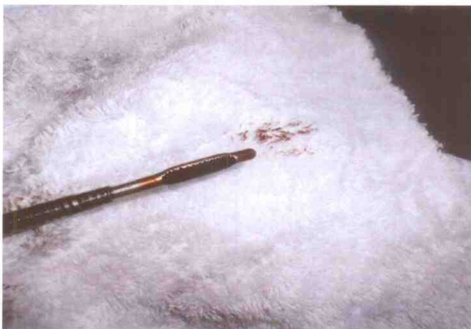
Photo 12 shows the engine oil dip stick of the Motor Car at the time of my inspection. The engine oil was observed to be of sufficient level and without any visible contamination.
