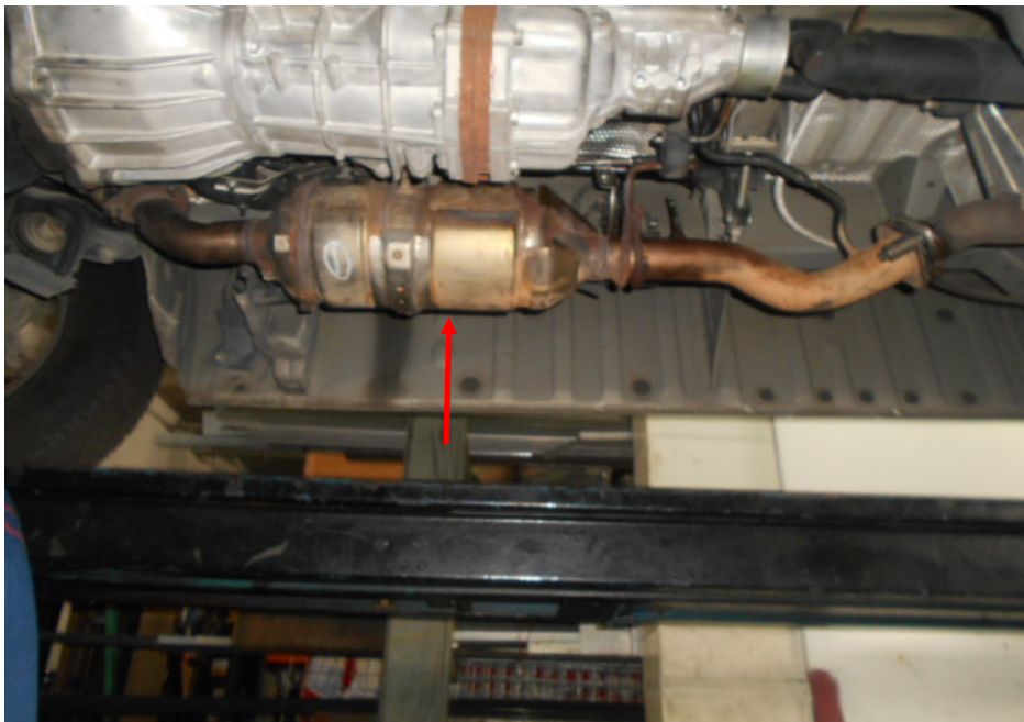
Photo 2 shows a general view of the motor van's Diesel Particulate Filter (DPF). The DPF (arrowed) was noted to be without any visible damage to its exterior body.
