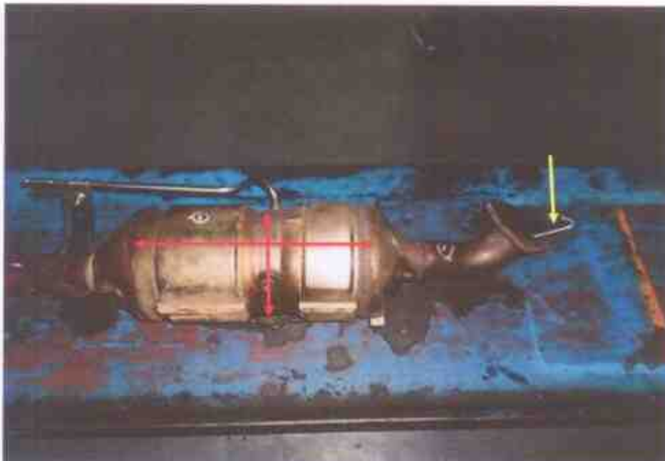
Photo 5 shows the metal strip (yellow arrow) was able to be inserted from one side of the DPF to the other side (horizontal red arrow). I was also able to move the metal strip sideways (vertical red arrow), from one side of the inner wall to the other side of the inner wall, inside the DPF. This would indicate that the filter element inside the DPF was removed.
