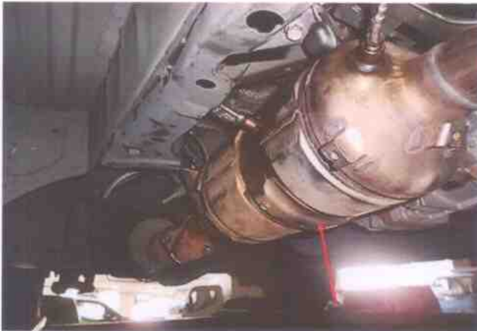
Photo 3 shows a general view of the motor van's Diesel Particulate Filter (DPF). The DPF (arrowed) was noted to be without any visible damage to its exterior body.
