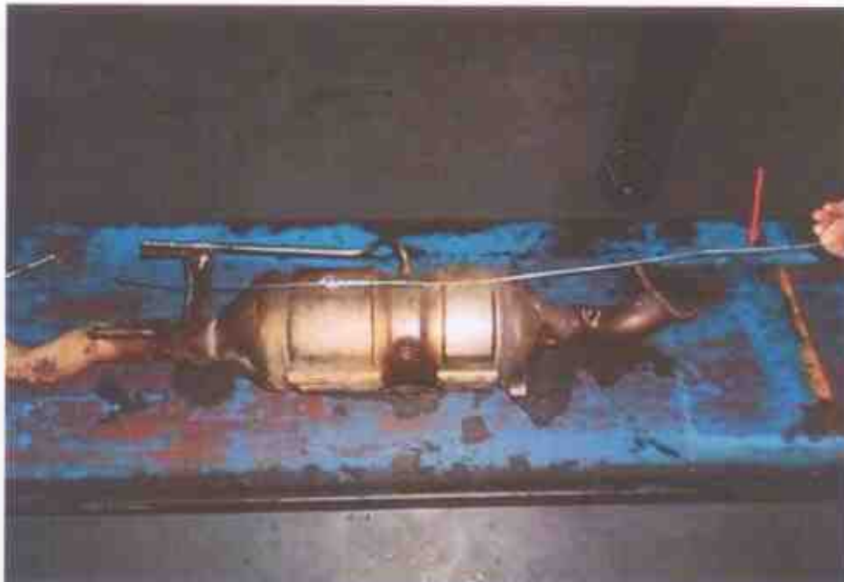
Photo 4 shows the motor van's DPF removed for further checks. A long metal strip (arrowed) was able to be inserted from one side of the DPF to the other side. I was also able to move the metal strip sideways, from one side of the inner wall to the other side of the inner wall, inside the DPF. This would indicate that the filter element inside the DPF was removed.
