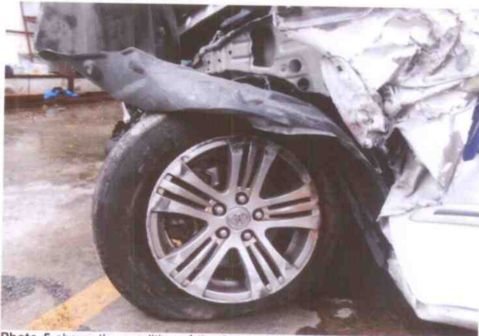
Photo 5 shows the condition of the front left tyre of the Police Car, which was observed to be deflated. The outer sidewall of the tyre was found to be cut. The wheel rim was also observed to be broken with marks of grazing nature on its outer spokes, all of which were a result of the accident.
