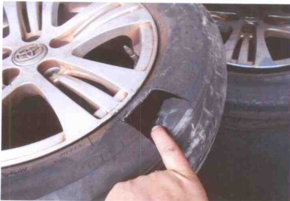
Photo 11 shows the cut observed on the outer sidewall of one of the tyres that were found in the rear boot compartment of the Police Car. The cut to the tyre and damage to the wheel rim were both arising from the accident.
