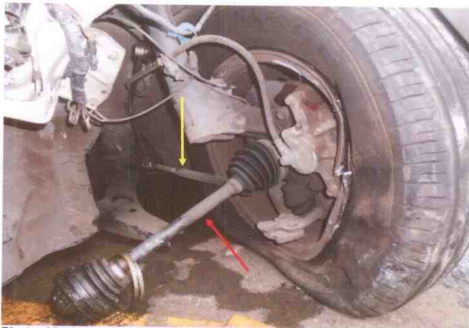
Photo 18 shows the undercarriage components at the front left wheel of the Police Car. My checks on the underside of the Police Car revealed damage to the undercarriage components at the front left wheel of the Police Car. Components like the front left suspension, front left lower arm, front left drive shaft (red arrow), front stabilizer bar and front left steering tie rod (yellow arrow) were all found to be have been damaged.
