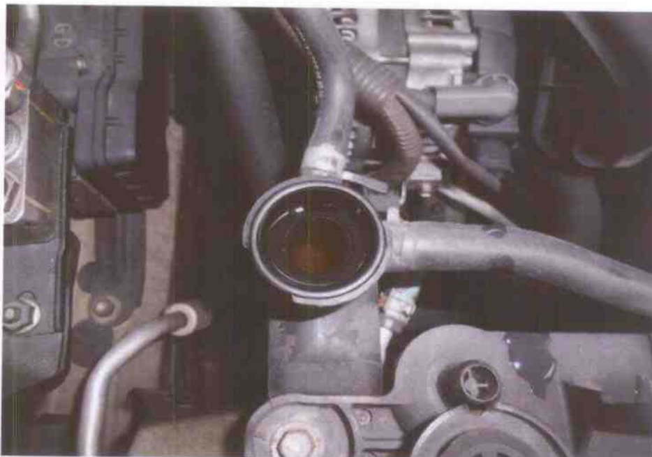
Photo 15 shows checks being carried out to the engine coolant of the Police Car at the time of my inspection. The engine coolant was observed to be of sufficient level and without any visible contamination.
