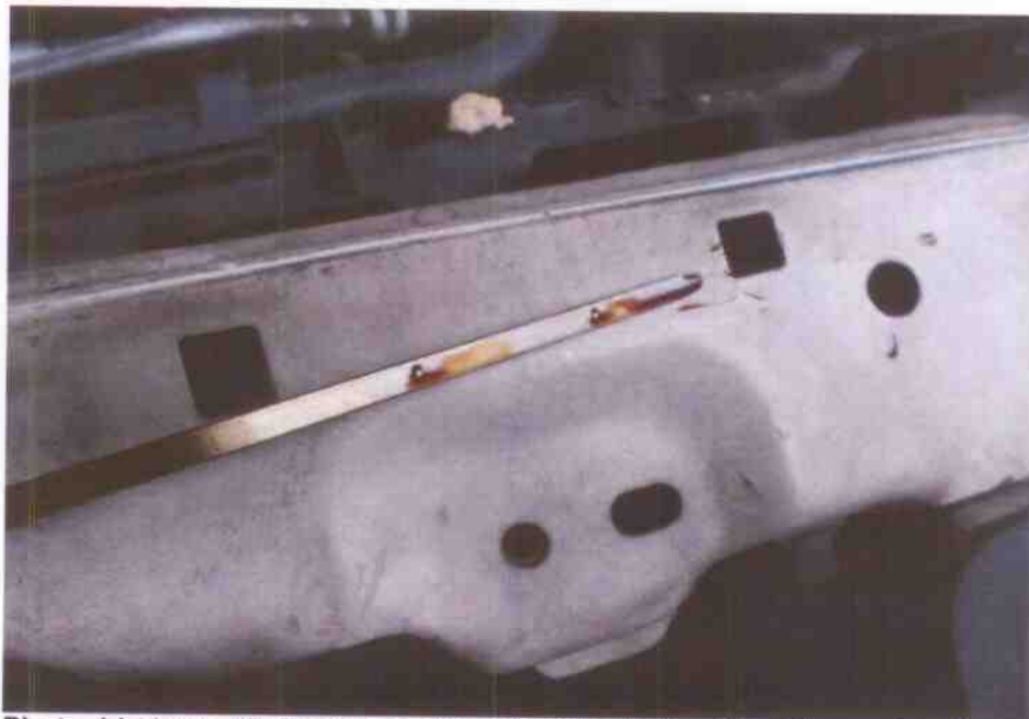
Photo 14 shows the engine oil dip stick of the Police Car. The engine oil was found to be sufficient level and without contamination for operating purposes.
