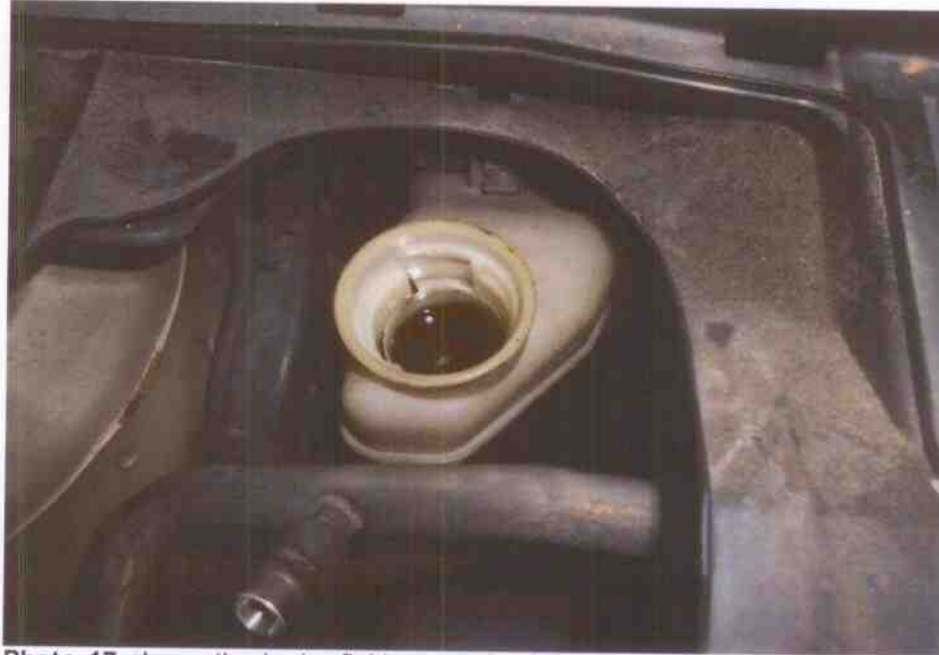
Photo 17 shows the brake fluid reservoir of the Police Car at the time of my inspection. The brake fluid was observed to be of sufficient level and without any visible contamination.
