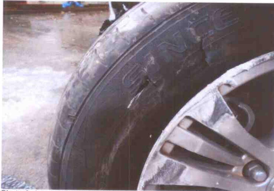
Photo 6 shows a closer view of the outer sidewall of the front left tyre, where the rubber was found to be cut. The wheel rim was also observed to be broken with marks of grazing nature on its outer spokes, all of which were a result of the accident.
