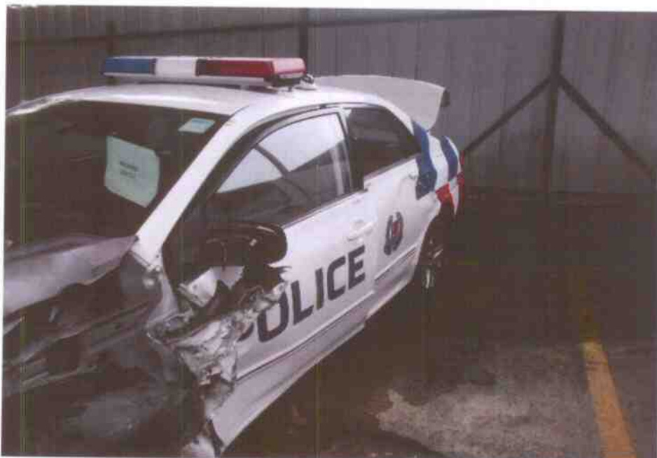
Photo 2 shows a closer view of the extent of damage along the left body of the Police Car. Its left wing mirror, front left fender and front left door were amongst the body parts that were severely damaged as a result of the impact force.
