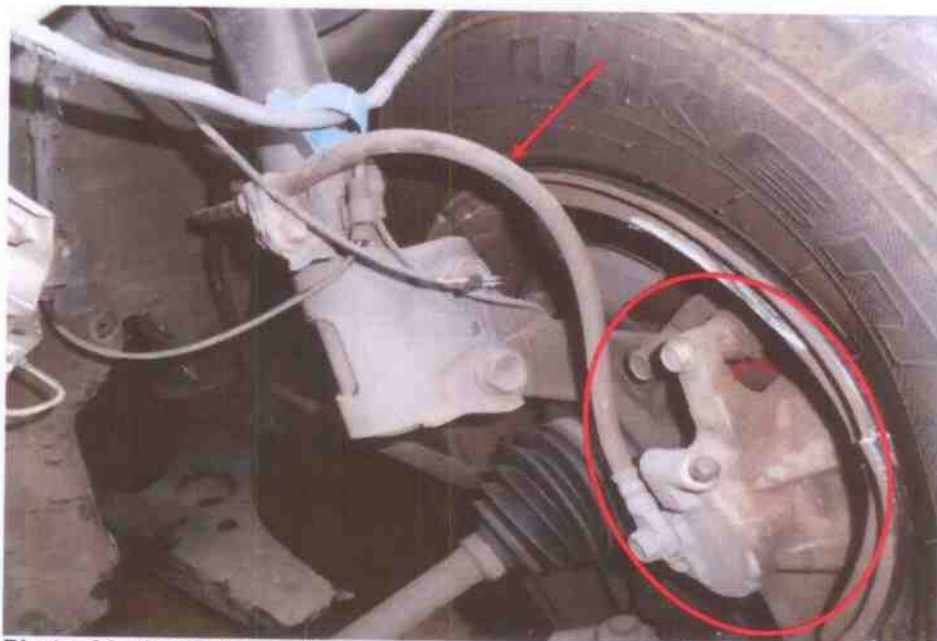
Photo 21 shows the undercarriage components at the front left wheel of the Police Car, in particular the brake hose (arrowed) and brake caliper (circled). The Police Car's braking system was likely to be in serviceable condition as my visual examination of the various mechanical parts in the braking system did not produce any observations that had suggested otherwise. This was also taking into consideration that the brake fluid was of sufficient level for operating purposes.
