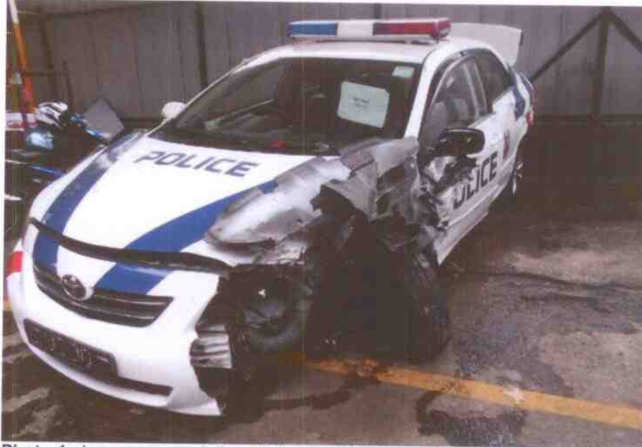
Photo 1 shows a general view of the front left body of the Police Car at the time of my inspection. The Police Car was observed to have sustained extensive impact damage along its left body. The impact force was relatively significant causing severe damage to its front bumper, front left headlamp, front left fender, front left wheel house, front bonnet and front left door amongst others.
