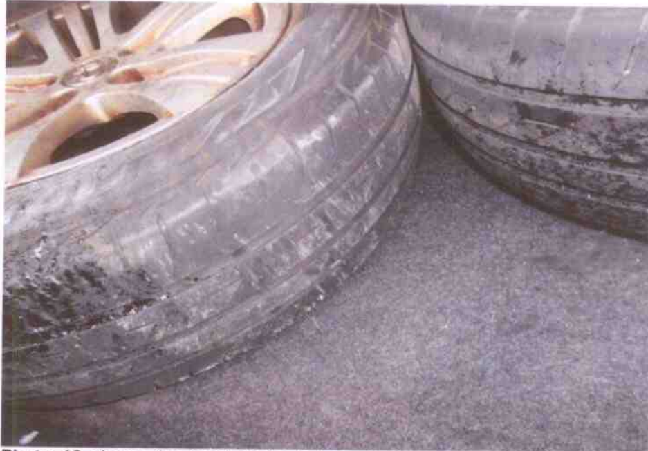
Photo 12 shows the tread of the 2 tyres that were found in the rear boot compartment of the Police Car. Although the 2 tyres were found to be deflated, both tyres can still be considered to be in serviceable condition prior to the accident as the remaining tread depth of the tyres were approximately 5mm with its tread pattern clearly visible.
