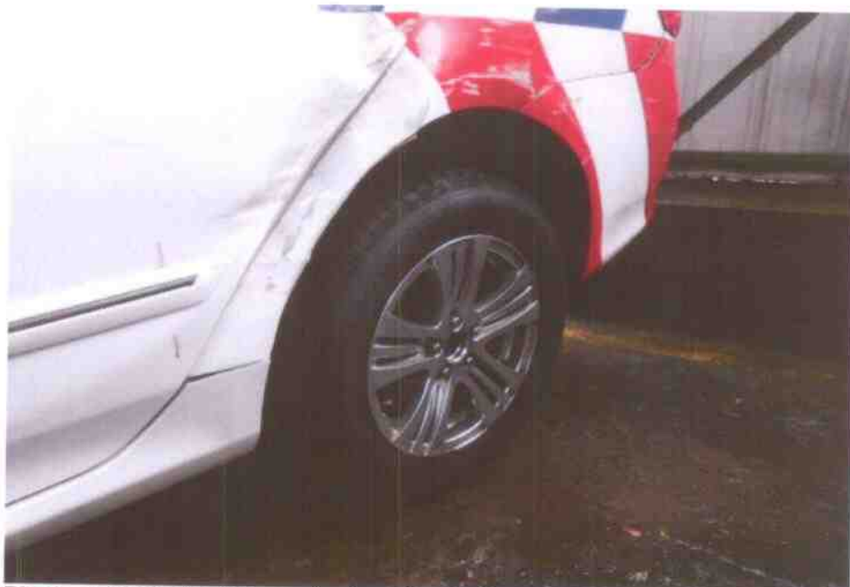
Photo 3 shows the left rear body of the Police Car. Its rear left door, left rear fender and rear bumper had also sustained damage arising from the accident.
