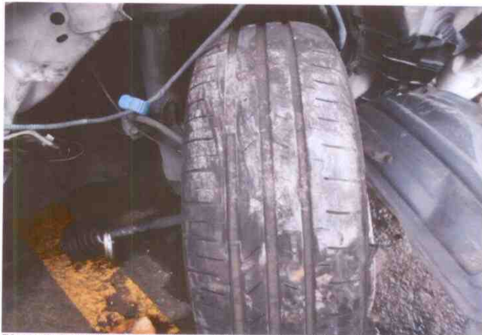
Photo 7 shows the tread of the front left tyre of the Police Car. Although the front left tyre was found to be deflated, it can still be considered to be in serviceable condition prior to the accident as the remaining tread depth of the tyre was approximately 5mm with its tread pattern clearly visible.
