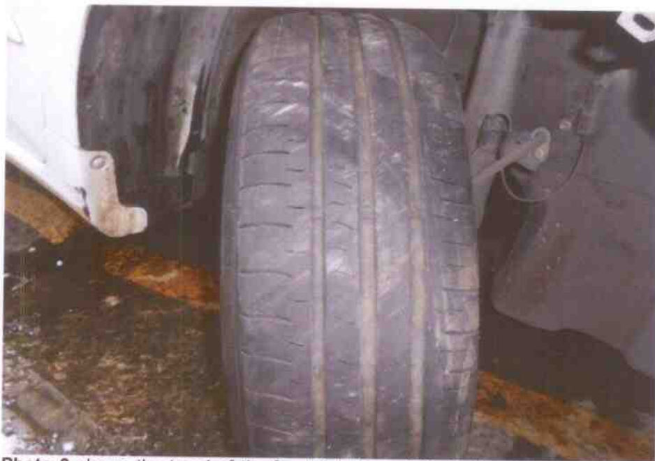
Photo 9 shows the tread of the front right tyre of the Police Car. Although the front right tyre was found to be deflated, it can still be considered to be in serviceable condition prior to the accident as the remaining tread depth of the tyre was approximately 5mm with its tread pattern clearly visible.
