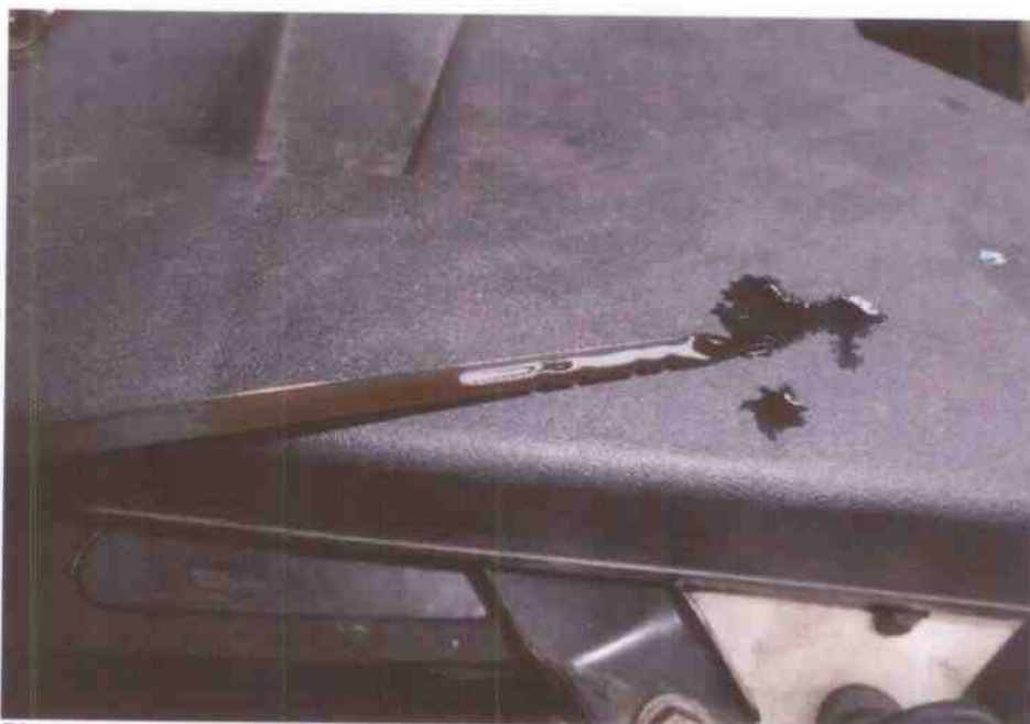
Photo 16 shows the transmission fluid dip stick of the Police Car. The transmission fluid was found to be sufficient level and without contamination for operating purposes.
