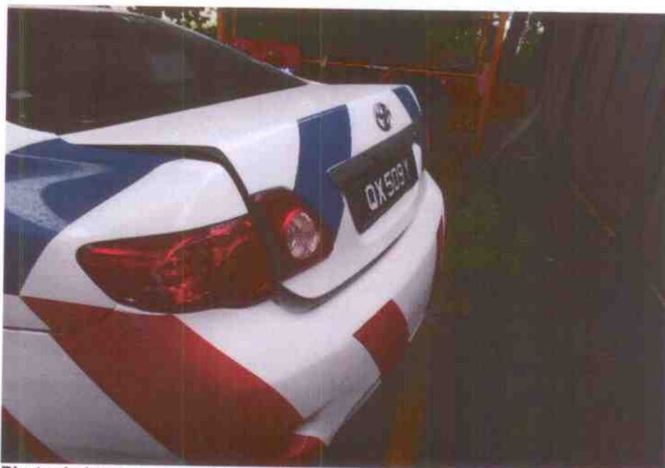
Photo 4 shows a general view of the rear body of the Police Car. The rear body and right side body of the Police Car were observed to be relatively unaffected from the accident.
