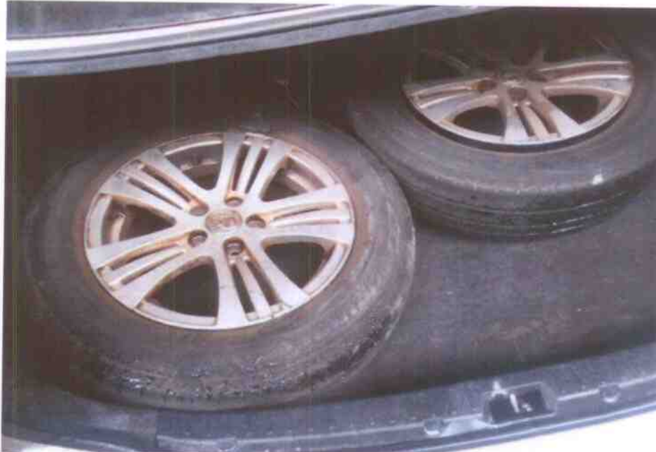
Photo 10 shows the 2 rear tyres of the Police Car that were found in the rear boot compartment. Both the tyres were found to be wrapped around their wheel rims and deflated. Both wheel rims were also found to be damaged as a result of the accident, with marks of grazing nature on their outer spokes.
