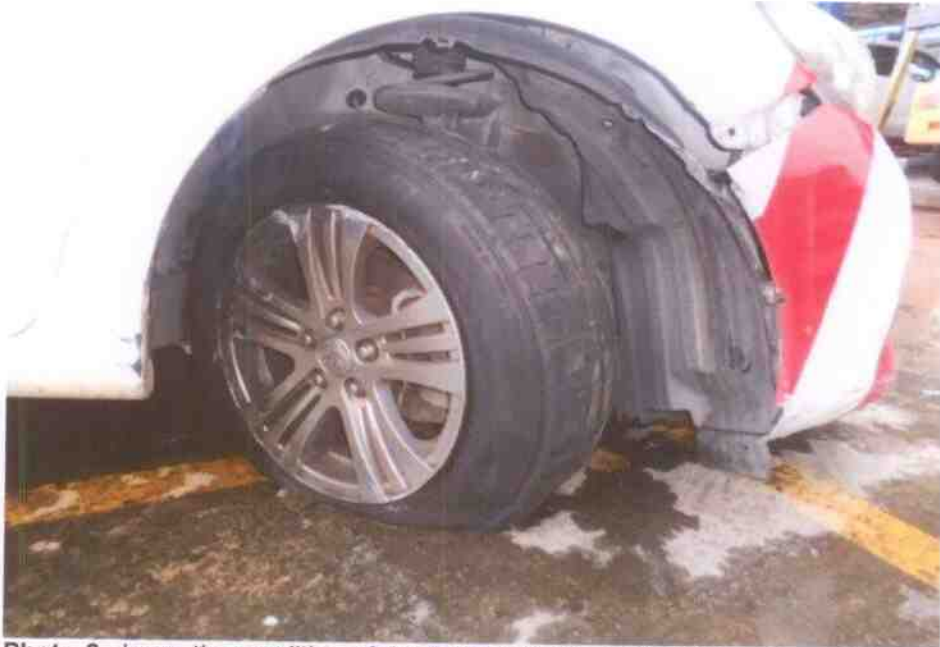
Photo 8 shows the condition of the front right tyre of the Police Car, which was observed to be deflated. The front right wheel rim was also observed to be damaged with marks of grazing nature on its outer spokes. The deflation of the tyre and damage to the wheel rim were both a result of the accident.
