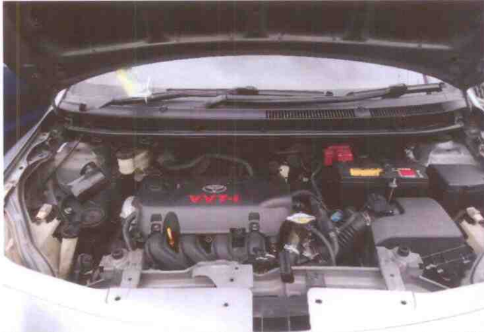
Photo 9 shows a general view of the Motor Car's engine compartment. The various parts and components inside the engine compartment were unaffected by the accident. There was also no sign(s) or indication(s) of fluid leakage and/or fluid stain within the engine compartment.
