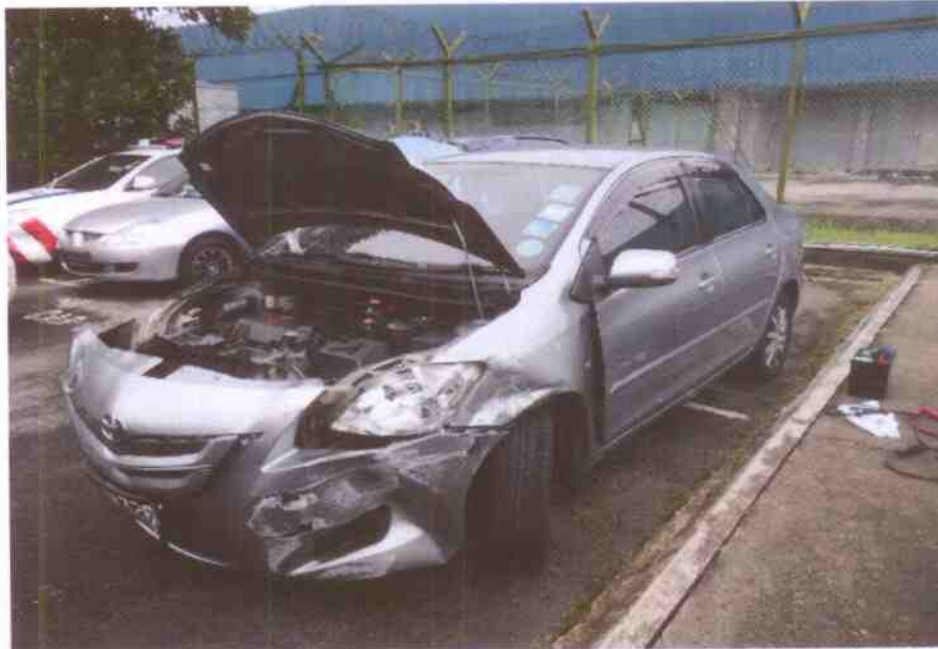
Photo 16 shows the front left wheel of the Motor Car turned to its full left. During my steering system test, I did not experience any abnormal free play and/or resistance when I had turned the steering wheel towards the left and right. This would suggest that the steering system of the Motor Car was likely to be in serviceable condition at the material time of accident.
