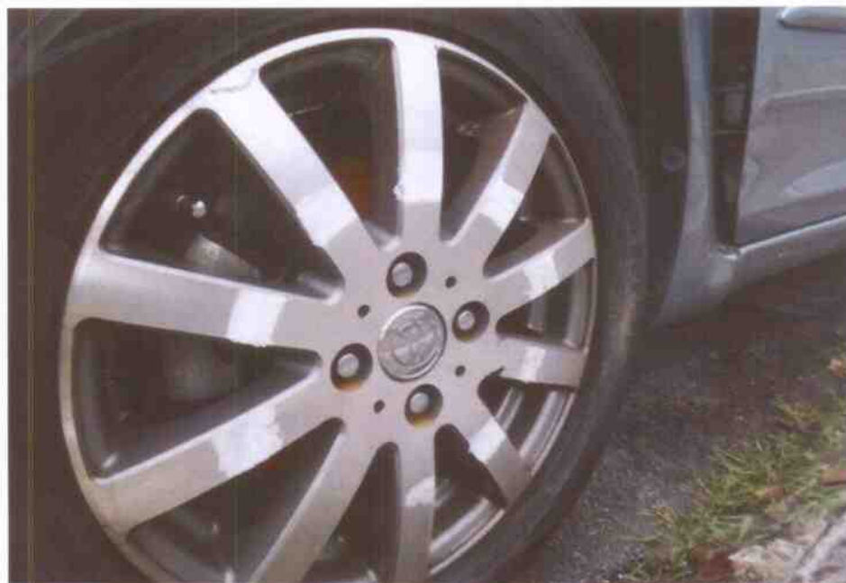
Photo 5 shows the front left wheel rim of the Motor Car. Fresh marks of grazing nature were observed on the outer spokes of the front left wheel rim.
