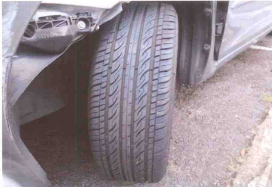
Photo 4 shows the condition of the front left tyre of the Motor Car, which was observed to be in serviceable condition with remaining tread depth of approximately 6mm. The tyre was wrapped around alloy wheel rim that was found to be with grazed marks on the outer spokes. The tyre was also observed to be sufficiently inflated for vehicular operation with no tear, cut or burst mark(s) on the outer and the inner sidewalls as well as across the tread.
