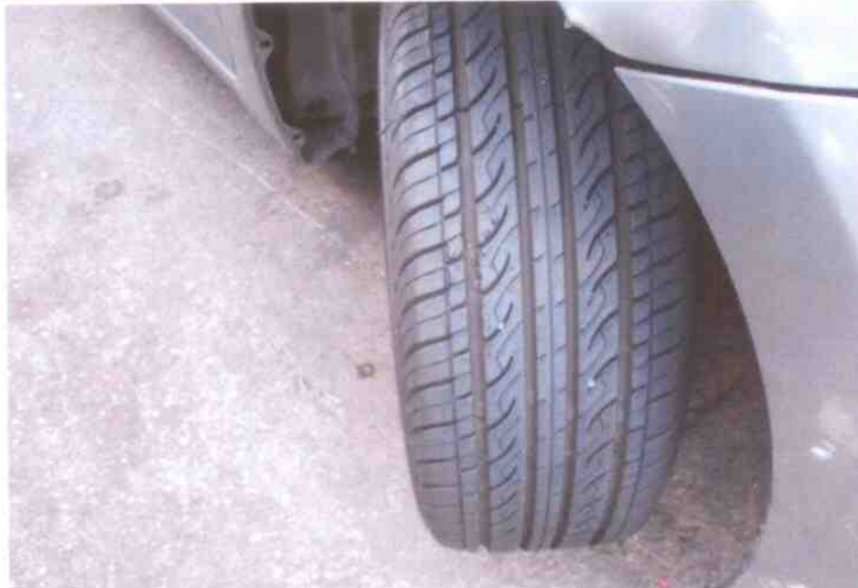
Photo 6 shows the condition of the front right tyre of the Motor Car, which was observed to be in serviceable condition with remaining tread depth of approximately 6mm. The tyre, which was wrapped around alloy wheel rim, was also observed to be sufficiently inflated for vehicular operation.
