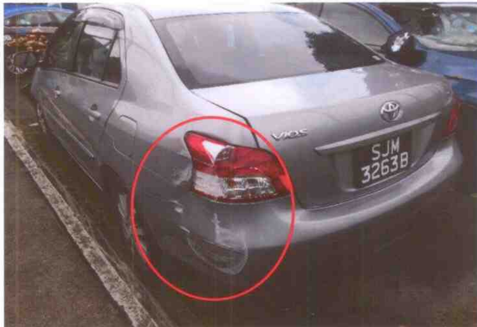
Photo 3 shows a general view of the Motor Car's rear left body at the time of my inspection. The rear bumper, left rear fender and rear left tail lamp of the Motor Car had sustained damage arising from the accident.
