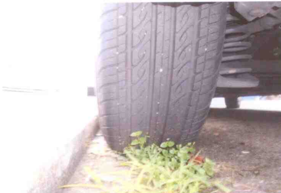
Photo 7 shows the condition of the rear left tyre of the Motor Car, which was observed to be in serviceable condition with remaining tread depth of approximately 6mm. The tyre, which was wrapped around alloy wheel rim, was also observed to be sufficiently inflated for vehicular operation. There was also no damage found on the 4 wheel rims of the Motor Car except for the front left wheel rim, which was damaged as a result of the accident.
