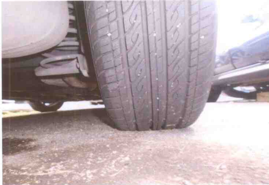
Photo 8 shows the condition of the rear right tyre of the Motor Car, which was observed to be in serviceable condition with remaining tread depth of approximately 6mm. There was also no tear, cut or burst mark(s) on the outer and the inner sidewalls as well as across the tread of the Motor Car's 4 tyres.
