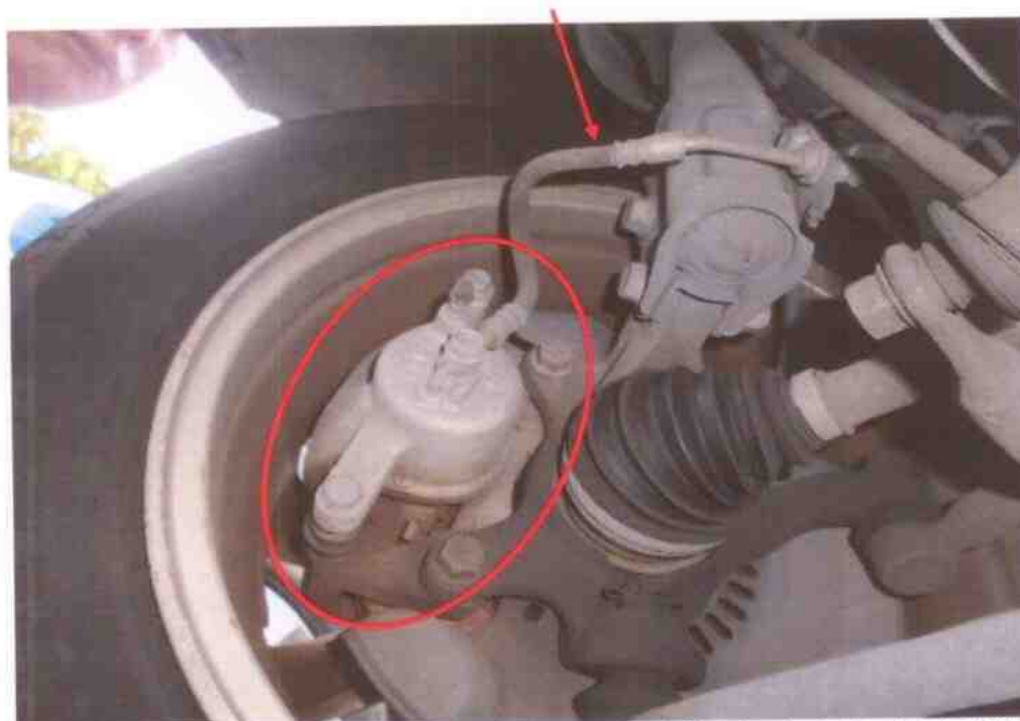
Photo 15 shows the brake hose/pipe (arrowed) at the front right wheel of the Motor Car. No leakage of brake fluid was observed. Visual examination of the various components of the braking system like the brake caliper (circled), brake booster, brake pedal etc had revealed all to be intact and without visible damage.
