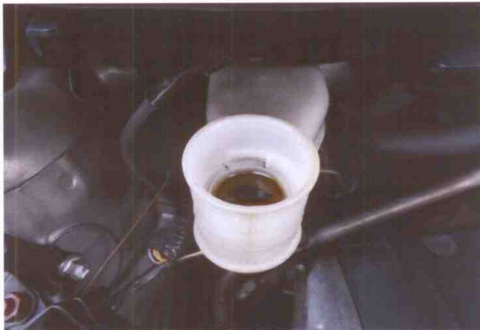
Photo 10 shows the brake fluid reservoir of the Motor Car at the time of my inspection. The brake fluid was observed to be of sufficient level and without any visible contamination.
