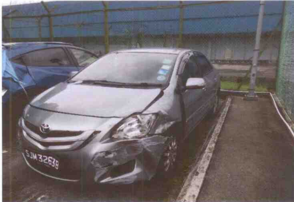
Photo 2 shows a general view of the front left body of the Motor Car at the time of my inspection. The front left body and left front body of the Motor Car were also damaged as a result of the accident. Body parts like the front bonnet, front left fender and front left headlamp were damaged.
