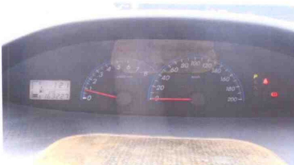
Photo 20 shows no warning lights illuminated on the instrument panel of the Motor Car after the engine was cranked. This would suggest that there was no abnormality to the various electronic operating systems of the Motor Car, like the ABS, PS and SRS etc.
