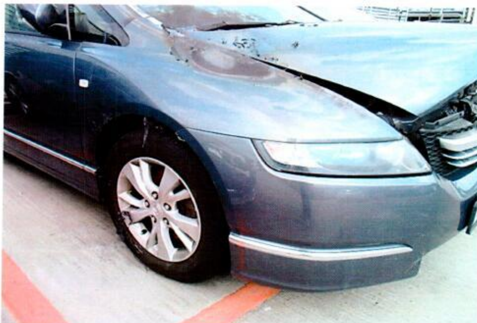
Photo 2 shows the general view of the front right portion of the Insured Vehicle at the time of our inspection. The fire damage to the Insured Vehicle was confined to its front portion. Its front bonnet and right side panel were amongst the body parts that were found to have been affected as a result of the fire.
