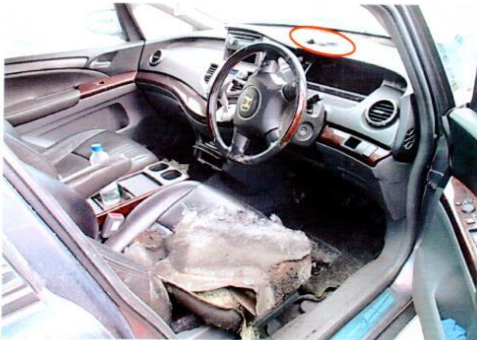
Photo 6 shows the interior compartment of the Insured Vehicle, which was observed to be partially burnt and/or melted. The dashboard (circled) and front windscreen were amongst the parts that were found to have been partially burnt and/or melted as a result of the fire.
