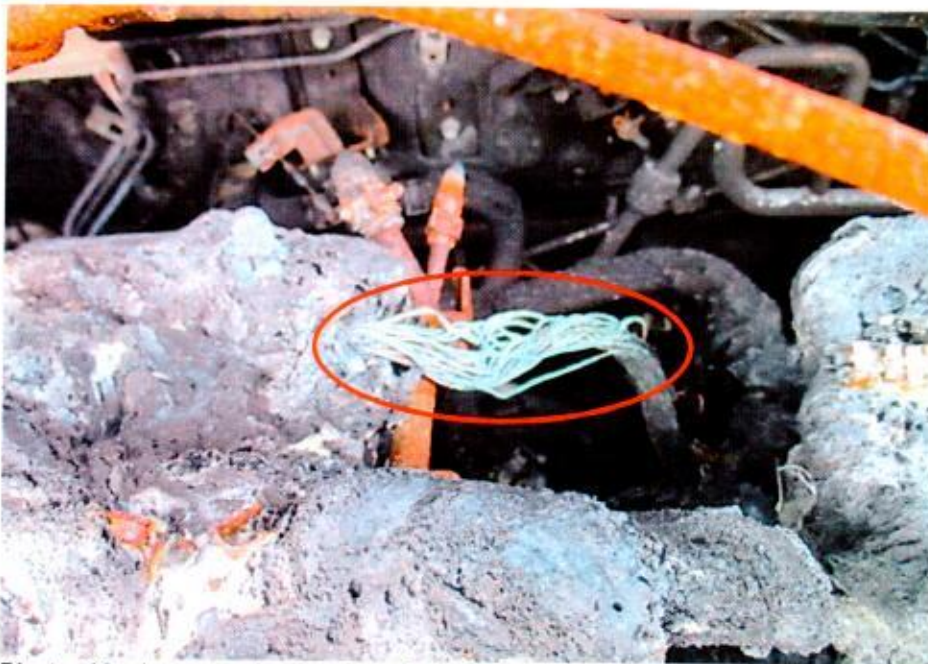
Photo 13 shows a closer view of the greenish residue found on the wirings (circled) at the rear centre portion of the engine compartment. The presence of such greenish residue suggests occurrence of an electrical short circuit.
