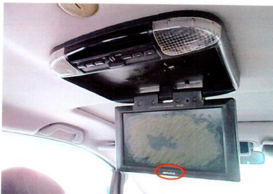
Photo 8 shows the in-car flip-down monitor which had sustained minor fire damage. The brand of the in-car flip-down monitor was 'ALPINE' (circled).
