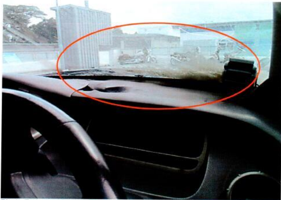
Photo 7 shows a closer view of the damaged front windscreen and dashboard of the Insured Vehicle (as viewed from the interior compartment).
