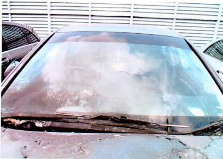
Photo 4 shows the general view of the front windscreen of the Insured Vehicle at the time of our inspection. The fire damage to the Insured Vehicle was confined to its front portion. Its windscreen, front windscreen wipers, front wiper panel garnish and front windscreen water nozzles were amongst the body parts that were found to have been affected as a result of the fire.
