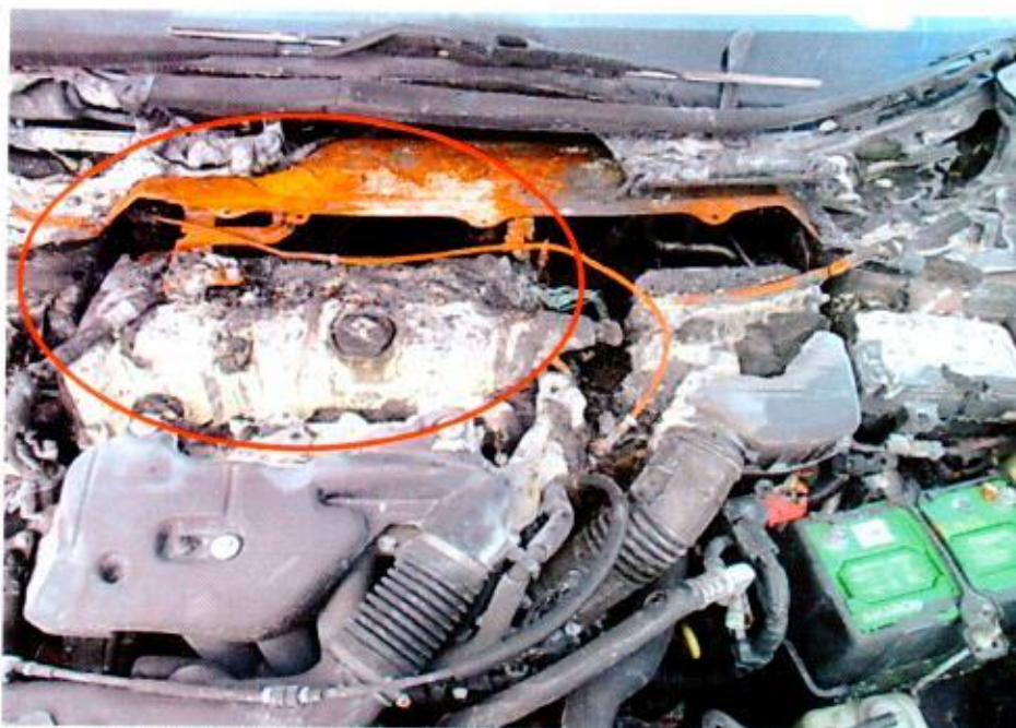
Photo 11 shows the fire extinguisher residue (circled) found on the rear centre portion of the engine compartment of the Insured Vehicle. The nature of fire damage is an indication as to where the fire started.
