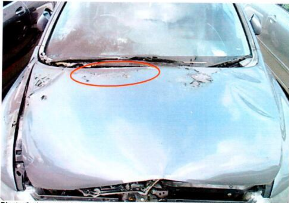
Photo 9 shows the burn pattern and whitish burn marks (circled) that were found on the rear centre side of the front bonnet of the Insured Vehicle. Such whitish burn marks are a result of exposure to prolonged heat intensity, which may indicate where the fire had started. Rust would also begin to develop on these areas soon after the fire.
