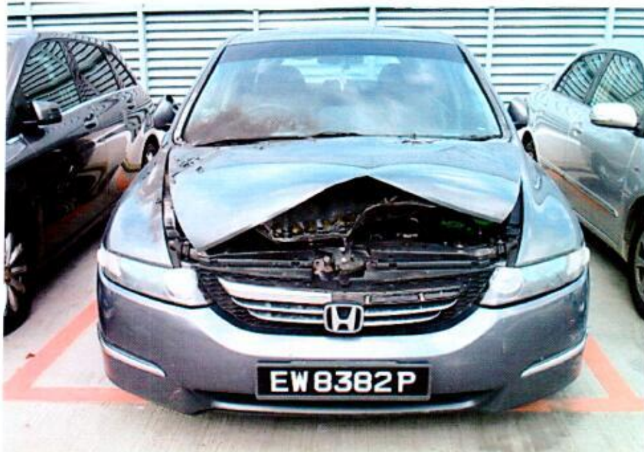
Photo 1 shows the general view of the front portion of the Insured Vehicle at the time of our inspection. The fire damage to the Insured Vehicle was confined to its front portion. Its front bonnet, front grille, front windscreen and front windscreen wipers were amongst the body parts that were found to have been affected as a result of the fire. The front bonnet of the Insured Vehicle was slightly buckled, likely due to rescue damage.
