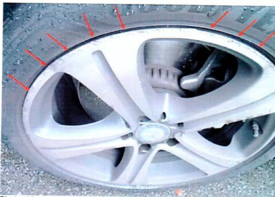
Photo 10 shows a close up view of the relatively minor marks of grazing observed on the edges of the front left wheel rim (red arrows).
