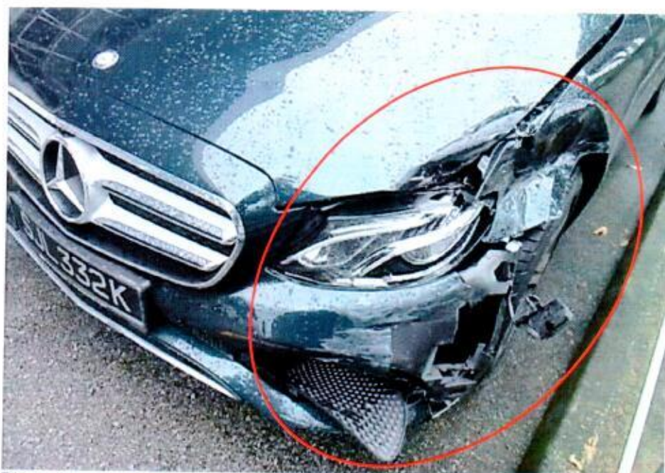
Photo 8 shows a closer view of the damaged front left portion of the Insured Vehicle. The Insured Vehicle had sustained significant damages to its left headlight, front bumper and left front panel (circled).
