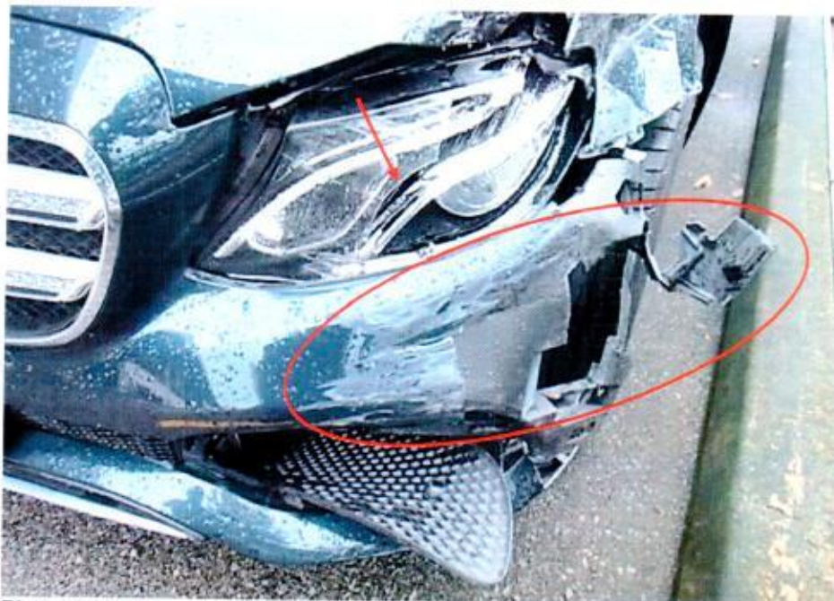
Photo 9 shows a close up view of the cracked left headlight (arrowed) and paint graze marks found on the front left portion of the front bumper which had buckled as a result of the accident (circled).
