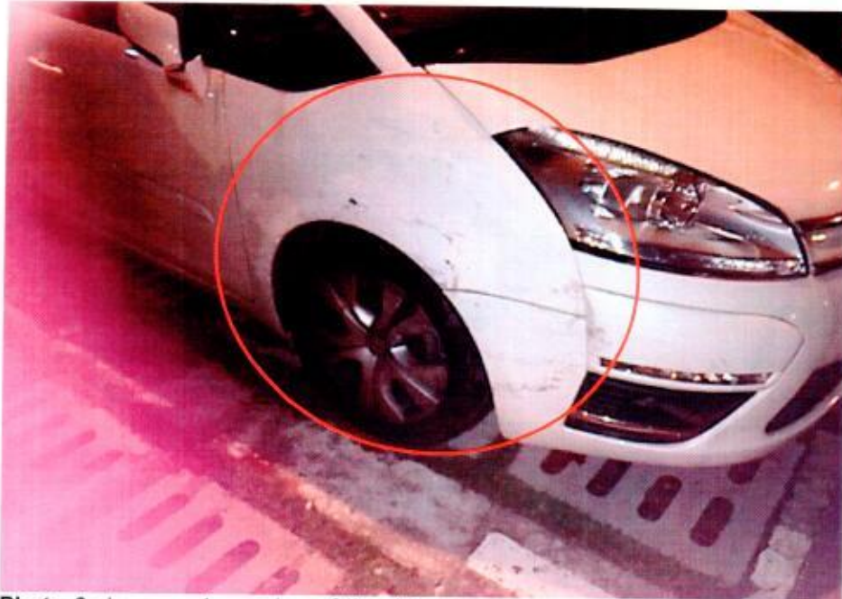
Photo 6 shows a closer view of the right side of the Citroen post- accident. We observed that the Citroen sustained dents and paint graze marks on its right front panel as well as some relatively minor marks of grazing nature on the edges of the front right wheel rim (circled).
