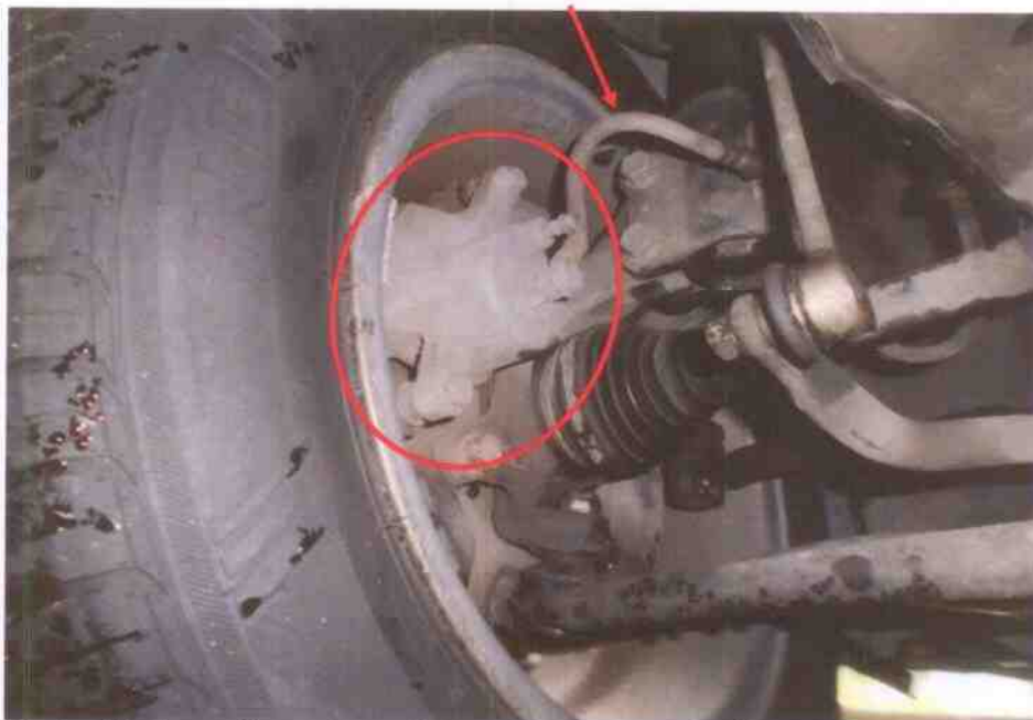
Photo 15 shows the undercarriage components at the front right wheel of the Motor Car, in particular the brake hose (arrowed) and brake caliper (circled). The Motor Car's braking system was likely to be in serviceable condition at the material time of accident as my visual examination of the various mechanical parts in the braking system did not produce any observations that had suggested otherwise. This was also taking into consideration that the brake fluid was of sufficient level for operating purposes.
