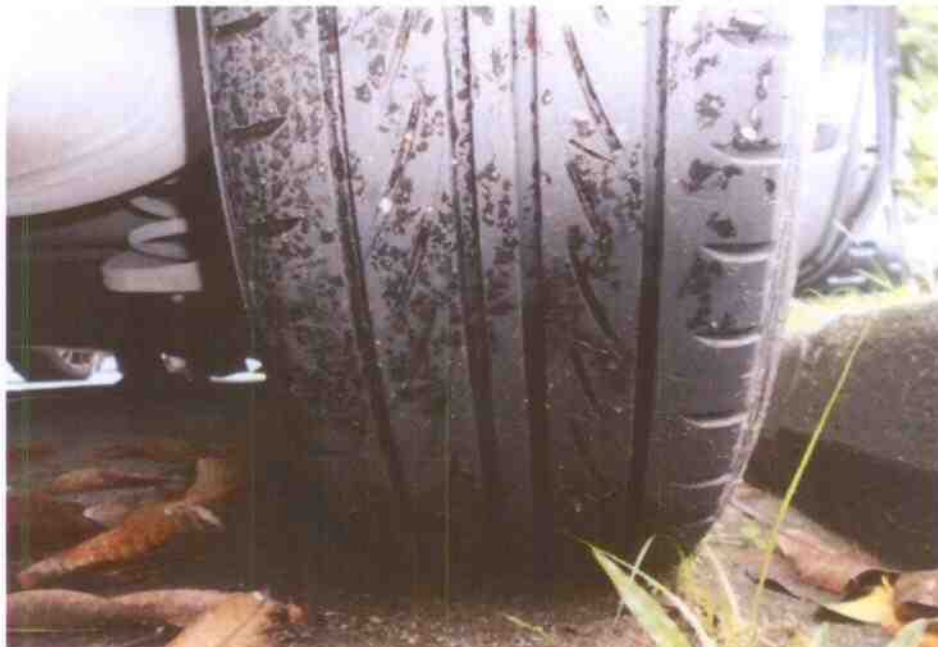
Photo 6 shows the condition of the rear right tyre of the Motor Car, which was observed to be in serviceable condition with remaining tread depth of approximately 4mm. There was no tear, cut or burst mark(s) on the outer and the inner sidewalls as well as across the tread of this tyre, which was sufficiently inflated for vehicular operation.
