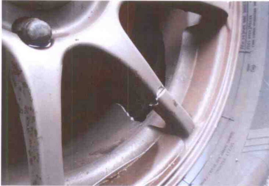
Photo 9 shows the front left wheel rim of the Motor Car was also cracked and broken as a result of the accident. The remaining 3 wheel rims were found to be without any significant damage.
