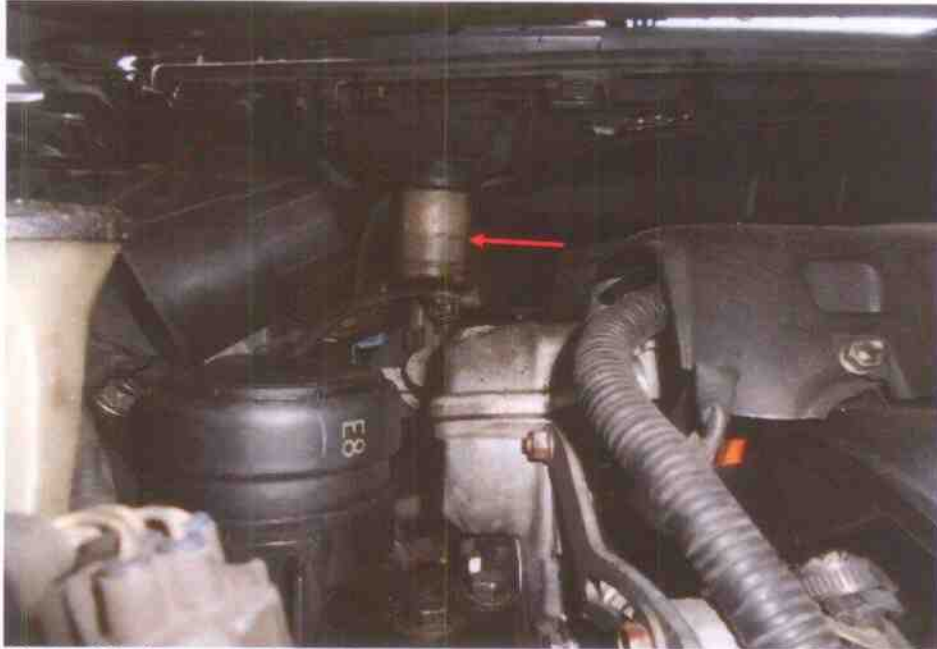
Photo 10 shows the brake fluid reservoir of the Motor Car at the time of my inspection. The brake fluid was observed to be of sufficient level for operating purposes. This was observed from gaps around the front bonnet given that the front bonnet could not be lifted for me to check the Motor Car's engine compartment.
