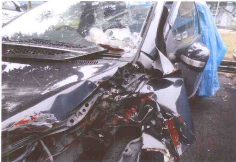
Photo 2 shows a closer view of the extent of damage at the left front body of the Motor Car. Its front bonnet, front left fender, front left wheel house and front left door were amongst the body parts that were severely damaged as a result of the impact force.
