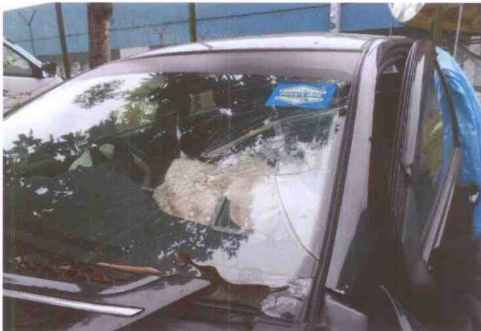
Photo 3 shows the front windscreen of the Motor Car cracked at the left side. Its front airbags were also activated as a result of the accident.
