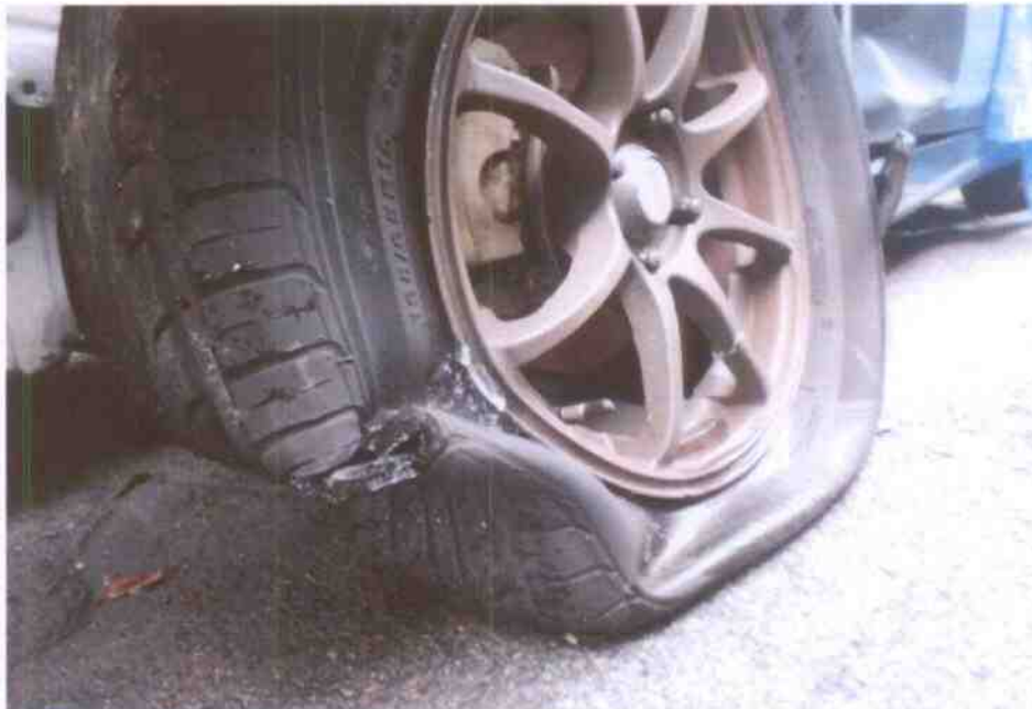
Photo 8 shows the condition of the front left tyre of the Motor Car, which was observed to be in serviceable condition with remaining tread depth of approximately 4mm. The tyre, which was wrapped around alloy wheel rim, was observed to be cut and deflated as a result of the accident.
