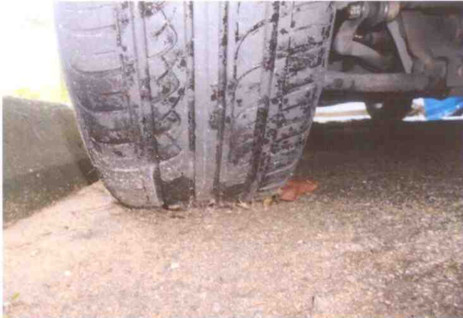
Photo 7 shows the condition of the front right tyre of the Motor Car, which was observed to be in serviceable condition with remaining tread depth of approximately 4mm. There was also no tear, cut or burst mark(s) on the outer and the inner sidewalls as well as across the tread of this tyre. The tyre, which was wrapped around a wheel rim, was also observed to be sufficiently inflated for vehicular operation.
