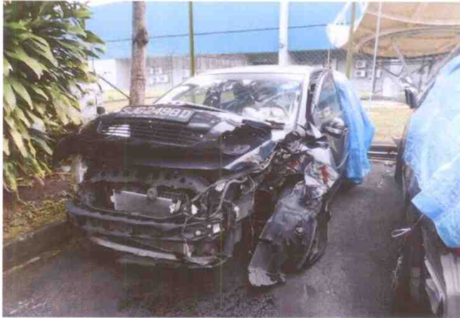
Photo 1 shows a general view of the front left body of the Motor Car at the time of my inspection. The Motor Car was observed to have sustained extensive impact damage at its left front body. The impact force was relatively significant causing severe damage to its front bumper, front left headlamp, front left fender, front left wheel house, front bonnet and front left door amongst others.
