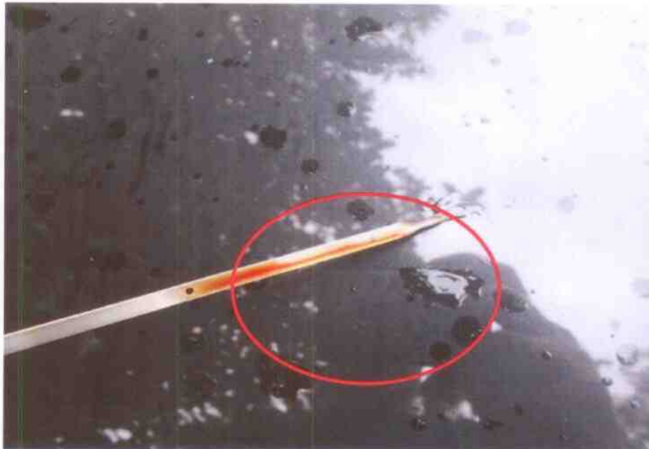
Photo 11 shows the engine oil dip stick of the Motor Car. I was able to pull the engine oil dip stick from the gaps around the front bonnet. The engine oil of the Motor Car was found to be sufficient level and without contamination for operating purposes.
