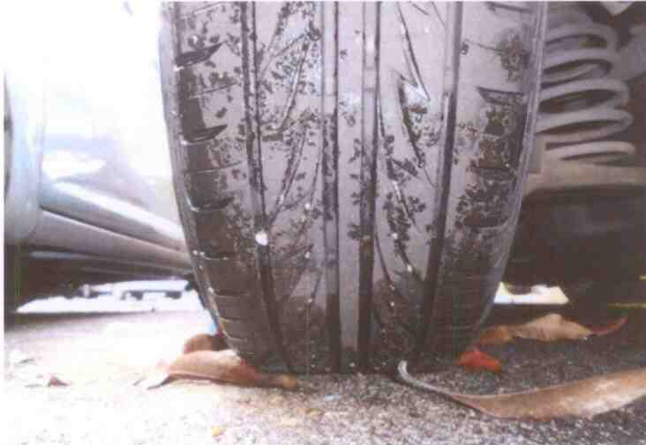
Photo 5 shows the condition of the rear left tyre of the Motor Car, which was observed to be in serviceable condition with remaining tread depth of approximately 4mm. There was no tear, cut or burst mark(s) on the outer and the inner sidewalls as well as across the tread of this tyre. The tyre, which was wrapped around alloy wheel rim, was also observed to be sufficiently inflated for vehicular operation.
