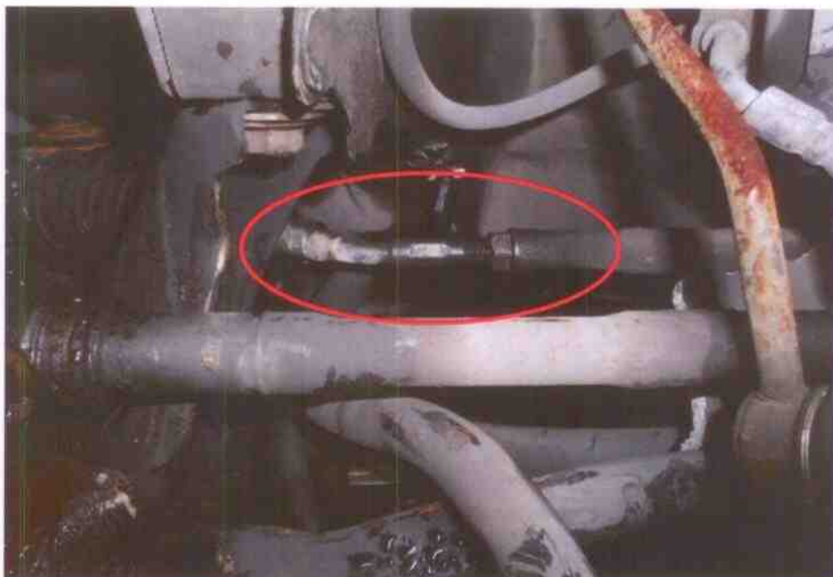
Photo 13 shows the bent steering tie rod (circled) at the front left wheel of the Motor Car. I was not able to conduct any tests on the steering system of the Motor Car due to the damage to the steering tie rod and other undercarriage components at the front left wheel of the Motor Car.
