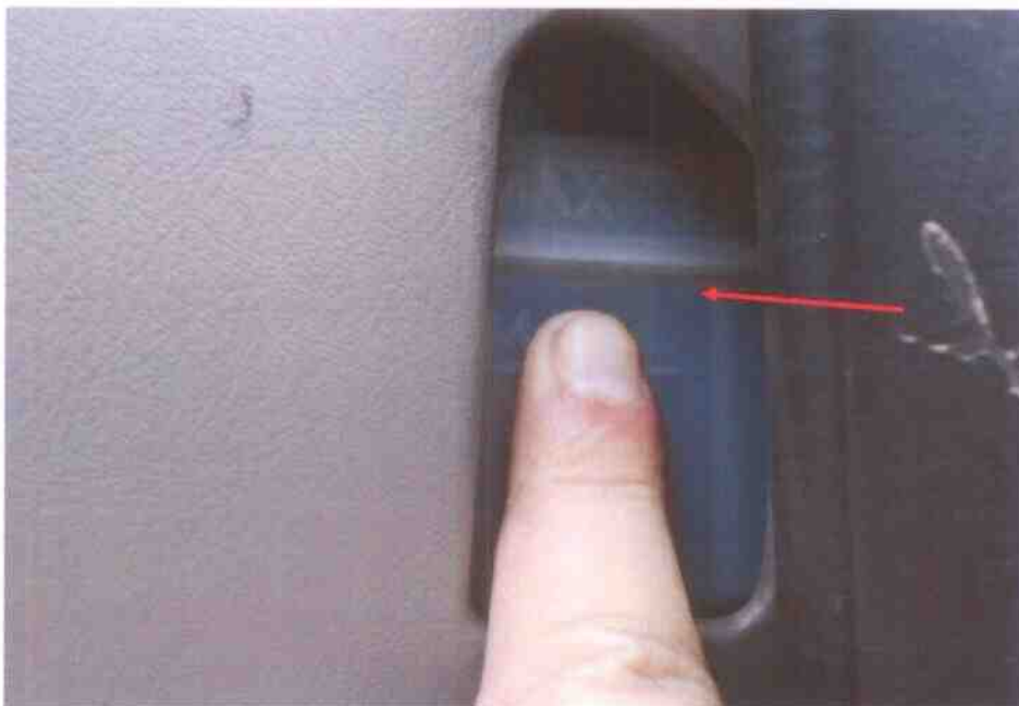
Photo 14 shows the brake fluid reservoir of the Motor Bus at the time of my inspection. The brake fluid was observed to be of sufficient level (arrowed) and without any visible contamination.
