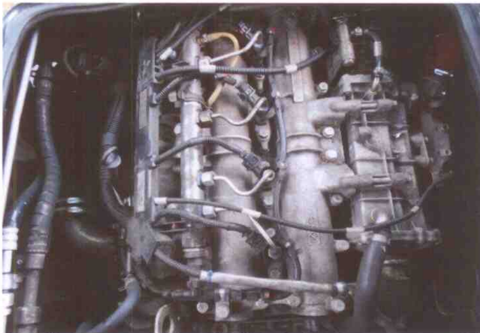
Photo 12 shows a general view of the Motor Bus's engine compartment, which was accessed from the interior of the Motor Bus by lifting the cover adjacent to the left side of the driver's seat. The various parts and components inside the engine compartment were unaffected by the accident. There was also no sign(s) or indication(s) of fluid leakage and/or fluid stain within the engine compartment.
