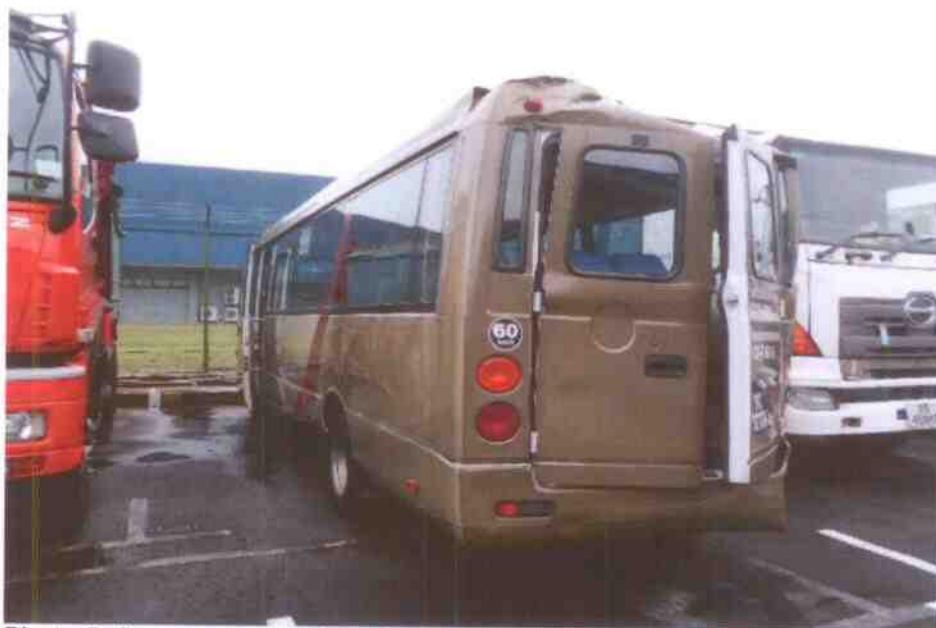
Photo 5 shows a general view of the Motor Bus's rear left body at the time of my inspection. The rear doors, rear bumper and rear right panel were amongst the body parts at the rear right of the Motor Bus that had sustained damages. Its roof panel was also observed to have been buckled as a result of the accident. The left side of the Motor Bus was relatively unaffected by the collision.
