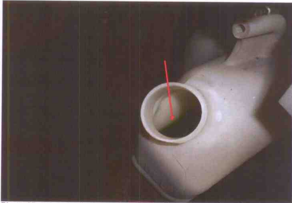
Photo 15 shows checks being carried out to the engine coolant of the Motor Bus at the time of my inspection. The engine coolant was observed to be of sufficient level (arrowed) and without any visible contamination.
