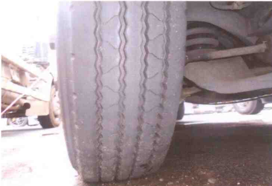
Photo 7 shows the condition of the front right tyre of the Motor Bus, which was observed to be in serviceable condition with remaining tread depth of approximately 6mm. The tyre, which was wrapped around standard alloy wheel rim, was also observed to be sufficiently inflated for vehicular operation.
