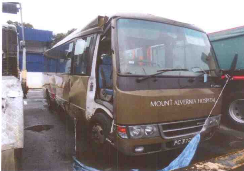
Photo 2 shows a general view of the front right body of the Motor Bus at the time of my inspection. The right front body of the Motor Bus was observed to have been damaged. Its roof panel was also observed to be affected while its driver's door was observed to have been removed for rescue purposes.
