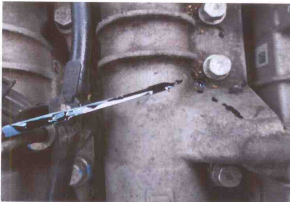
Photo 16 shows the engine dip stick of the Motor Bus at the time of my inspection. The engine oil was observed to be of sufficient level and without any visible contamination.
