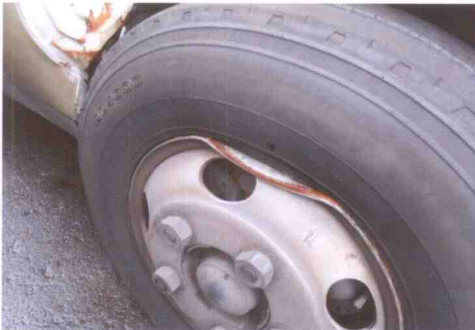
Photo 8 shows the front right tyre of the Motor Bus wrapped around standard alloy wheel rim. The front left wheel rim was observed to be dented due to the accident.
