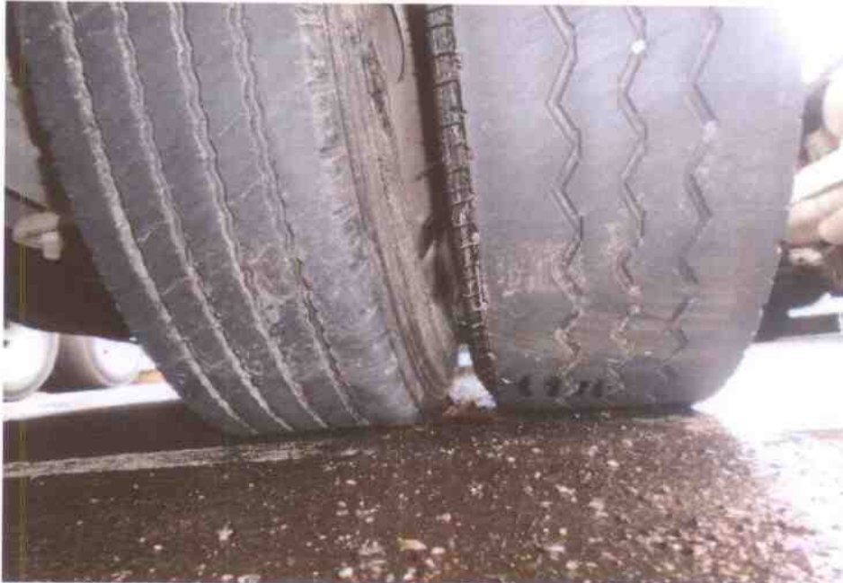
Photo 10 shows the condition of the rear right tyres of the Motor Bus, which were observed to be in serviceable condition with remaining tread depth of approximately 4mm. There was also no tear, cut or burst mark(s) on the outer and the inner sidewalls as well as across the tread of the 6 tyres that were fitted on the Motor Bus.
