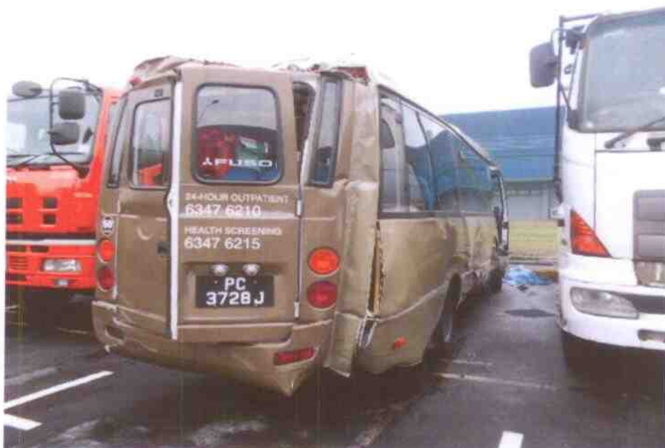
Photo 4 shows a general view of the Motor Bus's rear right body at the time of my inspection. The rear doors, rear bumper and rear right panel were amongst the body parts at the rear right of the Motor Bus that had sustained damages. Its roof panel was also observed to have been buckled as a result of the accident.
