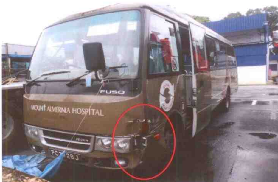
Photo 1 shows a general view of the front left body of the Motor Bus at the time of my inspection. The Motor Bus was observed to have sustained damage at its front left body. Its front bumper, front left signal lamp and front panel were amongst the body parts at the front left of the Motor Bus that had sustained damages as a result of the accident.
