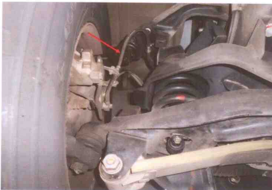
Photo 20 shows the undercarriage components at the front right wheel of the Motor Bus, in particular the brake hose (arrowed). The Motor Bus's braking system was likely to be in serviceable condition at the material time of accident as my visual examination of the various mechanical parts in the braking system did not produce any observations that had suggested otherwise. This was also taking into consideration that the brake fluid was of sufficient level and without any visible contamination.
