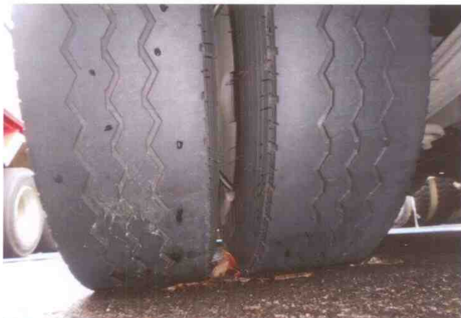
Photo 9 shows the condition of the rear left tyres of the Motor Bus, which was observed to be in serviceable condition with remaining tread depth of approximately 3mm. The tyres, which were wrapped around standard alloy wheel rim, were also observed to be sufficiently inflated for vehicular operation. There was also no damage found on all 6 standard alloy wheel rims of the Motor Bus except for the front right wheel rim and rear right outer wheel rim, which were both dented due to the accident.
