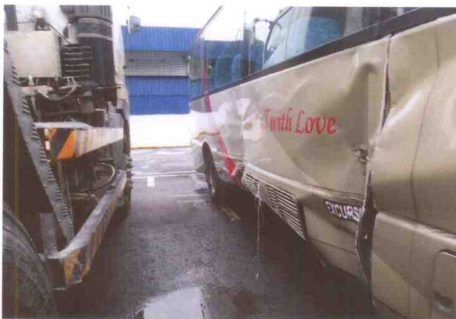
Photo 3 shows the right centre body of the Motor Bus. The body panels along the right side of the Motor Bus were observed to be have been dented/buckled.
