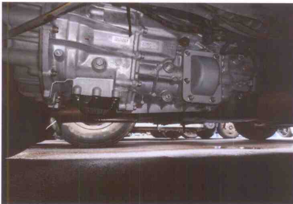
Photo 13 shows a general view of the Motor Bus's transmission housing, as viewed from the bottom of the Motor Bus. The engine and transmission, along with all its related parts, were found to be intact and unaffected by the accident. There was also no sign(s) or indication(s) of fluid leak/stain observed on the underside of the Motor Bus.
