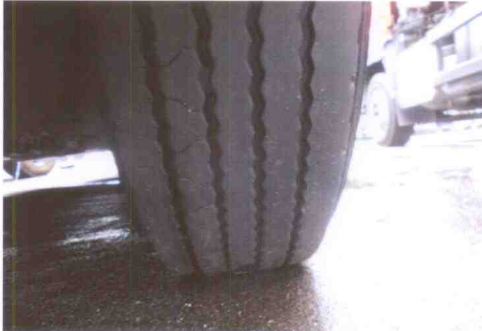
Photo 6 shows the condition of the front left tyre of the Motor Bus, which was observed to be in serviceable condition with remaining tread depth of approximately 5mm. The tyre, which was wrapped around standard alloy wheel rim, was also observed to be sufficiently inflated for vehicular operation. There was no tear, cut or burst mark(s) on the outer and the inner sidewalls as well as across the tread of the 6 tyres that were fitted on the Motor Bus.
