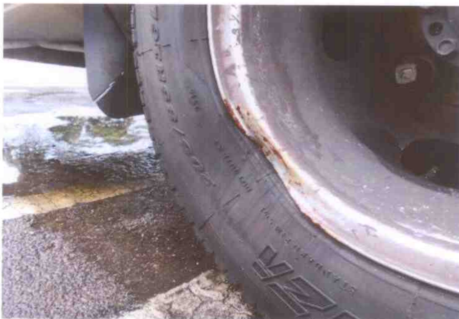
Photo 11 shows the rear right outer wheel rim of the Motor Bus which was observed to be dented due to the accident.
