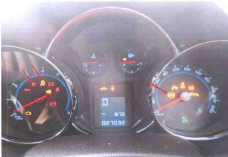
Photo 18 shows the warning lights for the various electronic operating systems of the Motor Car appearing on its instrument panel during the self-test when the engine is cranked, in particular the ABS light, TCS light and SRS light (arrowed).
