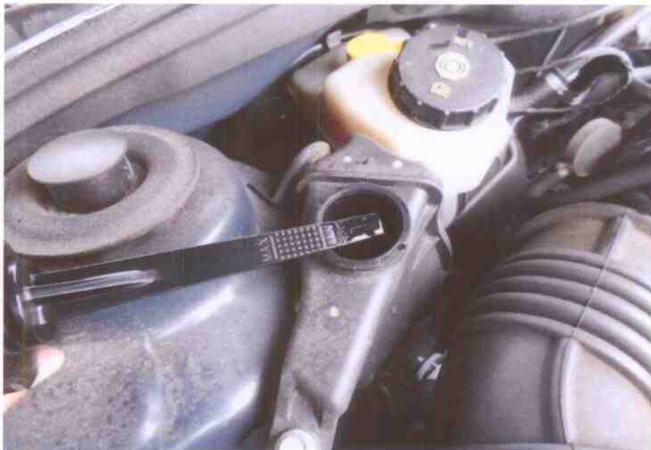
Photo 10 shows the power steering fluid reservoir of the Motor Car at the time of my inspection. The power steering fluid was observed to be of sufficient level and without any visible contamination.
