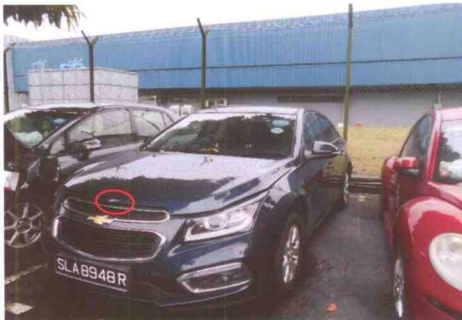
Photo 2 shows a general view of the front left body of the Motor Car at the time of my inspection. The Motor Car's exterior body was observed to be in good general condition. However I had observed a slight dent (circled) at the leading edge of its front bonnet.
