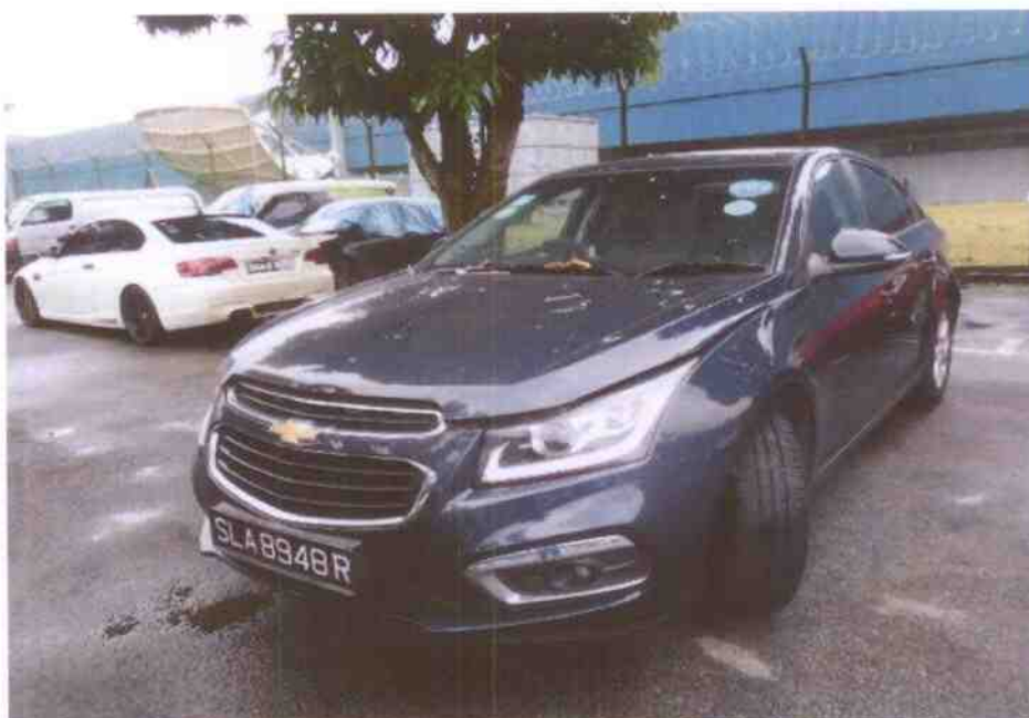
Photo 15 shows the front left wheel of the Motor Car turned to its full left. During my steering system test, I did not experience any abnormal free play and/or resistance when I had turned the steering wheel towards the left and right. This would suggest that the steering system of the Motor Car was likely to be in serviceable condition at the material time of accident.
