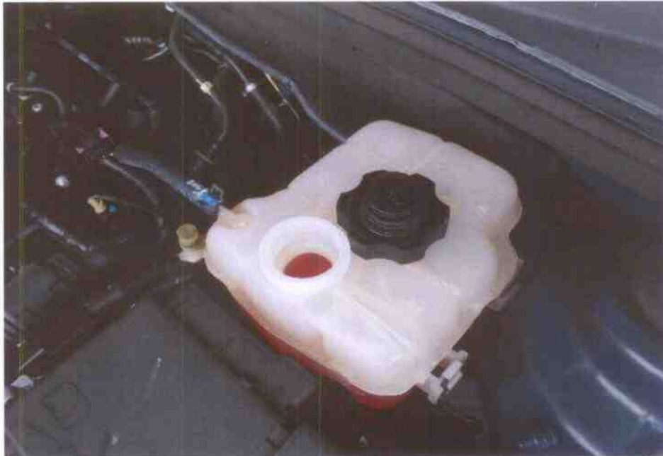
Photo 11 shows checks being carried out to the engine coolant of the Motor Car at the time of my inspection. The engine coolant was observed to be of sufficient level and without any visible contamination.
