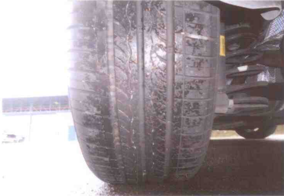
Photo 6 shows the condition of the rear left tyre of the Motor Car, which was observed to be in serviceable condition with remaining tread depth of approximately 4mm. The tyre, which was wrapped around alloy wheel rim, was also observed to be sufficiently inflated for vehicular operation. There was also no damage found on the 4 wheel rims of the Motor Car.
