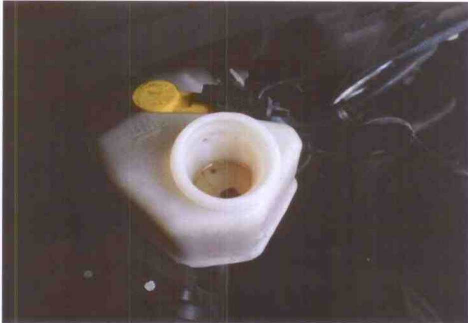
Photo 9 shows the brake fluid reservoir of the Motor Car at the time of my inspection. The brake fluid was observed to be of sufficient level and without any visible contamination.
