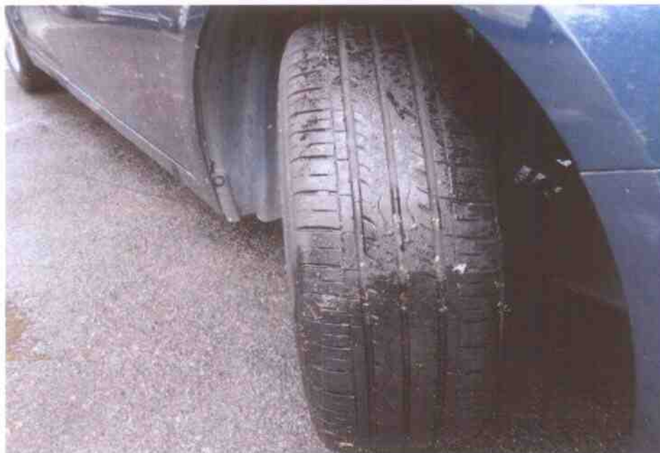
Photo 5 shows the condition of the front right tyre of the Motor Car, which was observed to be in serviceable condition with remaining tread depth of approximately 4mm. The tyre, which was wrapped around alloy wheel rim, was also observed to be sufficiently inflated for vehicular operation.
