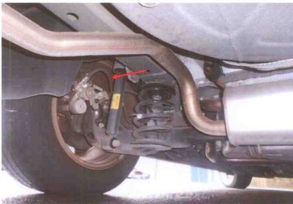
Photo 13 shows the brake hose/pipe (arrowed) at the rear left wheel of the Motor Car. I did not observe any leakage of brake fluid at the time of my inspection of the Motor Car. Static tests of the Motor Car's braking system had indicated that there was no internal leakage of pressure/vacuum. Hence the braking system was likely to be in serviceable condition at the material time of accident. The undercarriage components of the Motor Car were also all found to be intact and without any visible damage.
