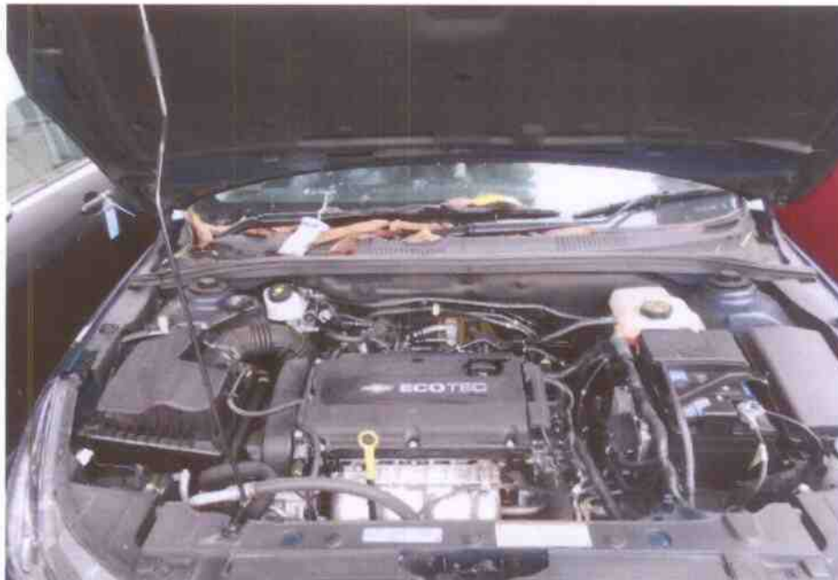
Photo 8 shows a general view of the Motor Car's engine compartment. The various parts and components inside the engine compartment were unaffected by the accident. There was also no sign(s) or indication(s) of fluid leakage and/or fluid stain within the engine compartment.
