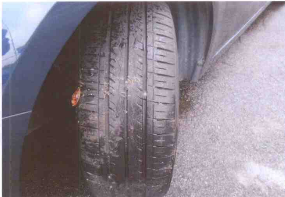
Photo 4 shows the condition of the front left tyre of the Motor Car, which was observed to be in serviceable condition with remaining tread depth of approximately 4mm. The tyre, which was wrapped around alloy wheel rim, was also observed to be sufficiently inflated for vehicular operation. There was no tear, cut or burst mark(s) on the outer and the inner sidewalls as well as across the tread of the 4 tyres.
