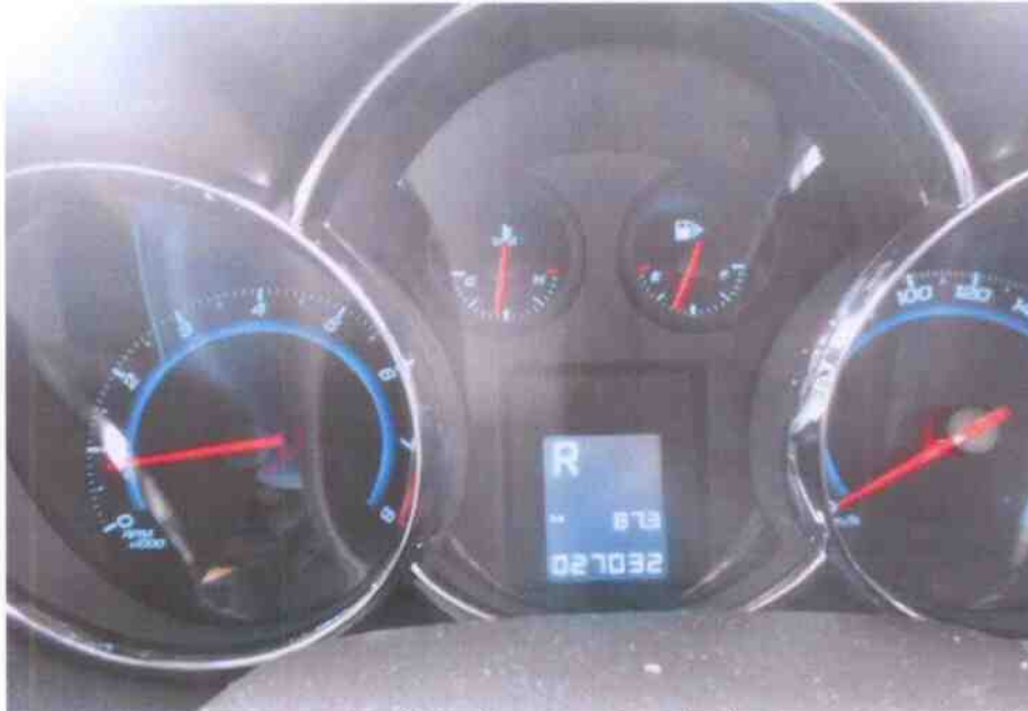
Photo 19 shows no warning lights illuminated on the instrument panel of the Motor Car after the engine was cranked. This would suggest that there was no abnormality to the various electronic operating systems of the Motor Car, like the ABS, TCS and SRS etc.
