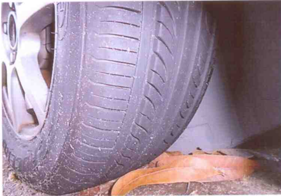
Photo 14 shows the condition of the front right tyre of the Motor Car, which was observed to be in serviceable condition. The 4 tyres were also observed to be sufficiently inflated for vehicular operation.
