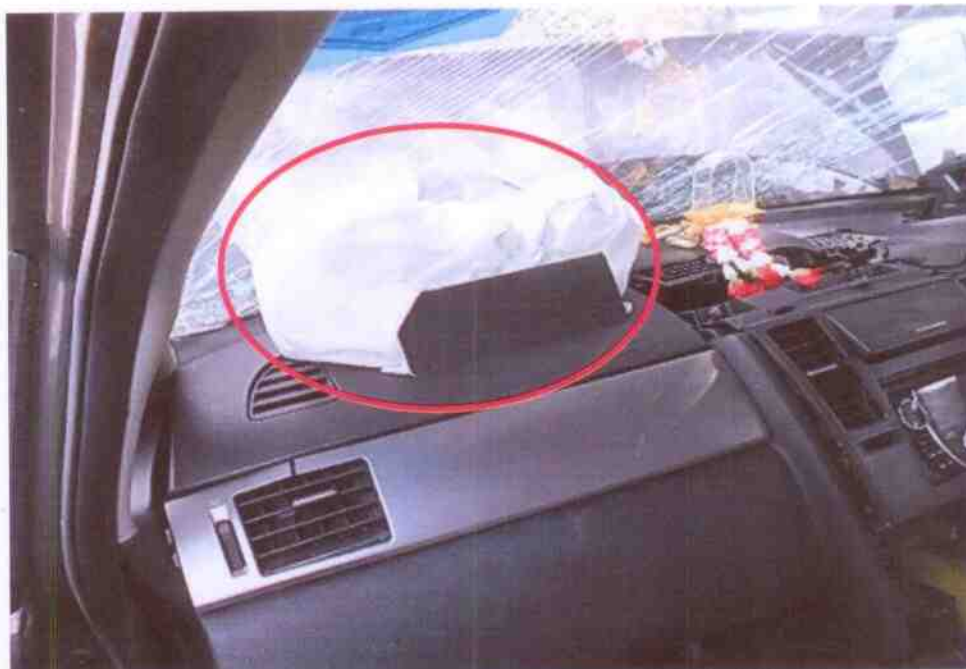
Photo 27 shows the Supplemental Restraint System (SRS) of the Motor Car was however likely to be in normal operating condition at the material time of the accident. The evidence of the deployed front passenger's airbag indicates that the impact sensors and control module of the Motor Car's SRS were all in serviceable condition at the material time of accident.
