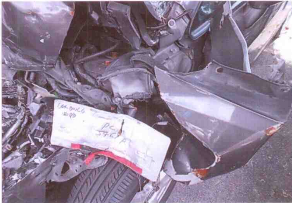
Photo 6 shows a closer view of the damage at the frontal left portion of the Motor Car. The impact force was significant, causing the various parts and components inside the engine compartment to be pushed inwards, towards the rear of the Motor Car.
