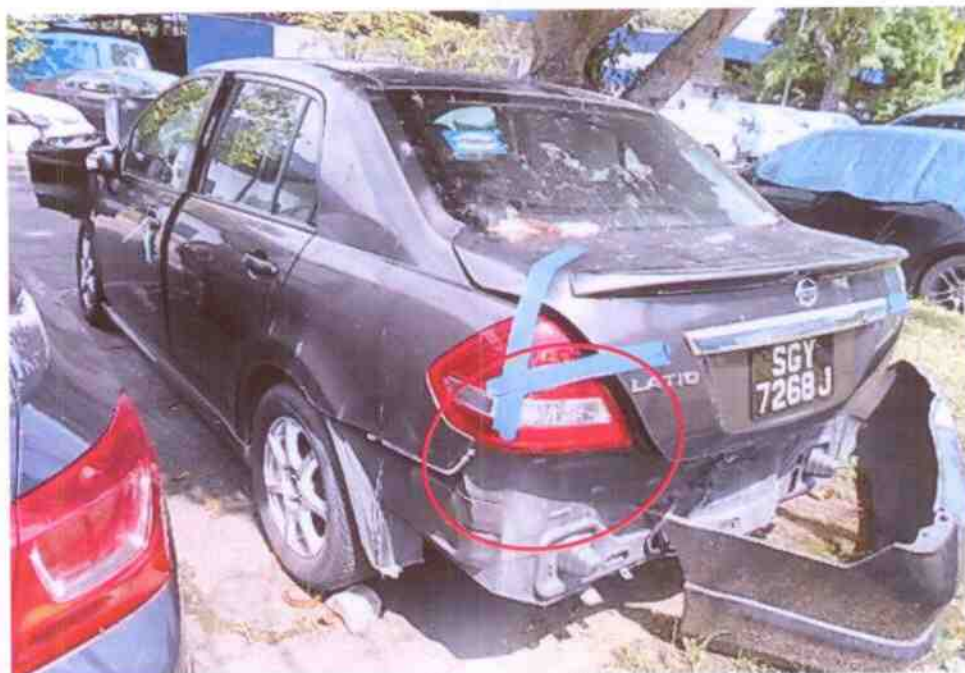
Photo 12 shows a general view of the rear left portion of the Motor Car at the time of our inspection. The rear portion was observed to be relatively sustained with minor impact by the accident that caused the rear bumper to be dislodged.
