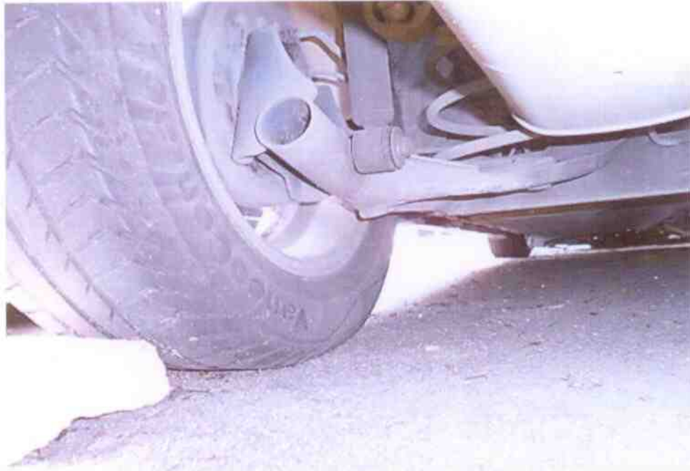
Photo 24 shows the braking & steering components at the left front wheel of the Motor Car. We did not observe any leakage of brake fluid at the time of our inspection of the Motor Car.
