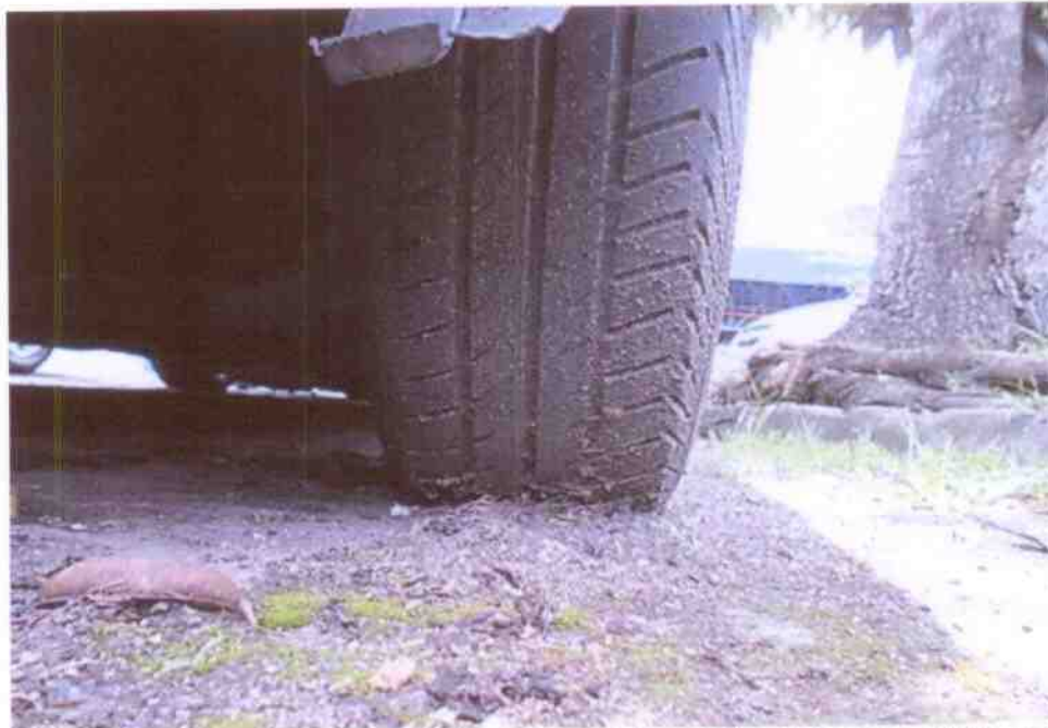
Photo 17 shows the condition of the rear right tyre of the Motor Car, which was observed to be in serviceable condition. The 4 tyres were also observed to be sufficiently inflated for vehicular operation.
