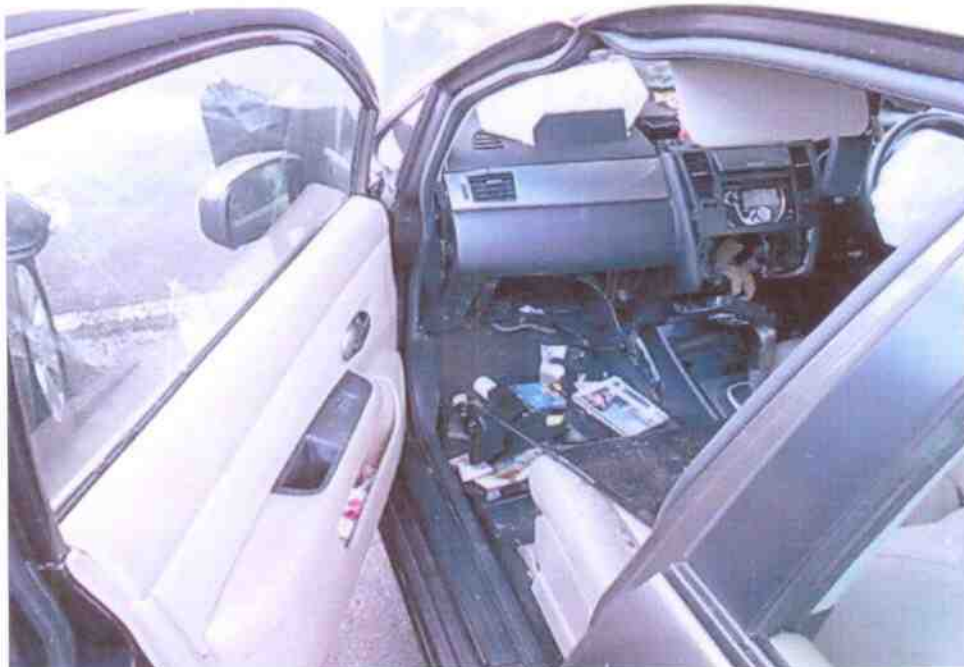
Photo 11 shows a closer view of the damage at the interior portion of the Motor Car. The driver & front passenger's airbag was noted to be activated due to the extensive impact collision at time of the accident.
