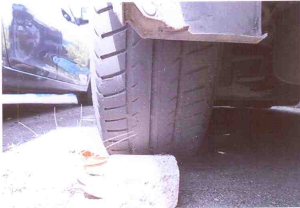
Photo 16 shows the condition of the rear left tyre of the Motor Car, which was observed to be in serviceable condition. The 4 tyres were also observed to be sufficiently inflated for vehicular operation.
