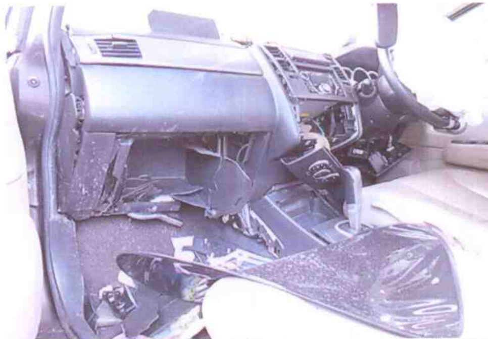
Photo 9 shows a closer view of the left front passenger seat of the Motor Car. The impact force was significant, causing the various parts and components inside the engine compartment to be pushed inwards, towards the rear of the Motor Car.
