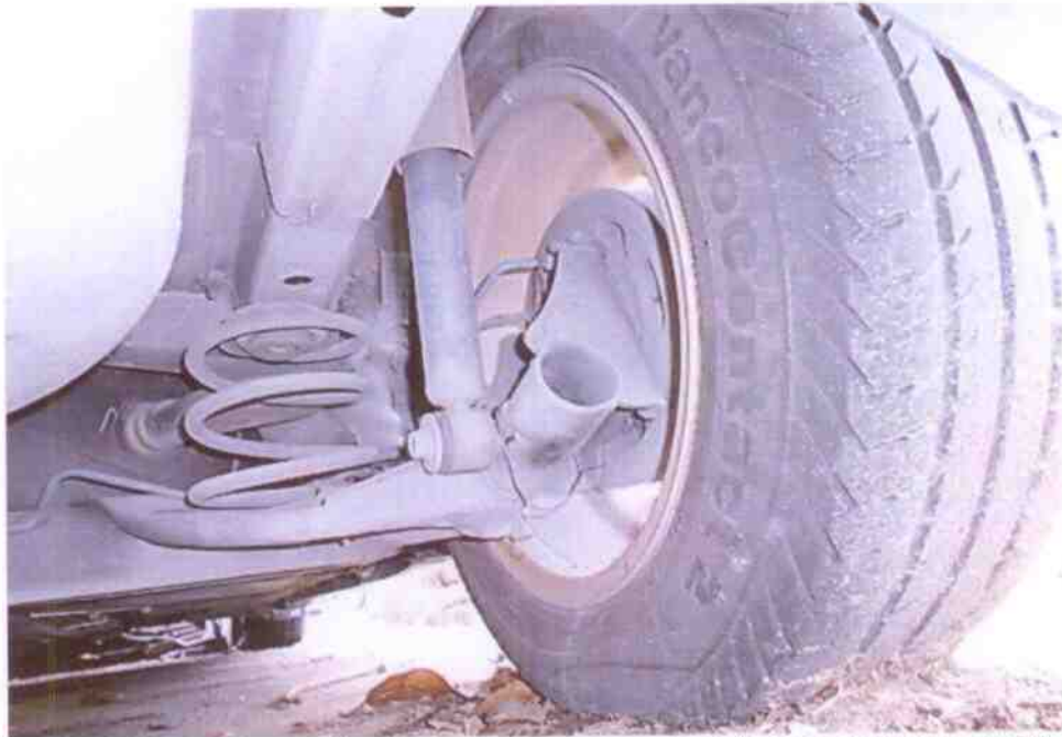
Photo 23 shows the braking & steering components at the rear right wheel of the Motor Car. We did not observe any leakage of brake fluid at the time of our inspection of the Motor Car.
