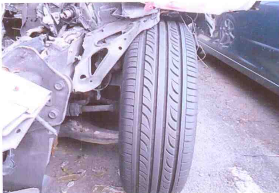
Photo 15 shows the condition of the front left tyre of the Motor Car, which was observed to be in serviceable condition. The 4 tyres were also observed to be sufficiently inflated for vehicular operation.
