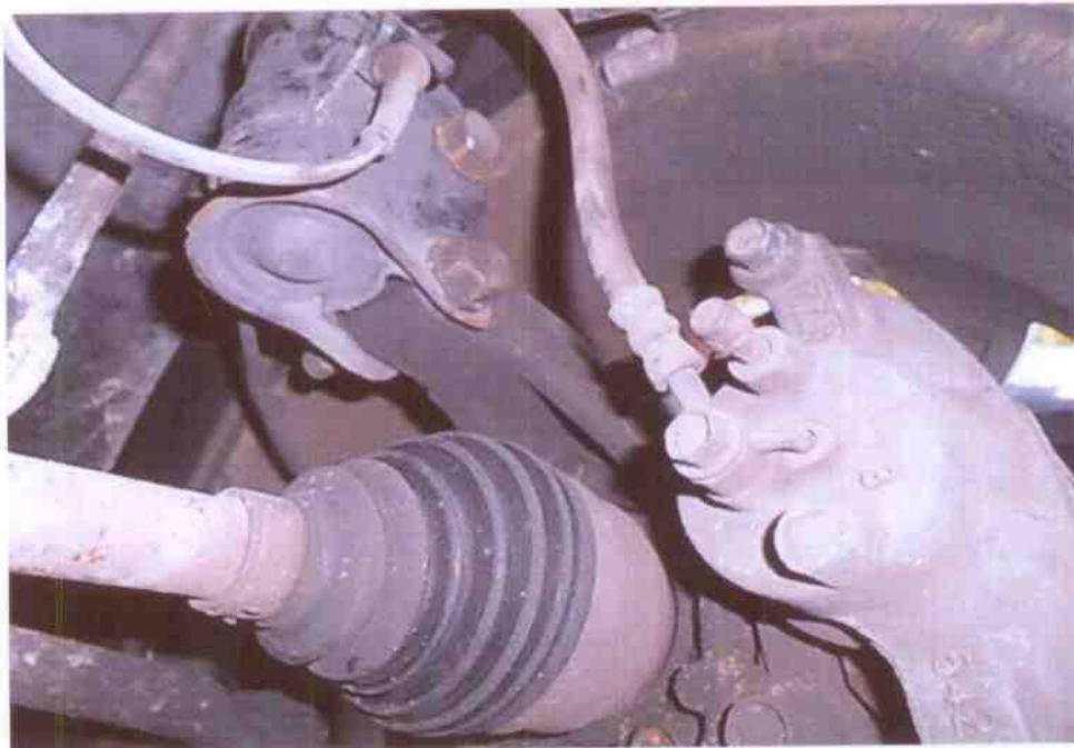
Photo 21 shows a close up view on the front right drive shaft of the Motor Car. We were not able to conduct any tests on the steering system of the Motor Car due to the damage to this components, as well as leakage of power steering fluid.
