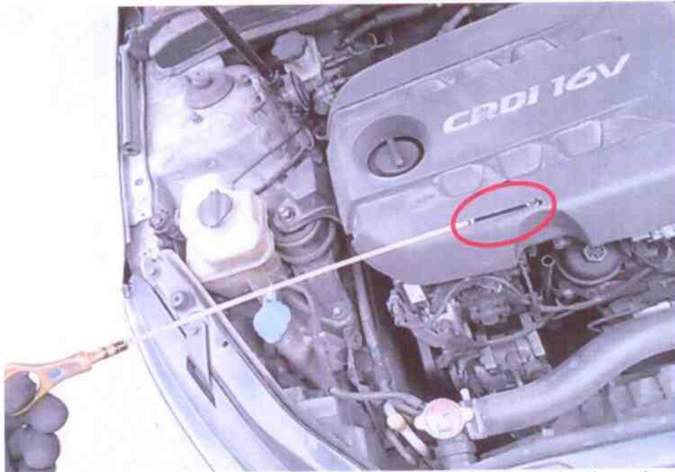
Photo 14 shows the engine oil dip stick of the Motor Taxi at the time of our inspection. The engine oil was observed to be of sufficient level and without any visible contamination.
