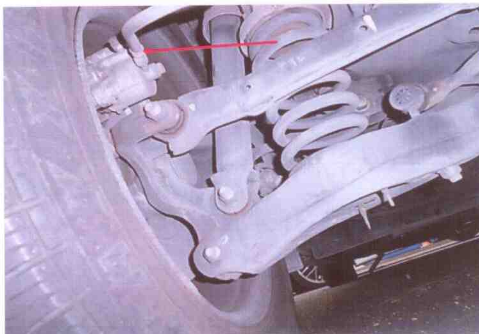
Photo 17 shows the brake hose (arrowed) at the rear right wheel of the Motor Taxi. We did not observe any leakage of brake fluid at the time of our inspection of the Motor Taxi. Our visual inspection of the various mechanical components of the Motor Taxi's braking system, including its brake calliper, revealed all to be intact and without visible damage, indicating that the braking system was likely to be in serviceable condition at the material time of accident.
