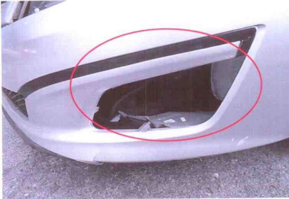
Photo 5 shows a close up view of the lower bumper of the Motor Taxi at the time of our inspection. The Motor Taxi had sustained relatively minor cracked at the lower bumper of the Motor Taxi.
