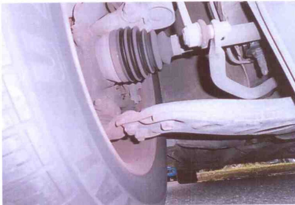
Photo 19 shows the various undercarriage components at the rear right wheel of the Motor Taxi. We did not observe any leakage of brake fluid at the time of our inspection of the Motor Taxi. Our visual inspection of the various mechanical components of the Motor Taxi's braking system revealed all to be intact and without visible damage, indicating that the braking system was likely to be in serviceable condition at the material time of accident.
