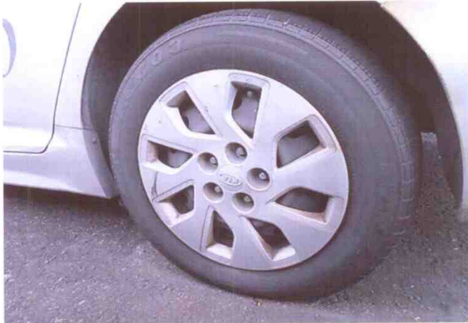
Photo 6 shows the 4 tyres were observed to be wrapped around standard wheel rims with wheel caps fitted on its outer side. Multiple grazed marks that are commonly associated to grazing against a road kerb were found on all the wheel caps of the Motor Taxi.
