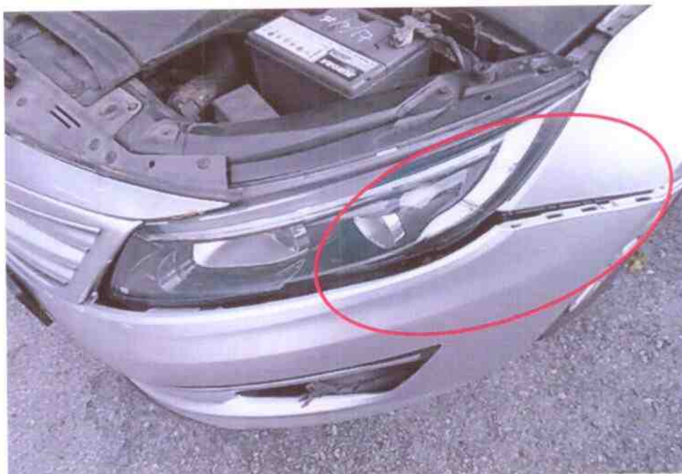
Photo 4 shows a close up view of the front bonnet of the Motor Taxi at the time of our inspection. The Motor Taxi had sustained relatively minor misalignment at the front bonnet of the Motor Taxi.
