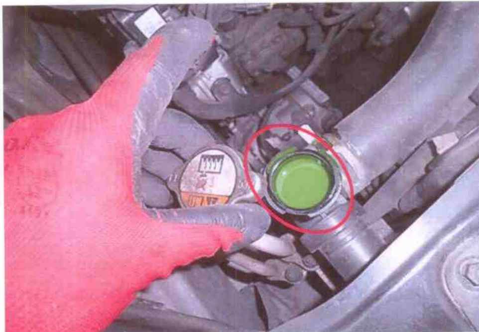
Photo 15 shows the coolant fluid at radiator tank of the Motor Taxi at the time of our inspection. The coolant fluid was observed to be of sufficient level and without any visible contamination.
