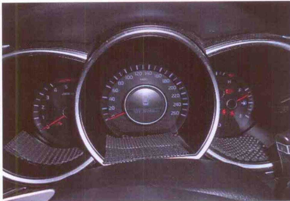
Photo 20 shows the warning lights for the various electronic operating systems of the Motor Taxi appearing on its instrument panel during the ignition start, in particular the ABS light and SRS light. Despite the engine was unable to be started at time of inspection.
