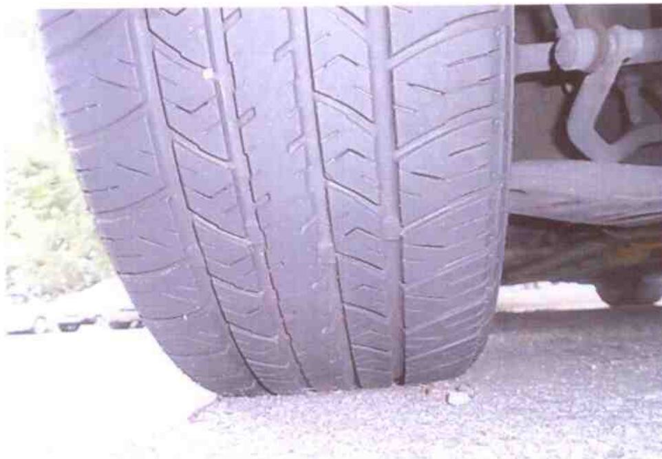
Photo 9 shows the condition of the front right tyre of the Motor Taxi, which was observed to be in serviceable condition with remaining tread depth of approximately 5mm.
