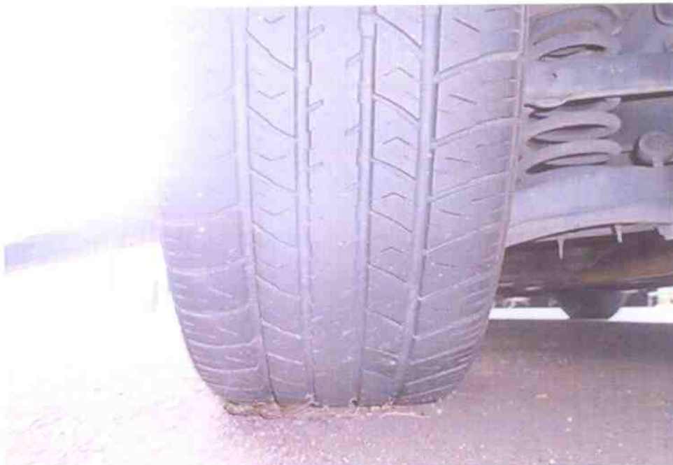
Photo 8 shows the condition of the rear left tyre of the Motor Taxi, which was observed to be in serviceable condition with tread depth of approximately 4mm.
