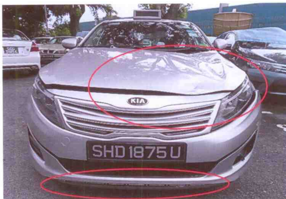
Photo 2 shows a general view of the front body of the Motor Taxi at the time of our inspection. The Motor Taxi was observed to have sustained minor damages at the frontal portion.
