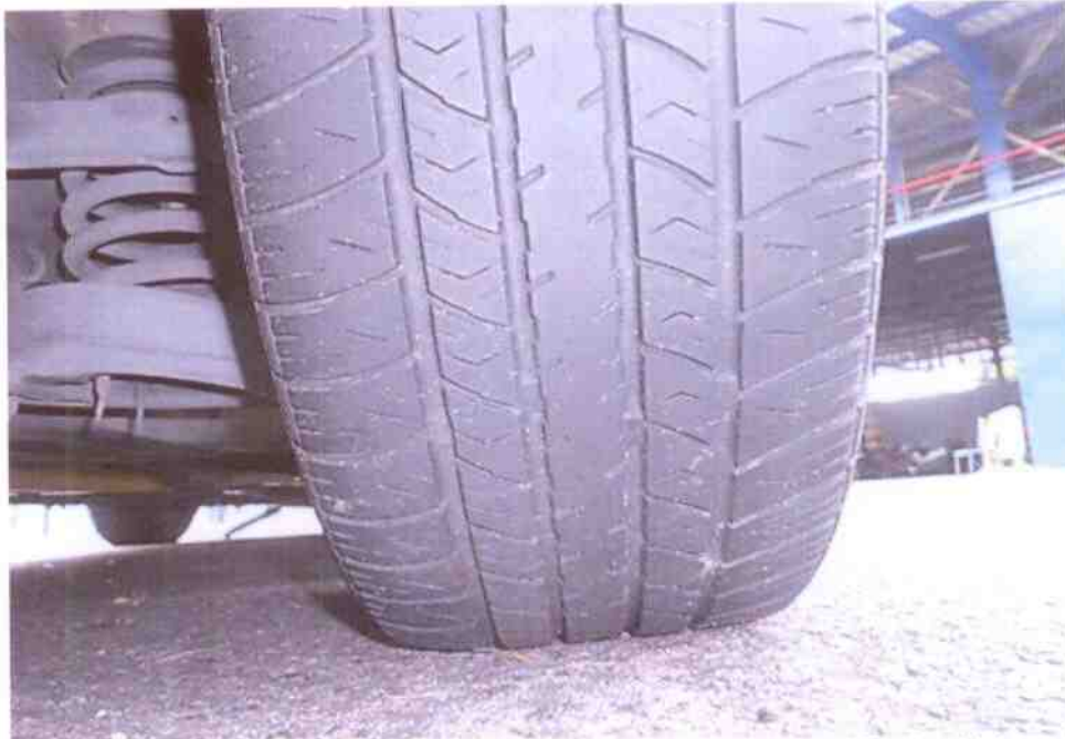
Photo 7 shows the condition of the rear right tyre of the Motor Taxi, which was observed to be in serviceable condition with remaining tread depth of approximately 4mm.
