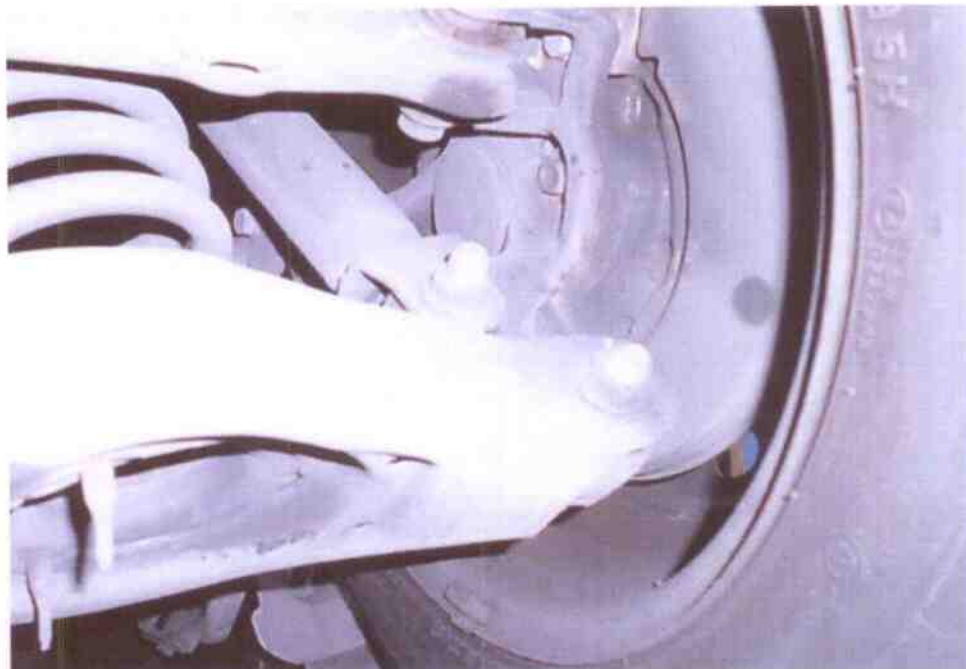
Photo 16 shows the rear left wheel of the Motor Taxi. We did not observe any leakage of brake fluid at the time of our inspection of the Motor Taxi.
