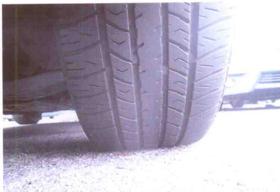
Photo 10 shows the condition of the front left tyre of the Motor Taxi, which was observed to be in serviceable condition with remaining tread depth of approximately 4mm.
