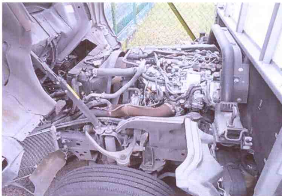
Photo 12 shows a general view of the Motor Lorry's engine compartment, which was accessed by lifting the front cabin of the Motor Lorry. The various parts and components inside the engine compartment were unaffected by the accident. There was also no sign(s) or indication(s) of fresh fluid leakage and/or fluid stain within the engine compartment (photograph shows the engine compartment as viewed from the left front side of the Motor Lorry).
