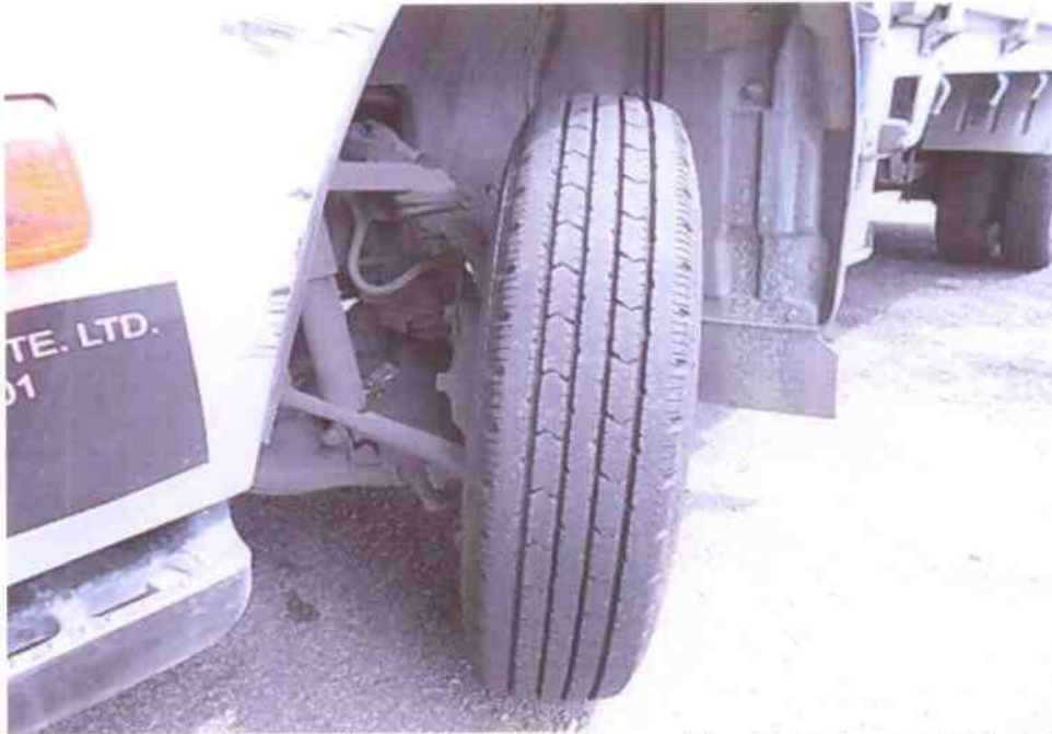
Photo 8 shows the condition of the front left tyre of the Motor Lorry, which was observed to be in serviceable condition with remaining tread depth of approximately 6mm. The tyre, which was wrapped around standard alloy wheel rim, was also observed to be sufficiently inflated for vehicular operation. There was no tear, cut or burst mark(s) on the outer and the inner sidewalls.
