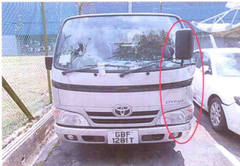
Photo 1 shows a general view of the front left body of the Motor Lorry at the time of our inspection. The Motor Lorry was observed to have sustained damages at its front left panel, front left wiper panel, front left bumper, front left side mirror, headlamp and left passenger door were amongst the body parts that were damaged as a result of the accident. (circled).
