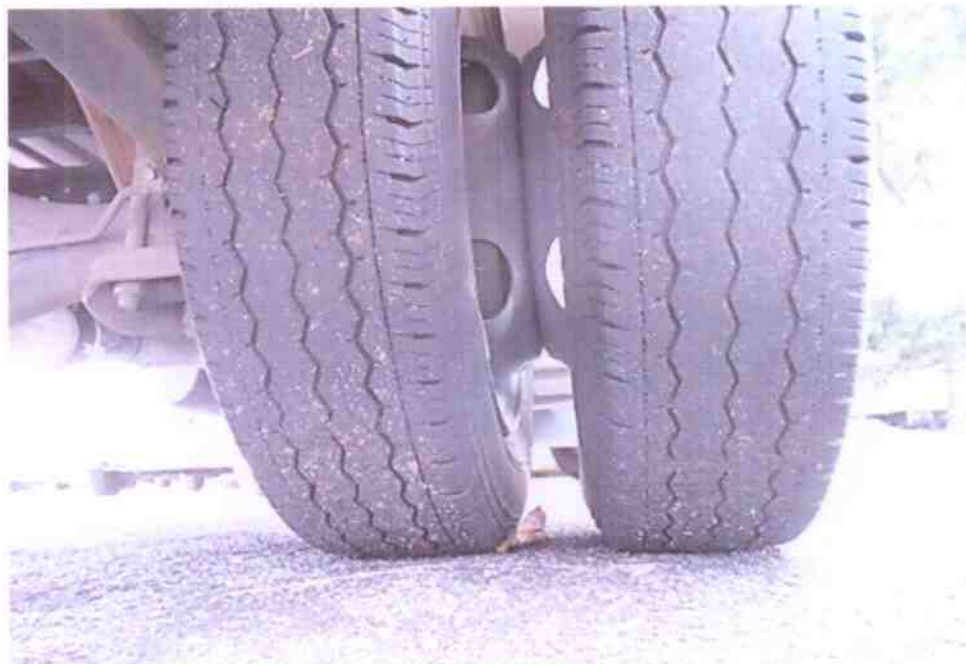
Photo 11 shows the condition of the rear right tyres of the Motor Lorry, which were observed to be in serviceable condition with remaining tread depth of approximately 2mm. There was also no tear, cut or burst mark(s) on the outer and the inner sidewalls.
