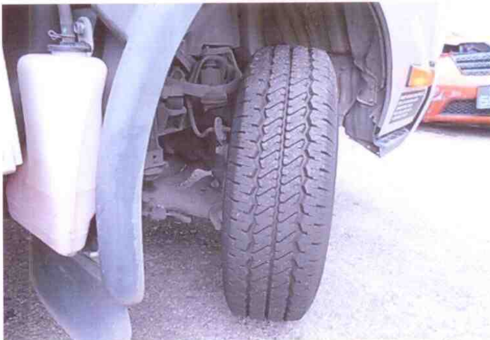
Photo 9 shows the condition of the front right tyre of the Motor Lorry, which was observed to be in serviceable condition with remaining tread depth of approximately 9mm. The tyre, which was wrapped around standard alloy wheel rim, was also observed to be sufficiently inflated for vehicular operation.
