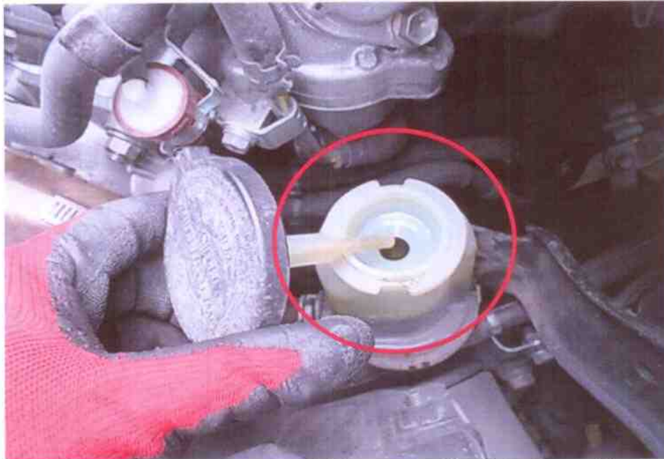
Photo 15 shows the power steering fluid reservoir of the Motor Lorry at the time of our inspection. The power steering fluid (circled) was observed to be of sufficient level and without any visible contamination.
