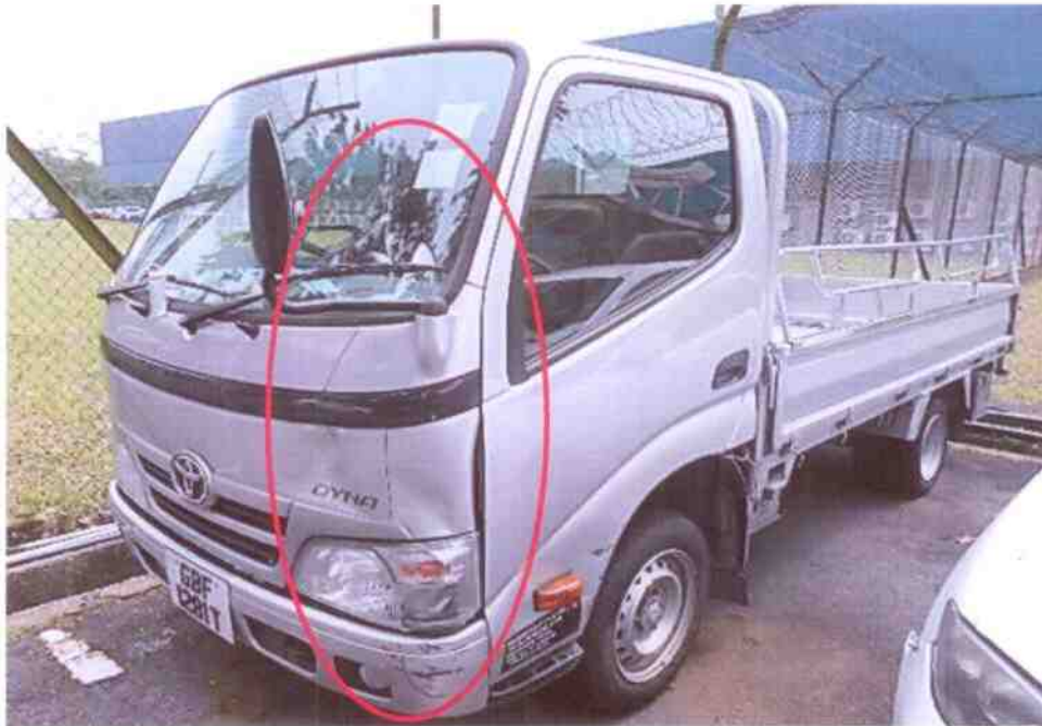
Photo 2 shows a general view of the front left body of the Motor Lorry at the time of my inspection. The Motor Lorry was observed to have sustained damages at its front left panel, front left wiper panel, front left bumper, front left side mirror, headlamp and left passenger door were amongst the body parts that were damaged as a result of the accident. (circled).
