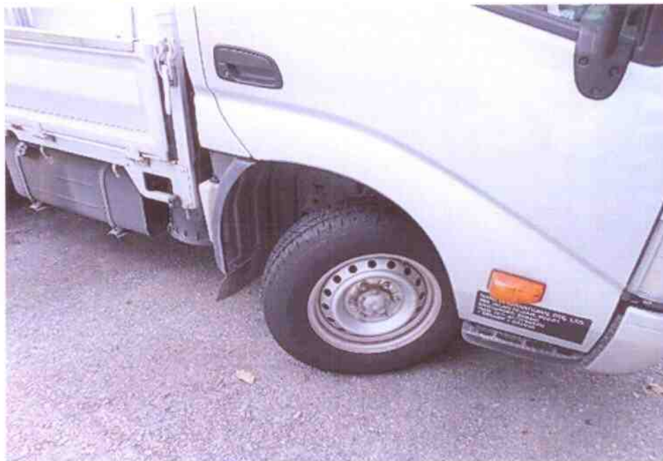
Photo 18 shows the front right wheel of the Motor Lorry turned to its full left. During our steering system test, we did not experience any abnormal free play and/or resistance when we had turned the steering wheel towards full left and full right. This would suggest that the steering system of the Motor Lorry was likely to be in serviceable condition at the material time of accident.
