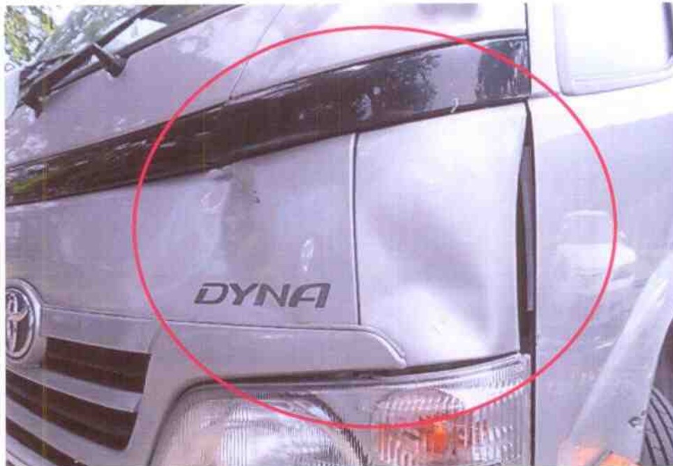
Photo 4 shows the damage sustained on the front left panels as a result of the accident.
