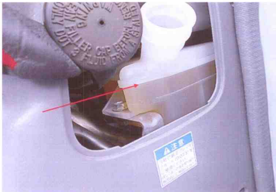
Photo 13 shows the brake fluid reservoir of the Motor Lorry at the time of our inspection. The brake fluid was observed to be of sufficient level and without any visible contamination.
