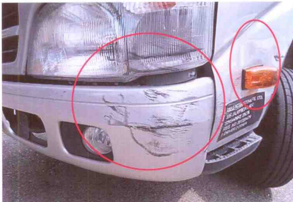
Photo 5 shows the damage sustained on the front left lower bumper & left passenger door as a result of the accident.
