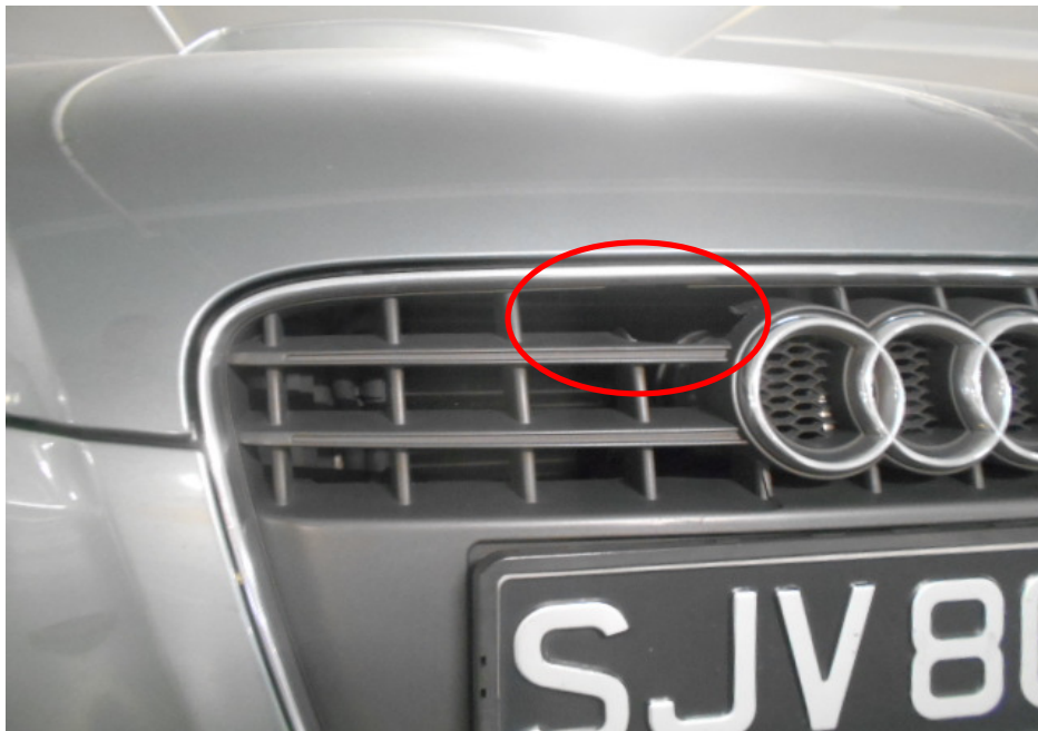
Photo 12 shows a general view of the crack (circled) to the front grille of the Insured Vehicle, at the top centre area of the front grille.
