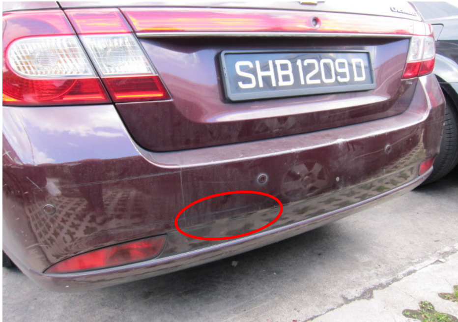
Photo 1 shows a general view of the rear portion of the Motor Taxi at the time of inspection on 07 July 2017. The Motor Taxi was observed to be generally in good condition. What appears to be an inverted L shape imprint mark was however observed towards the left of the Motor Taxi's rear bumper (circled).
