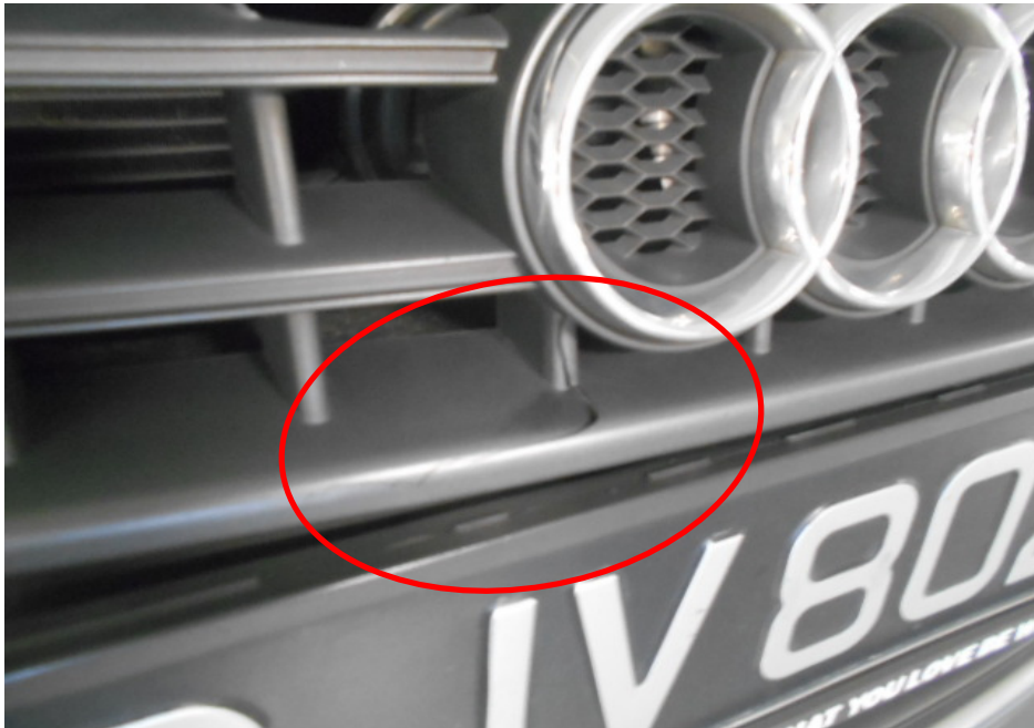
Photo 11 shows a close up view of the crack (circled) to the front grille of the Insured Vehicle, at the area directly above the front number plate.
