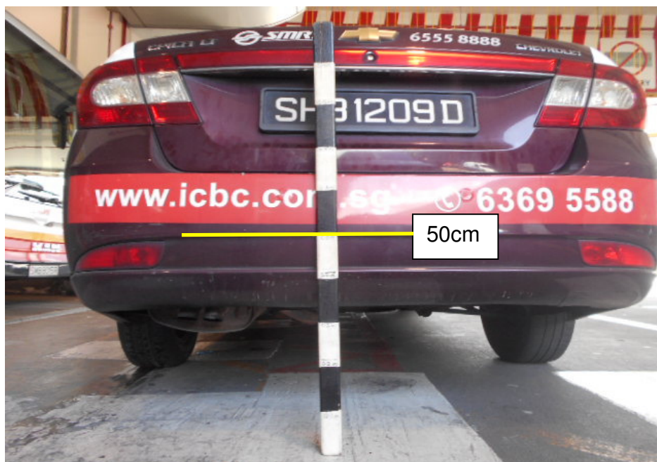
Photo 17 shows the height measurement that was conducted on the rear portion of the Motor Taxi. The height of the top horizontal end of the Insured Vehicle's front number plate frame was at similar height above ground level on the Motor Taxi where the inverted L shape imprint mark on its rear bumper was found (refer to photograph 2 and 3 above).
