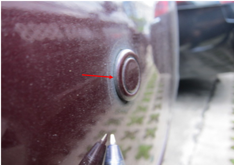
Photo 4 shows a close up view of the left reverse sensor of the Motor Taxi. The reverse sensor was observed to have been slightly pushed inwards, at the left side of the reverse sensor (arrowed).
