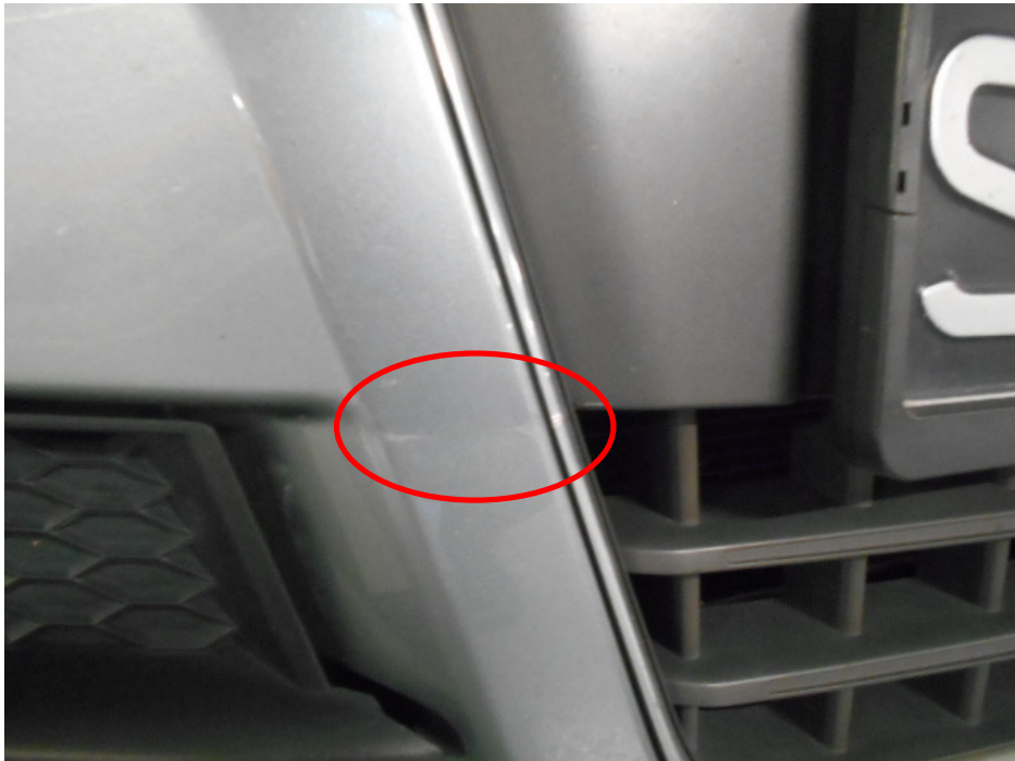
Photo 10 shows a close up view of the distortion (circled) to the front bumper of the Insured Vehicle, at the area slightly towards the right of the front number plate.
