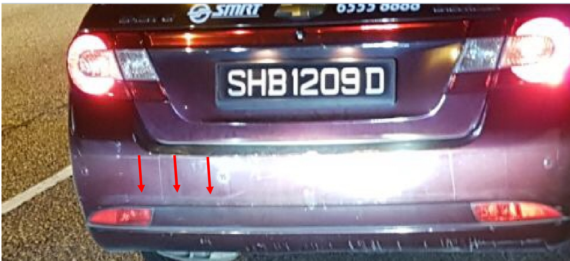
Photo 14 shows an enlarged view of the Motor Taxi's rear bumper, using photograph 13 above. I had observed what appears to be the same inverted L shape imprint mark on the rear bumper of the Motor Taxi, similar to what was observed from the photographs of the Motor Taxi that were taken at the time of inspection by LKK Auto Consultants Pte Ltd (refer to photograph 2 above for comparison).
