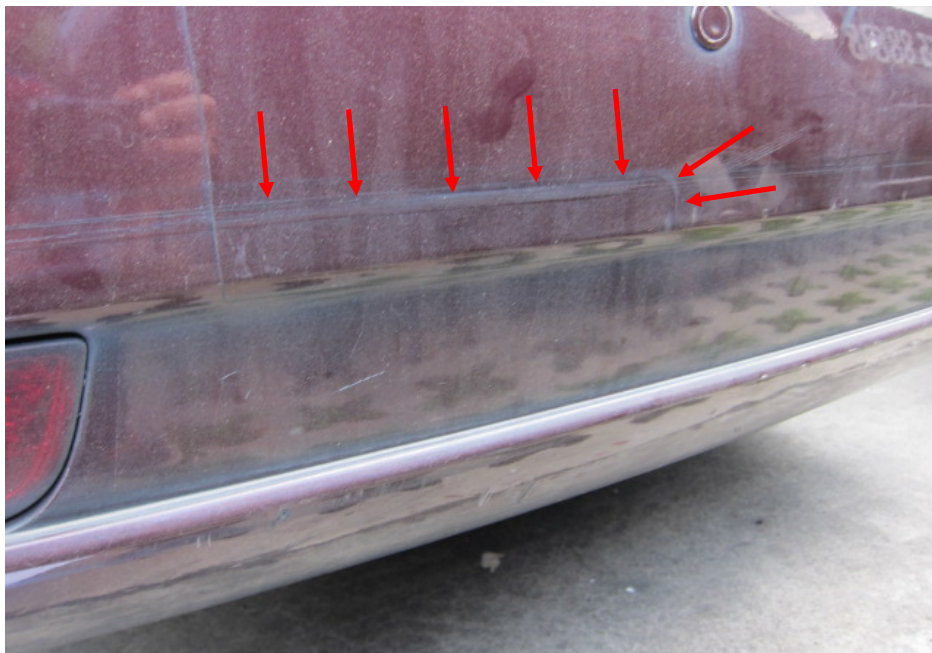
Photo 2 shows a closer view of the area where the inverted L shape imprint mark was found (arrowed). This was towards the left of the Motor Taxi's rear bumper. The imprint mark was a result of a load/force from a similarly shaped object (inverted L) pressing onto the rear bumper, inwards.
