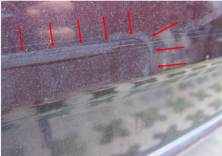
Photo 3 shows a close up view of the inverted L shape imprint mark which was caused by a load/force from a similarly shaped object (inverted L) pressing onto the rear bumper, inwards.
