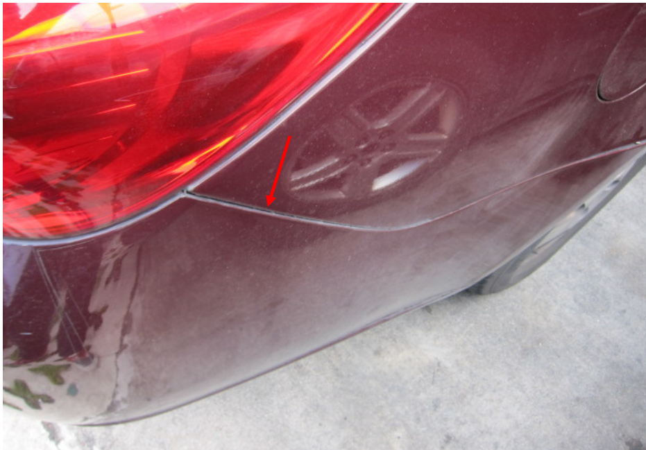
Photo 6 shows the right corner edges of the rear bumper, adjacent to the rear right fender of the Motor Taxi. There was no obvious misalignment at the right corner edges of the rear bumper (arrowed) as compared to the left corner edges. This would indicate that the impact onto the rear portion of the Motor Taxi was relatively light and was more towards the left of the rear bumper given that there was slight misalignment to the left corner edges.
