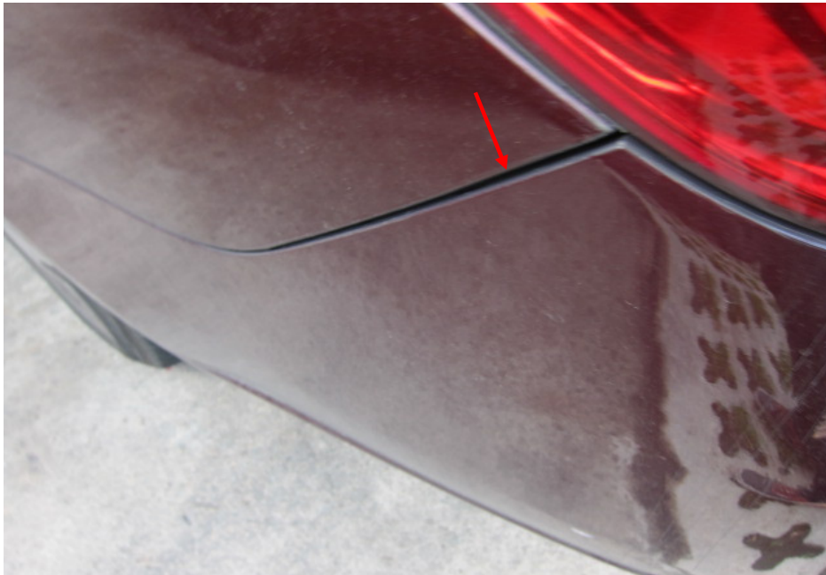
Photo 5 shows the slight misalignment (arrowed) at the left corner edges of the rear bumper, adjacent to the rear left fender of the Motor taxi. Such misalignment indicates that the Motor Taxi had sustained an impact directly onto its rear portion. This impact was however relatively light given that the misalignment was observed to be slight.
