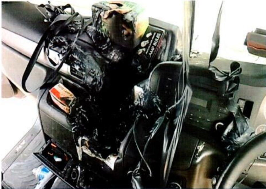
Photo 18 shows the interior compartment of the Insured Vehicle after the fire was extinguished. In general, the extensive damages sustained to the centre portion of the instrument panel had corresponded to the events that were related to us by Mr Chai, which is the fire started from the interior compartment.
