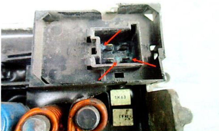
Photo 16 shows a close up view of the greenish residue found on the air- conditioning blower connector contact point (circled). The presence of such greenish residue suggests occurrence of an electrical short circuit.
