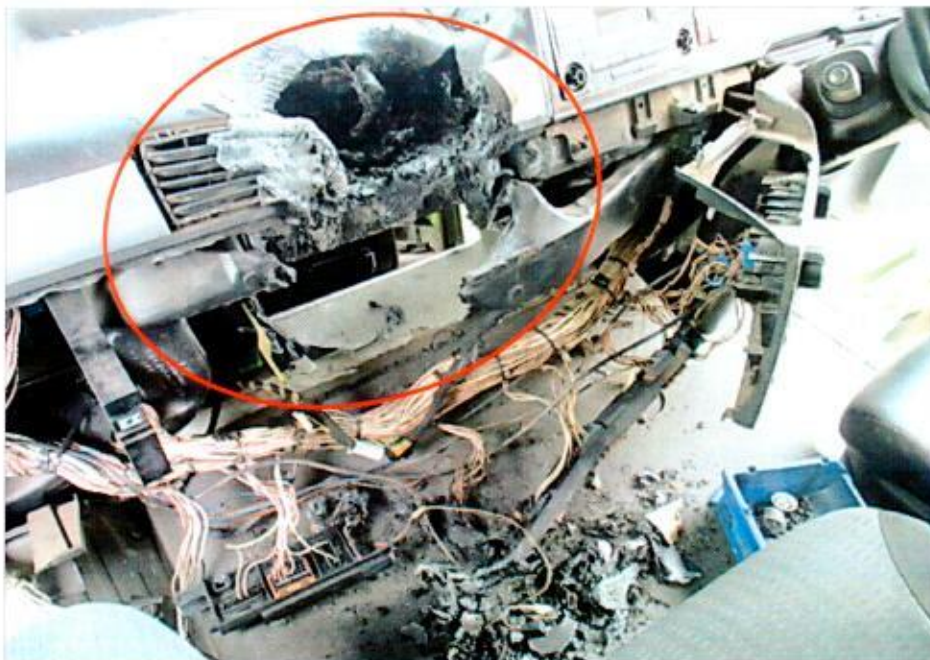
Photo 7 shows the centre of the dashboard of the Insured Vehicle. The fire seemed to have originated from the centre portion of the instrument panel basing on the area where the extent of fire damage was most severe. Various components of the instrument panel were observed to have been burnt and/or partly melted from prolonged exposure to high heat intensity which included the upper and central parts of the instrument panel assembly, air outlet assembly, beaker holder assembly and carrier assembly, amongst others (circled).
