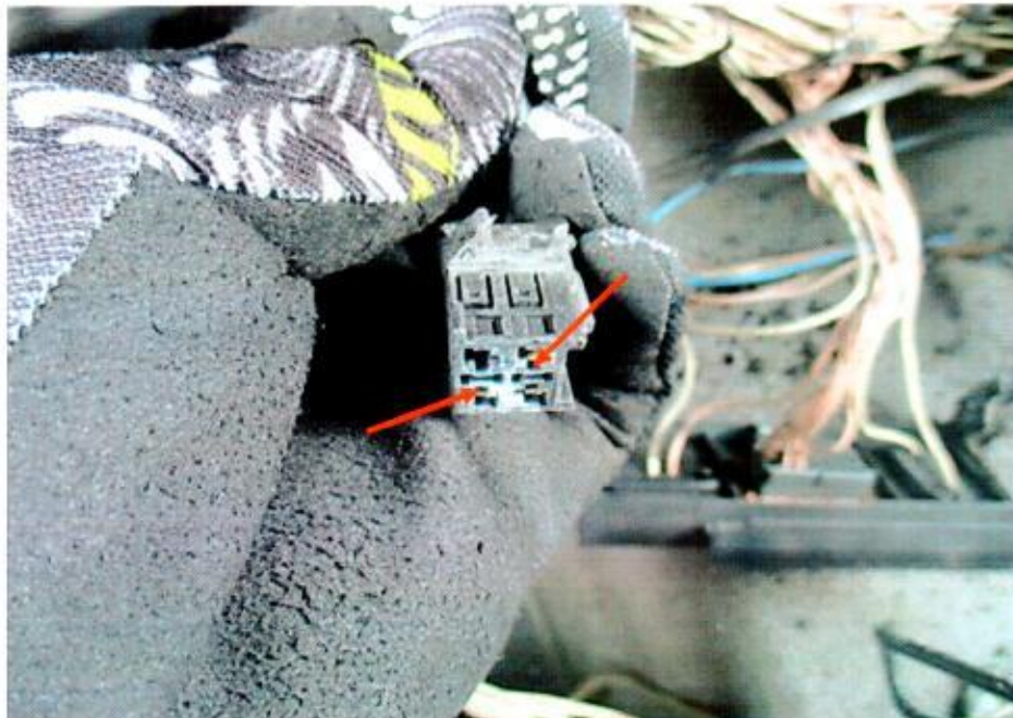
Photo 13 shows a close up view of the greenish residue found on the front portion of the air- conditioning blower connector (red arrows). The presence of such greenish residue suggests occurrence of an electrical short circuit.
