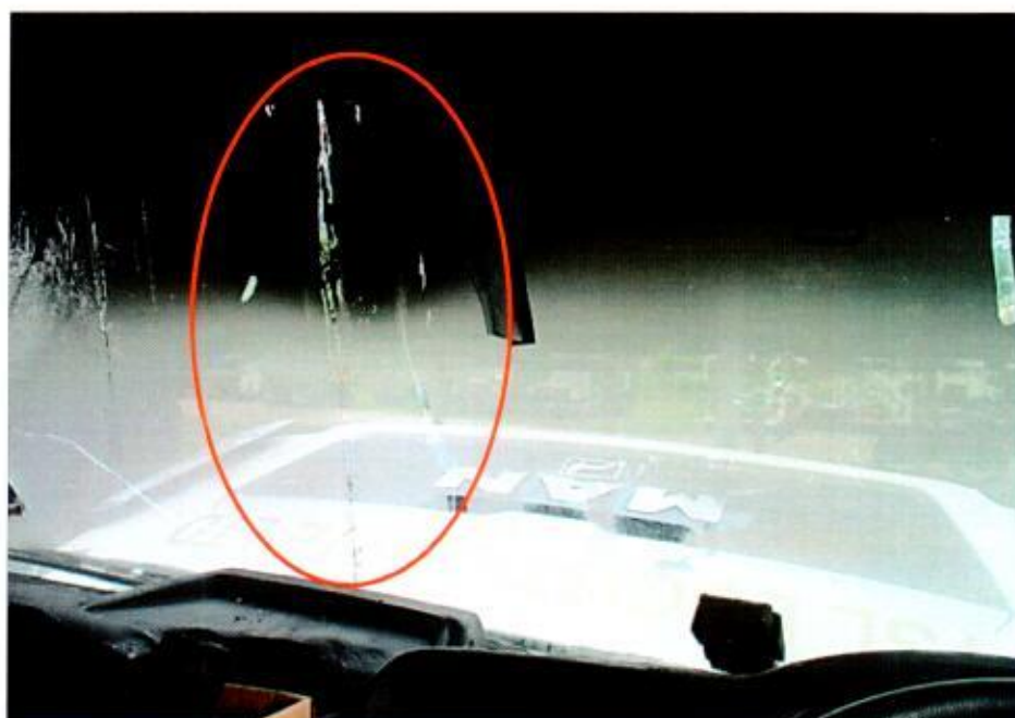
Photo 2 shows the general view of the front windscreen of the Insured Vehicle (as viewed from the interior compartment). The centre portion of the windscreen seemed to have sustained visible fire damage (circled).
