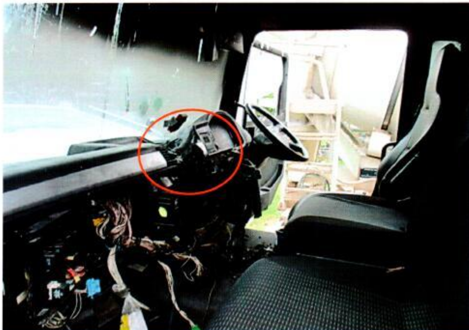
Photo 6 shows the interior compartment of the Insured Vehicle at the time of inspection. Most of the components in the centre of the dashboard (circled) were found to be burnt and/or melted as a result of the fire.
