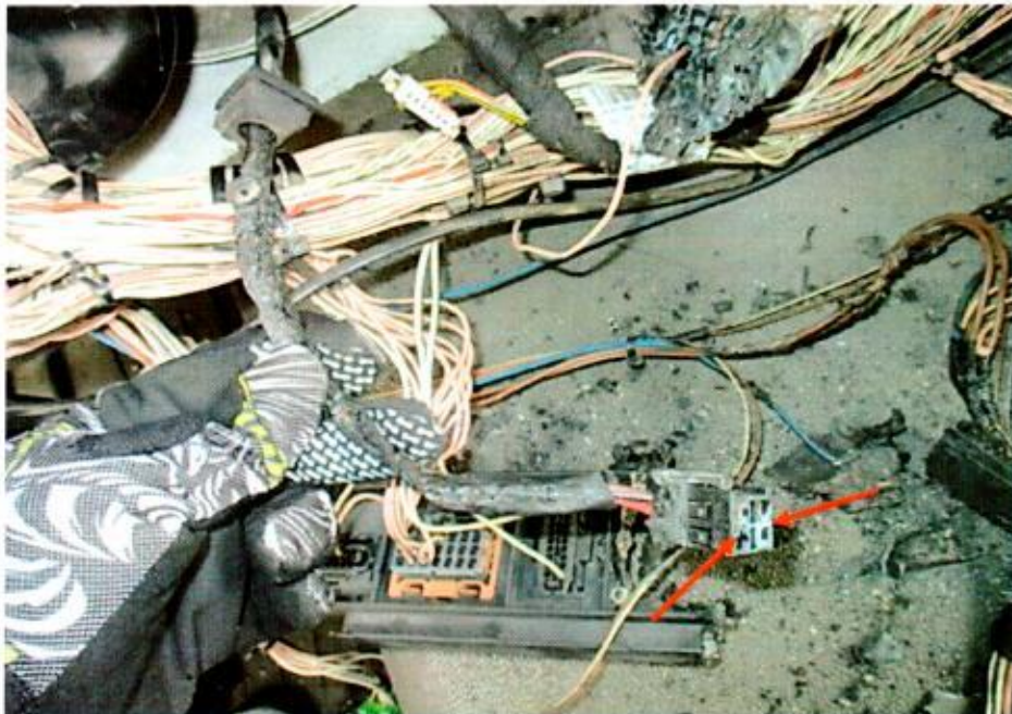
Photo 12 shows traces of greenish residue found on the front portion of the air-conditioning blower connector (red arrows). The presence of such greenish residue suggests occurrence of an electrical short circuit.
