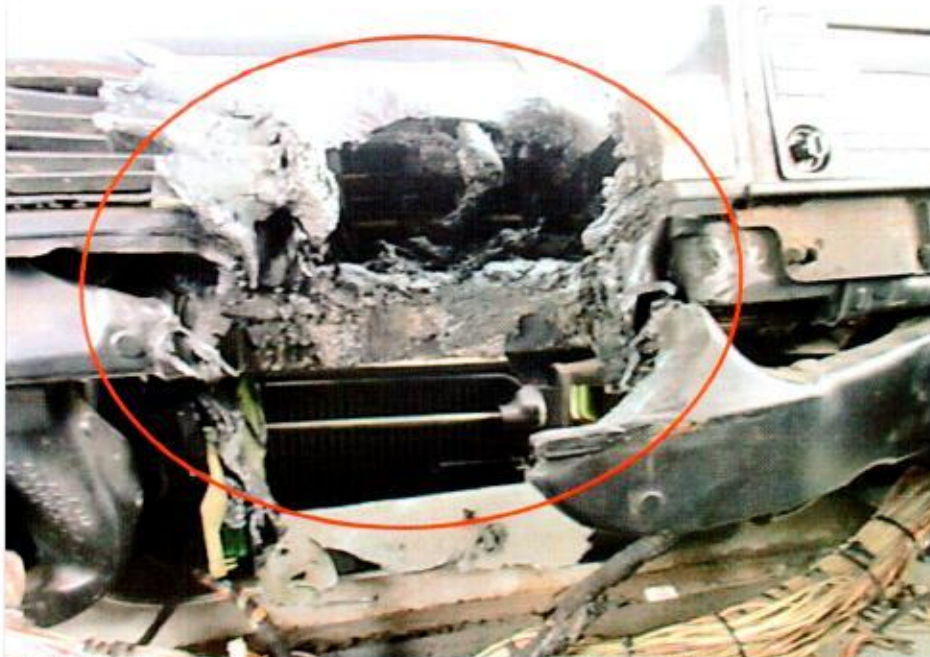
Photo 8 shows a closer view of the centre portion of the instrument panel. Various components of the instrument panel were observed to have been burnt and/or partly melted from prolonged exposure to high heat intensity which included the upper and central parts of the instrument panel assembly, air outlet assembly, beaker holder assembly and carrier assembly, amongst others (circled).
