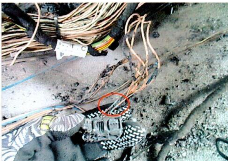
Photo 10 shows some original factory fitted wirings leading to a connector with greenish residue (circled). The presence of such greenish residue suggests occurrence of an electrical short circuit.
