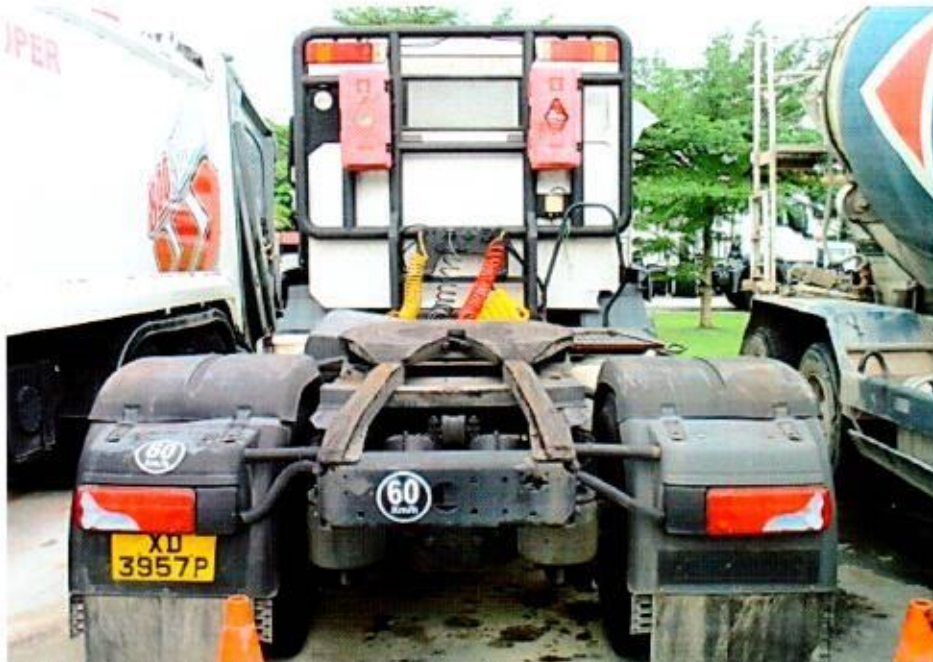
Photo 5 shows the rear view of the Insured Vehicle at the time of our inspection. The fire damage to the Insured Vehicle was confined to its interior compartment. The rear portion was observed to have been unaffected by the fire.
