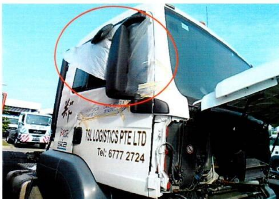
Photo 3 shows the right side view of the Insured Vehicle at the time of our inspection. The fire damage to the Insured Vehicle was confined to its interior compartment. The right side was observed to have been unaffected by the fire except for the driver door window (circled).
