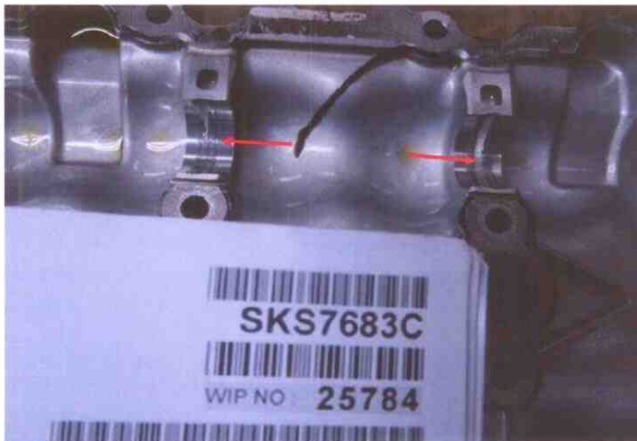
Photo 6 shows the scoring marks (arrowed) that were seen on the under surface of the engine top cover, at the area where the camshaft lobes sit (from the photographs that were provided to me). Such scoring marks are usually due to moving/rotating mechanical parts inside the engine coming into contact with each other as a result of insufficient lubricant (engine oil).
