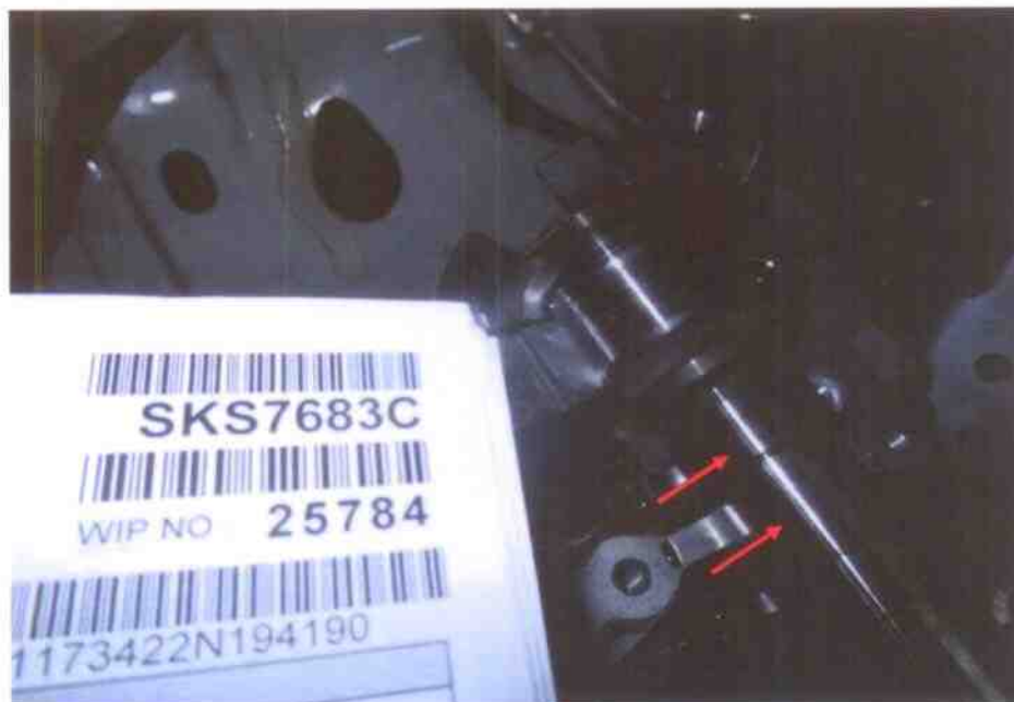
Photo 5 shows the scoring marks (arrowed) that were seen on the camshaft lobe of the Insured Vehicle (from the photographs that were provided to me). Such scoring marks are usually due to moving/rotating mechanical parts inside the engine coming into contact with each other as a result of insufficient lubricant (engine oil).
