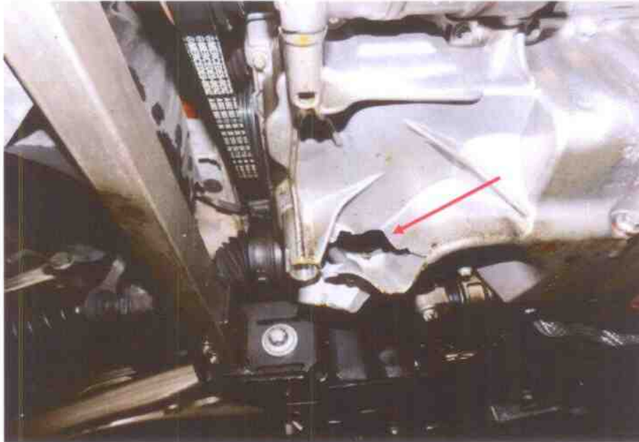
Photo 3 shows a closer view of the broken engine oil sump (red arrow) of the Insured Vehicle. The damage profile of the engine oil sump corresponds to the Insured Vehicle going over an object.
