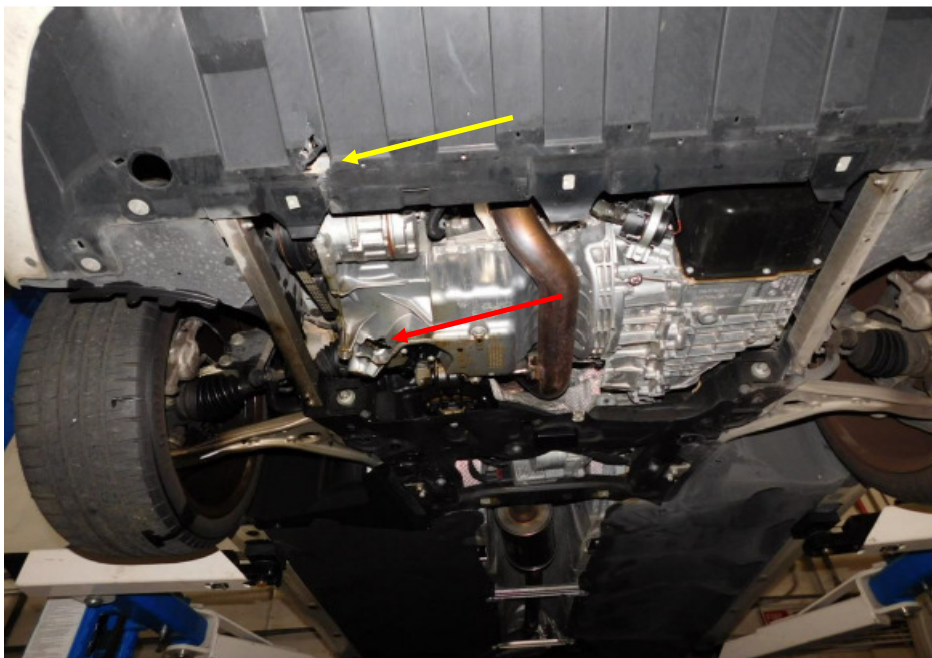
Photo 2 shows the torn front engine undercover (yellow arrow) and broken engine oil sump (red arrow) of the Insured Vehicle.
