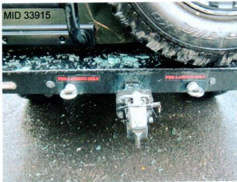
Pic A-4: Zoom in photo of scratched tow eye of MID 33915.
