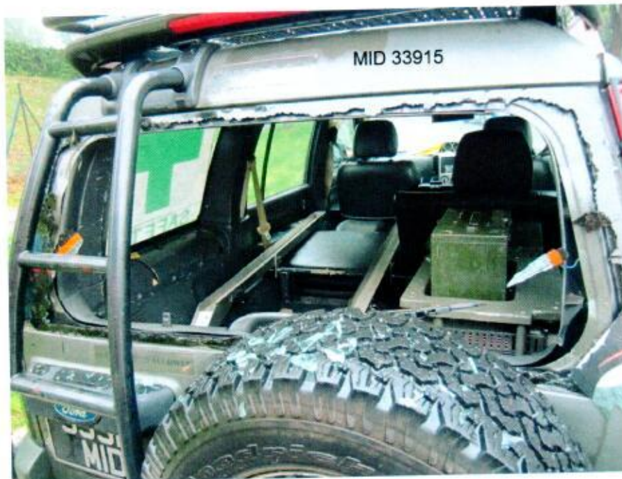
Pic A-4: Rear windscreen shattered and scratches to tow eye of MID 33915
