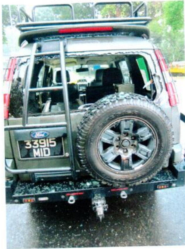
Pic A-4: Rear windscreen shattered and scratches to tow eye of MID 33915
