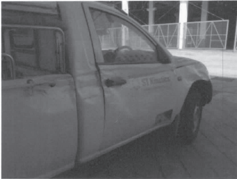
Pic A-7. Dents on Right Side Door and Chassis of STK Pickup Truck
