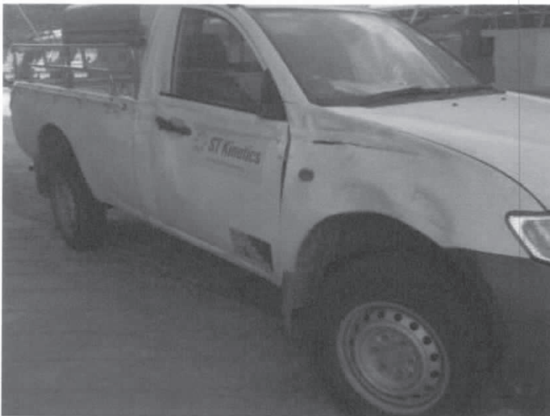
Pic A-6. Dents on Right Fender of STK Pickup Truck
