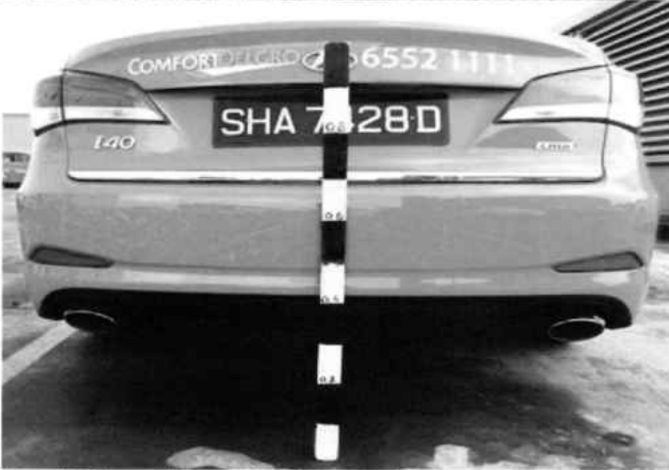
Shows the damaged front number plate taken by insured at the accident scene Shows the height measurement conducted on a similar make & model as the taxi
