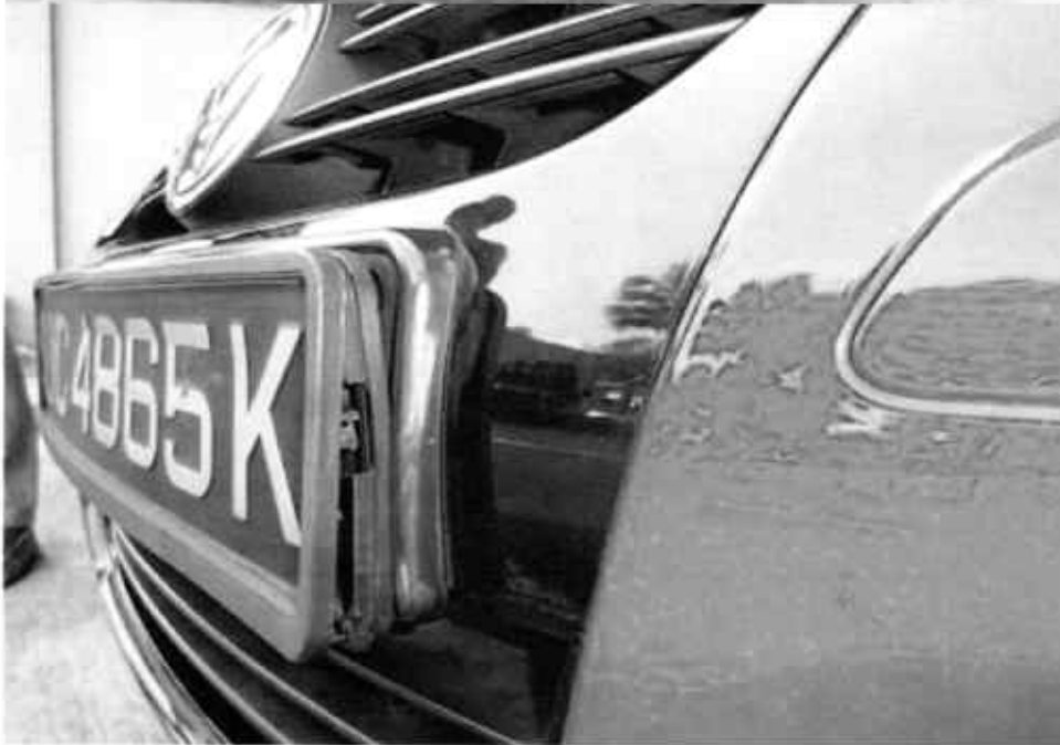
Shows the indentation on the Volkswagen front number plate Shows a closer view of the damaged front number plate & frame holder
