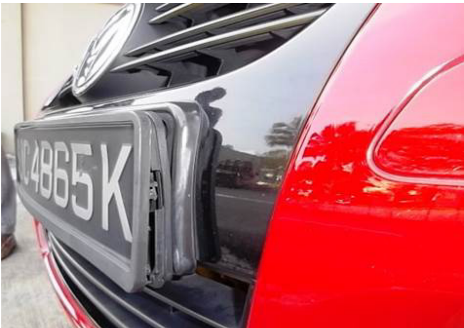
Shows the indentation on the Volkswagen front number plate damaged front number plate & frame holder
