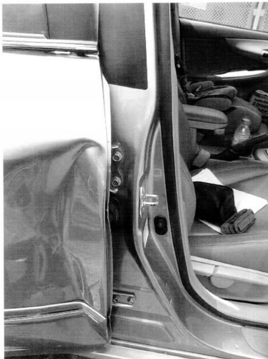
5/5: Photographs of Damaged Parts Centre Door Pillar R/H
