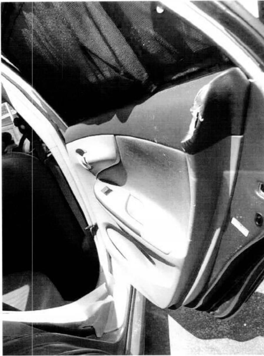
4/5: Photographs of Damaged Parts Rear Door Trim Board R/H
