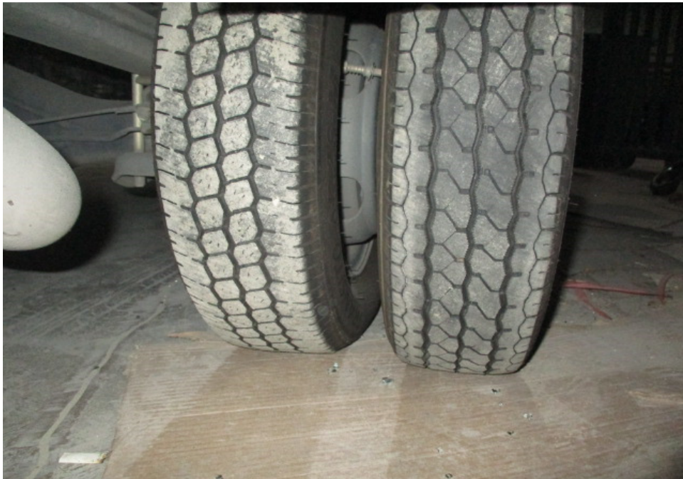
Photo 5 shows the right rear tyres of the Insured Vehicle at the time of our inspection. The right rear tyres of the Insured Vehicle were observed to be in serviceable condition. The pattern of the tread was generally still visible. The remaining tread depth was measured to be approximately 4mm.
