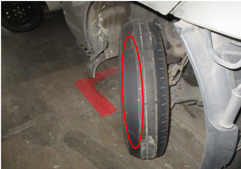
Photo 10 shows the left front tyre of the Insured Vehicle at the time of our inspection. The rubber at the outer side of the tread was partially worn (circled). The pattern at some areas on the outer side of the tread was vaguely visible due to worn rubber however the reinforcing belts that are found within the tyre were not exposed at the time of our inspection.
