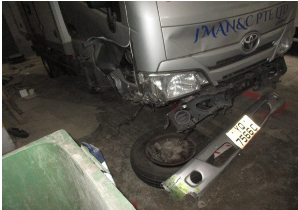
Photo 2 shows the close up view of the right frontal body of the Insured Vehicle at the time of our inspection. Its right front door was observed to be damaged as a result of the incident. The right front tyre was also found to be dislodged as a result of the incident.
