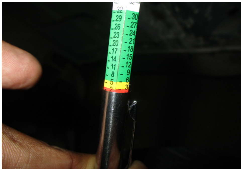
Photo 17 shows a close up view of the measurements being conducted on the remaining tread depth of the left front tyre of the Insured Vehicle. The remaining tread depth at the inner side of the left front tyre was measured to be approximately 2mm.
