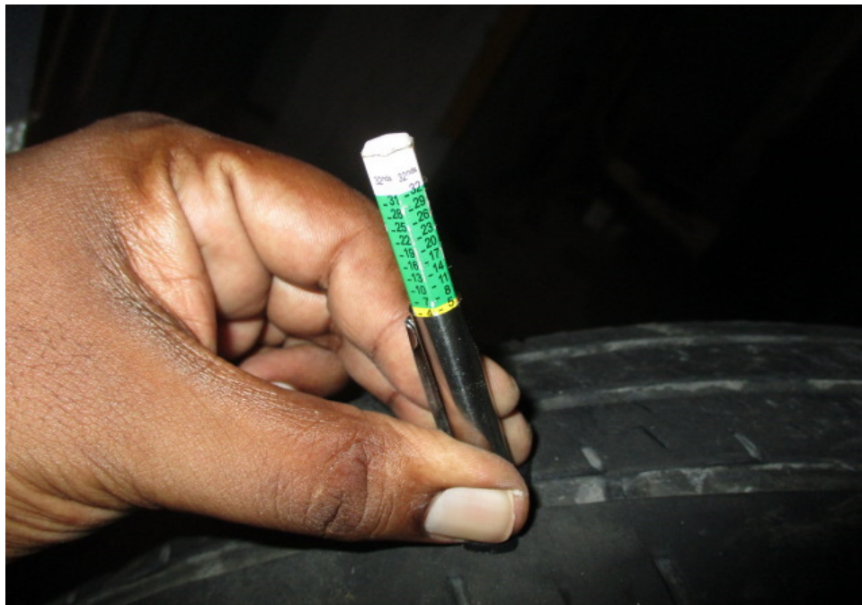
Photo 8 shows measurements being conducted on the remaining tread depth of the dislodged right front tyre of the Insured Vehicle. The remaining tread depth was measured to be approximately 4mm which is within the LTA requirements.
