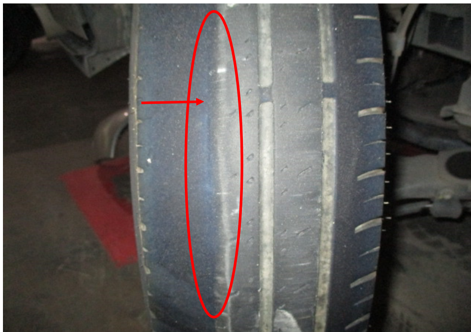
Photo 11 shows a close up view of the left front tyre of the Insured Vehicle at the time of our inspection. The rubber at the outer side of the tread was partially worn (circled). The pattern at the outer side of the tread was also observed to be flushed with the tyre wear indicator (arrowed).
