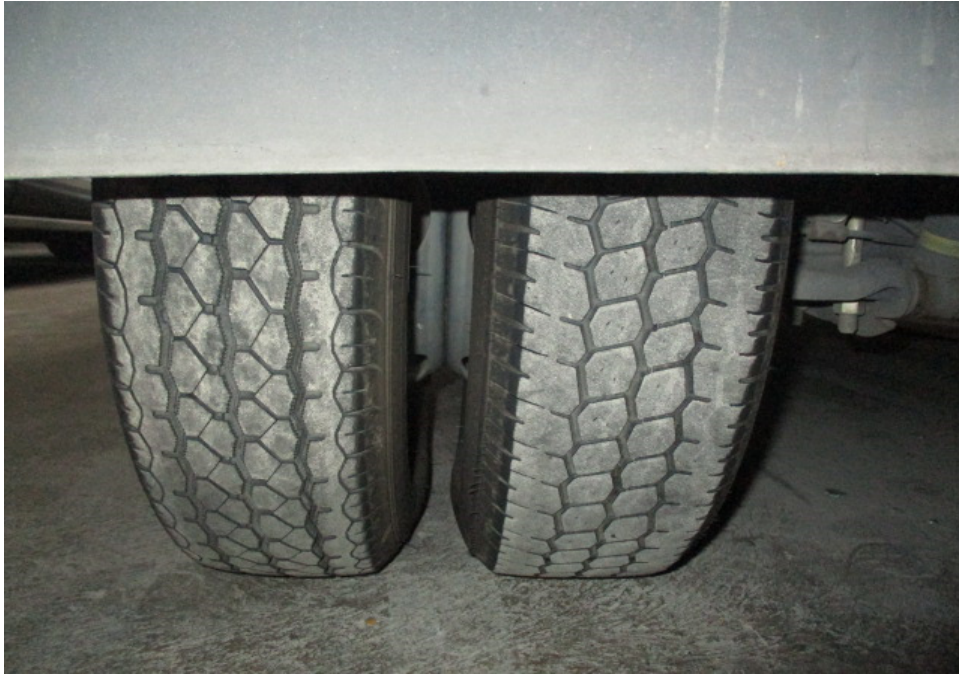
Photo 4 shows the left rear tyres of the Insured Vehicle at the time of our inspection. The left rear tyres of the Insured Vehicle were observed to be in serviceable condition. The pattern of the tread was generally still visible. The remaining tread depth was measured to be approximately 3mm.
