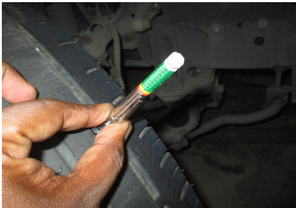
Photo 16 shows measurements being conducted on the remaining tread depth of the left front tyre of the Insured Vehicle. The remaining tread depth at the inner side of the left front tyre was measured to be approximately 2mm.
