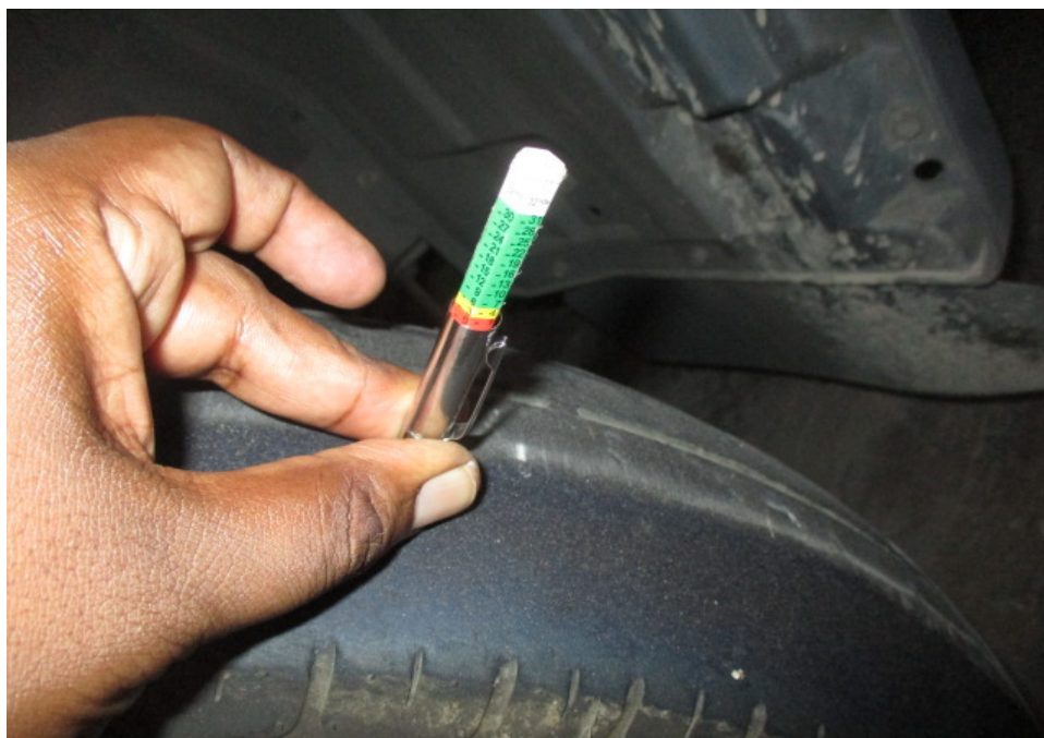
Photo 12 shows measurements being conducted on the remaining tread depth of the left front tyre of the Insured Vehicle. The remaining tread depth was measured to be approximately 0.0mm and 0.2mm which is not within the LTA requirements.
