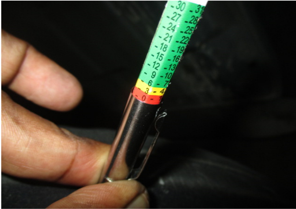
Photo 13 shows a close up view of the measurements being conducted on the remaining tread depth of the left front tyre of the Insured Vehicle. The remaining tread depth at the outer side of the left front tyre was measured to be approximately 0.0mm and 0.2mm which is not within the LTA requirements.
