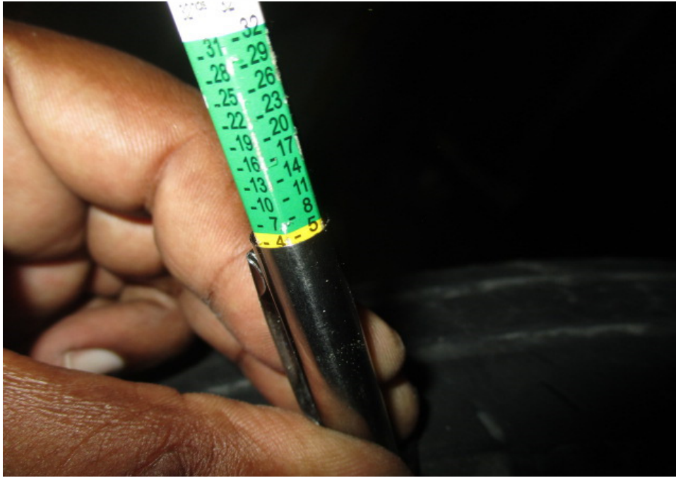
Photo 9 shows a close up view of the measurements being conducted on the remaining tread depth of the dislodged right front tyre of the Insured Vehicle. The remaining tread depth at the outer side of the right front tyre was measured to be approximately 4mm.
