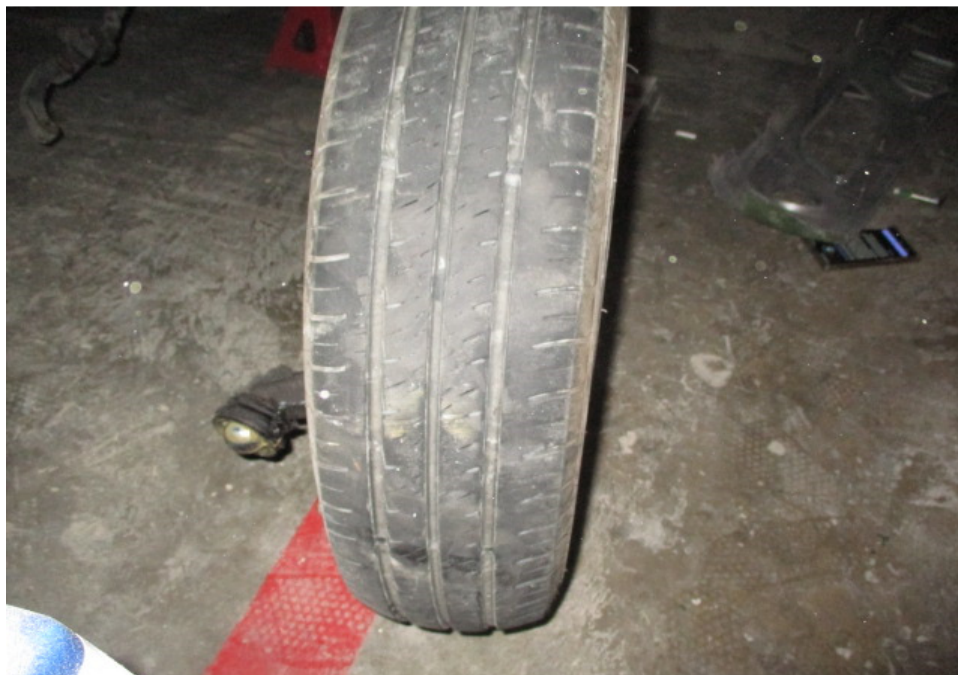
Photo 6 shows the dislodged right front tyre of the Insured Vehicle at the time of our inspection. The right front tyre of the Insured Vehicle was observed to be in serviceable condition. The pattern of the tread was generally still visible. The remaining tread depth was measured to be approximately 4mm.
