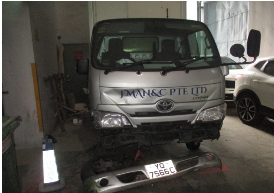
Photo 1 shows a general view of the frontal portion of the Insured Vehicle at the time of our inspection. The Insured Vehicle was observed to have sustained damage at its frontal portion and right front body. Its front body panel, right headlamp and front bumper were amongst the body parts damaged as a result of the incident.
