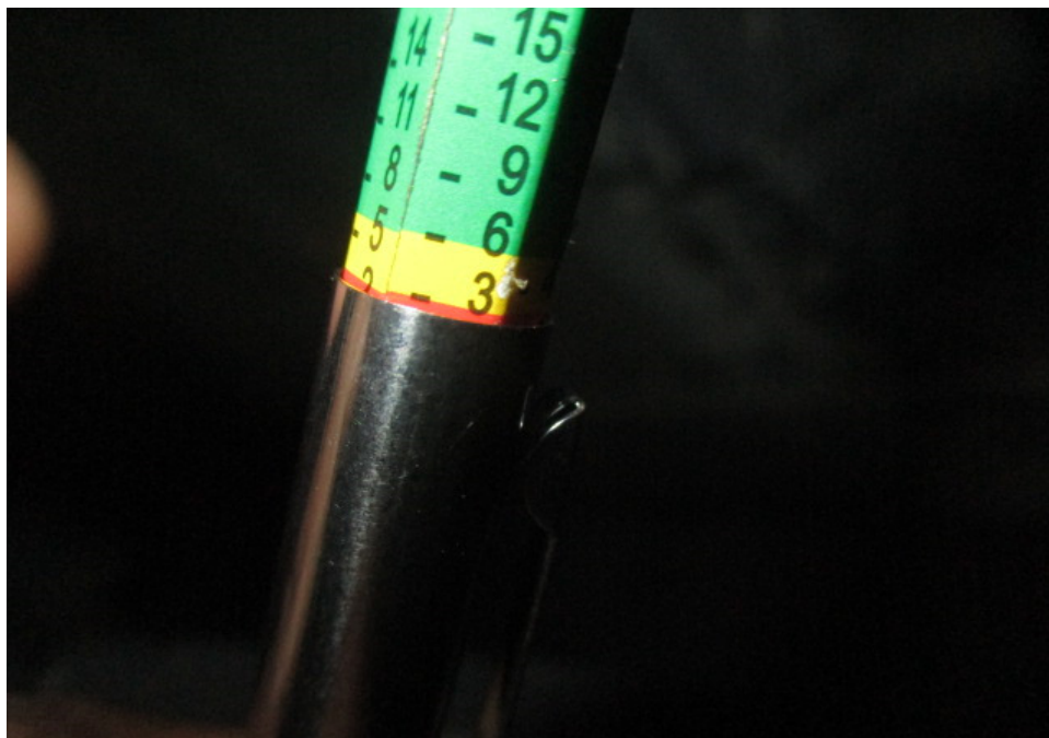
Photo 15 shows a close up view of the measurements being conducted on the remaining tread depth of the left front tyre of the Insured Vehicle. The remaining tread depth at the centre of the left front tyre was measured to be approximately 2mm.
