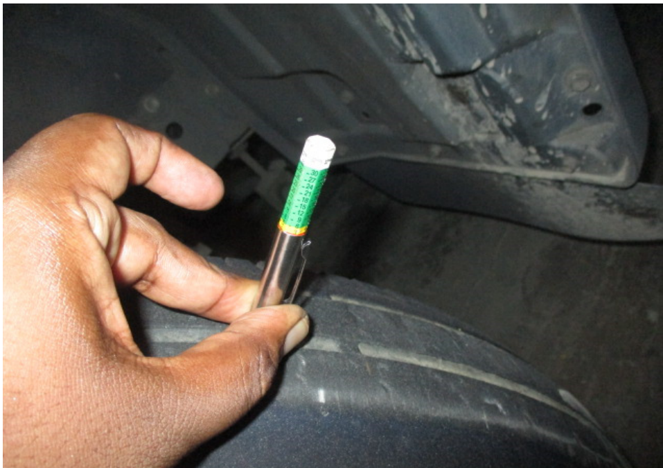
Photo 14 shows measurements being conducted on the remaining tread depth of the left front tyre of the Insured Vehicle. The remaining tread depth at the centre of the left front tyre was measured to be approximately 2mm.
