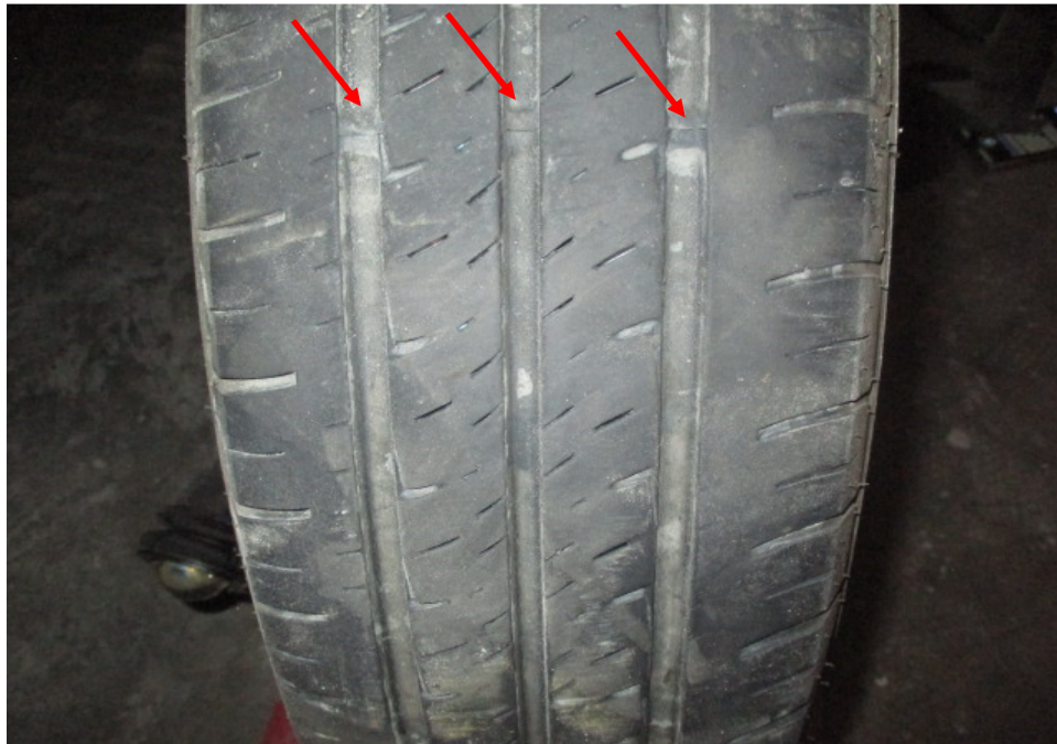
Photo 7 shows a closer view of the dislodged right front tyre of the Insured Vehicle at the time of our inspection. The pattern of the tread was generally still visible. The tyre wear indicators (arrowed), normally built into the groove of the tread pattern, were also observed to be not flushed with the tread pattern.
