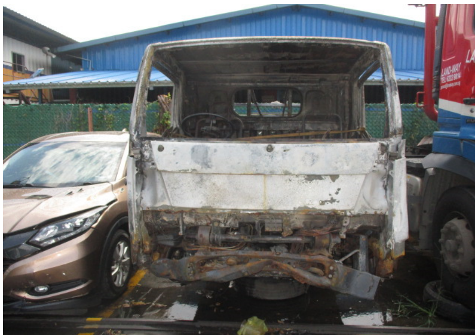
Photo 2 shows the general view of the frontal portion of the Insured Vehicle at the time of our inspection. The Insured Vehicle was observed to have sustained extensive fire damage all around. Its engine compartment and interior compartment were completely burnt. Rust had accumulated all over the Insured Vehicle as a result of exposure to environmental condition for a period of time.
