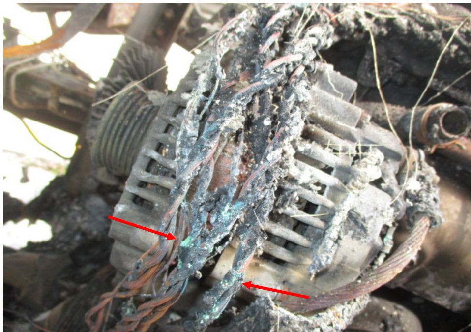
Photo 11 shows a close up view of the greenish residue found on the wirings around the centre portion of the engine compartment of the Insured Vehicle (arrowed). This physical evidence would then appear to suggest that the cause of fire to the Insured Vehicle could have possibly been due to electrical in nature.
