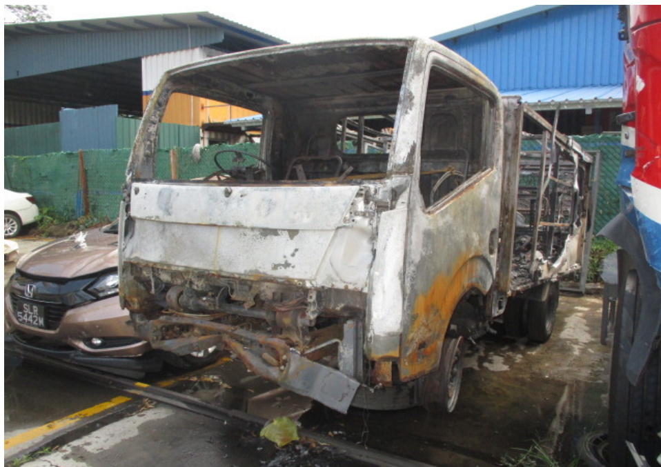
Photo 3 shows the general view of the left body of the Insured Vehicle at the time of our inspection. The Insured Vehicle was observed to have sustained extensive fire damage all around. Rust had accumulated all over the Insured Vehicle as a result of exposure to environmental condition for a period of time.
