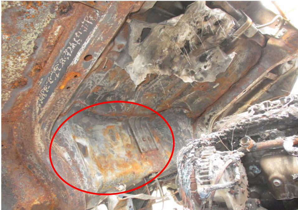
Photo 6 shows the whitish burn marks that were found on the underside of the cab of the Insured Vehicle (circled). Such whitish burn marks are a result of exposure to prolonged heat intensity.
