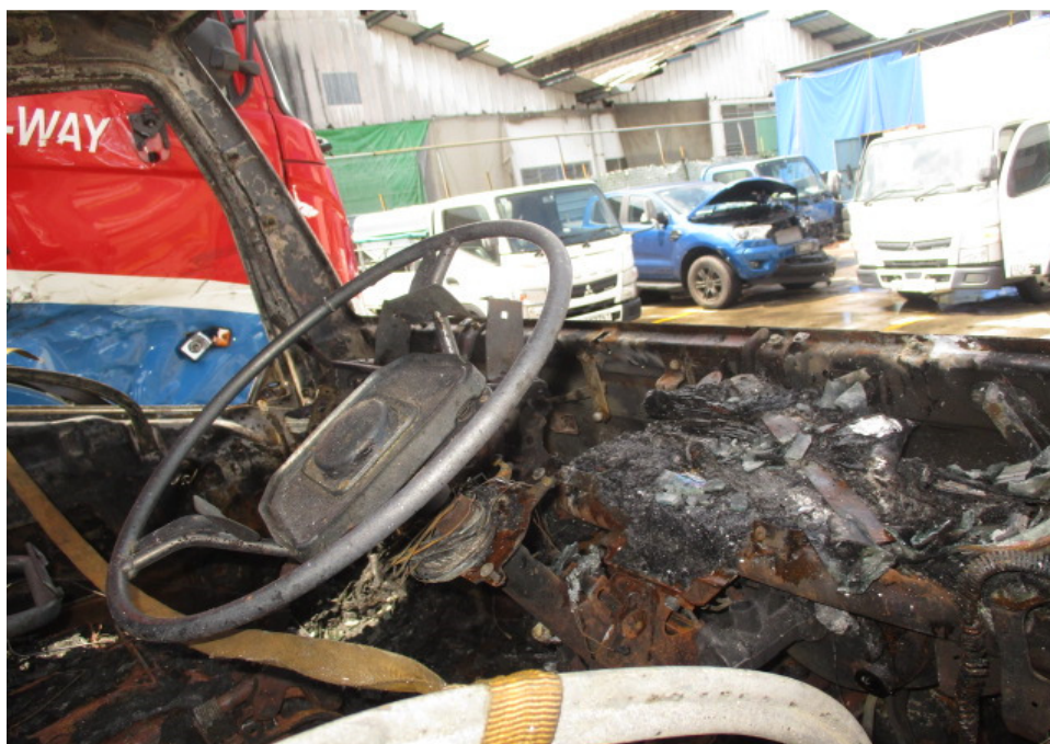
Photo 4 shows the general view of the interior compartment of the Insured Vehicle at the time of our inspection. Its interior compartment was completely burnt.
