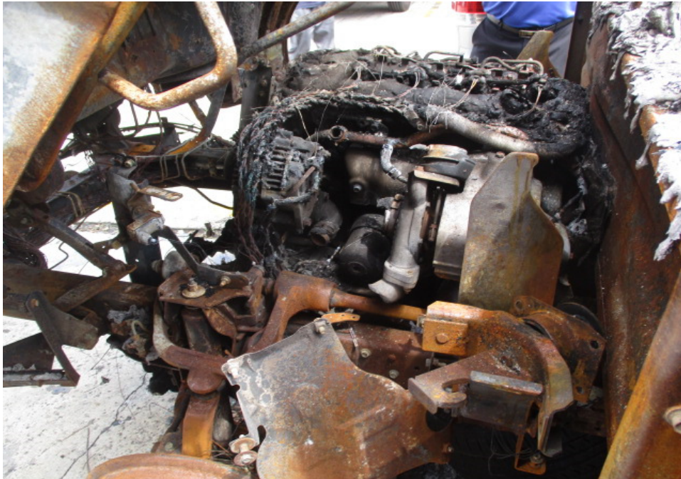
Photo 5 shows the engine compartment of the Insured Vehicle which is situated beneath the cab at the time of our inspection. The entire engine compartment of the Insured Vehicle was observed to be severely burnt. Most of the parts inside the engine compartment were found to be burnt and/or melted as a result of the fire.
