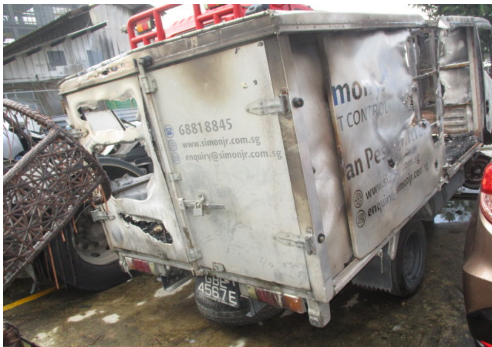
Photo 1 shows the general view of the rear portion of the Insured Vehicle at the time of our inspection. The Insured Vehicle was observed to have sustained extensive fire damage all around.
