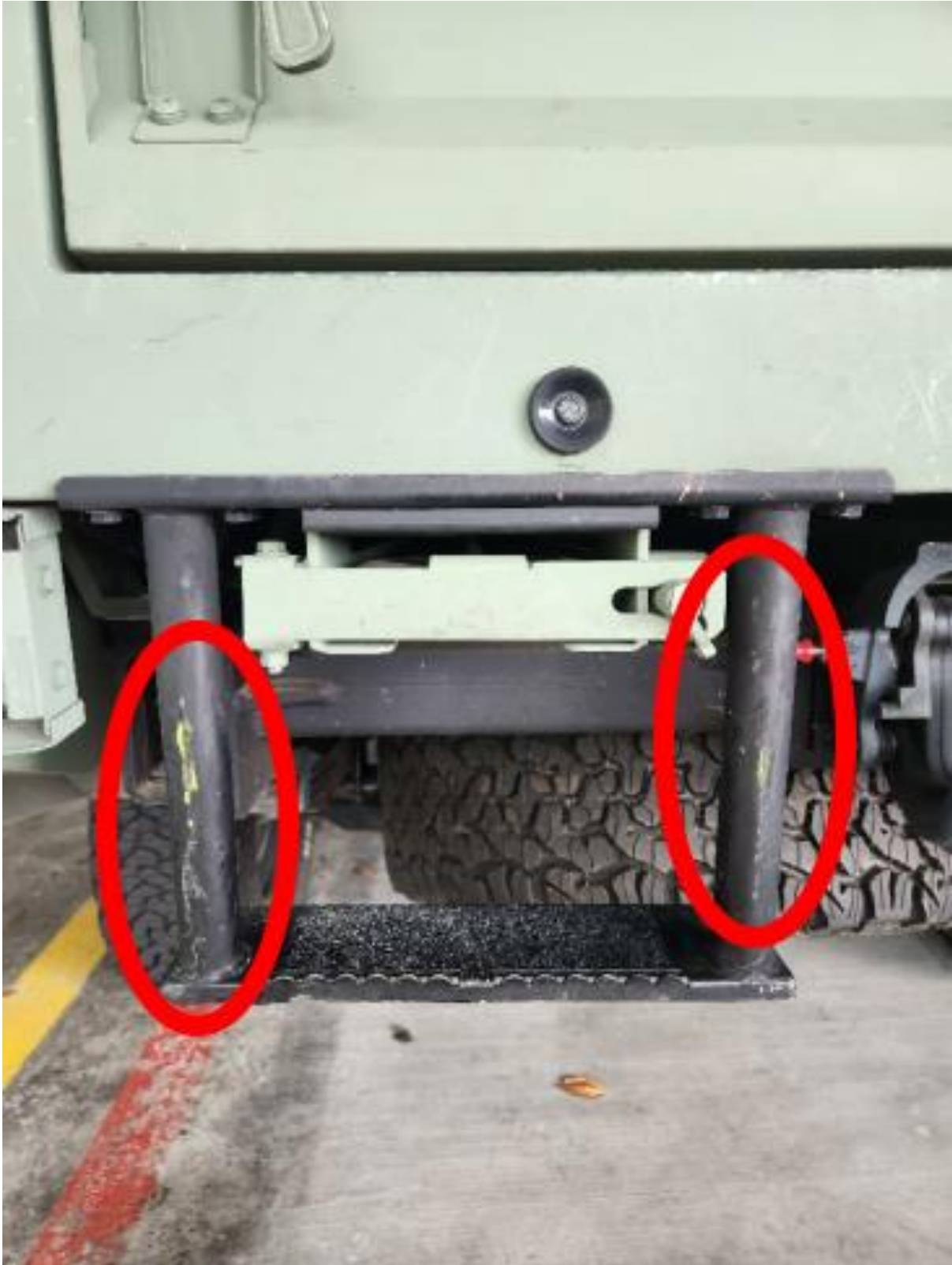
Figure B-6: Zoomed-in View of MID36113 Damages
