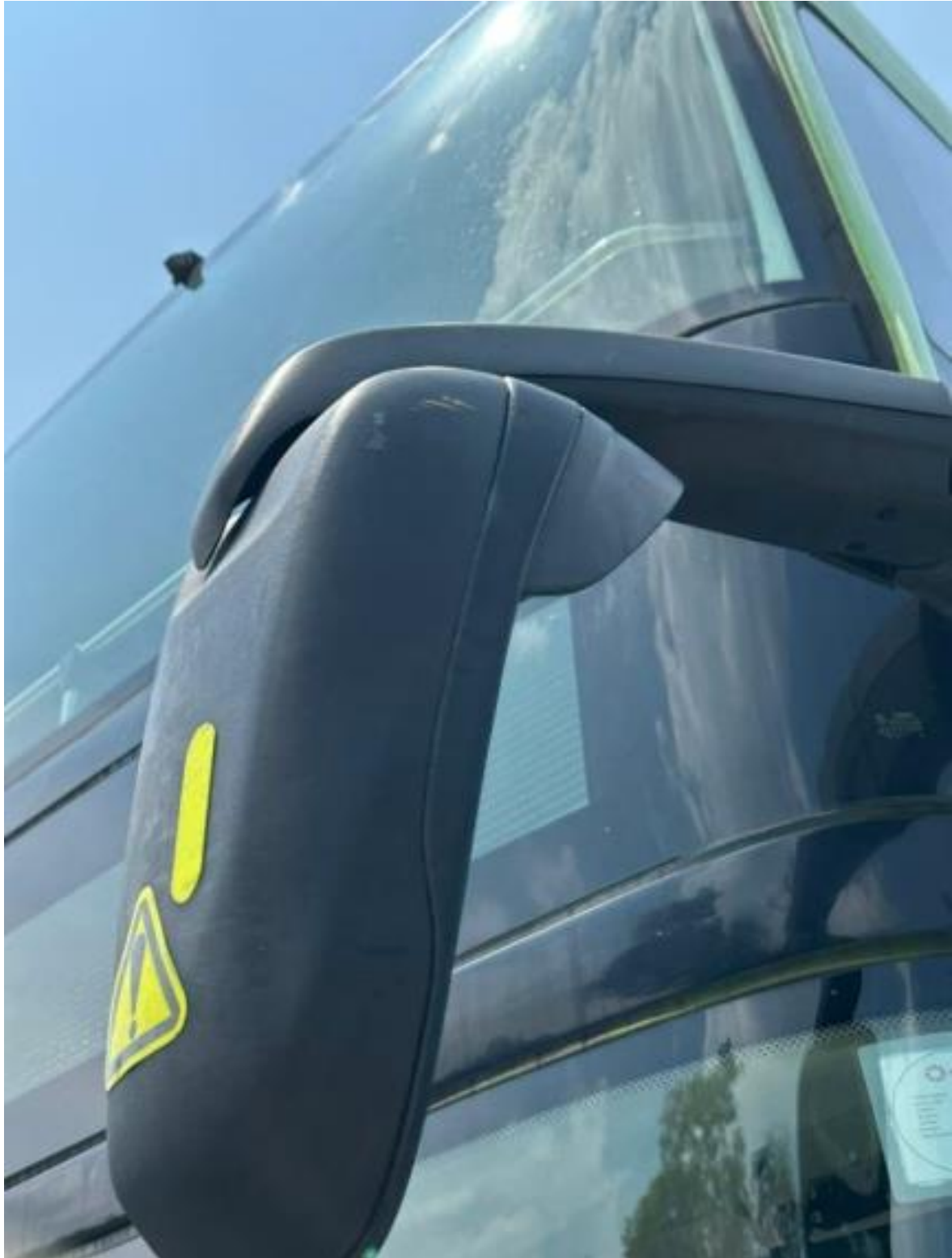
Figure B-3: G5850 damage - yellow paint marks on the top edge of the left mirror of the bus
