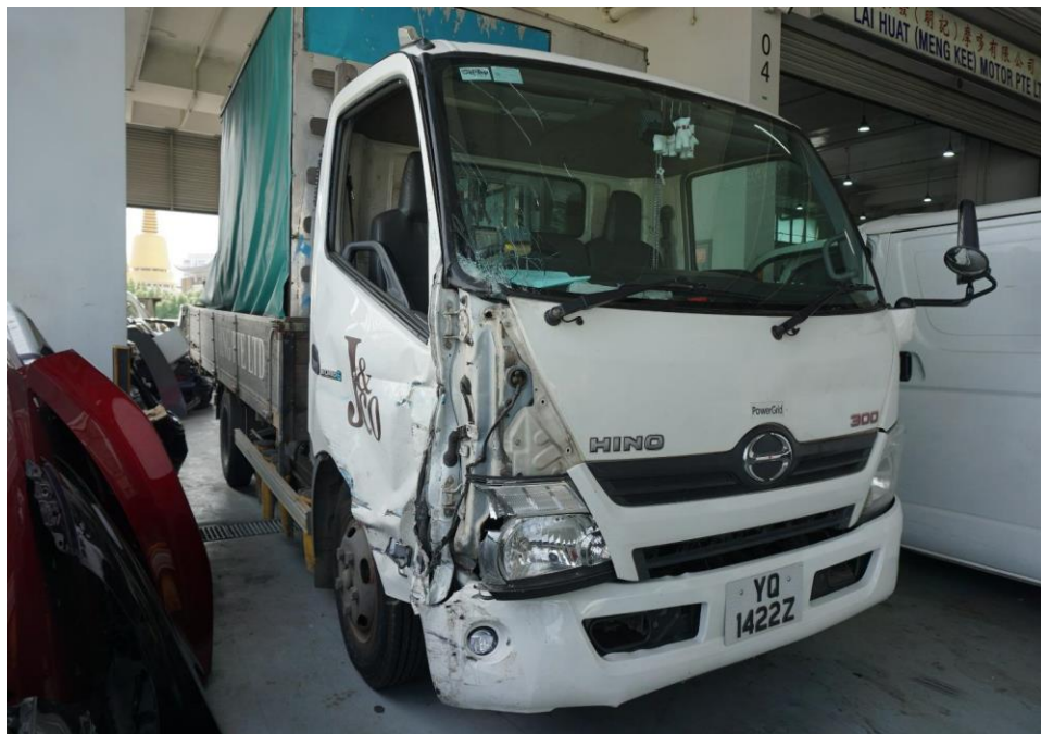
Photo 1 shows a general view of the Insured Vehicle front portion at the time of my inspection. The Insured Vehicle was observed to have sustained damage at its front portion. Its front windscreen, front body panel, front right headlamp and front bumper was amongst the body parts damaged as a result of the accident.
