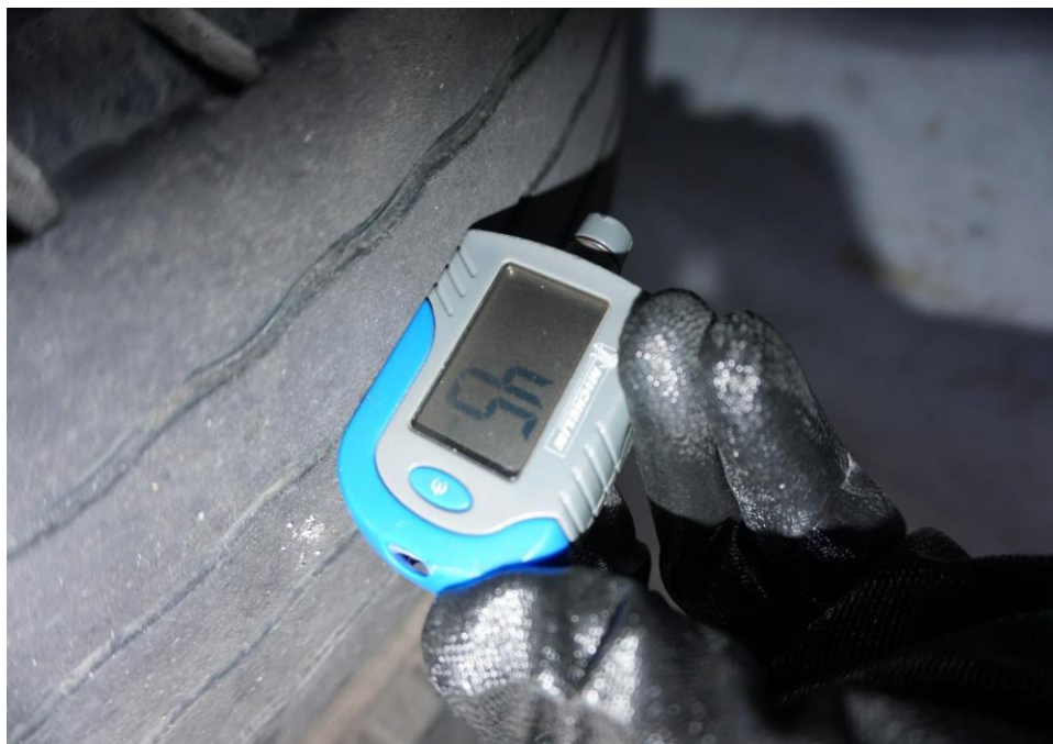
Photo 8 shows the tread depth of the rear right outer tyre on the insured vehicle at the time of my inspection. The remaining tread depth is 4.5mm which is within the LTA requirements.
