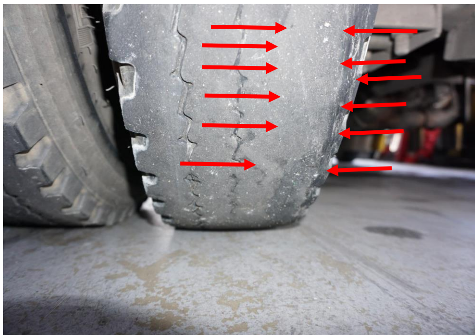
Photo 16 shows a general view of the rear left inner tyre of the insured vehicle at the time of my inspection. The rubber compound at the inner side of the tyre, around 50% of its circumference, was observed to be worn (red arrows).
