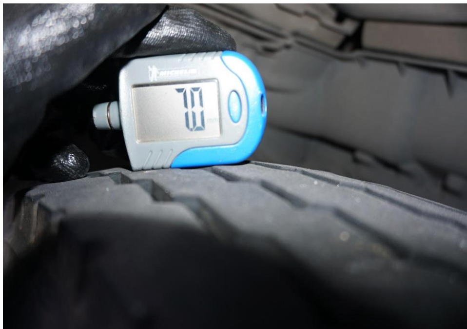
Photo 4 shows the tread depth of the front right tyre on the insured vehicle at the time of my inspection. The remaining tread depth is 7mm which is within the LTA requirements.
