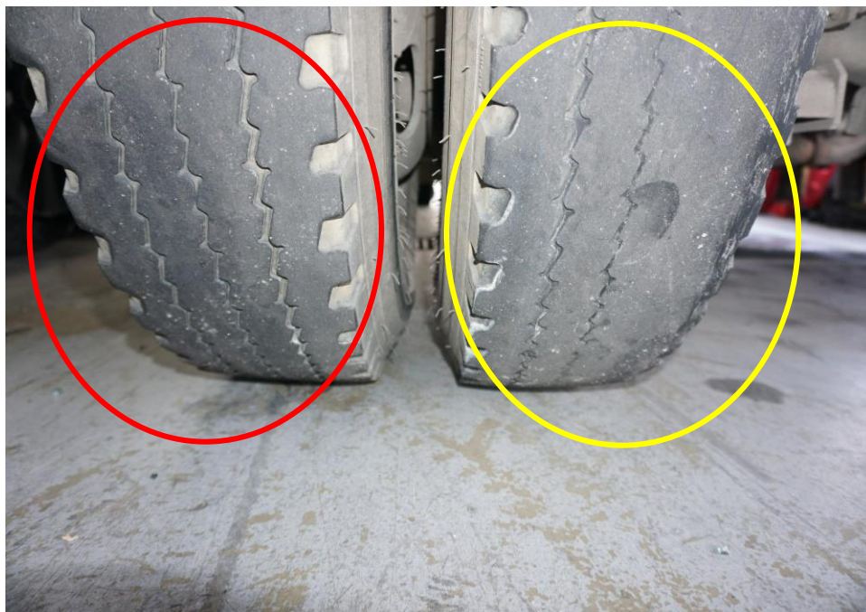
Photo 15 shows rear left tyre of the insured vehicle at the time of my inspection. The rear left tyres of the insured vehicle with remaining tread depth of 4.4mm on the rear left outer tyre (red circle) and 0.0mm on the rear left inner tyre (yellow circle).
