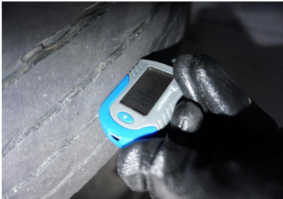
Photo 11 shows the tread depth of the rear left outer tyre on the insured vehicle at the time of my inspection. The remaining tread depth is 4.4mm which is within the LTA requirements.
