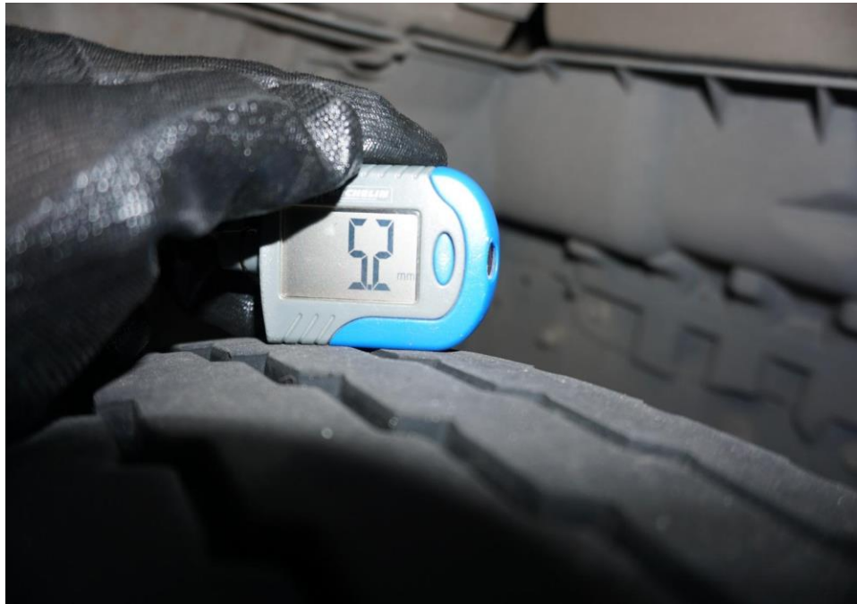
Photo 9 shows the tread depth of the rear right inner tyre on the insured vehicle at the time of my inspection. The remaining tread depth is 4.5mm which is within the LTA requirements.
