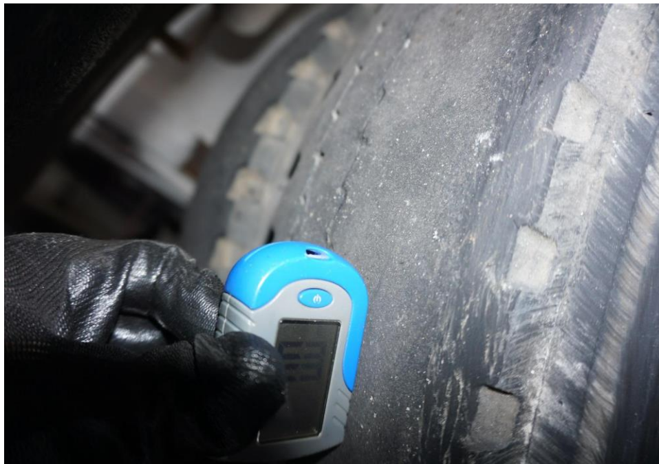
Photo 13 shows the tread depth of the rear left inner tyre (inner tread) on the insured vehicle at the time of my inspection. The remaining tread depth is 0.0mm which is not within the LTA requirements
