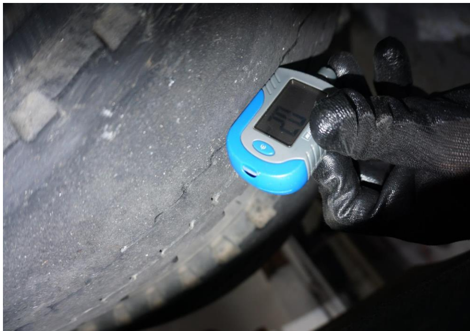
Photo 14 shows the tread depth of the rear left inner tyre (inner tread) on the insured vehicle at the time of my inspection. The remaining tread depth is 0.2mm which is not within the LTA requirements
