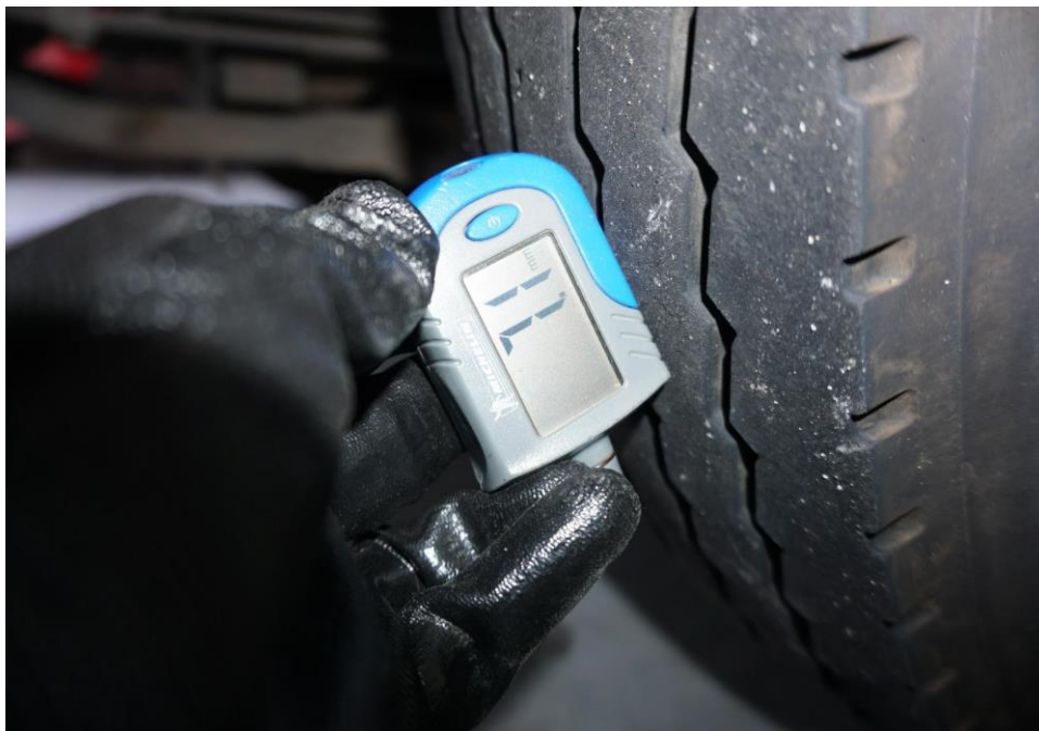
Photo 6 shows the tread depth of the front left tyre on the insured vehicle at the time of my inspection. The remaining tread depth is 7.1mm which is within the LTA requirements.
