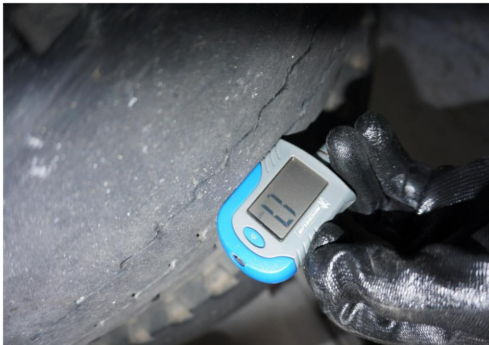
Photo 12 shows the tread depth of the rear left inner tyre (outer tread) on the insured vehicle at the time of my inspection. The remaining tread depth is 1.7mm which is within the LTA requirements.
