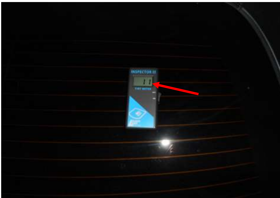
Photo 17 shows the window tint reading of the rear windscreen on the Insured Vehicle at the time of my inspection. The rear windscreen tint percentage is measured at 11% (red arrow) Visible Light Transmission (VLT) which is not within LTA requirements, as 25% of light must be able to pass through the rear windscreen and two rear side windows.
