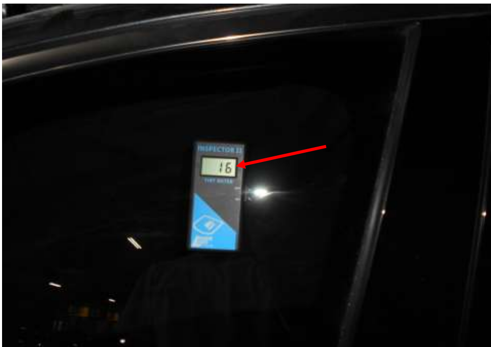
Photo 13 shows the window tint reading of the front left side window on the Insured Vehicle at the time of my inspection. The front left side window tint is measured at 16% (red arrow) Visible Light Transmission (VLT) which is not within LTA requirements, as 70% of light must be able to pass through the front windscreen and two front side windows.
