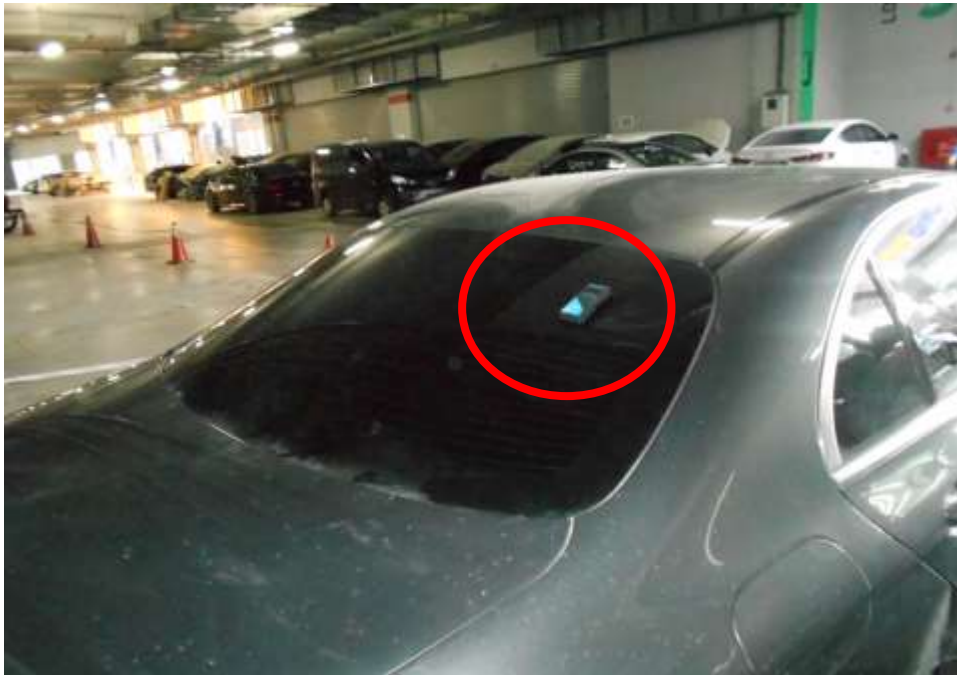
Photo 16 shows a general view of the measurement of the rear windscreen tint of the Insured Vehicle using a tint meter (red circle). Which measures the amount of Visible Light Transmission (VLT) that passes through a material. The Visible Light Transmission (VLT) measured on a scale of 0- 100%, with 0% meaning no light passes through and 100% meaning all light passes through.
