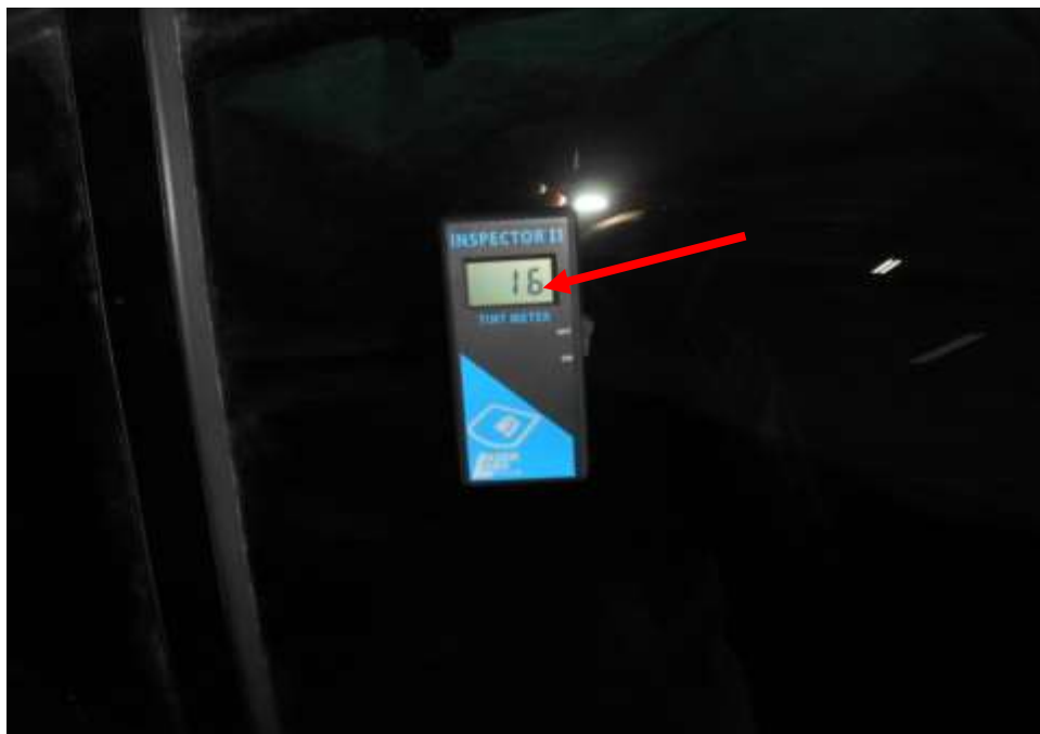
Photo 11 shows the window tint reading of the rear right side window on the Insured Vehicle at the time of my inspection. The rear right side window tint is measured at 16% (red arrow) Visible Light Transmission (VLT) which is not within LTA requirements, as 25% of light must be able to pass through the rear windscreen and two rear side windows.
