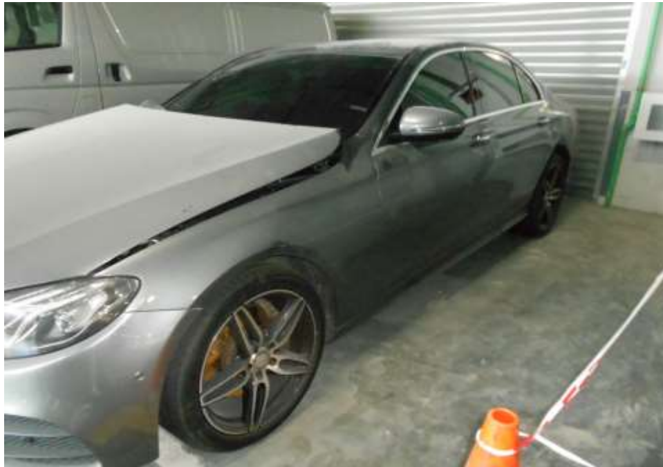
Photo 3 shows a general view of the Insured Vehicle left body at the time of my inspection. The Insured Vehicle was observed to have sustained damage at its left body. Its front left fender was amongst the body parts damaged as a result of the accident.
