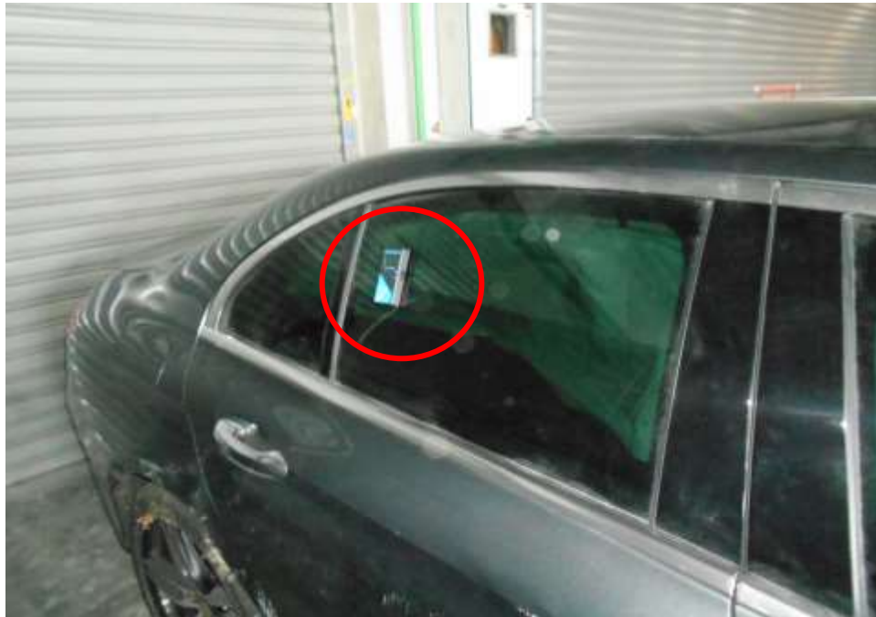
Photo 10 shows a general view of the measurement of the rear right window tint of the Insured Vehicle using a tint meter (red circle). Which measures the amount of Visible Light Transmission (VLT) that passes through a material. The Visible Light Transmission (VLT) measured on a scale of 0- 100%, with 0% meaning no light passes through and 100% meaning all light passes through.
