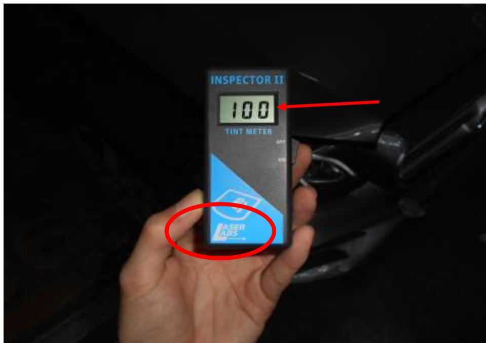
Photo 5 shows the Tint Meter used to measure the Visible Light Transmission (VLT) on the Insured Vehicle's windscreen and windows which has been recalibrated (red arrow) before the testing of the Visible Light Transmission (VLT) of the window and windscreen tints. The brand of the Tint Meter was 'Laser ABS'
