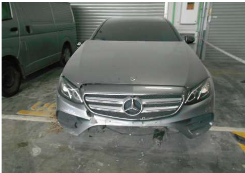
Photo 1 shows a general view of the Insured Vehicle front portion at the time of my inspection. The Insured Vehicle was observed to have sustained damage at its front portion. Its front bonnet and front bumper was amongst the body parts damaged as a result of the accident.
