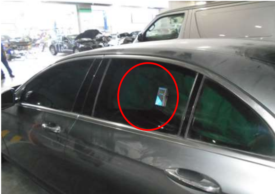
Photo 14 shows a general view of the measurement of the rear left window tint of the Insured Vehicle using a tint meter (red circle). Which measures the amount of Visible Light Transmission (VLT) that passes through a material. The Visible Light Transmission (VLT) measured on a scale of 0- 100%, with 0% meaning no light passes through and 100% meaning all light passes through.
