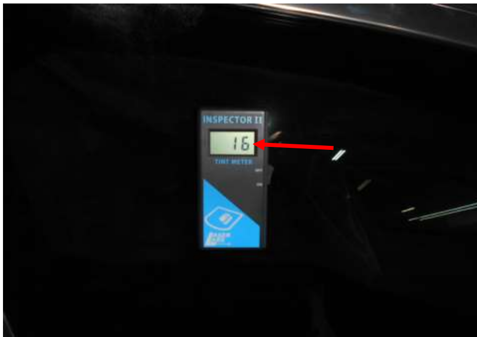
Photo 9 shows the window tint reading of the front right side window on the Insured Vehicle at the time of my inspection. The front right window tint is measured at 16% (red arrow) Visible Light Transmission (VLT) which is not within LTA requirements, as 70% of light must be able to pass through the front windscreen and two front side windows.
