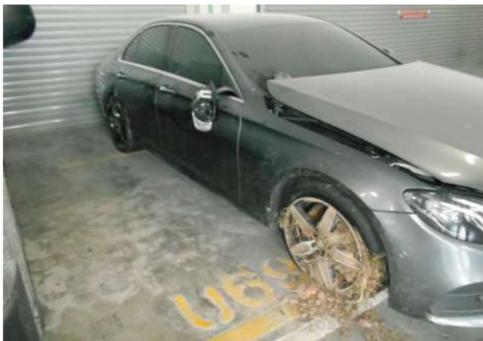
Photo 2 shows a general view of the Insured Vehicle right body at the time of my inspection. The Insured Vehicle was observed to have sustained damage at its right body. Its front right rear view mirror was amongst the body parts damaged as a result of the accident.
