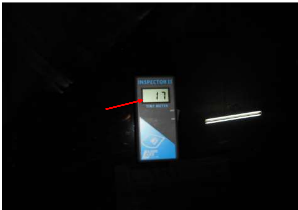
Photo 7 shows the window tint reading of the front windscreen on the Insured Vehicle at the time of my inspection. The front windscreen tint is measured at 17% (red arrow) Visible Light Transmission (VLT) which is not within LTA requirements, as 70% of light must be able to pass through the front windscreen and two front side windows.
