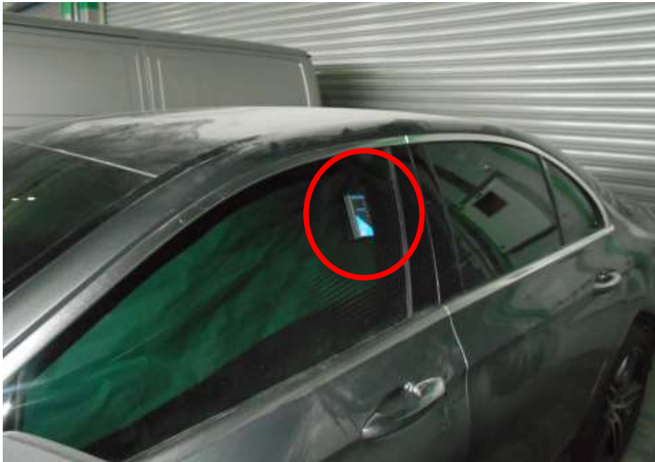
Photo 12 shows a general view of the measurement of the front left window tint of the Insured Vehicle using a tint meter (red circle). Which measures the amount of Visible Light Transmission (VLT) that passes through a material. The Visible Light Transmission (VLT) measured on a scale of 0- 100%, with 0% meaning no light passes through and 100% meaning all light passes through.
