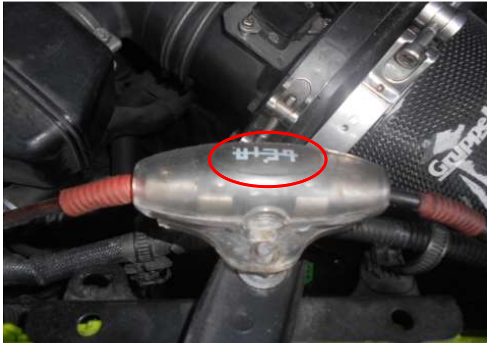
Photo 27 shows the close up view of the non- standard battery voltage stabilizer onto the Insured Vehicle upon our inspection (circled). The brand of the battery voltage stabilizer was 'bEiA' (circled).
