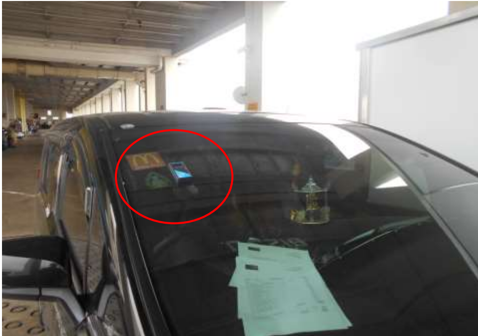
Photo 6 shows a general view of the measurement of the front windscreen tint of the Insured Vehicle using a tint meter (red circle) which measures the amount of Visible Light Transmission (VLT) that passes through a material. The Visible Light Transmission (VLT) measured on a scale of 0- 100%, with 0% meaning no light passes through and 100% meaning all light passes through.
