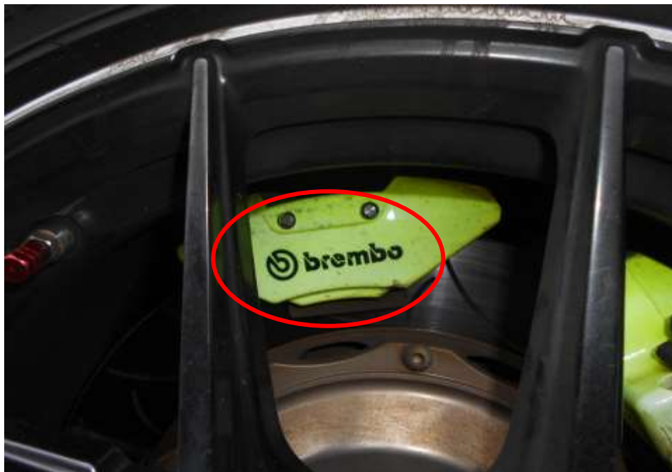
Photo 30 shows a close up view of the non- standard rear brake kit (circled) fitted onto the Insured Vehicle upon our inspection. The brand of the brake kit was 'brembo' (circled).
