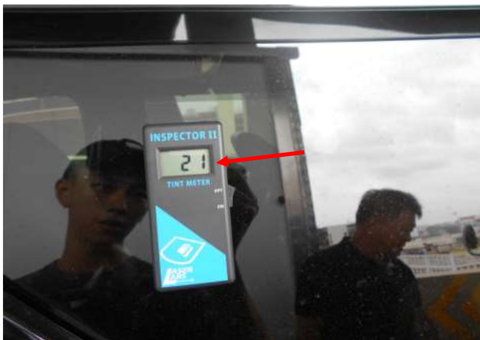
Photo 17 shows the window tint reading of the rear left centre side window on the Insured Vehicle at the time of my inspection. The rear left side window tint is measured 21% (red arrow) Visible Light Transmission (VLT) which is not within LTA requirements, as 25% of light must be able to pass through the rear windscreen and two rear side windows.
