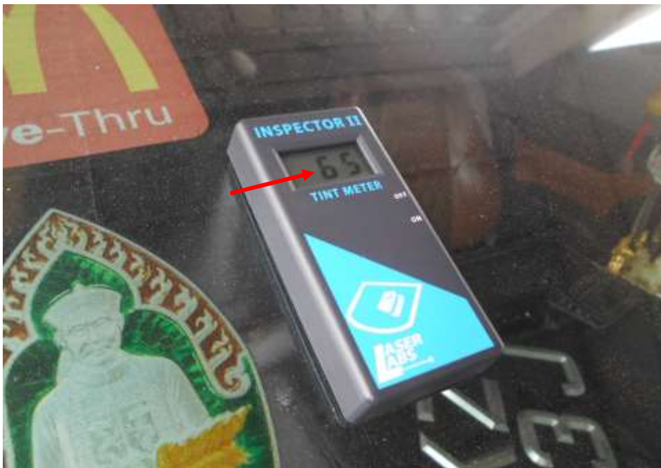
Photo 7 shows the window tint reading of the front windscreen on the Insured Vehicle at the time of my inspection. The front windscreen tint is measured at 65% (red arrow) Visible Light Transmission (VLT) which is not within LTA requirements, as 70% of light must be able to pass through the front windscreen and two front side windows.
