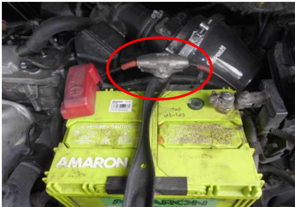
Photo 26 shows the general view close up view of the non- standard battery voltage stabilizer fitted onto the Insured Vehicle upon our inspection (circled).
