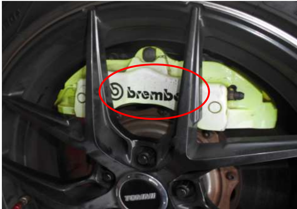
Photo 29 shows a close up view of the non- standard front brake kit (circled) fitted onto the Insured Vehicle upon our inspection. The brand of the brake kit was 'brembo' (circled).
