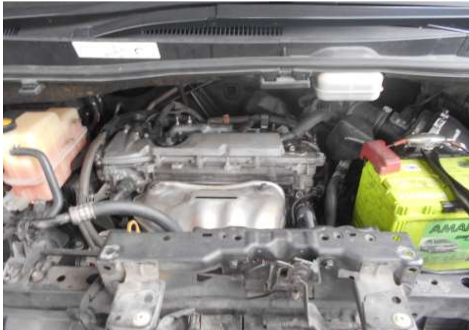
Photo 23 shows a general view of the engine compartment of the Insured Vehicle. Additional non-standard parts were found fitted. This includes a non-standard open pod air filter and a battery voltage stabilizer.
