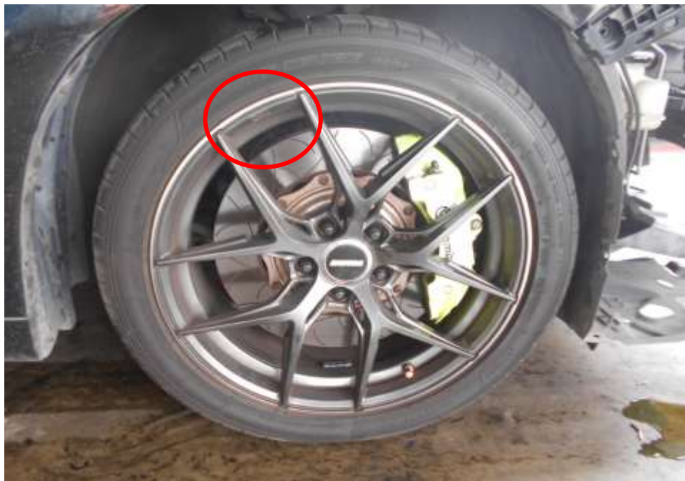
Photo 28 shows the non-standard rim and non- standard front brake kit found to be fitted on the Insured Vehicle at the time of our inspection. The 19- inch alloy rims fitted on the Insured Vehicle were not the standard type for the Insured Vehicle. The brand of the non- standard rims was 'TOMMI' (red circle).
