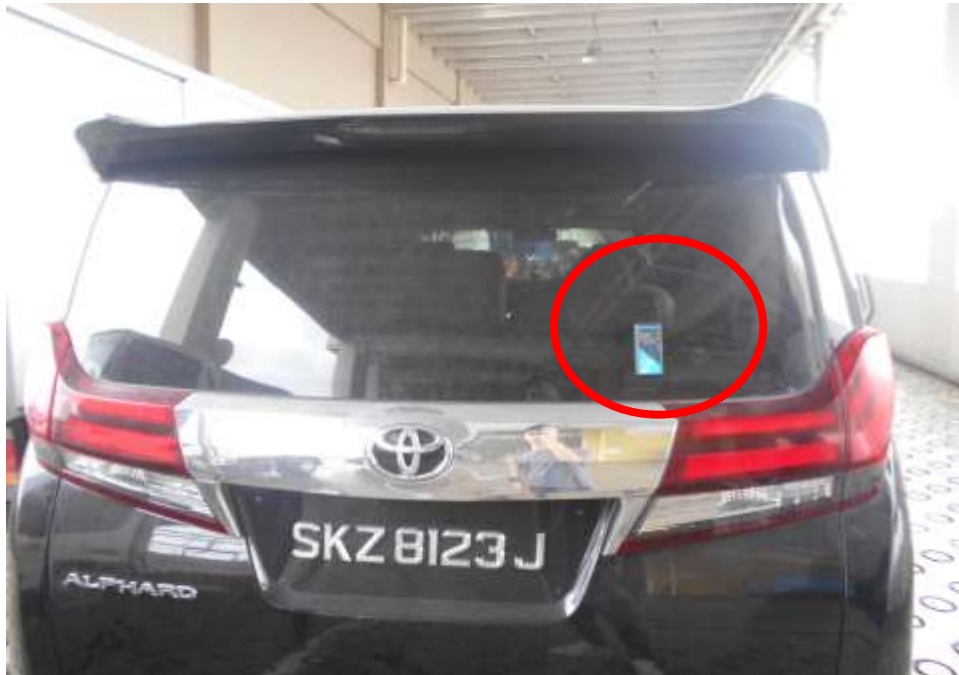
Photo 20 shows a general view of the measurement of the rear windscreen tint of the Insured Vehicle using a tint meter (red circle). Which measures the amount of Visible Light Transmission (VLT) that passes through a material. The Visible Light Transmission (VLT) measured on a scale of 0- 100%, with 0% meaning no light passes through and 100% meaning all light passes through.
