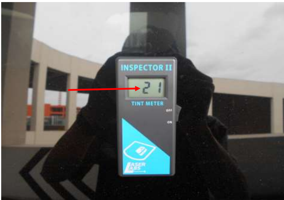
Photo 13 shows the window tint reading of the rear right side window on the Insured Vehicle at the time of my inspection. The rear right side window tint is measured at 21% (red arrow) Visible Light Transmission (VLT) which is not within LTA requirements, as 25% of light must be able to pass through the rear windscreen and two rear side windows.
