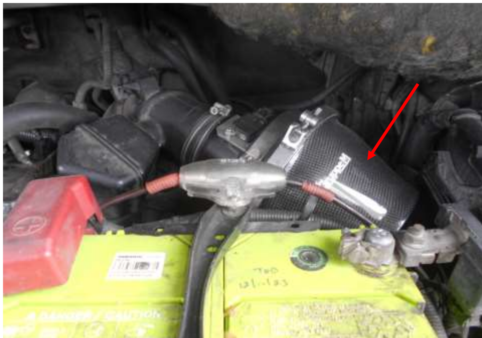
Photo 24 shows the general view close up view of the non- standard open pod air filter fitted onto the Insured Vehicle upon our inspection (arrowed).
