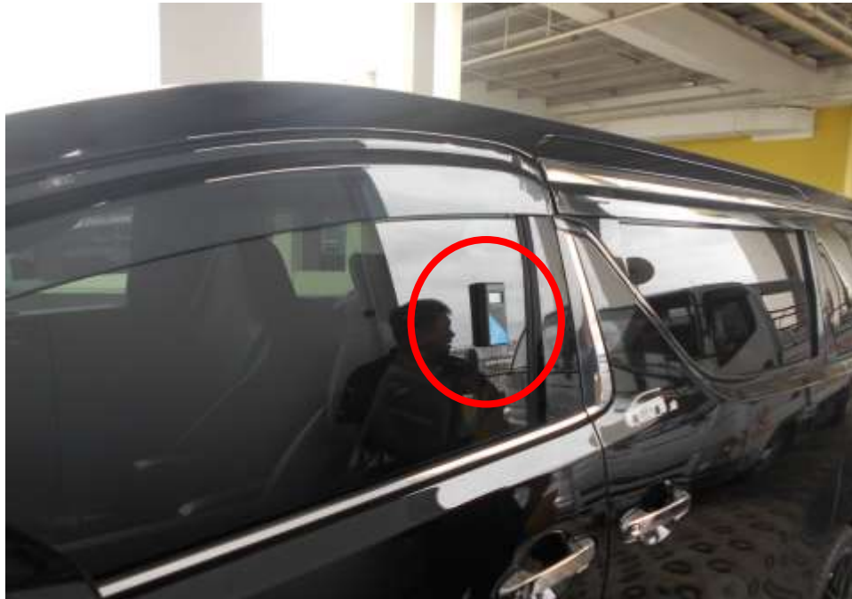
Photo 14 shows a general view of the measurement of the front left window tint of the Insured Vehicle using a tint meter (red circle). Which measures the amount of Visible Light Transmission (VLT) that passes through a material. The Visible Light Transmission (VLT) measured on a scale of 0- 100%, with 0% meaning no light passes through and 100% meaning all light passes through.
