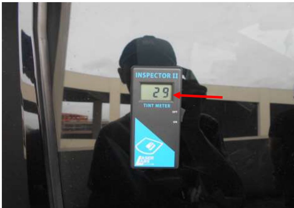
Photo 9 shows the window tint reading of the front right side window on the Insured Vehicle at the time of my inspection. The front right window tint is measured at 29% (red arrow) Visible Light Transmission (VLT) which is not within LTA requirements, as 70% of light must be able to pass through the front windscreen and two front side windows.
