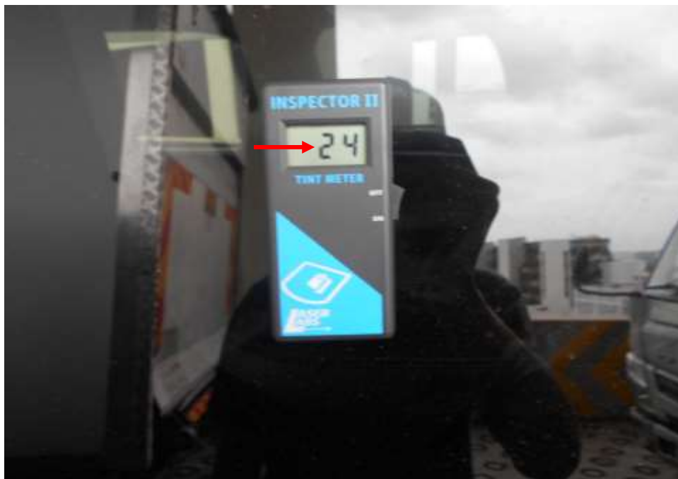
Photo 19 shows the window tint reading of the rear left side window on the Insured Vehicle at the time of my inspection. The rear left side window tint is measured 24% (red arrow) Visible Light Transmission (VLT) which is not within LTA requirements, as 25% of light must be able to pass through the rear windscreen and two rear side windows.
