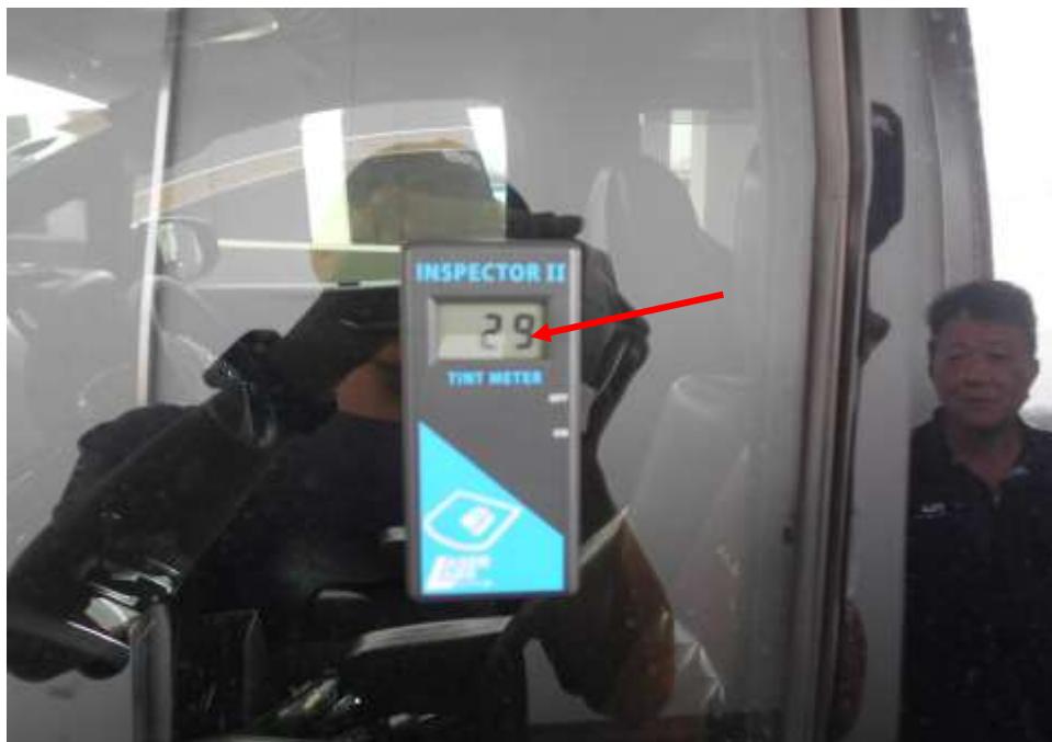
Photo 15 shows the window tint reading of the front left side window on the Insured Vehicle at the time of my inspection. The front left side window tint is measured at 5% (red arrow) Visible Light Transmission (VLT) which is not within LTA requirements, as 70% of light must be able to pass through the front windscreen and two front side windows.
