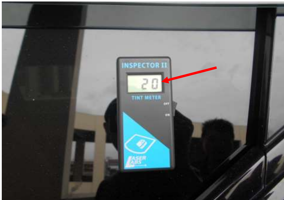
Photo 11 shows the window tint reading of the rear right side centre window on the Insured Vehicle at the time of my inspection. The rear right side window tint is measured at 20% (red arrow) Visible Light Transmission (VLT) which is not within LTA requirements, as 25% of light must be able to pass through the rear windscreen and two rear side windows.
