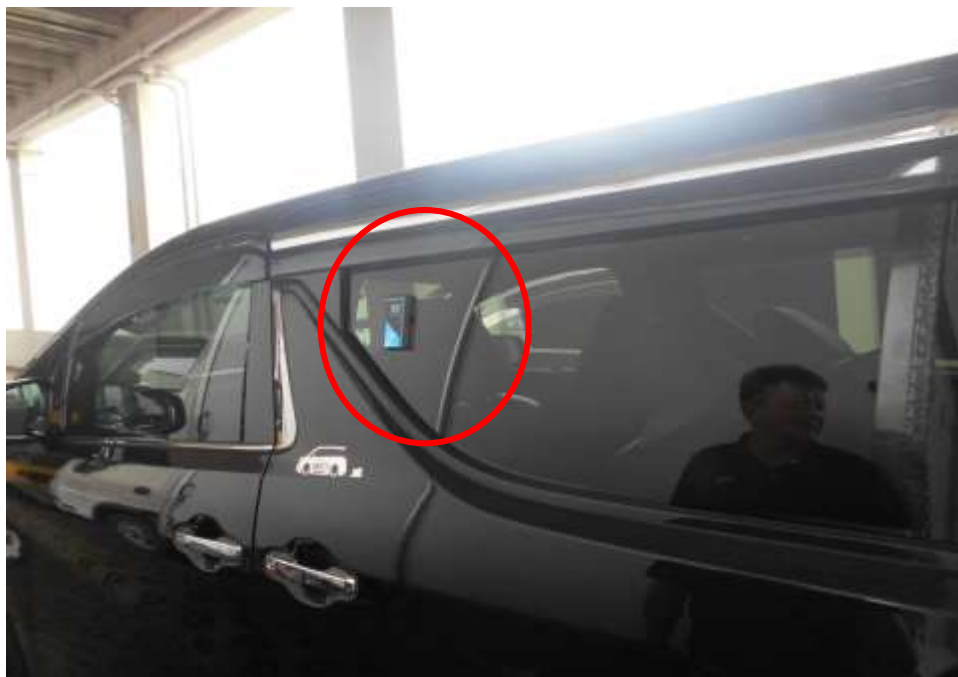
Photo 16 shows a general view of the measurement of the rear left centre window tint of the Insured Vehicle using a tint meter (red circle). Which measures the amount of Visible Light Transmission (VLT) that passes through a material. The Visible Light Transmission (VLT) measured on a scale of 0- 100%, with 0% meaning no light passes through and 100% meaning all light passes through.
