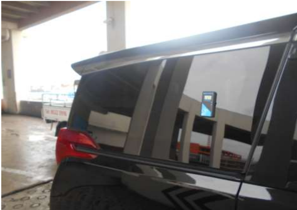
Photo 12 shows a general view of the measurement of the rear right window tint of the Insured Vehicle using a tint meter (red circle). Which measures the amount of Visible Light Transmission (VLT) that passes through a material. The Visible Light Transmission (VLT) measured on a scale of 0- 100%, with 0% meaning no light passes through and 100% meaning all light passes through.
