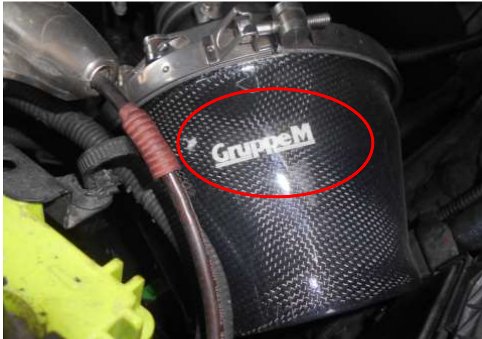
Photo 25 shows the close up view of the non- standard open pod air filter fitted onto the Insured Vehicle upon our inspection (circled). The brand of the open pod air filter was 'GruppeM' (circled).
