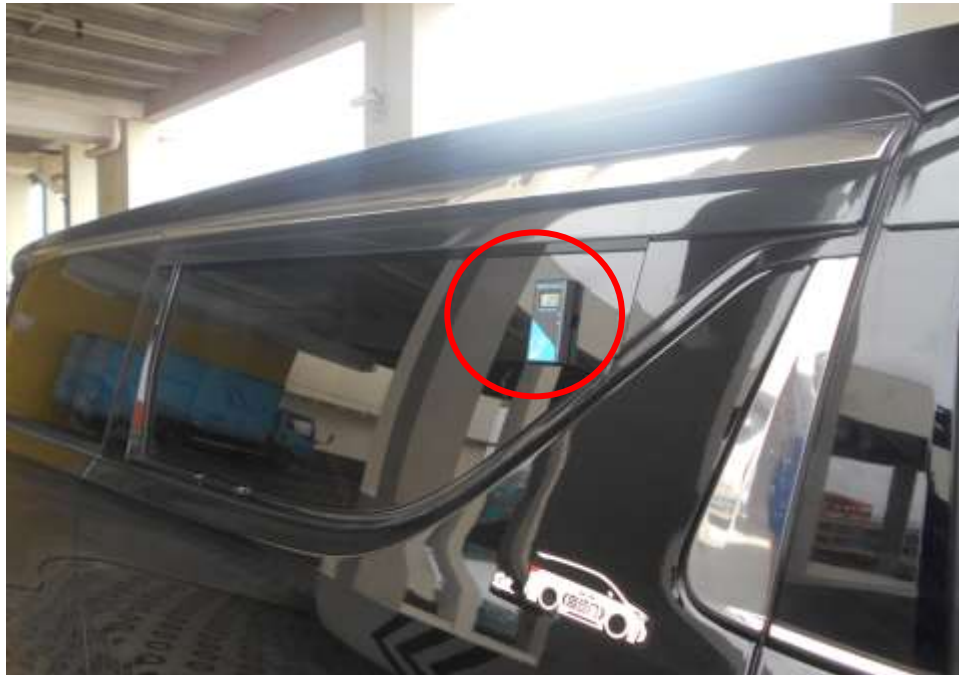
Photo 10 shows a general view of the measurement of the rear right centre window tint of the Insured Vehicle using a tint meter (red circle). Which measures the amount of Visible Light Transmission (VLT) that passes through a material. The Visible Light Transmission (VLT) measured on a scale of 0- 100%, with 0% meaning no light passes through and 100% meaning all light passes through.
