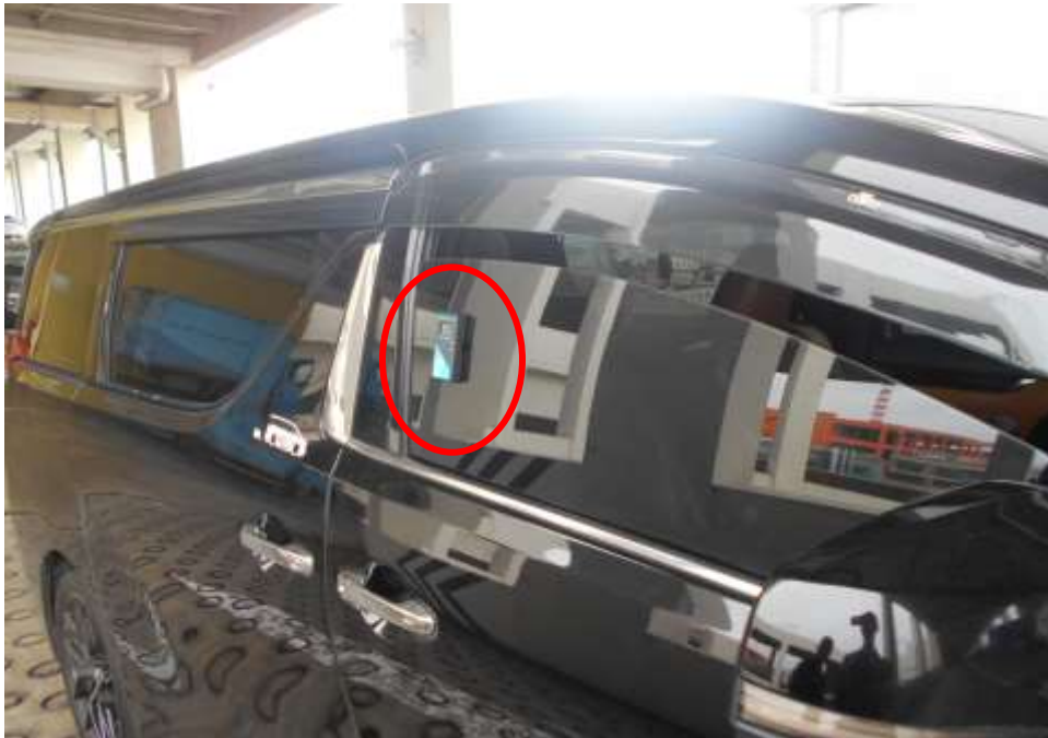
Photo 8 shows a general view of the measurement of the front right window tint of the Insured Vehicle using a tint meter (red circle). Which measures the amount of Visible Light Transmission (VLT) that passes through a material. The Visible Light Transmission (VLT) measured on a scale of 0- 100%, with 0% meaning no light passes through and 100% meaning all light passes through.
