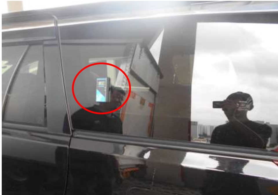
Photo 18 shows a general view of the measurement of the rear left window tint of the Insured Vehicle using a tint meter (red circle). Which measures the amount of Visible Light Transmission (VLT) that passes through a material. The Visible Light Transmission (VLT) measured on a scale of 0- 100%, with 0% meaning no light passes through and 100% meaning all light passes through.
