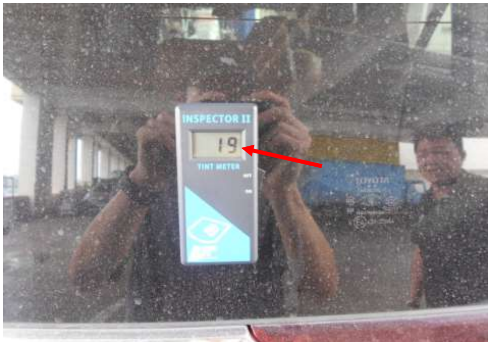
Photo 21 shows the window tint reading of the rear windscreen on the Insured Vehicle at the time of my inspection. The rear windscreen tint percentage is measured at 19% (red arrow) Visible Light Transmission (VLT) which is not within LTA requirements, as 25% of light must be able to pass through the rear windscreen and two rear side windows.
