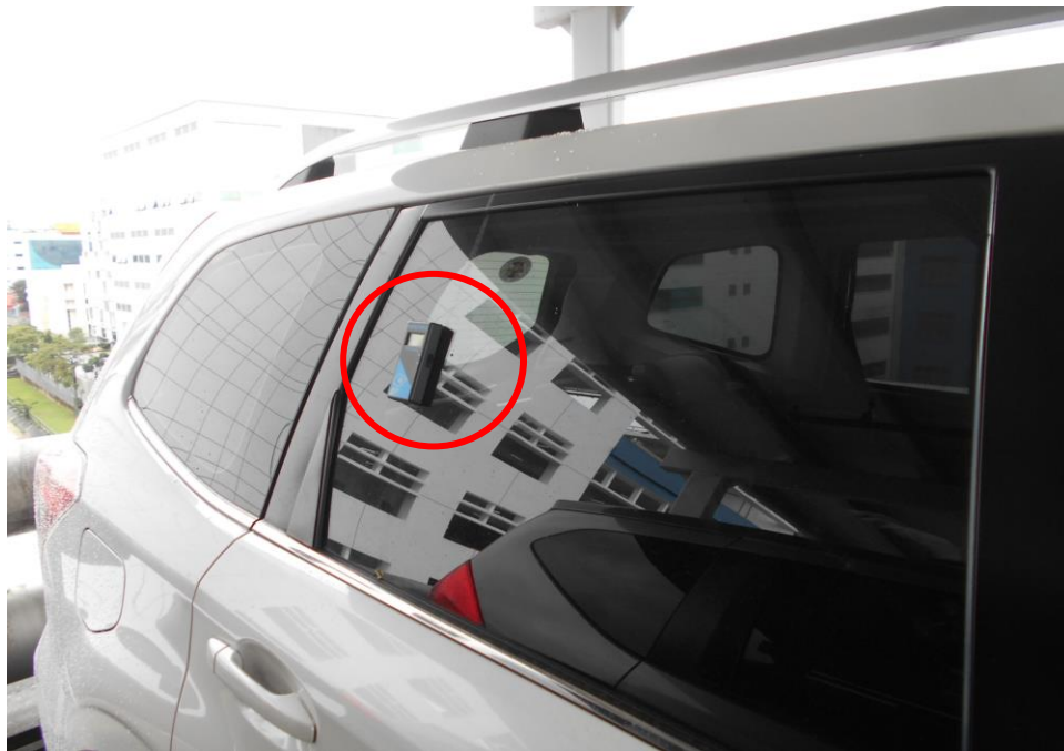
Photo 6 shows a general view of the measurement of the rear right window tint of the Insured Vehicle using a tint meter (red circle). Which measures the amount of Visible Light Transmission (VLT) that passes through a material. The Visible Light Transmission (VLT) measured on a scale of 0- 100%, with 0% meaning no light passes through and 100% meaning all light passes through.
