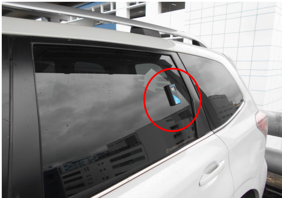
Photo 8 shows a general view of the measurement of the rear left window tint of the Insured Vehicle using a tint meter (red circle). Which measures the amount of Visible Light Transmission (VLT) that passes through a material. The Visible Light Transmission (VLT) measured on a scale of 0- 100%, with 0% meaning no light passes through and 100% meaning all light passes through.
