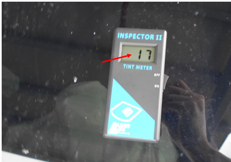
Photo 13 shows the window tint reading of the front windscreen on the Insured Vehicle at the time of my inspection. The front windscreen tint is measured at 17% (red arrow) Visible Light Transmission (VLT) which is not within LTA requirements, as 70% of light must be able to pass through the front windscreen and two front side windows.
