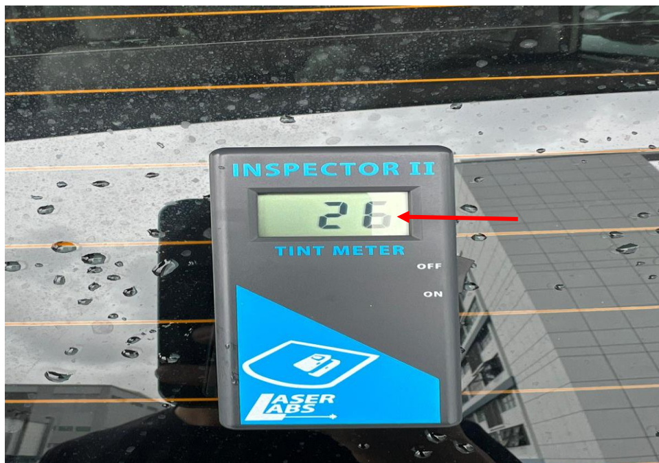
Photo 10 shows the window tint reading of the rear windscreen on the Insured Vehicle at the time of my inspection. The rear windscreen tint percentage is measured at 26% (red arrow) Visible Light Transmission (VLT) which is within the LTA requirements, as 25% of light must be able to pass through the rear windscreen and two rear side windows.
