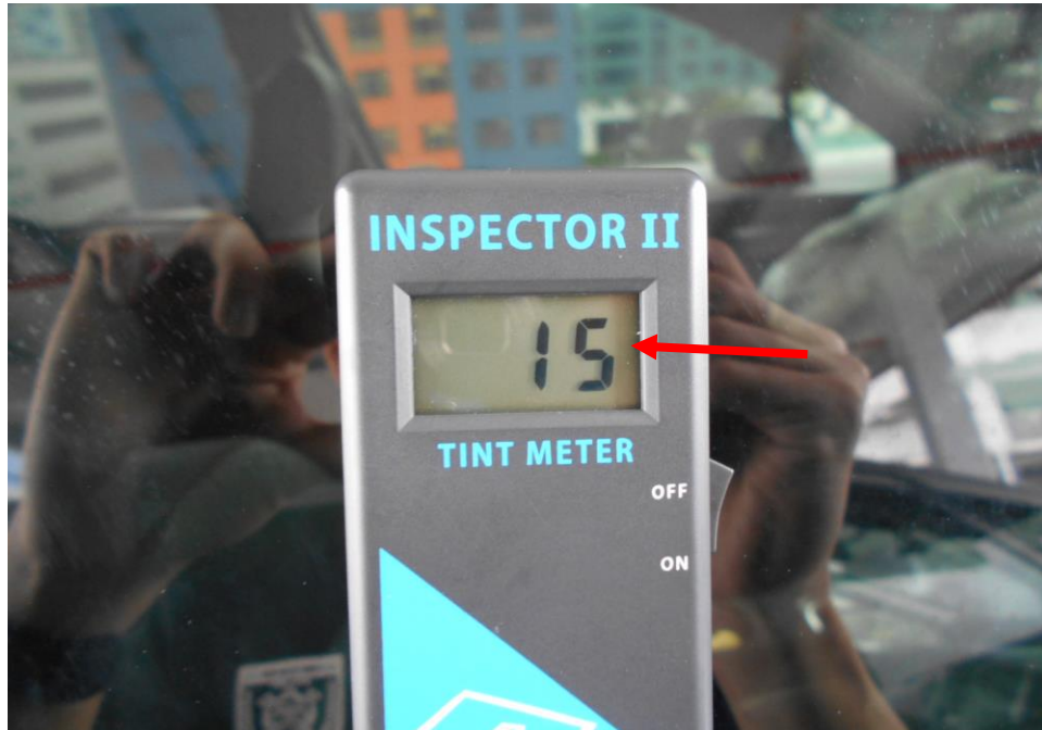
Photo 15 shows the window tint reading of the front right side window on the Insured Vehicle at the time of my inspection. The front right window tint is measured at 15% (red arrow) Visible Light Transmission (VLT) which is not within LTA requirements, as 70% of light must be able to pass through the front windscreen and two front side windows.
