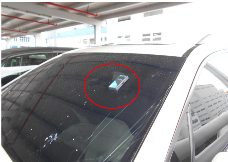
Photo 12 shows a general view of the measurement of the front windscreen tint of the Insured Vehicle using a tint meter (red circle) which measures the amount of Visible Light Transmission (VLT) that passes through a material. The Visible Light Transmission (VLT) measured on a scale of 0- 100%, with 0% meaning no light passes through and 100% meaning all light passes through.
