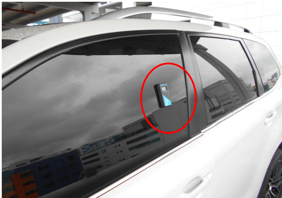
Photo 16 shows a general view of the measurement of the front left window tint of the Insured Vehicle using a tint meter (red circle). Which measures the amount
