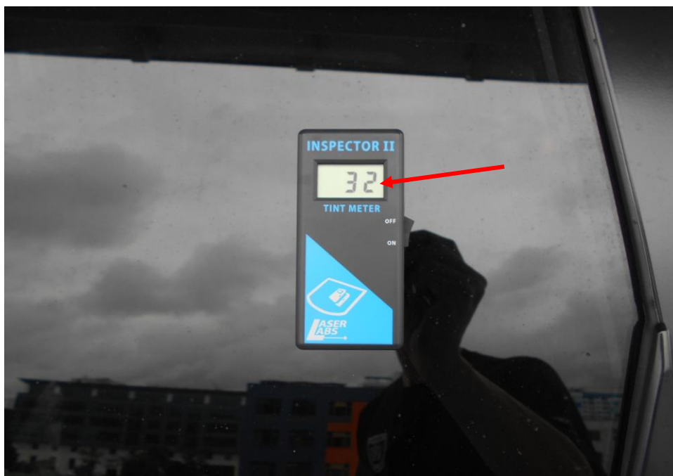
Photo 9 shows the window tint reading of the rear left side window on the Insured Vehicle at the time of my inspection. The rear right side window tint is measured at 32% (red arrow) Visible Light Transmission (VLT) which is within the
