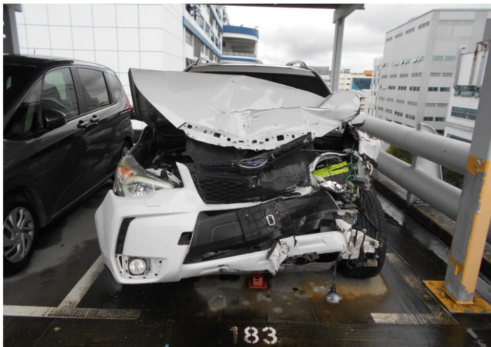
Photo 1 shows a general view of the Insured Vehicle front portion at the time of my inspection. The Insured Vehicle was observed to have sustained damage at its front portion. Its front windscreen, front bonnet, front headlamps and front bumper was amongst the body parts damaged as a result of the accident.
