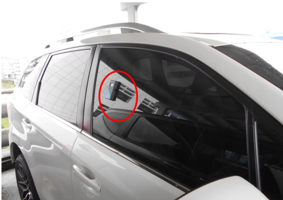
Photo 14 shows a general view of the measurement of the front right window tint of the Insured Vehicle using a tint meter (red circle). Which measures the amount
