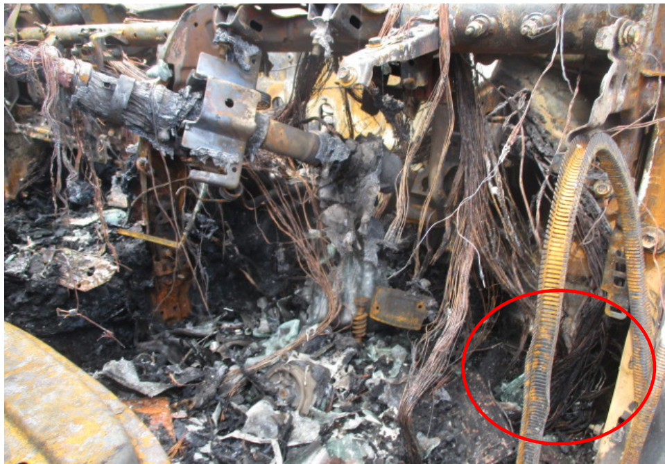
Photo 7 shows the wirings around the right bottom portion of the driver dashboard panel, which is in the immediate vicinity where the fire to the Insured Vehicle had likely started. We noticed faint traces of greenish residue on several stretches of burnt wirings (circled). The presence of greenish residue indicates internal heating of copper wires, a sign of an electrical short circuit occurring.
