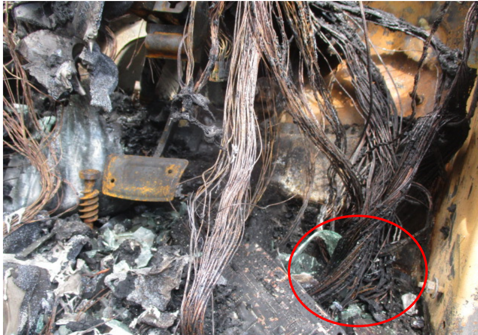
Photo 8 shows a closer view of the burnt wirings around the right bottom portion of the driver dashboard panel. We noticed faint traces of greenish residue on several stretches of the burnt wirings (circled). The greenish residue is normally left behind from oxidation as a result of chemical reaction involving the copper wires.
