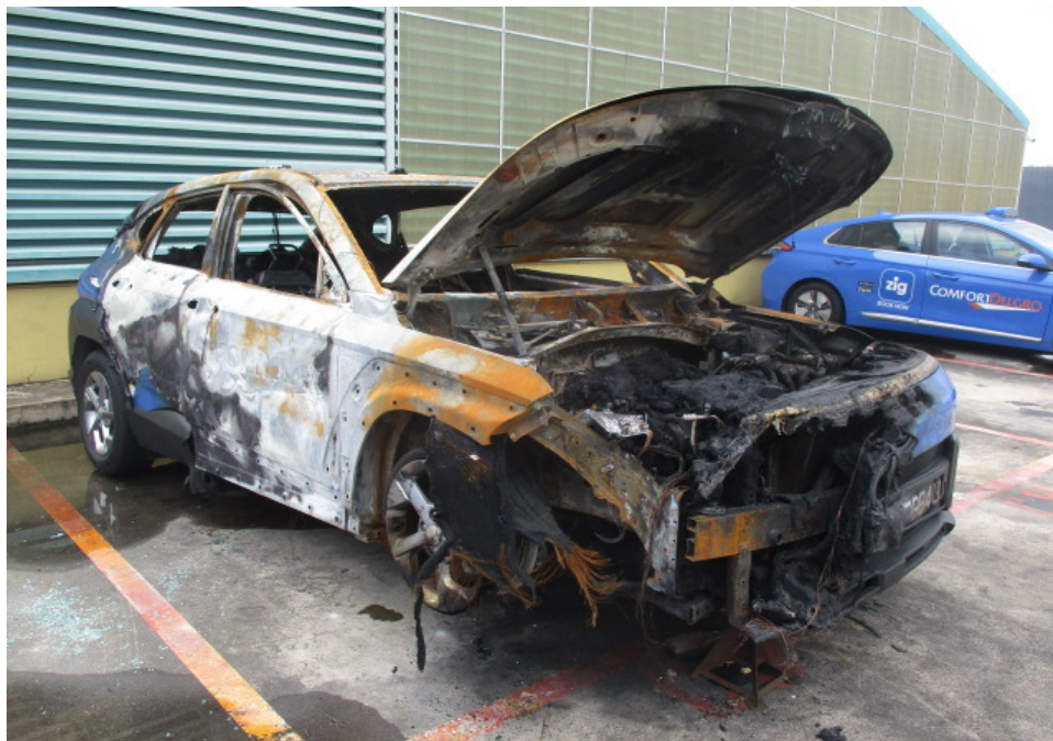
Photo 3 shows the closer view of the right front body of the Insured Vehicle at the time of our inspection. The fire damage to the Insured Vehicle was confined to its frontal portion, left body and right body. Its front bumper, front bonnet, front support panel, front grille, front headlamps, front windscreen, front wheel rims, left body, right body and front tyres were amongst the body parts that were found to have been affected by the fire.
