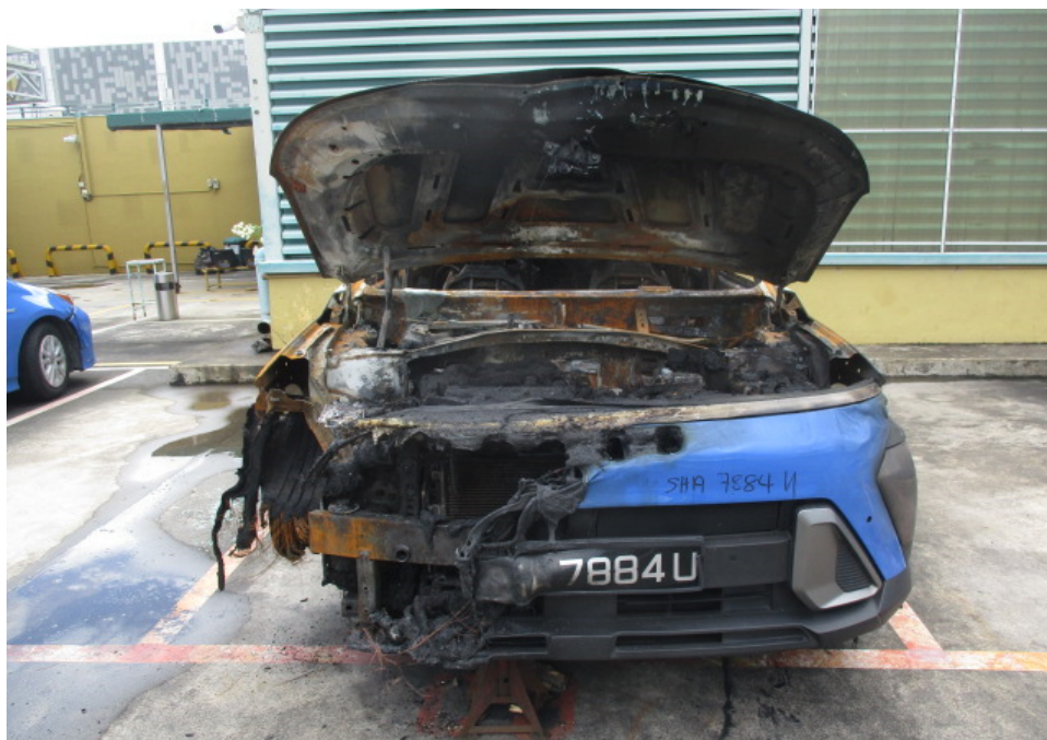
Photo 2 shows the general view of the frontal portion of the Insured Vehicle at the time of our inspection. The fire damage to the Insured Vehicle was confined to its frontal portion, left body and right body. The entire engine compartment of the Insured Vehicle was observed to be severely burnt while the interior compartment was observed to be severely affected by the fire.
