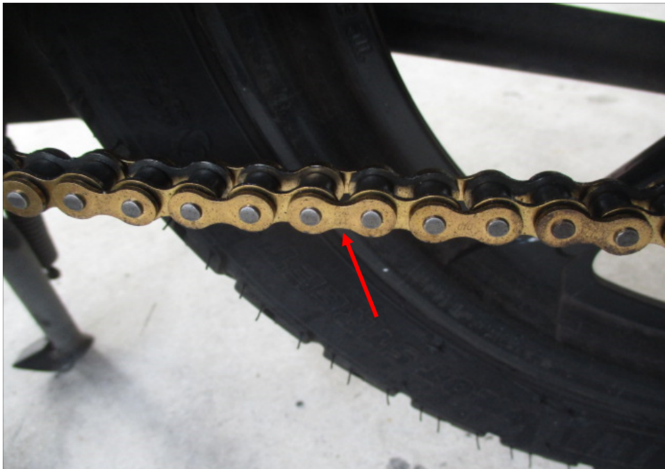
Photo 24 shows the closer view of the gear train (arrowed) of the Motorcycle, which was observed to be intact with no misalignment. It was also adequately lubricated for operating purposes.
