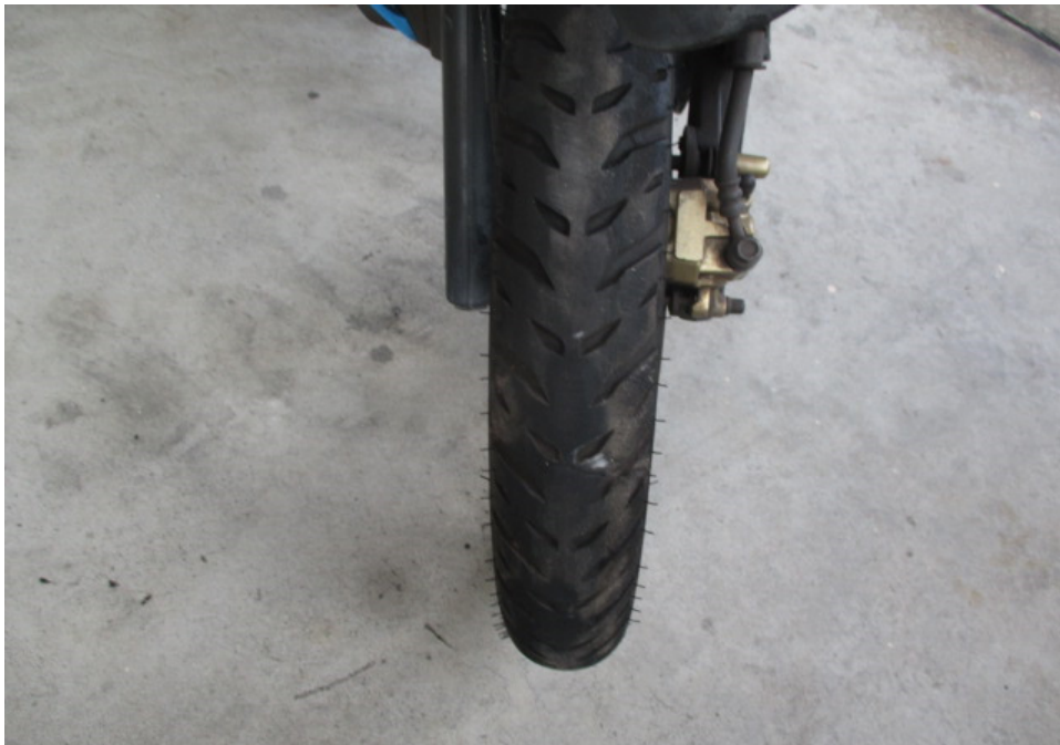
Photo 19 shows the condition of the Motorcycle's front tyre. The front tyre was observed to be in serviceable condition with remaining tread depth of approximately 3mm. There was no tear, burst mark(s) and/or punctured hole(s) on the sidewalls as well as across the tread of the front tyre. The front tyre was also observed to be sufficiently inflated for vehicular operation.
