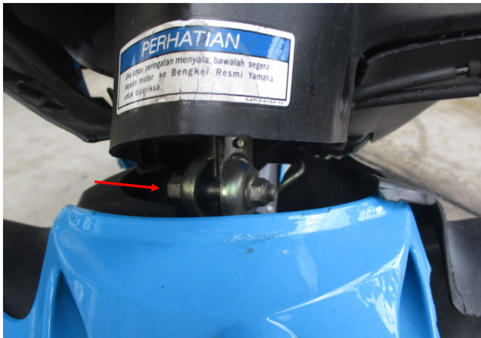
Photo 26 shows a close up view of the bent steering stem of the Motorcycle most likely as a result of the accident (arrowed). We were hence not able to conduct any tests on the steering system of the Motorcycle.
