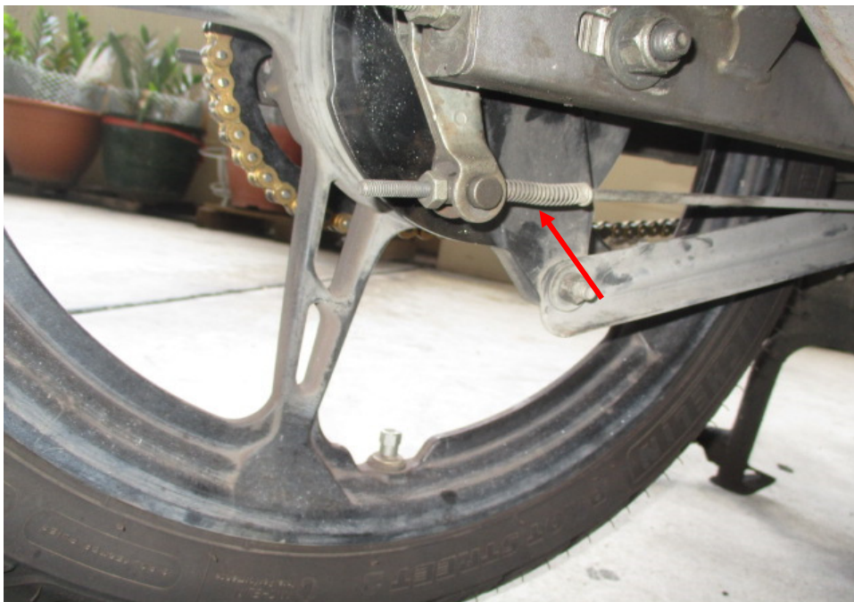
Photo 30 shows the rear wheel of the Motorcycle. The type of brake system for the rear wheel was of a mechanical type, controlled by the brake foot pedal of the Motorcycle. Our checks of the cable (arrowed), spring and drum which are all part of the components in the rear brake system of the Motorcycle reveal all to be intact and without damage.
