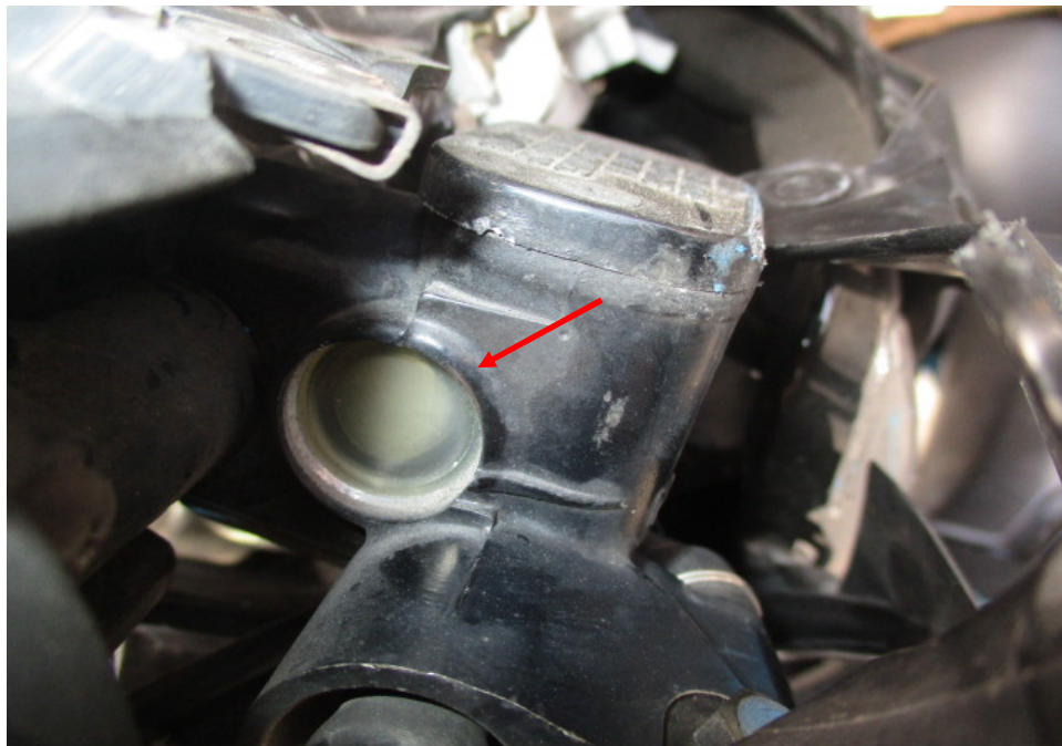
Photo 28 shows the brake fluid reservoir for the front brake of the Motorcycle. The brake fluid was found to be of sufficient level for operating purposes (arrowed).
