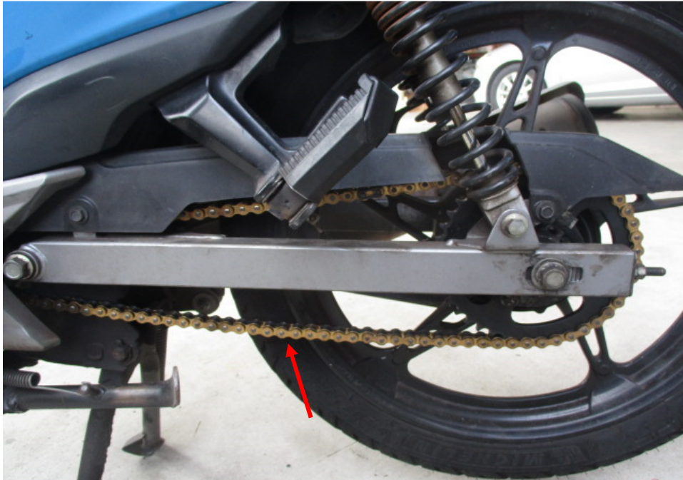
Photo 23 shows the gear train (arrowed) of the Motorcycle, which was observed to be intact with no misalignment. It was also adequately lubricated for operating purposes. The gear train rotates the rear wheel of the Motorcycle.
