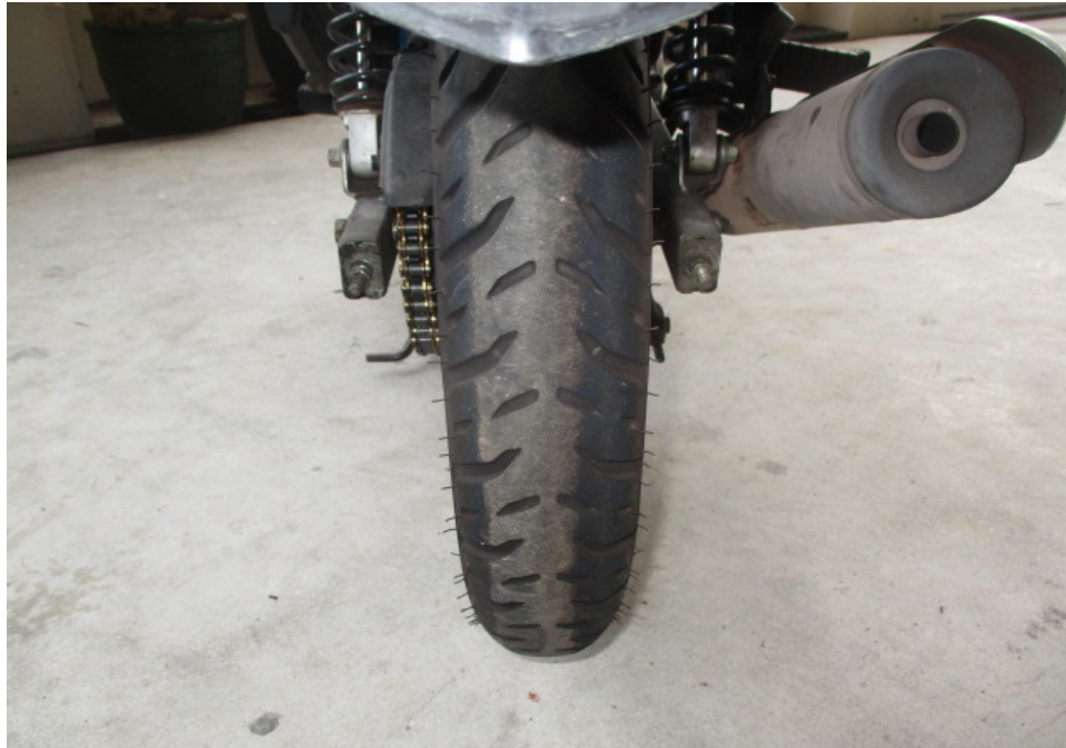
Photo 20 shows the condition of the Motorcycle's rear tyre. The rear tyre was observed to be in serviceable condition with remaining tread depth of approximately 3mm. We did not observe any tear, burst mark(s) and/or punctured hole(s) on the sidewalls as well as across the tread of the rear tyre. The rear tyre was also observed to be sufficiently inflated for vehicular operation.
