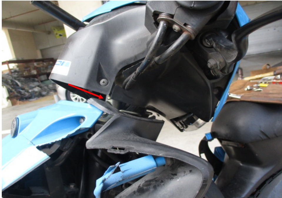
Photo 25 shows the steering stem of the Motorcycle. The steering stem was observed to be bent most likely as a result of the accident (arrowed). We were hence not able to conduct any tests on the steering system of the Motorcycle.
