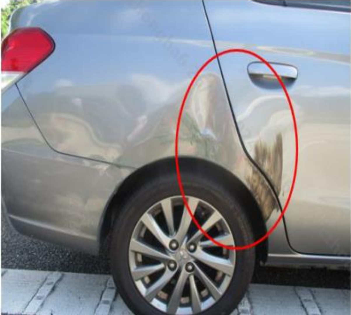
Figure B-10: Close-up View of Damaged Area of SLW 8727X Damage Assessment: Civilian Car right hand rear dented
